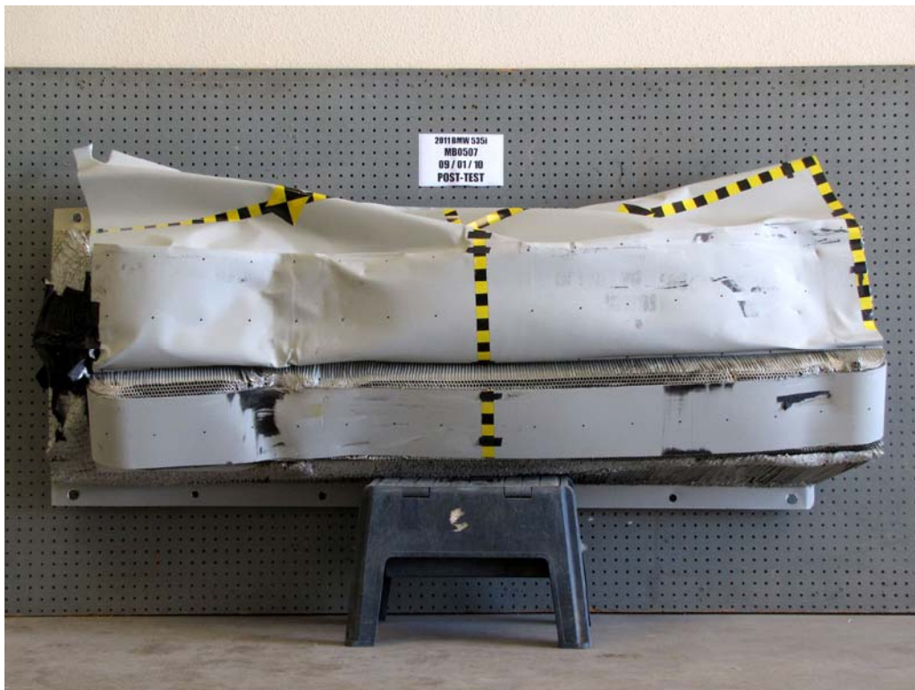
FIGURE 82. Post-Test Front View of MDB Impactor Face
