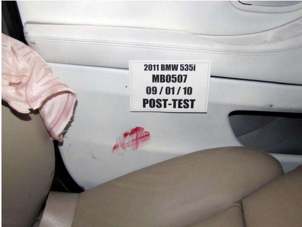
FIGURE 51. Post-Test Driver Dummy Close-Up Pelvis Contact
