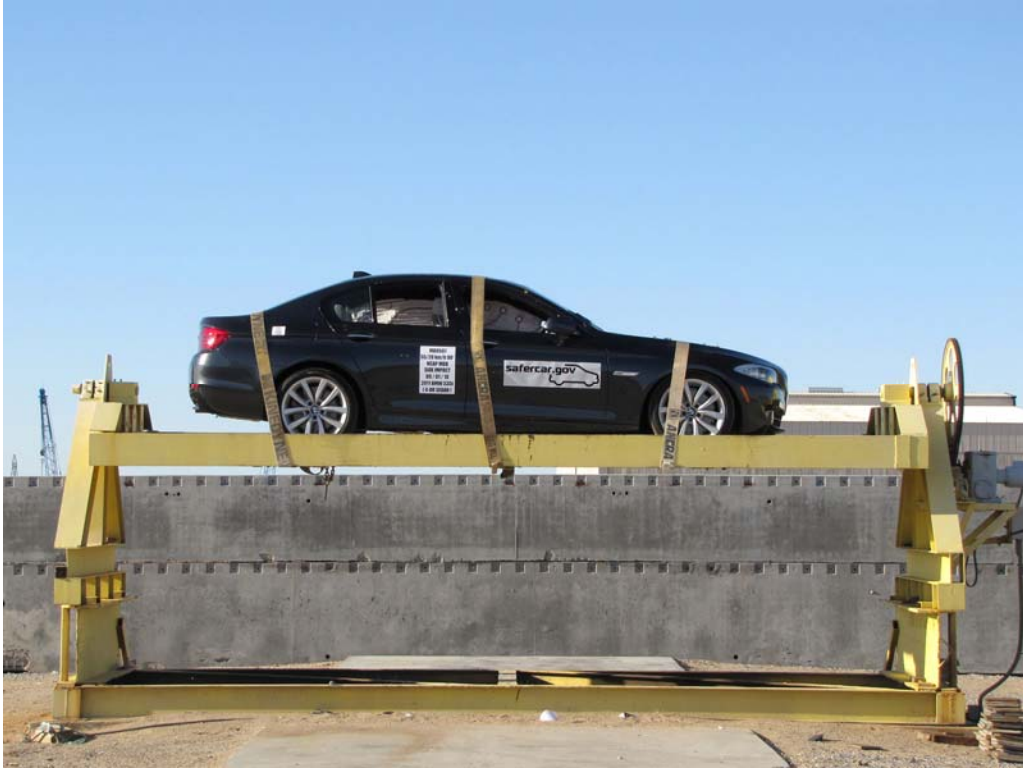
FIGURE 93. FMVSS No. 301-305 Rollover 0 Degrees
