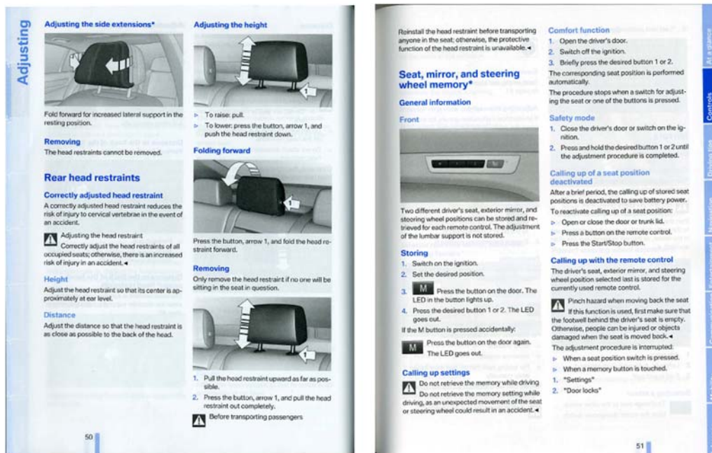
FIGURE 101. Left Rear Passenger Head Restraint Use and Adjustment Information from Vehicle Manual
