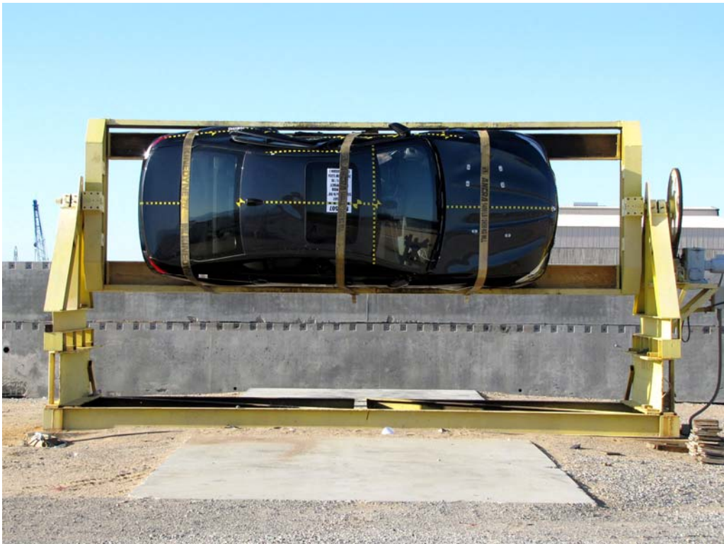
FIGURE 94. FMVSS No. 301-305 Rollover 90 Degrees
