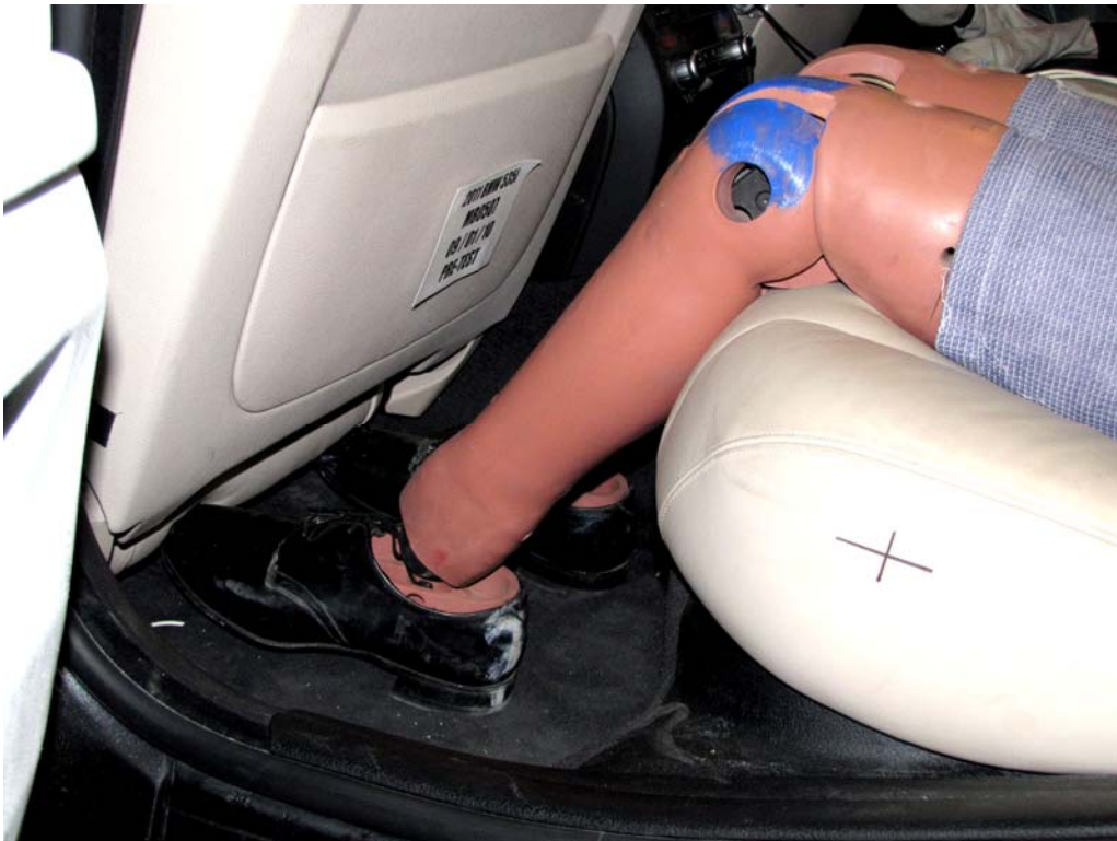
FIGURE 62. Pre-Test Placement of Rear Passenger Dummy's Feet
