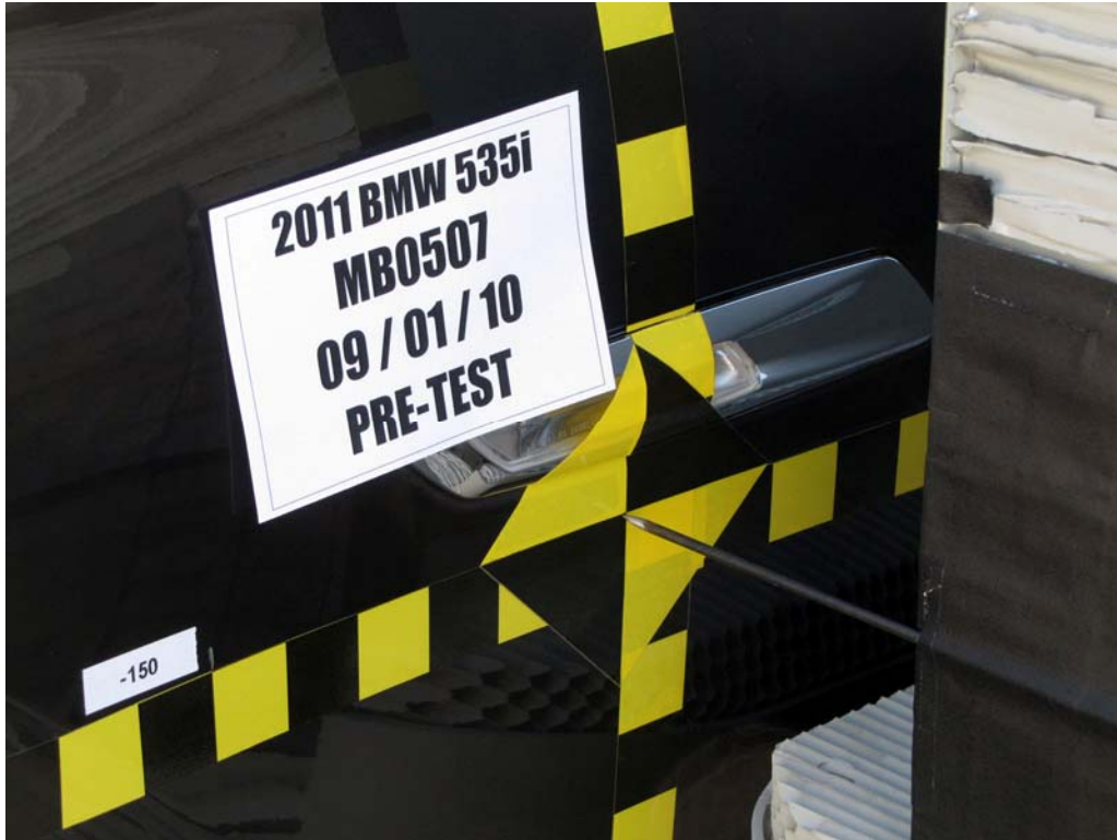
FIGURE 19. Pre-Test Close-Up View of Impact Point Target
