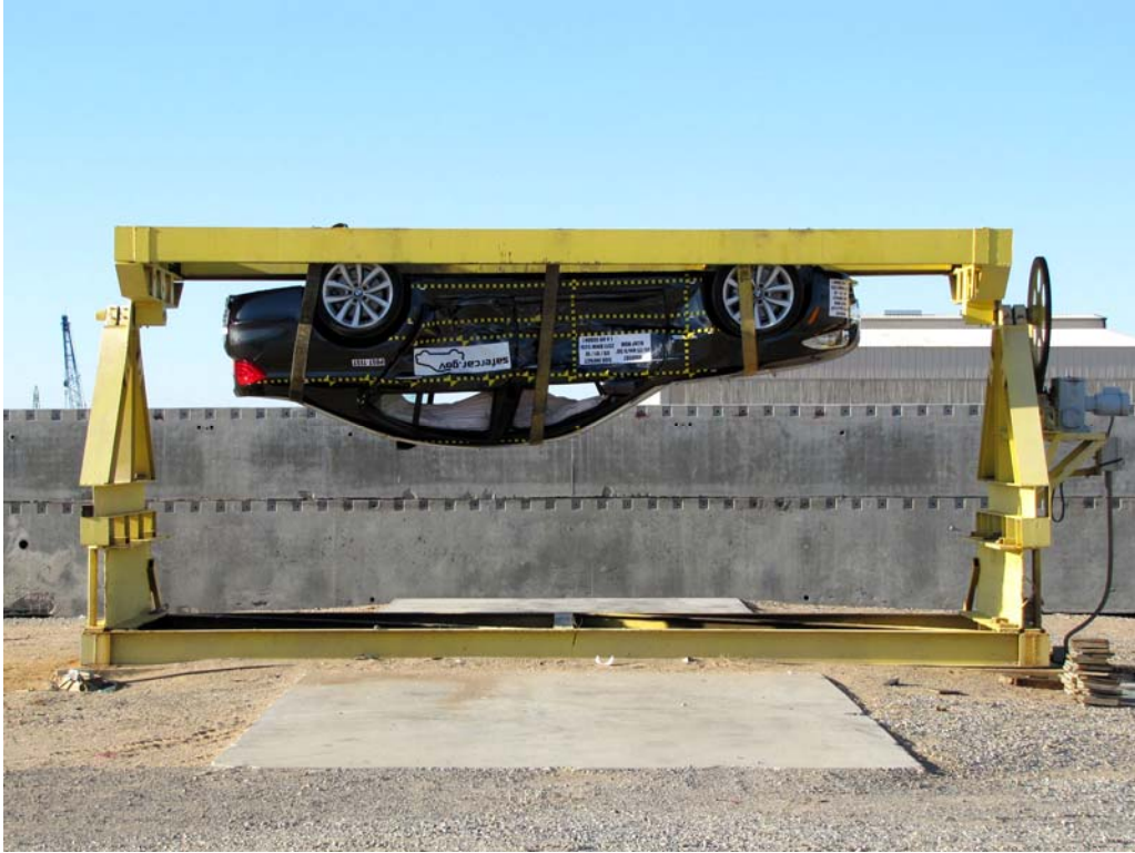
FIGURE 95. FMVSS No. 301-305 Rollover 180 Degrees
