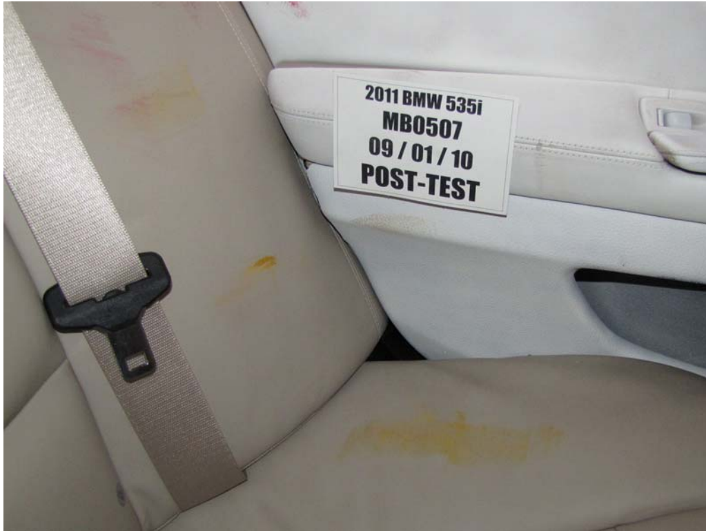
FIGURE 77. Post-Test Rear Passenger Dummy Close-Up Pelvis Contact View
