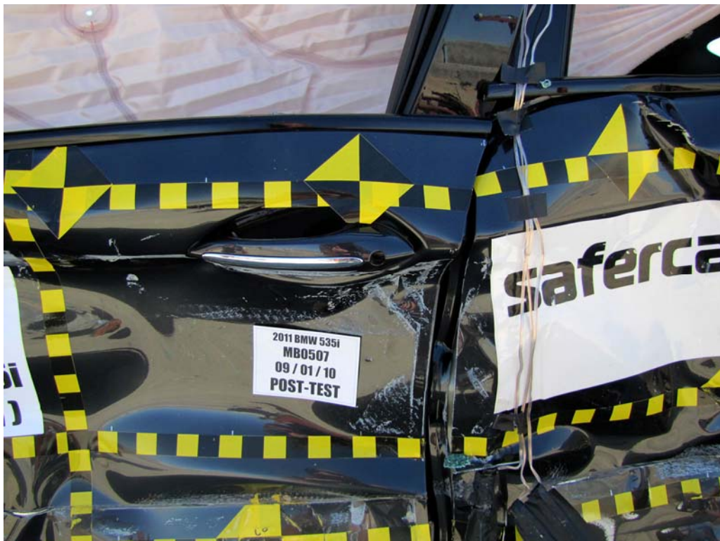
FIGURE 22. Post-Test Left Front Door Latch Close-Up
