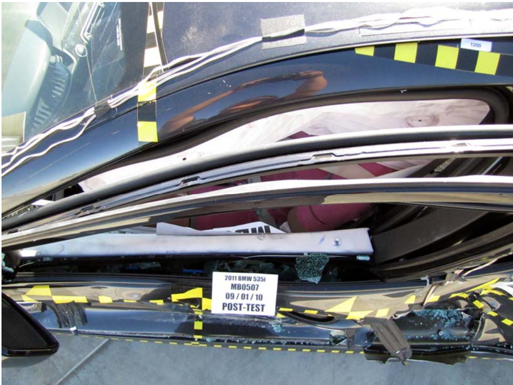
FIGURE 42. Post-Test Driver Dummy and Door Clearance View
