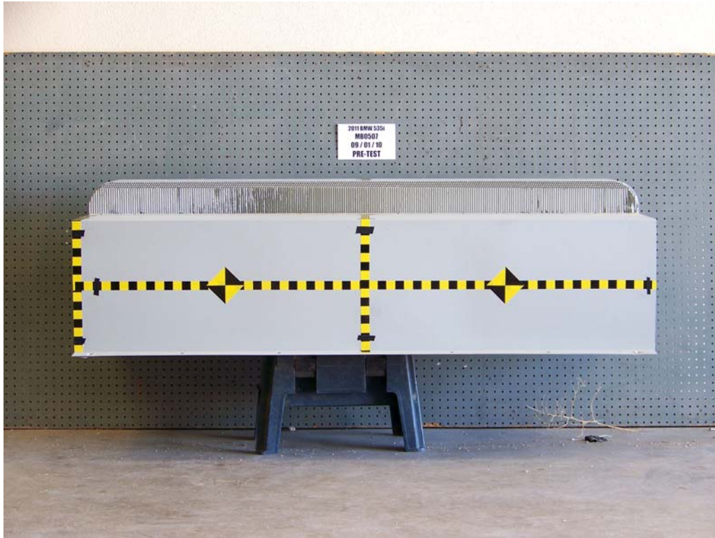
FIGURE 83. Pre-Test Top View of MDB Impactor Face
