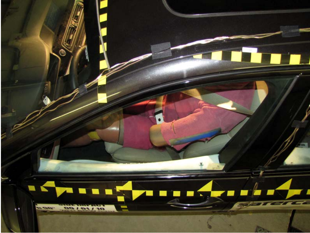
FIGURE 41. Pre-Test Driver Dummy and Door Clearance View
