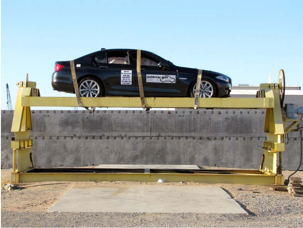
FIGURE 97. FMVSS No. 301-305 Rollover 360 Degrees
