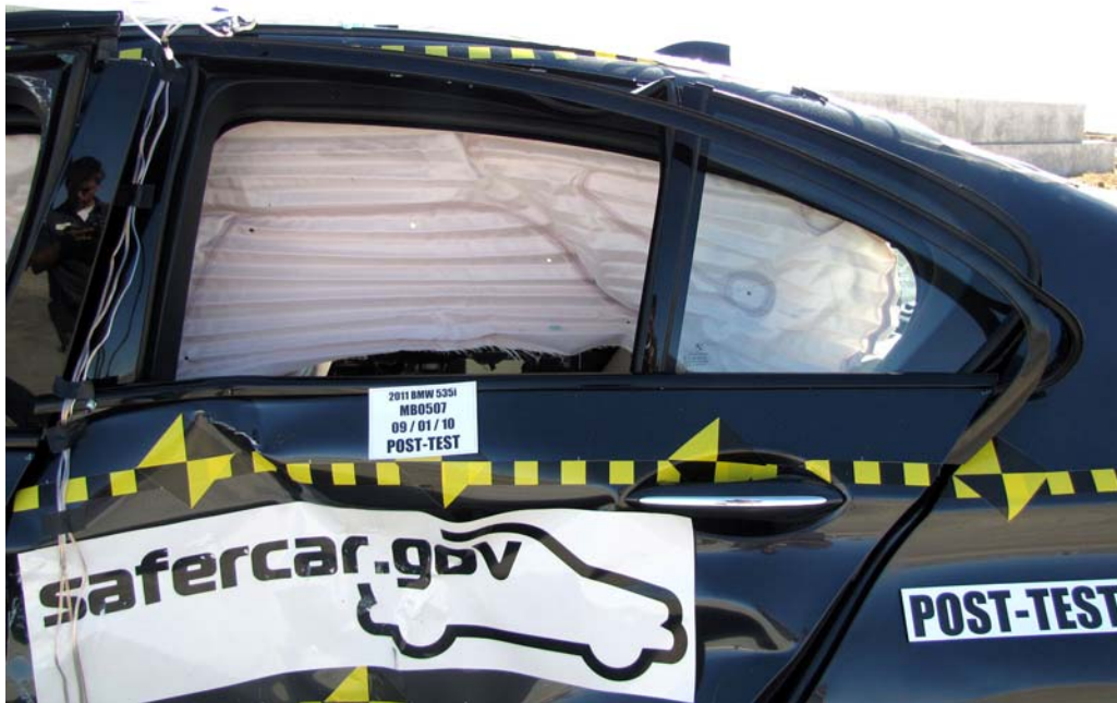
FIGURE 55. Post-Test Left Side View of Rear Passenger Dummy Shoulder and Door Top View
