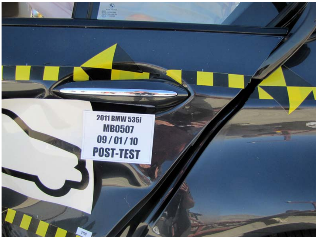
FIGURE 24. Post-Test Left Rear Door Latch Close-Up
