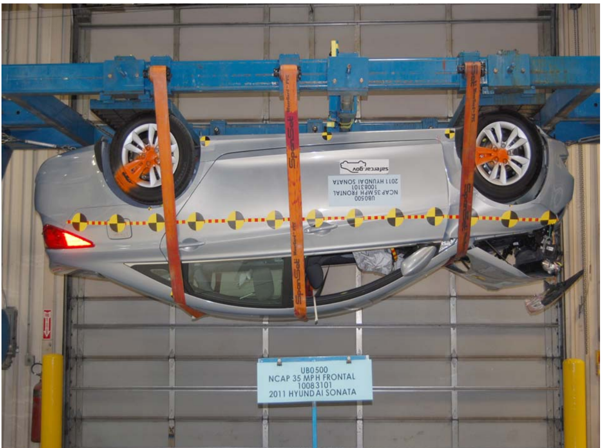
Vehicle at 180 Degrees on Static Rollover Device
