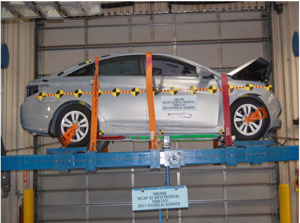
Vehicle at 360 Degrees on Static Rollover Device
