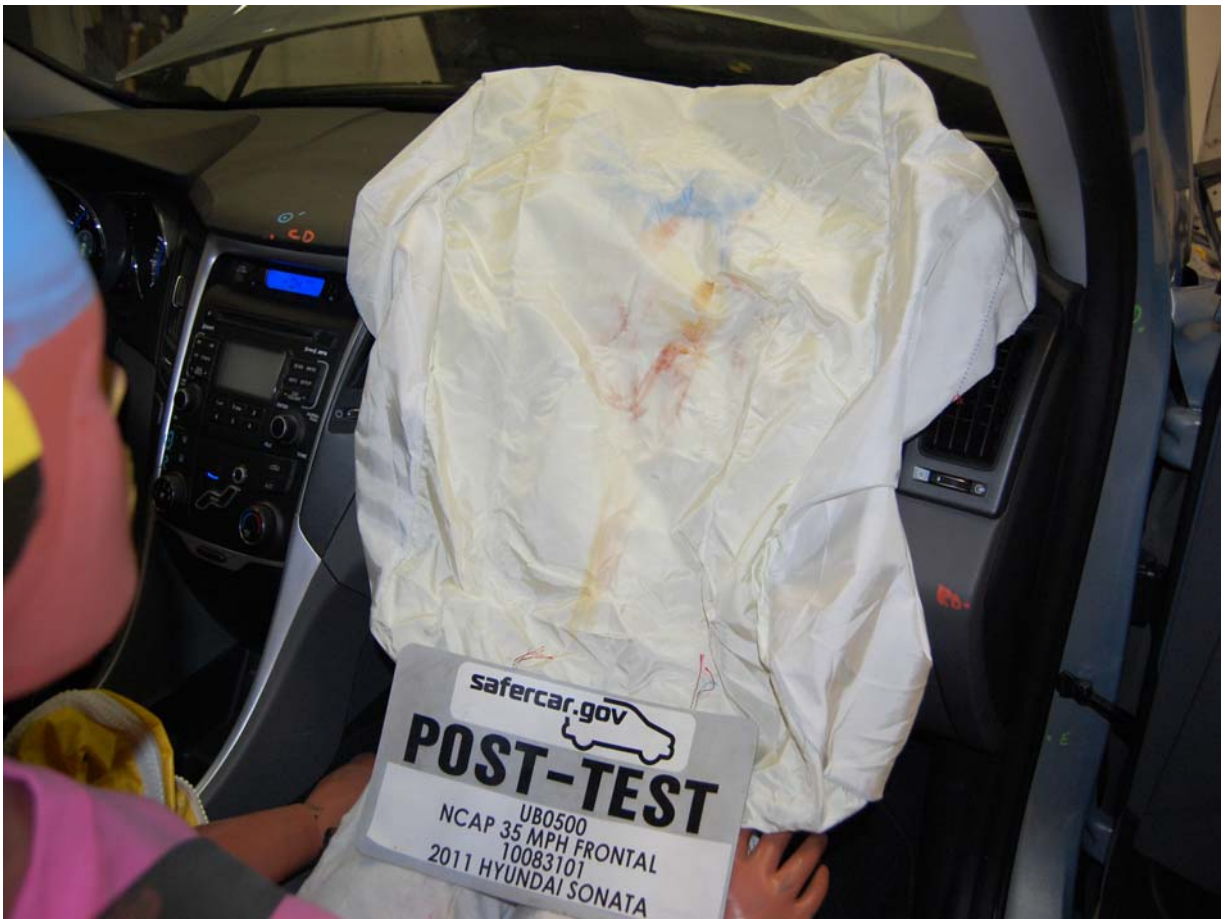
Post-Test Passenger Dummy Contact with Airbag
