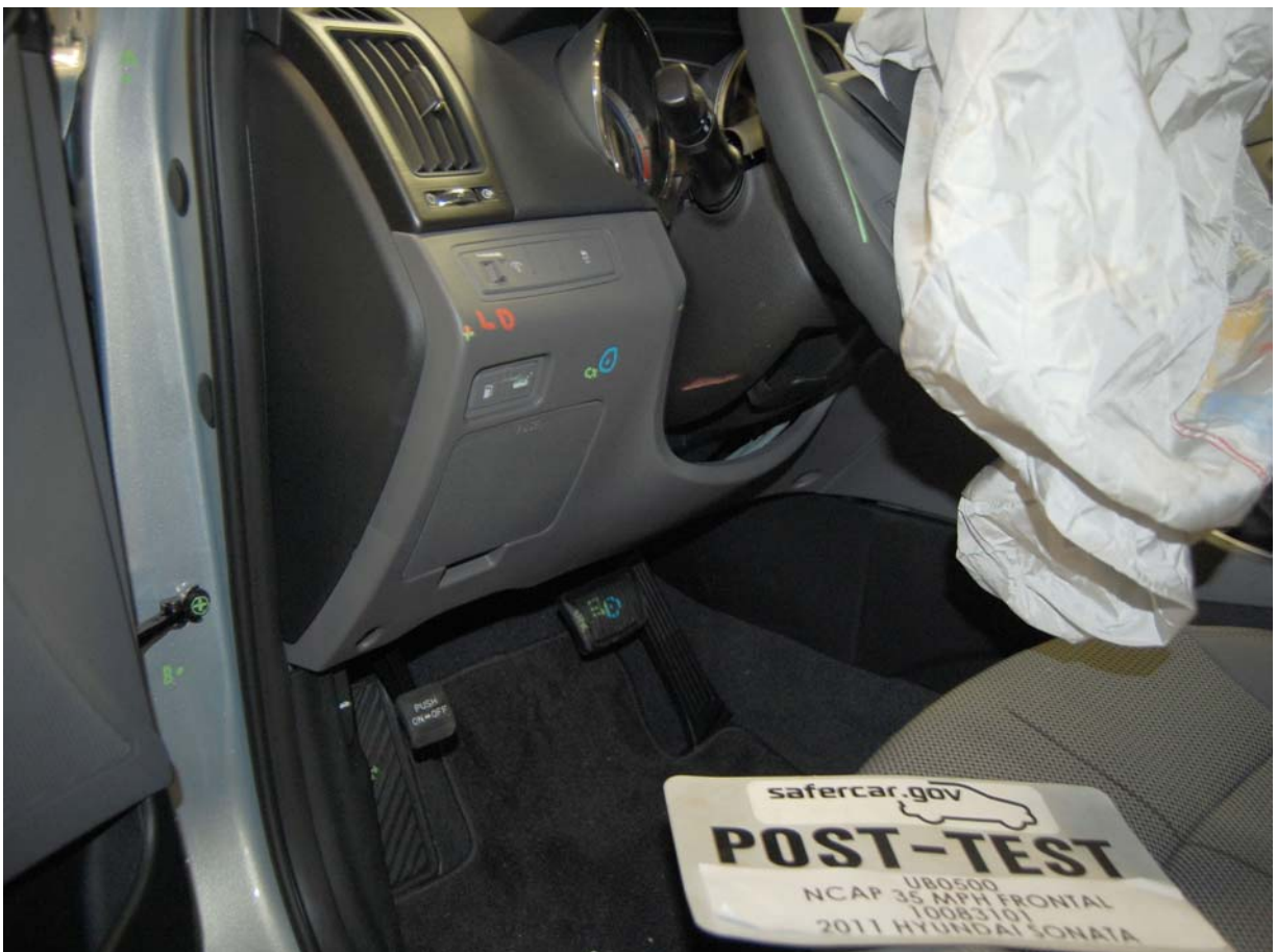
Post-Test Driver's Side Knee Bolster (without dummy)
