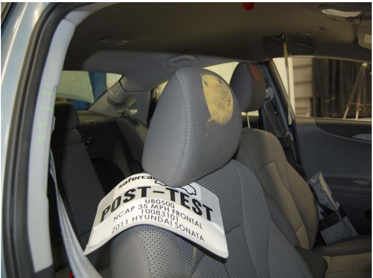
Post-Test Passenger Dummy Contact with Headrest
