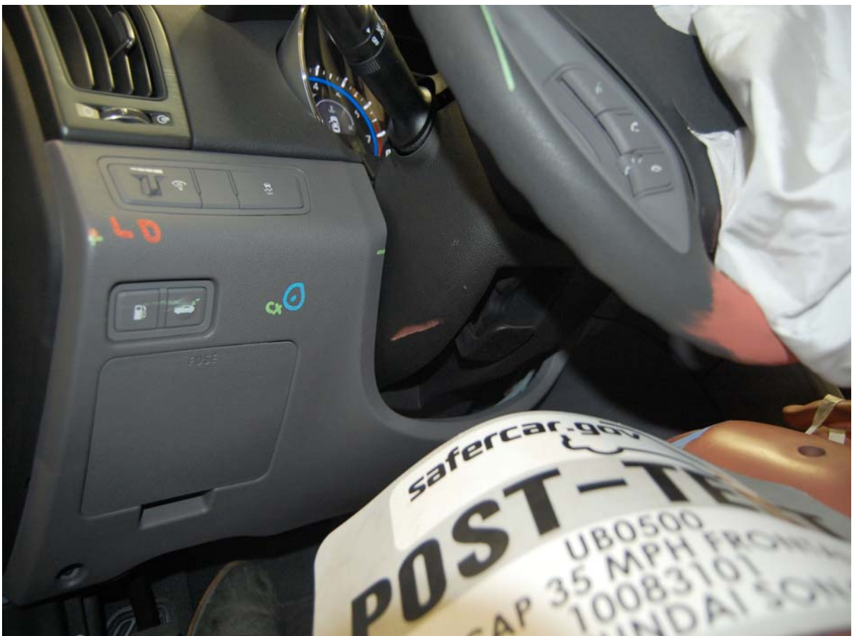
Post-Test View of Steering Column Shear Capsule
