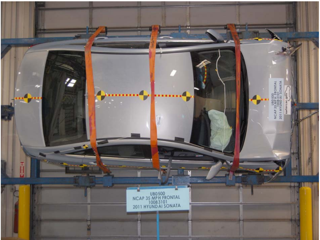
Vehicle at 270 Degrees on Static Rollover Device
