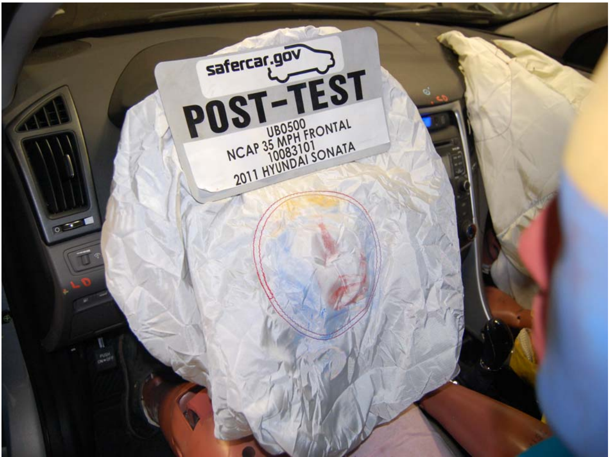
Post-Test Driver Dummy Contact with Airbag
