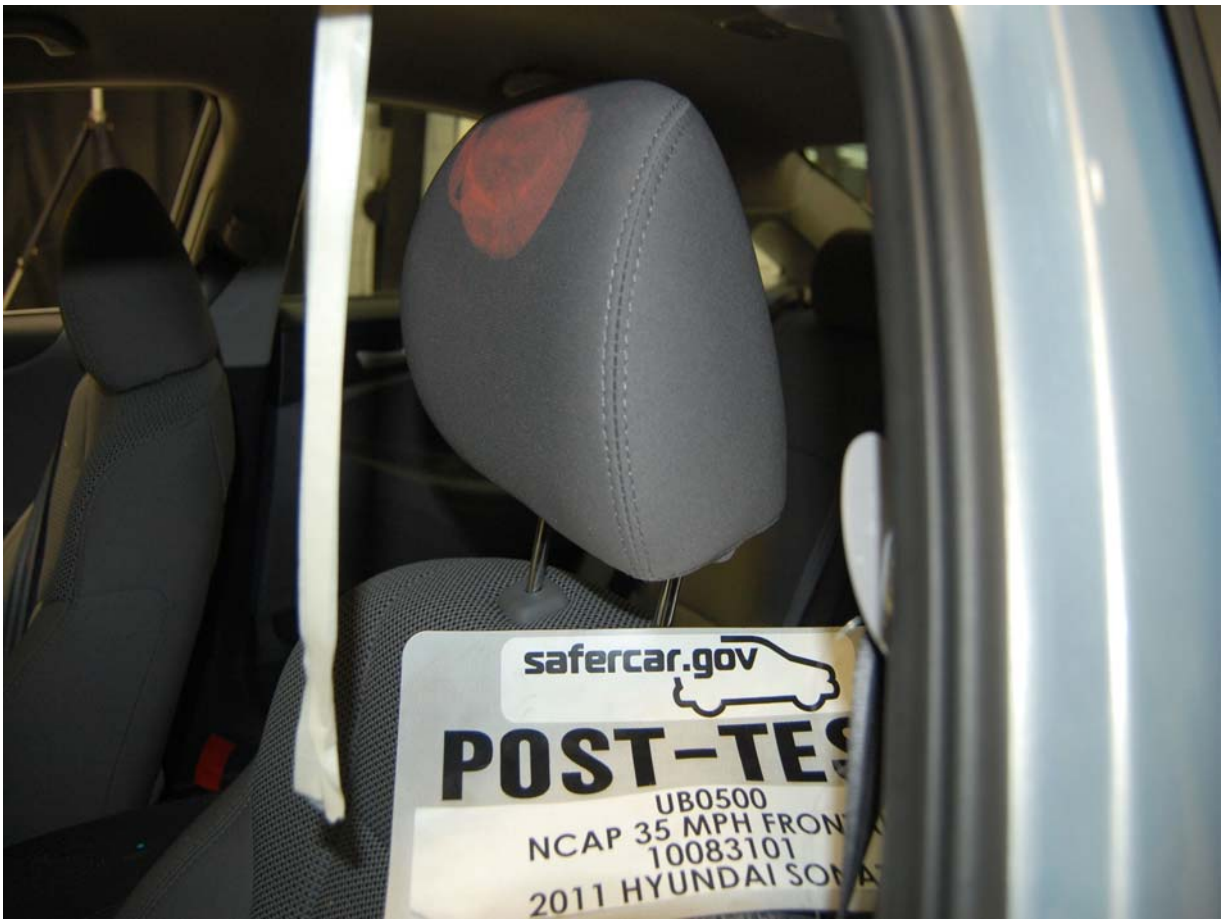
Post-Test Driver Dummy Contact with Headrest
