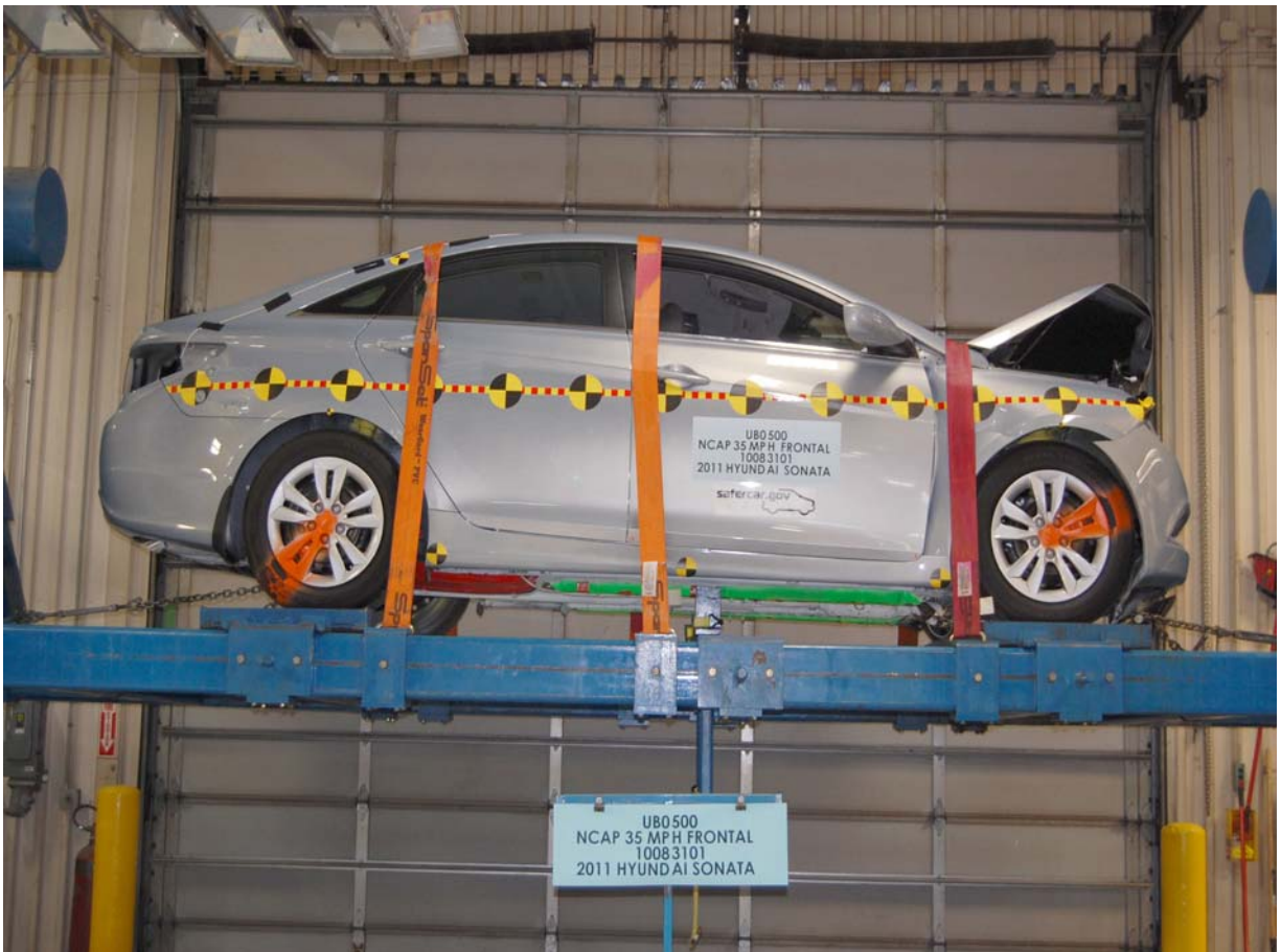
Vehicle at 0 Degrees on Static Rollover Device
