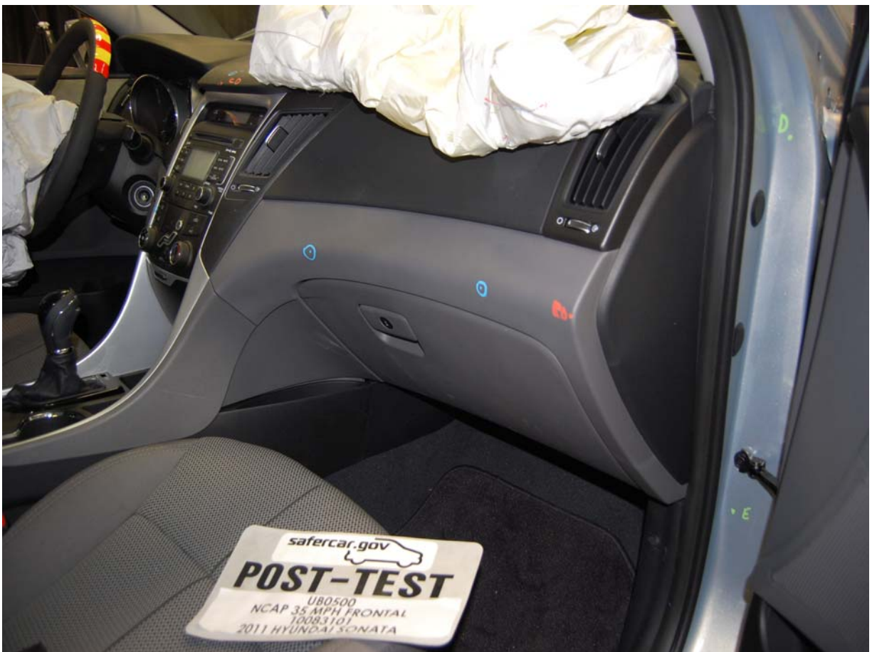
Post-Test Passenger's Side Knee Bolster (without dummy)
