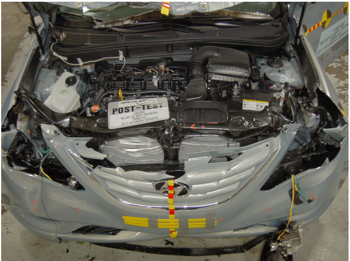
Post-Test Engine Compartment View
