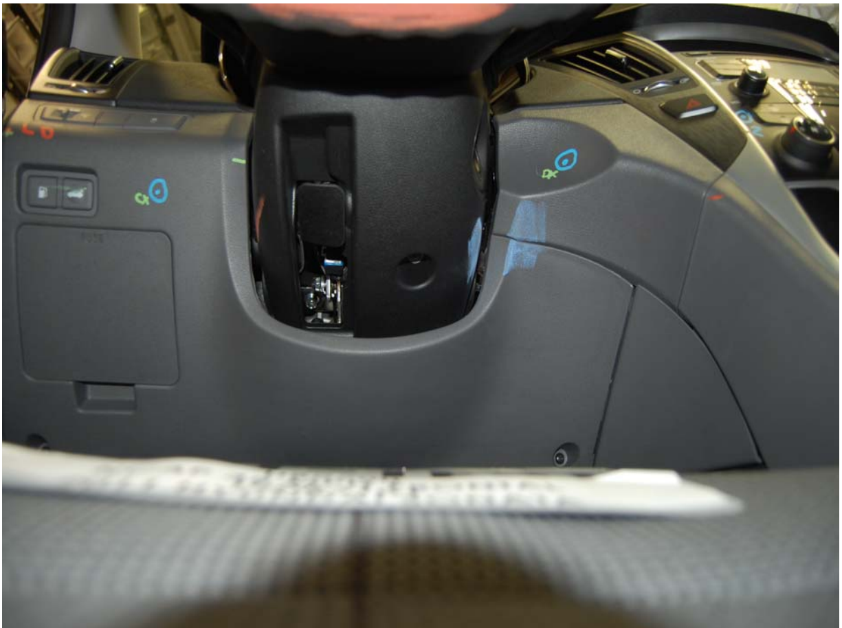
Post-Test Driver Dummy Contact with Knee Bolster
