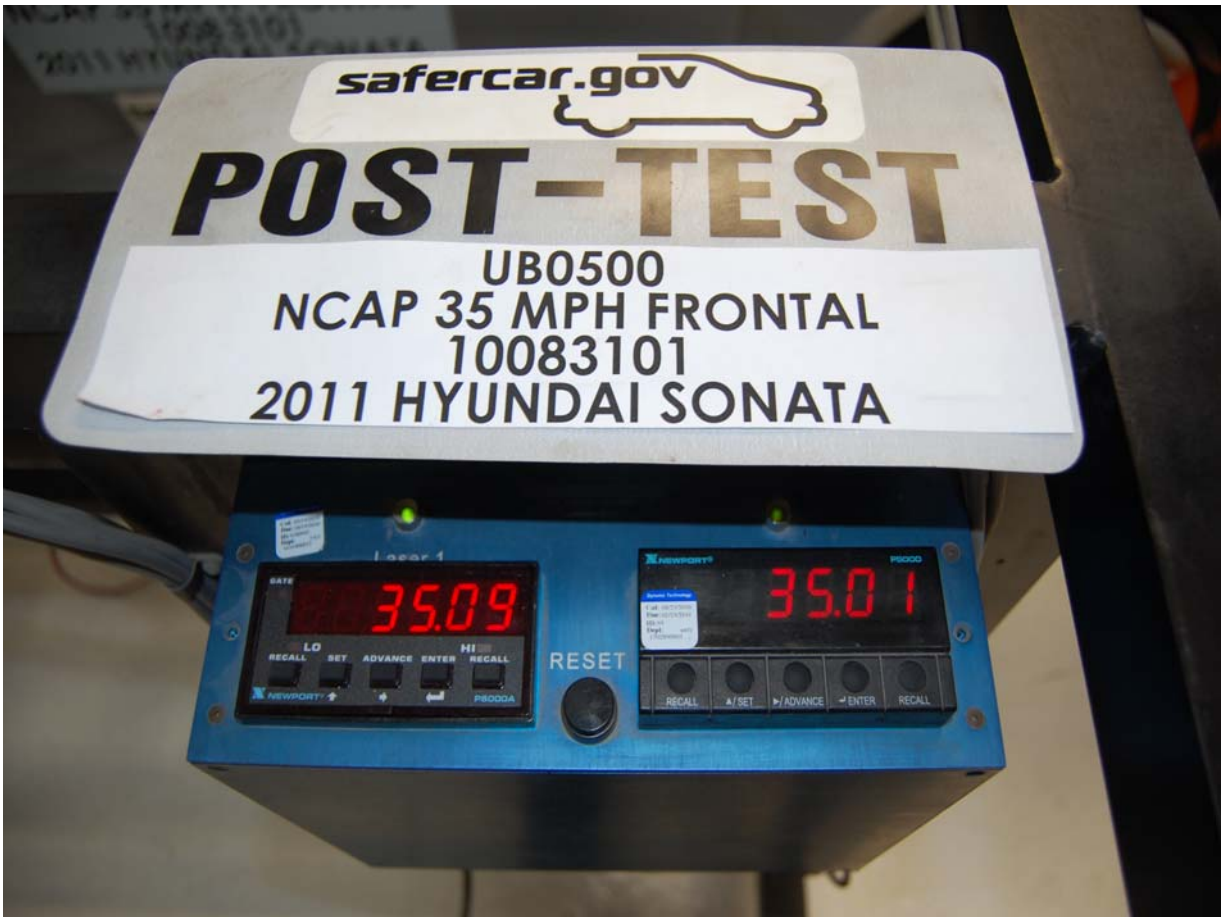
Post-Test Speed Trap Read-Out
