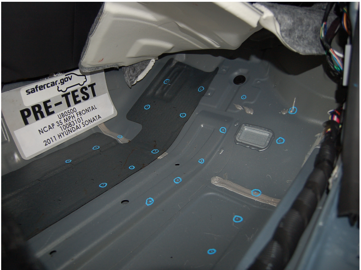
Pre-Test Passenger's Side Floorpan
