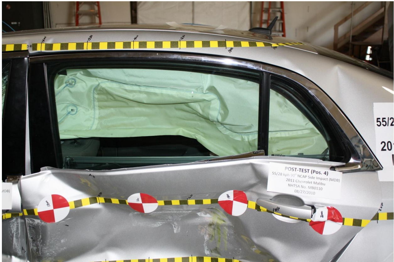
Figure A-55: Post-test Left Side View of Passenger Dummy Shoulder and Door Top View
