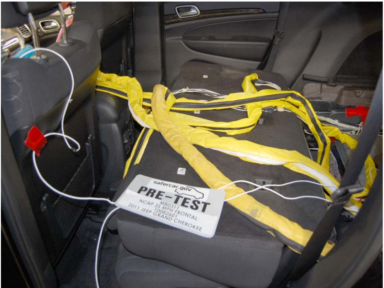
Pre-Test Dummy Cable Routing
