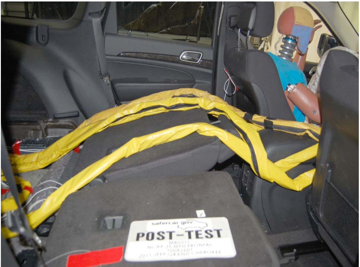
Post-Test Dummy Cable Routing
