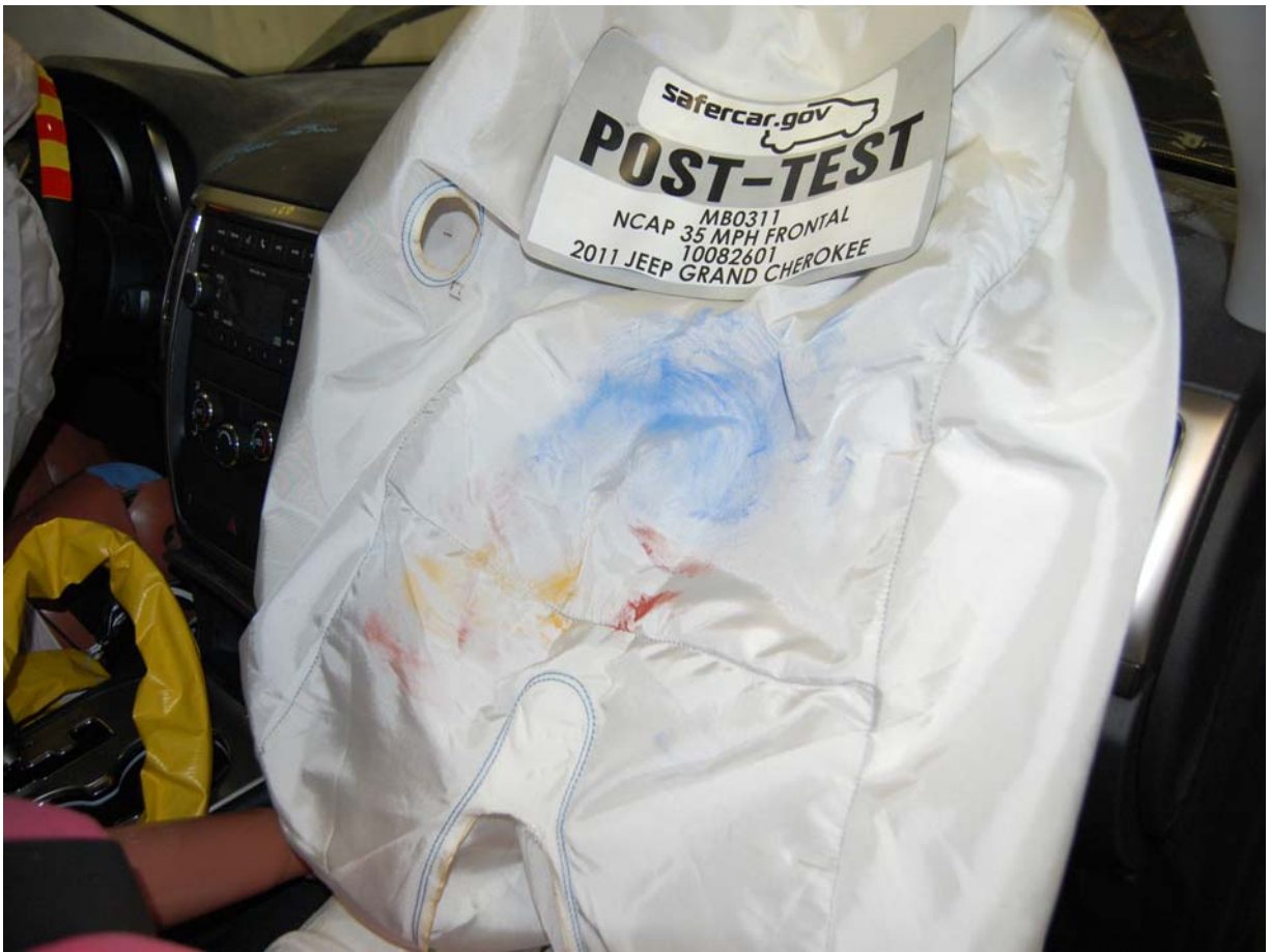
Post-Test Passenger Dummy Contact with Airbag
