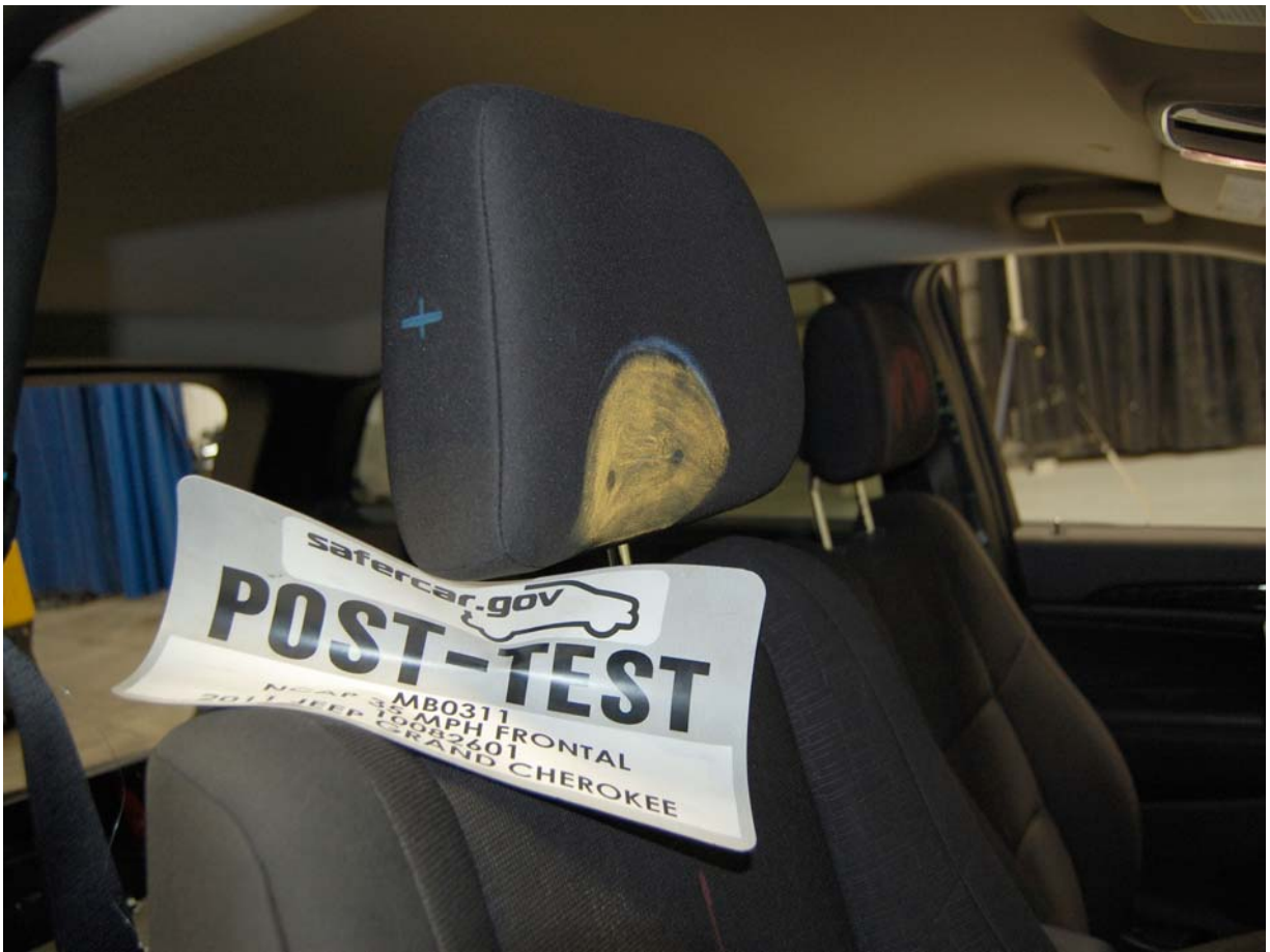
Post-Test Passenger Dummy Contact with Headrest
