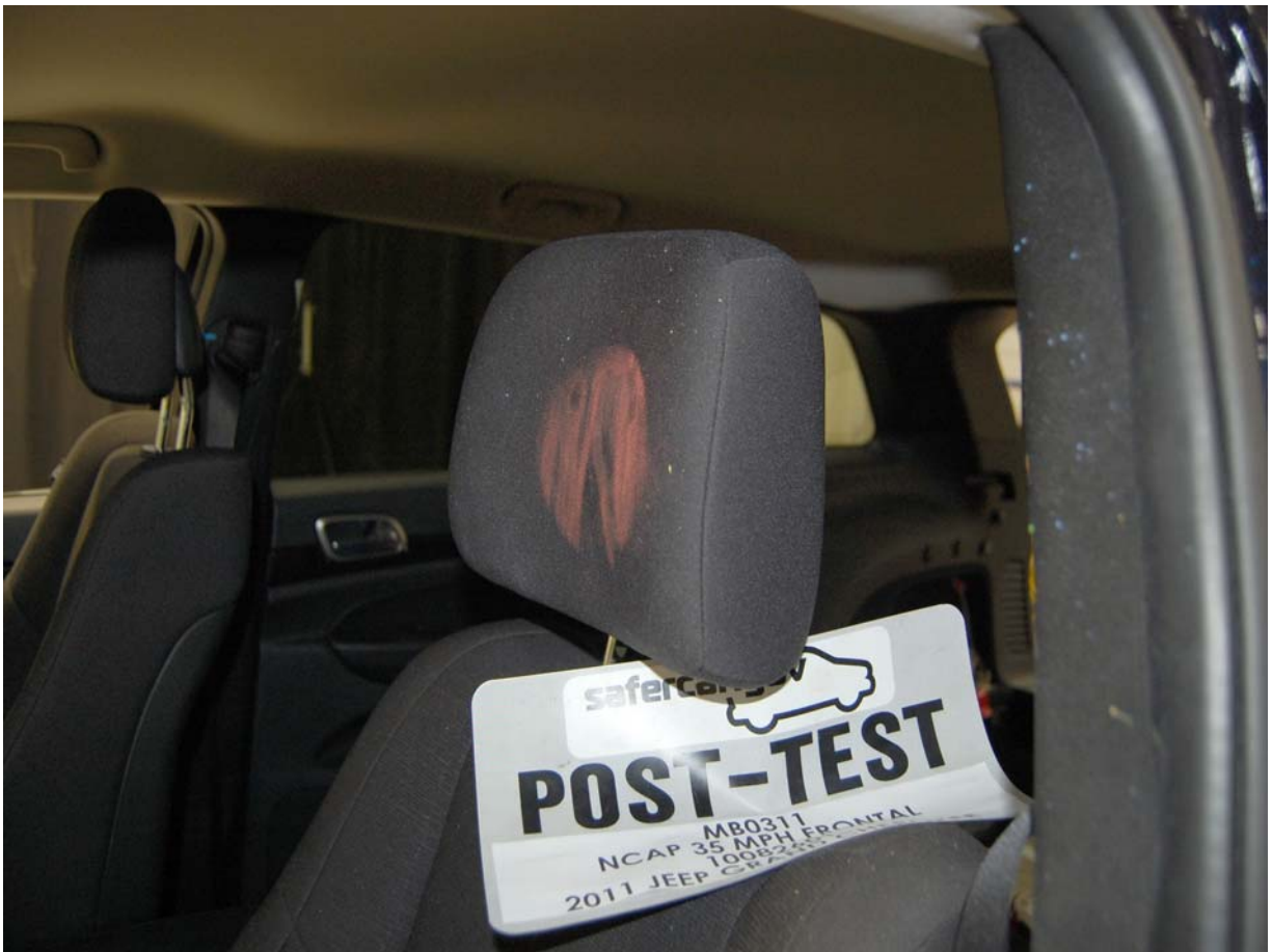
Post-Test Driver Dummy Contact with Headrest
