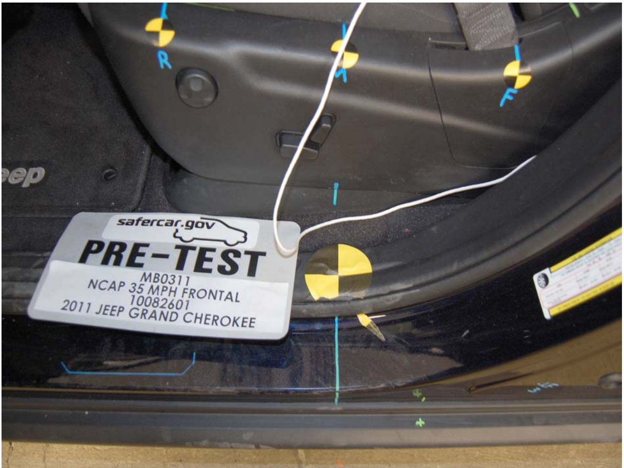
Pre-Test Driver's Seat Fore-Aft Markings
