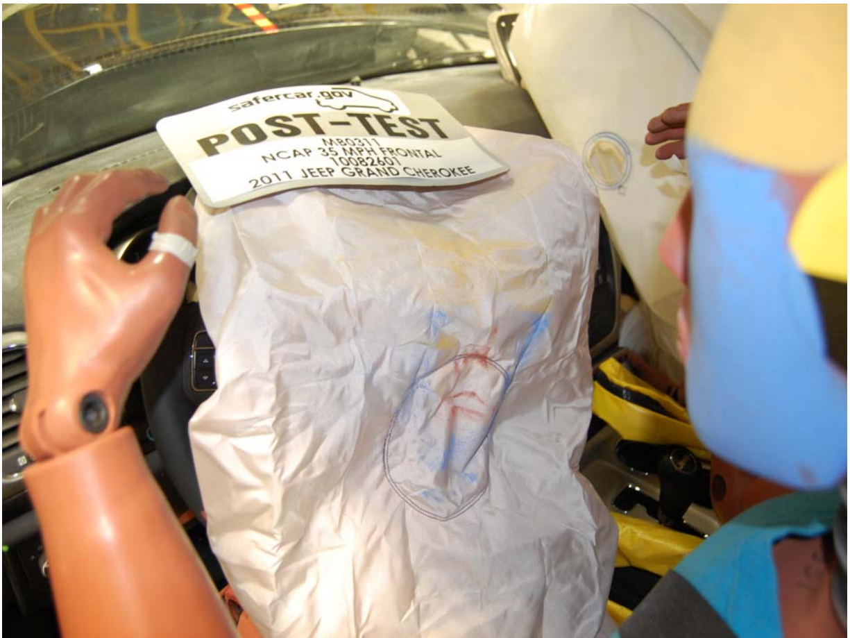
Post-Test Driver Dummy Contact with Airbag
