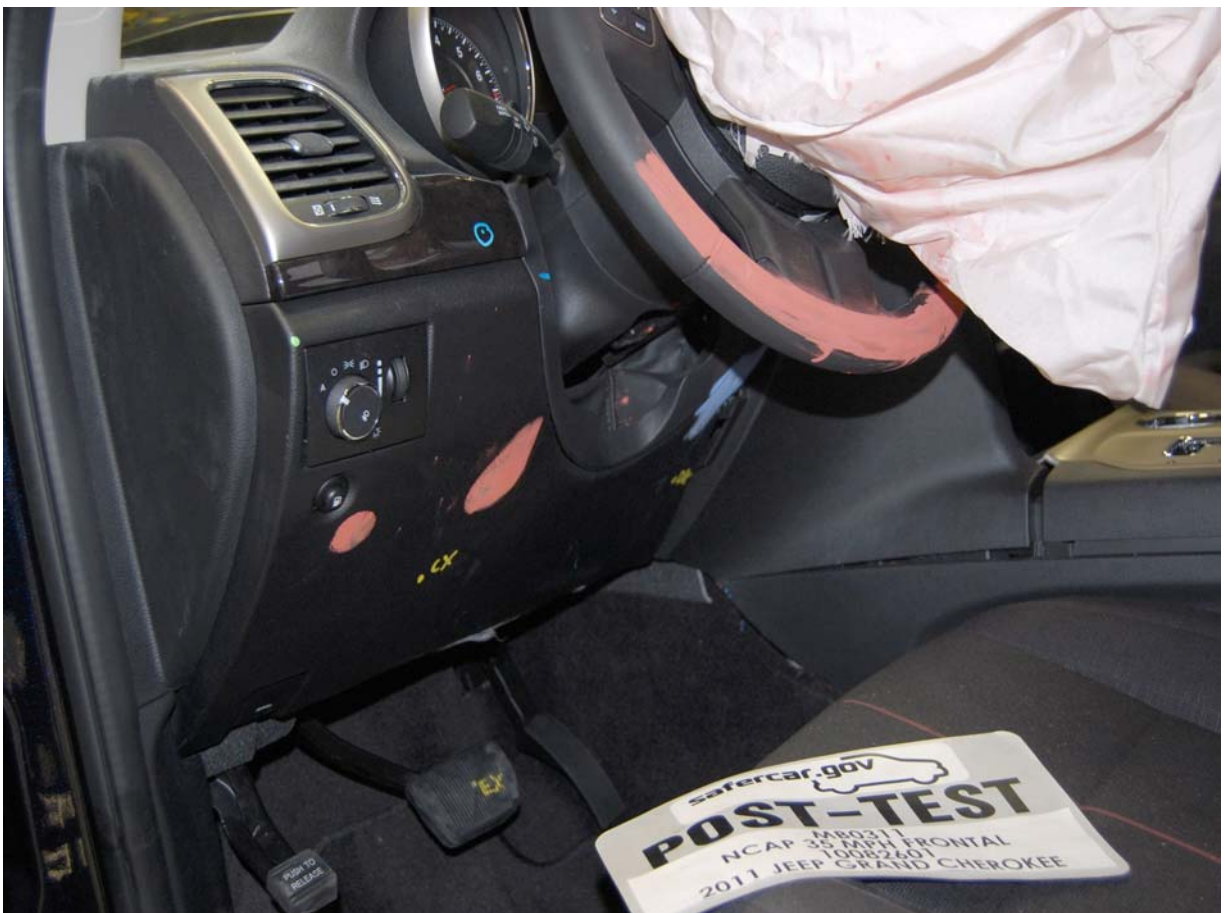
Post-Test View of Steering Column Shear Capsule
