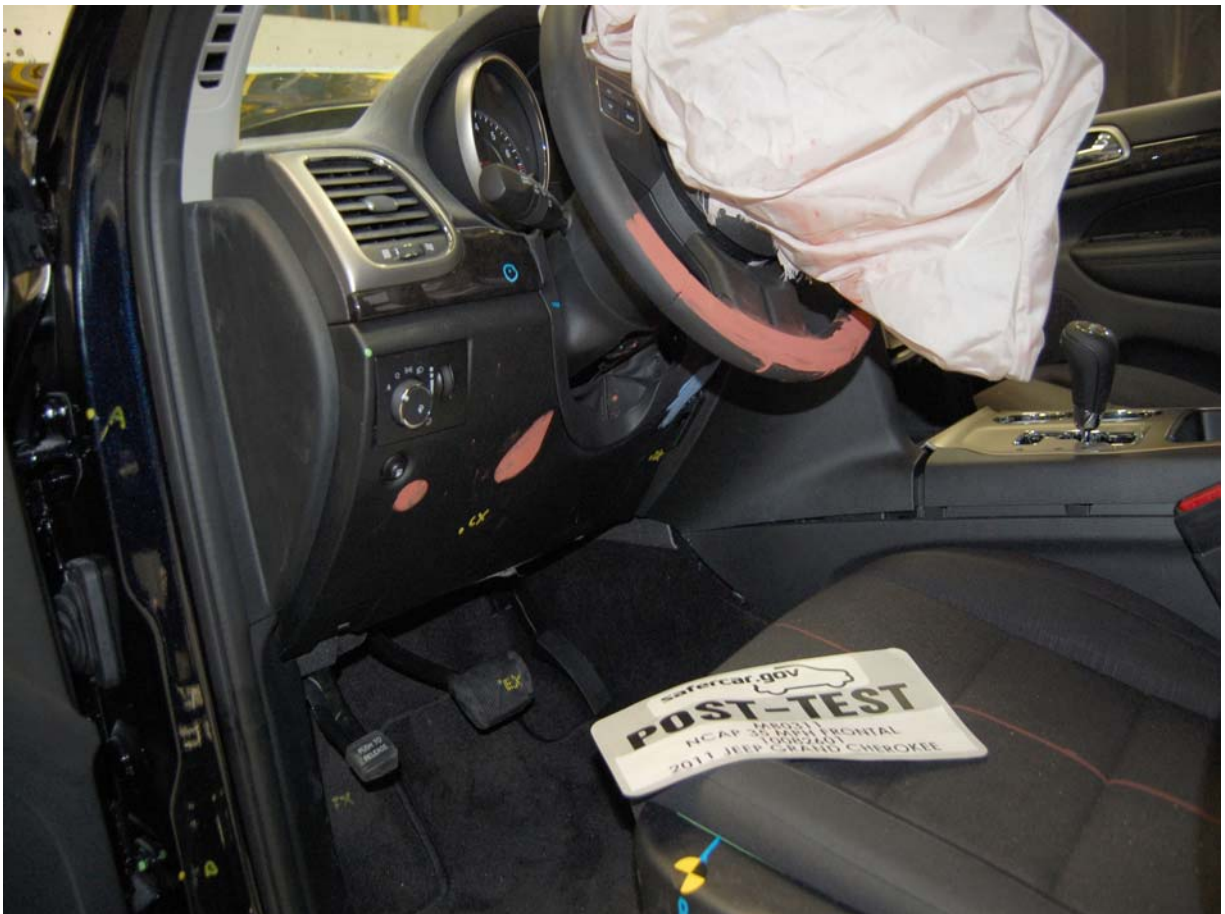
Post-Test Driver's Side Knee Bolster (without dummy)
