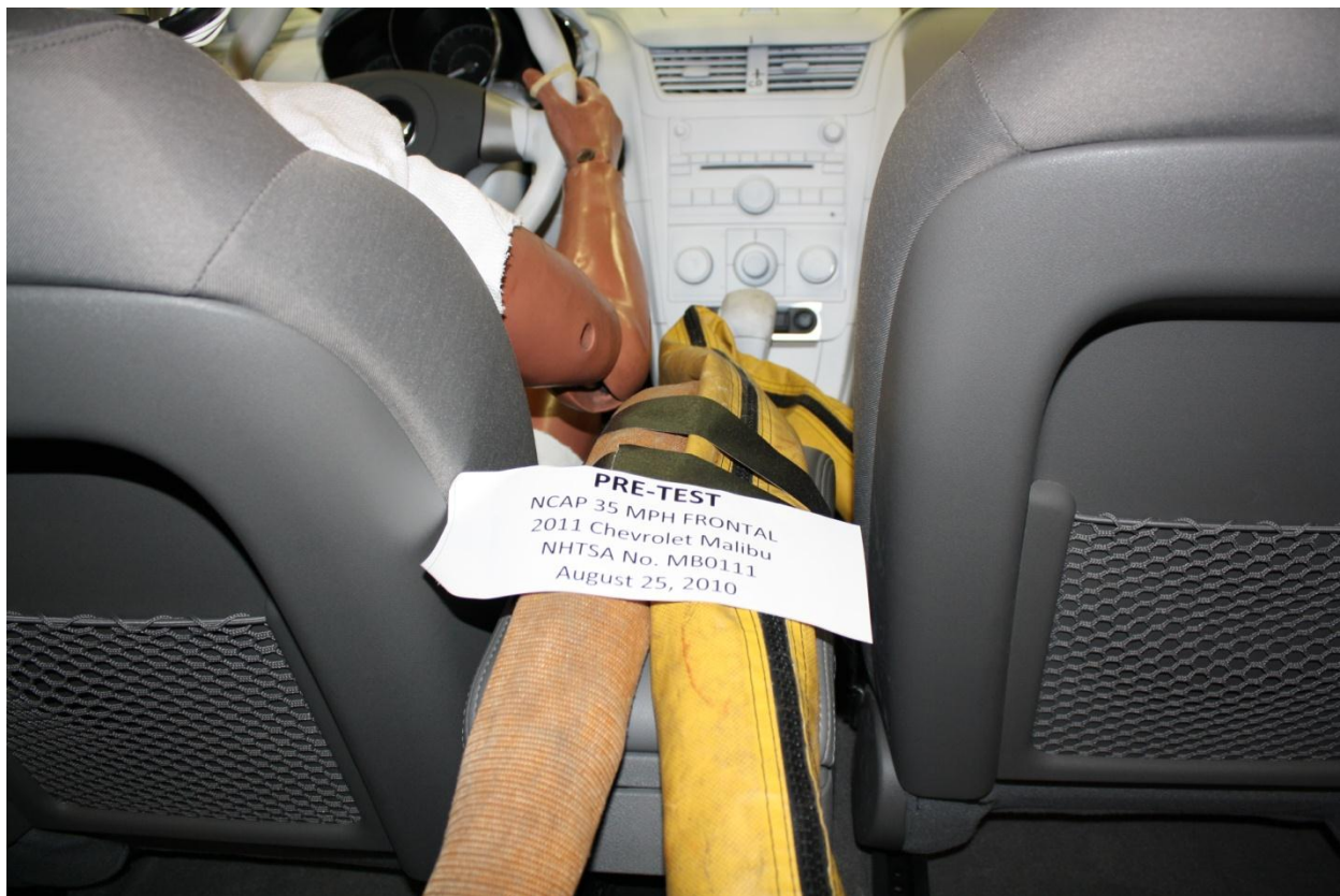
Figure A-27: Pre-Test Dummy Cable Routing
