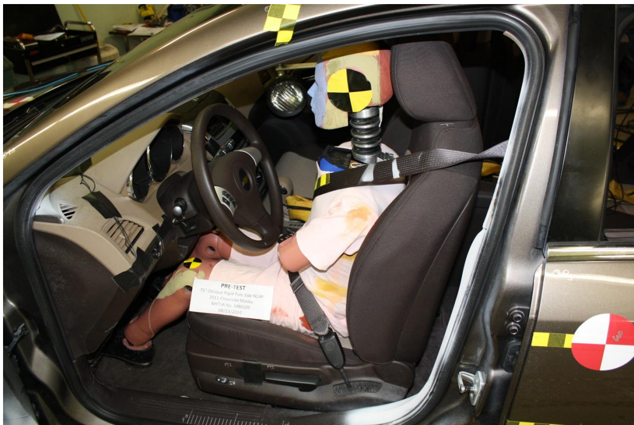
Figure A-23: Pre-Test Left Side View of Dummy Showing Belt, Chalking, and Contact Switches (Door Open)
