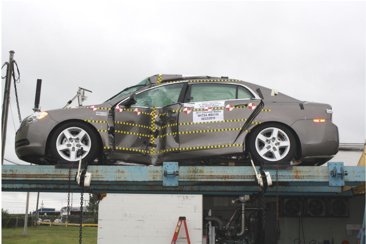
Figure A-65: FMVSS No. 301 Rollover 360°
