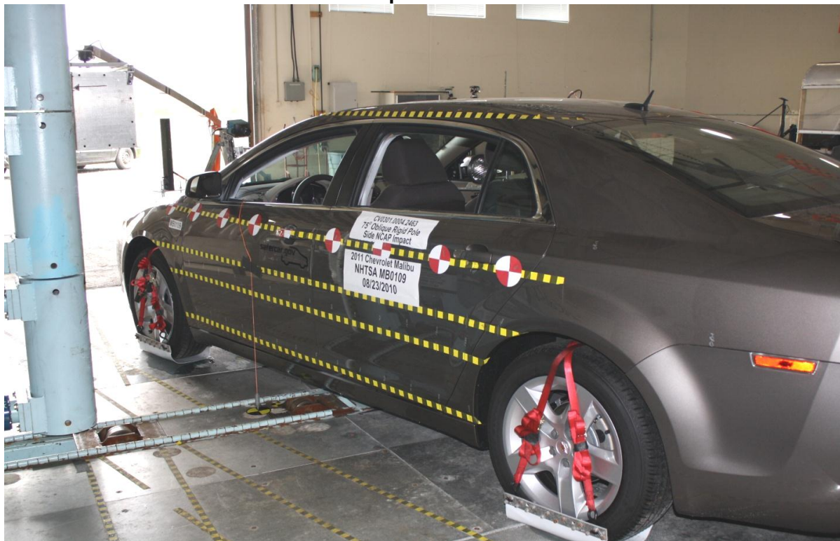
Figure A-18: Pre-Test Right Side View of Pole Positioned Against Side of Vehicle at Ideal Impact Point
