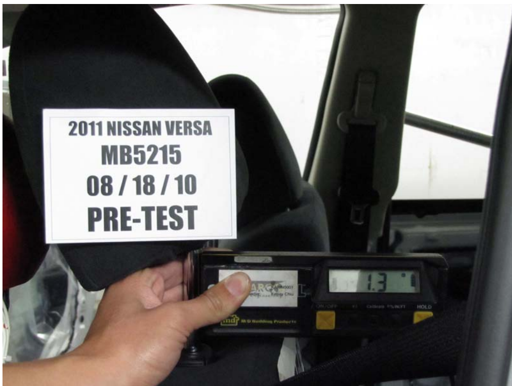
FIGURE 38. Pre-Test Close-Up View of Driver Seat Back or Head Restraint Showing Seat Back Test Position
