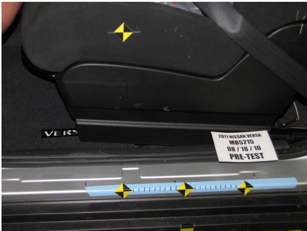
FIGURE 36. Pre-Test Close-Up Left Side View of Driver Seat Track Showing Test Position
