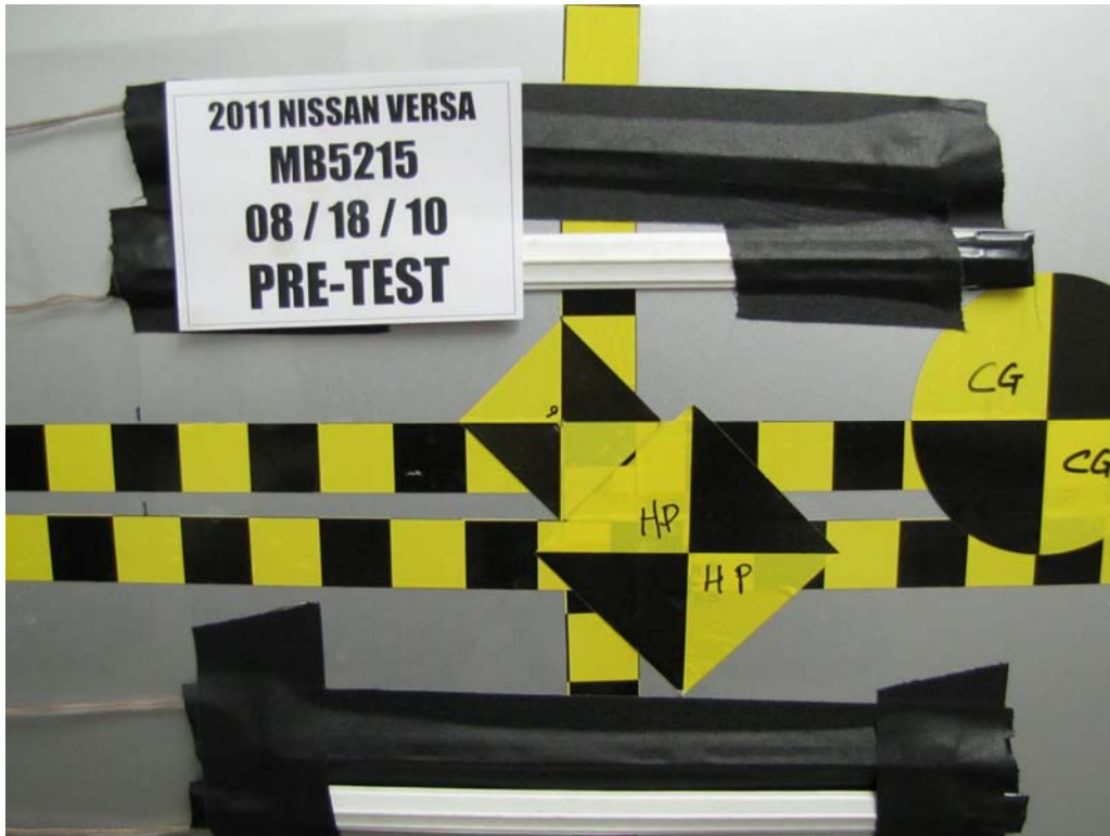
FIGURE 19. Pre-Test Close-Up View of Impact Point Target
