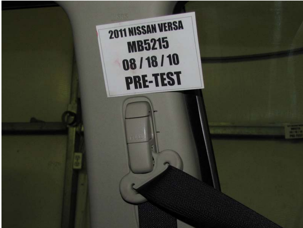
FIGURE 33. Pre-Test View of Belt Anchorage for Dummy to Show Position
