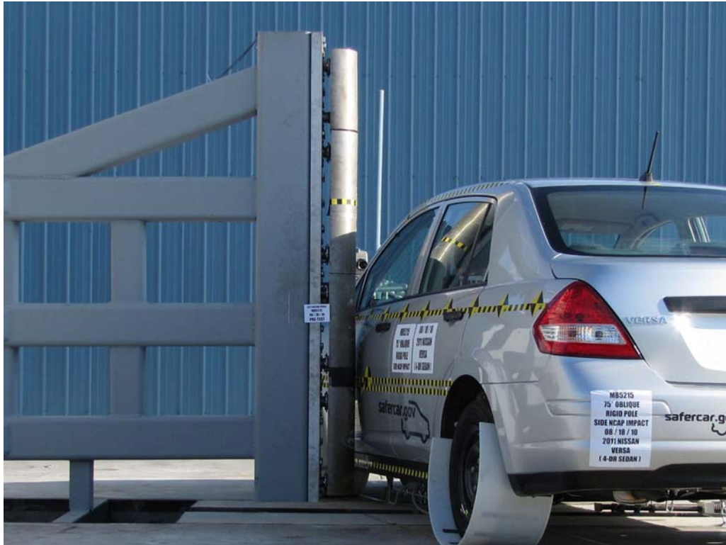
FIGURE 17. Pre-Test Left Side View of Pole Positioned Against Side of Vehicle at Ideal Impact Point
