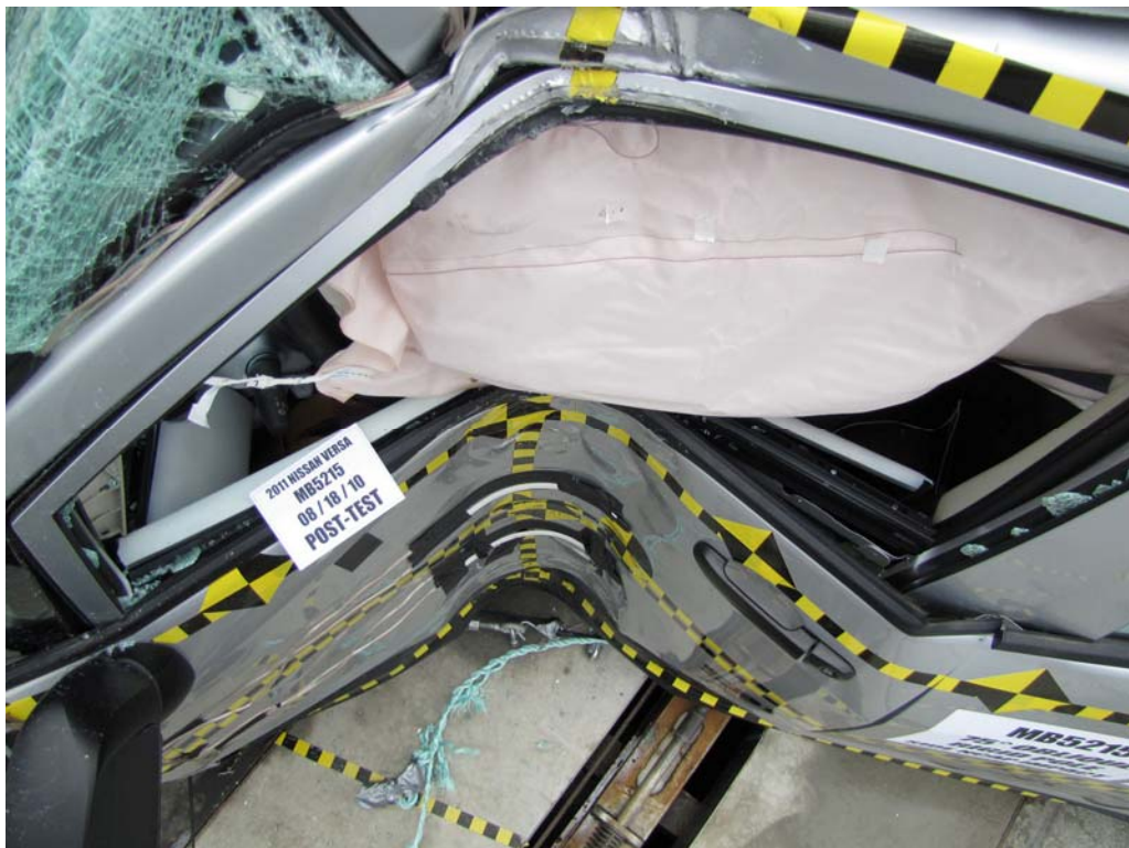
FIGURE 40. Post-Test Driver Dummy and Door Clearance
