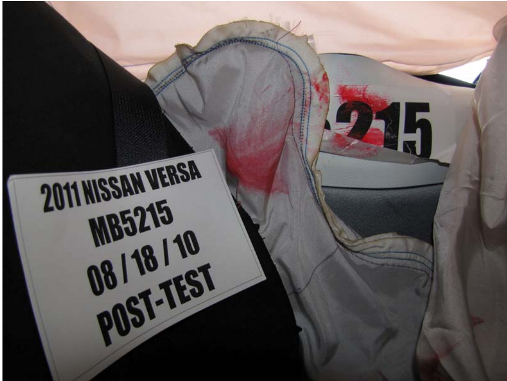
FIGURE 47. Post-Test Dummy Close-Up Torso Contact with Vehicle Interior View
