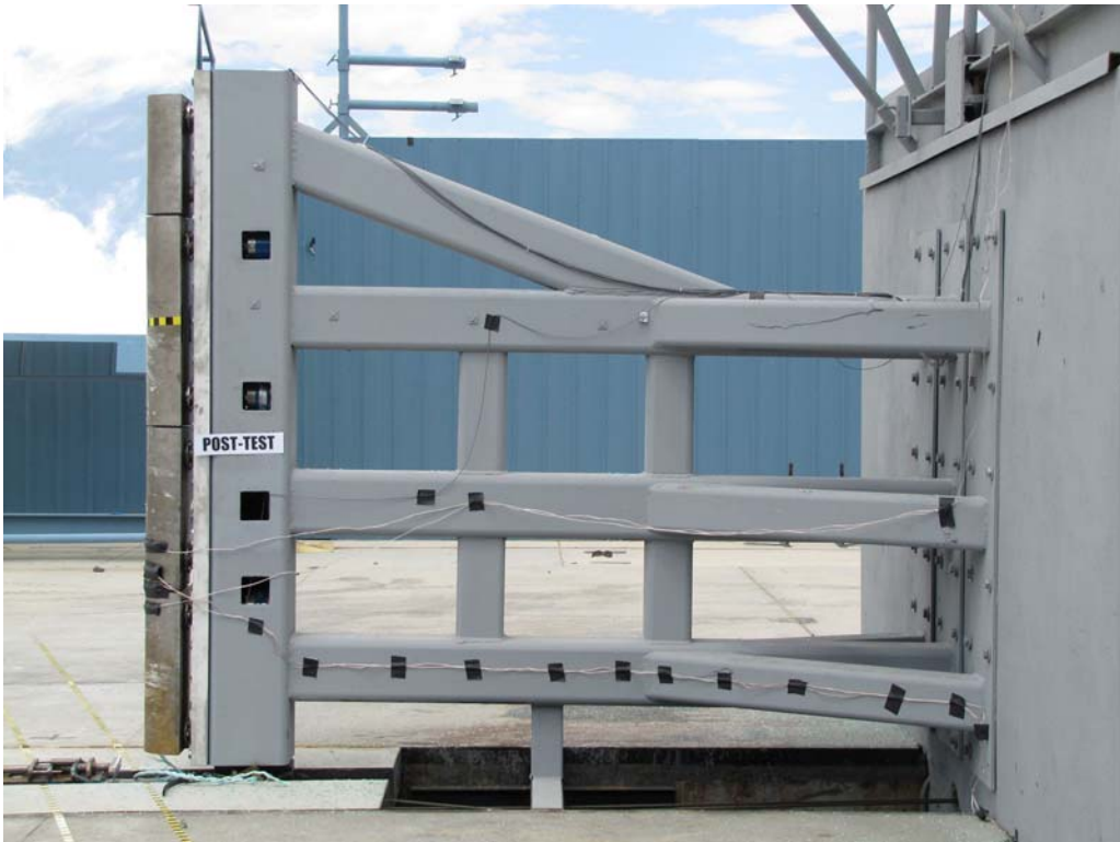
FIGURE 58. Post-Test Pole Barrier Side View
