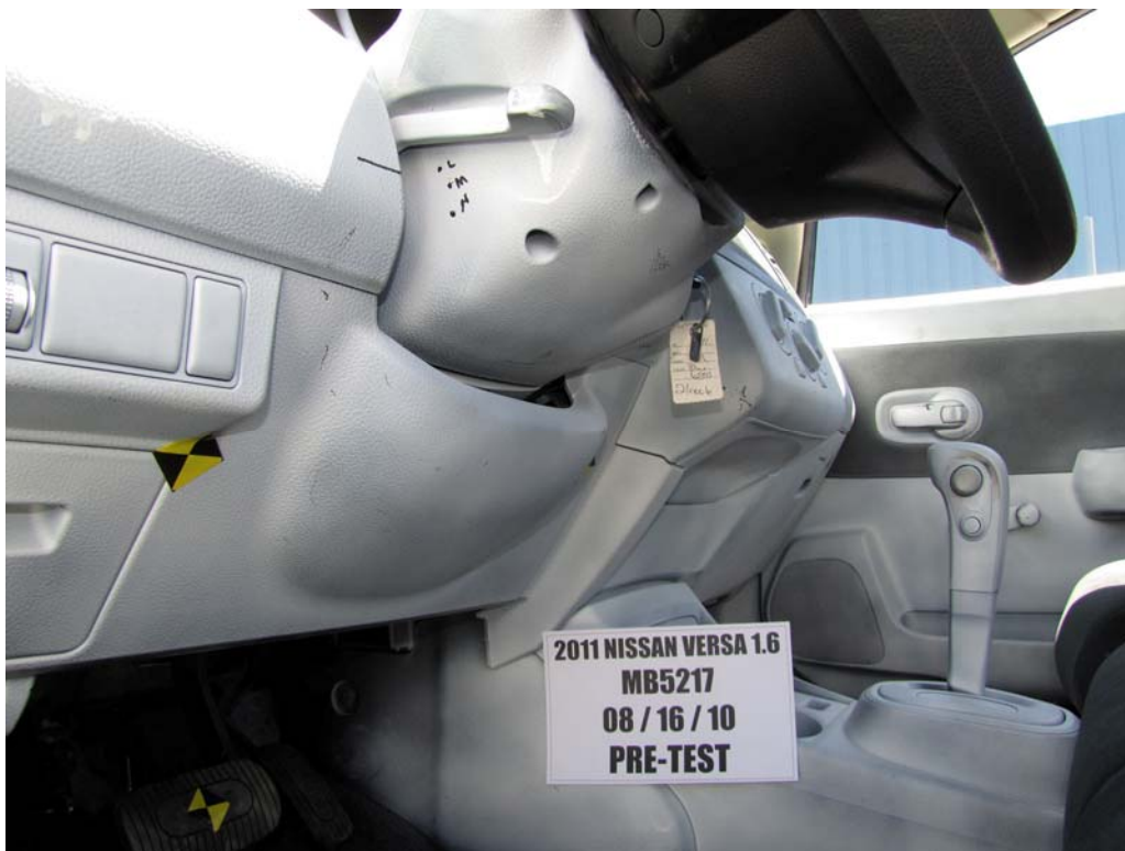
FIGURE 44. Pre-Test View of Steering Column Shear Capsule
