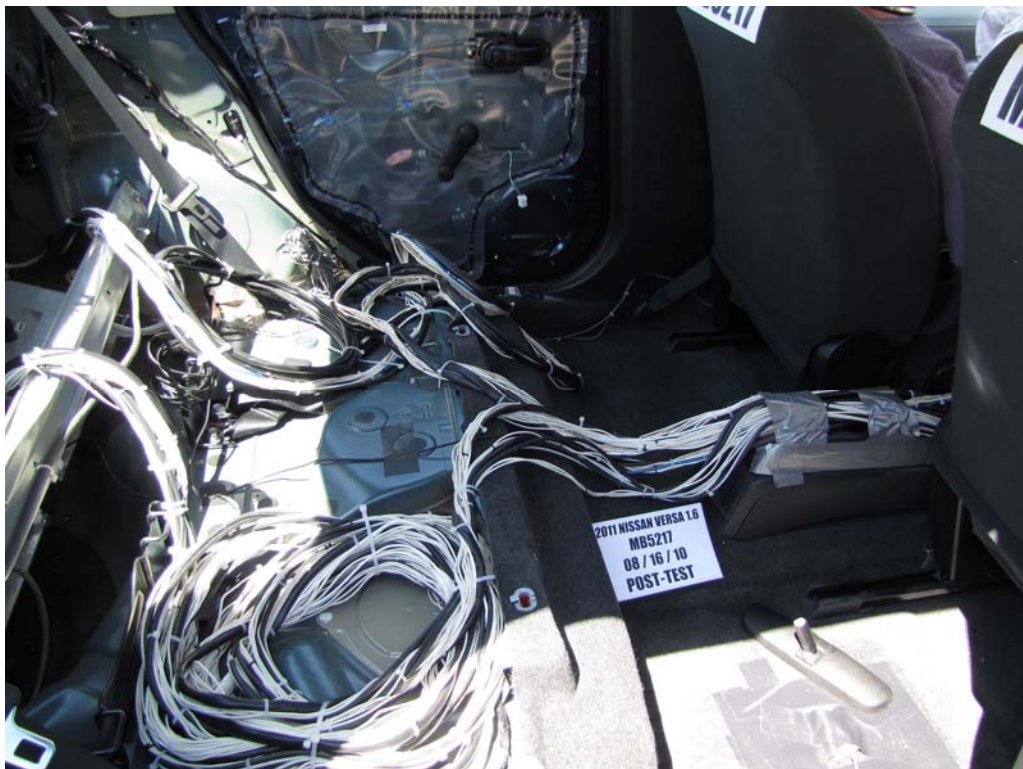
FIGURE 28. Post-Test Dummy Cable Routing
