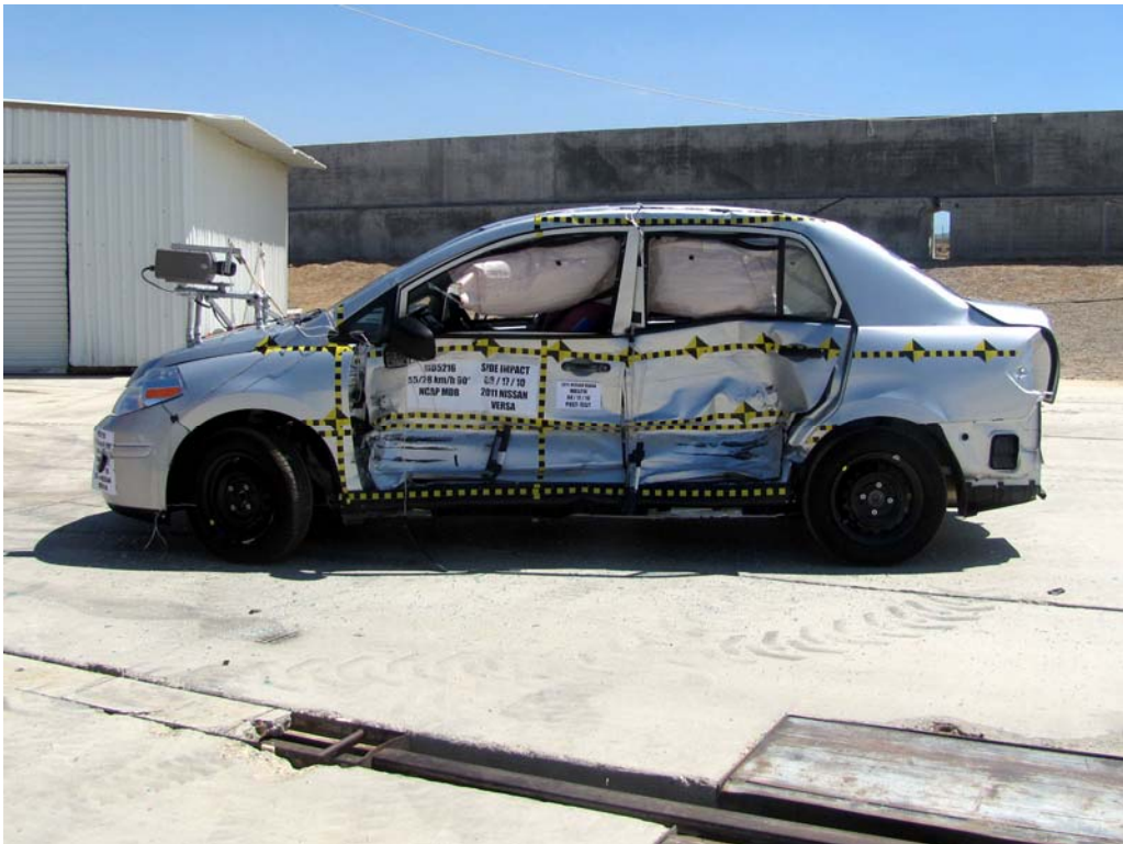
FIGURE 8. Post-Test Left Side View of Test Vehicle
