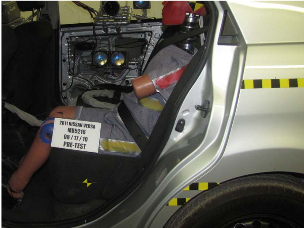
FIGURE 65. Pre-Test Close-Up Left Side View of Rear Passenger Seat Back Showing Test Position
