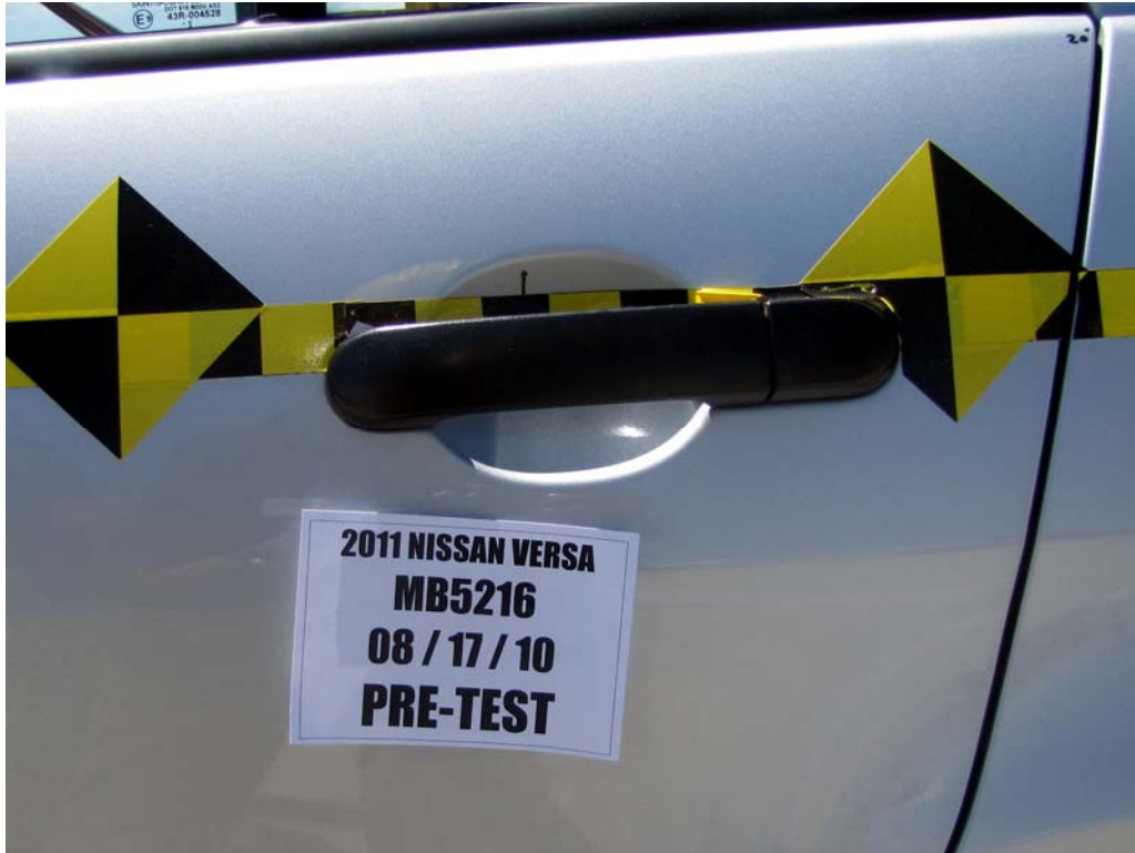
FIGURE 23. Pre-Test Left Rear Door Latch Close-Up
