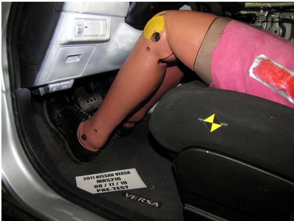
FIGURE 34. Pre-Test Placement of Driver Dummy's Feet
