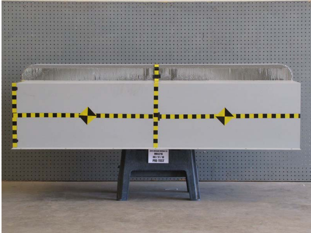
FIGURE 83. Pre-Test Top View of MDB Impactor Face
