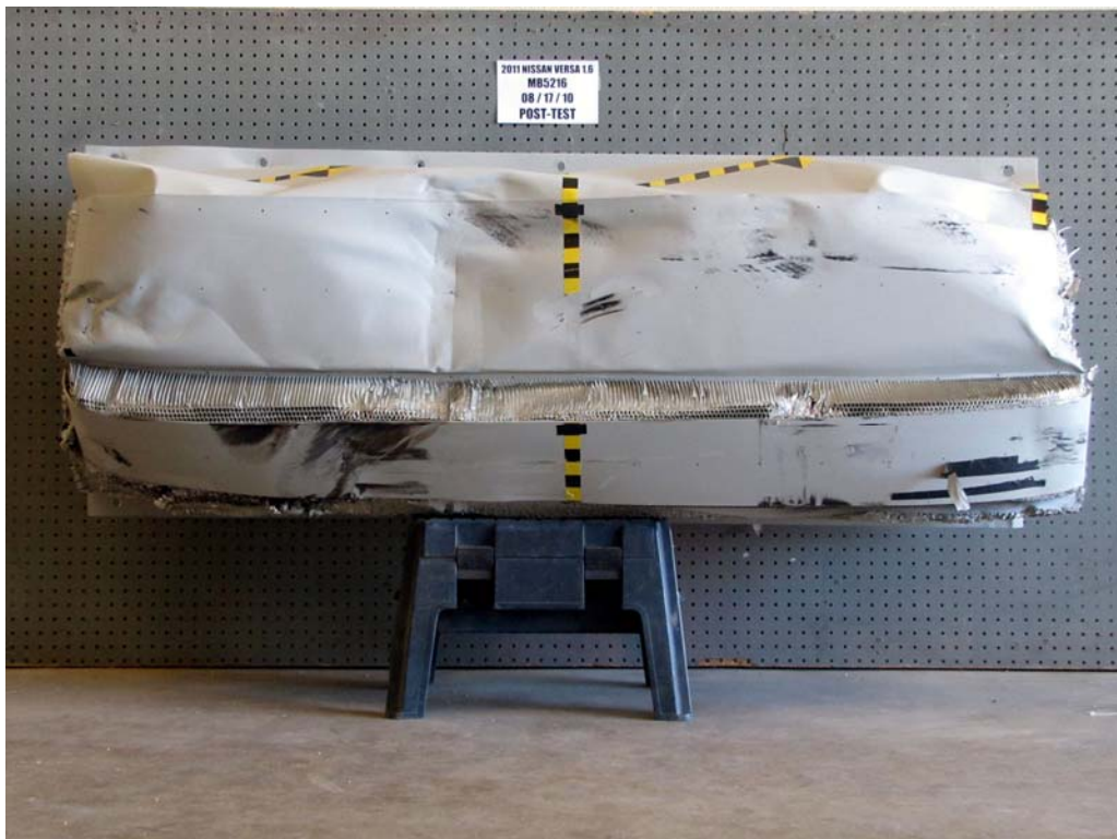
FIGURE 82. Post-Test Front View of MDB Impactor Face
