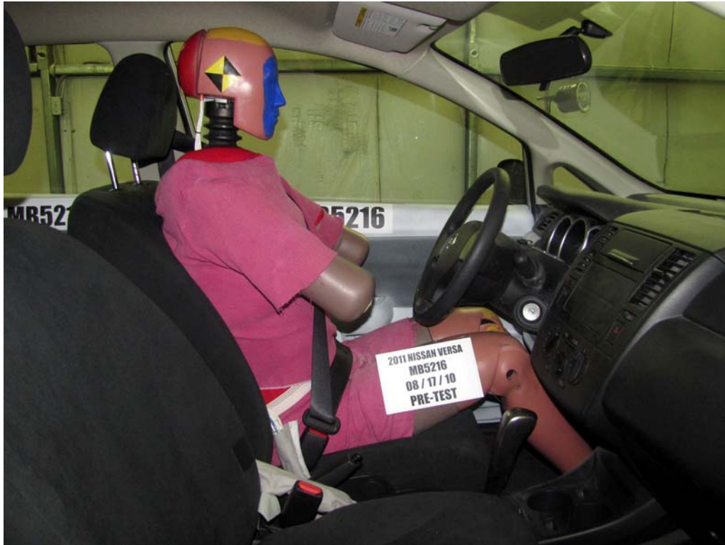
FIGURE 43. Pre-Test Right Side View of Driver Dummy and Front Seat of Occupant Compartment
