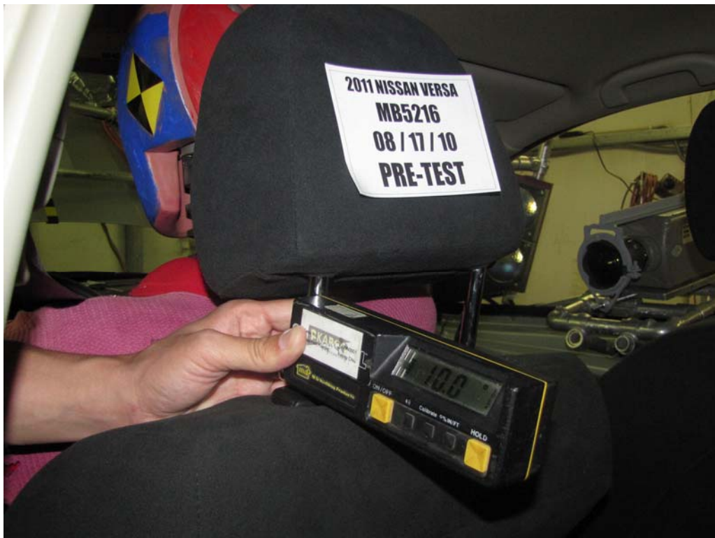
FIGURE 40. Pre-Test Close-Up View of Driver Seat Back or Head Restraint Showing Seat Back Test Position
