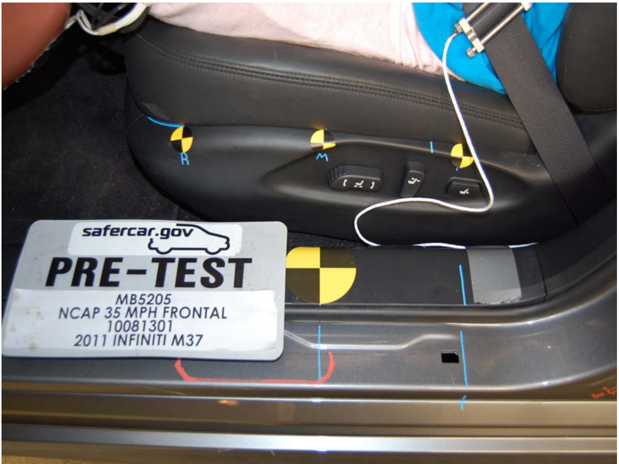
Pre-Test Driver's Seat Fore-Aft Markings
