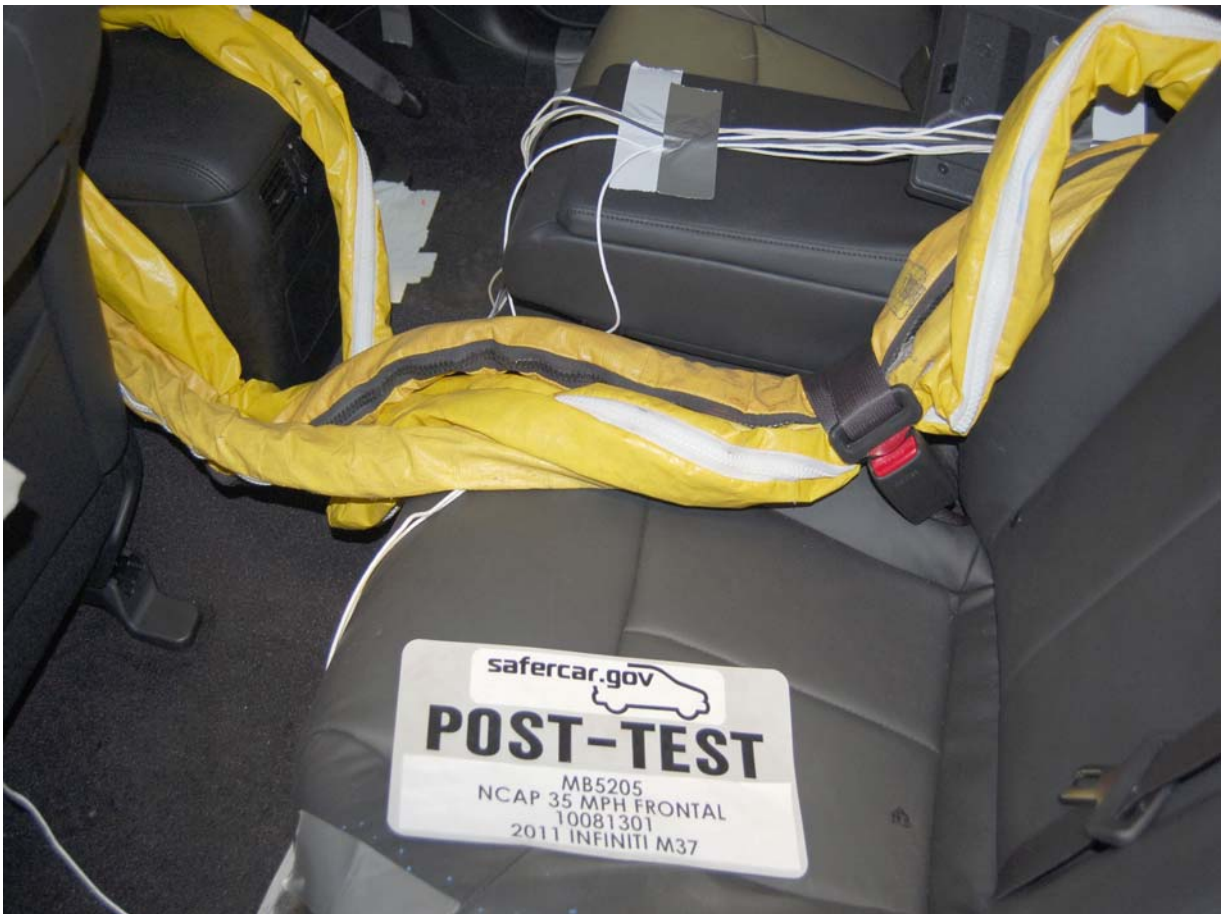
Post-Test Dummy Cable Routing
