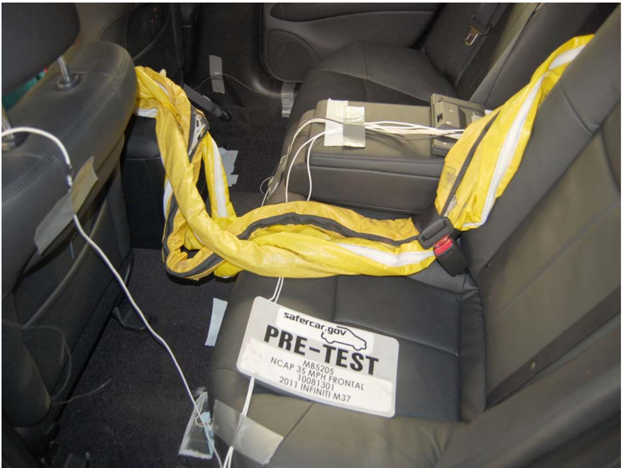
Pre-Test Dummy Cable Routing
