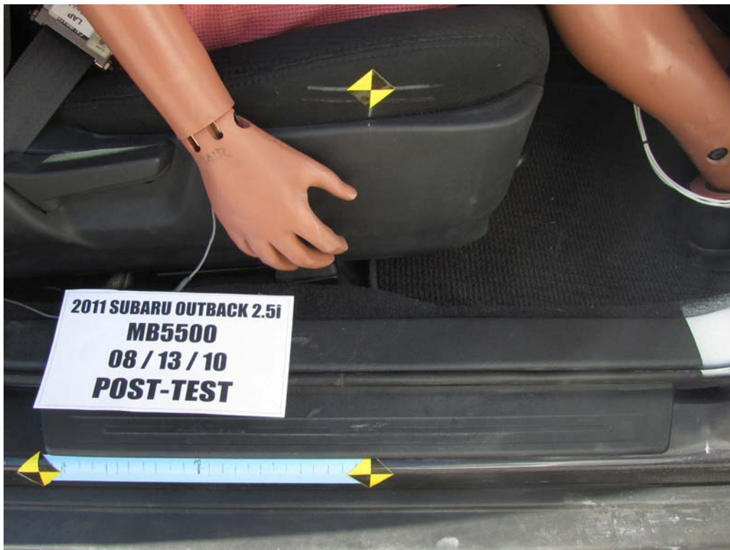
FIGURE 53. Post-Test Passenger's Seat Fore-Aft Markings
