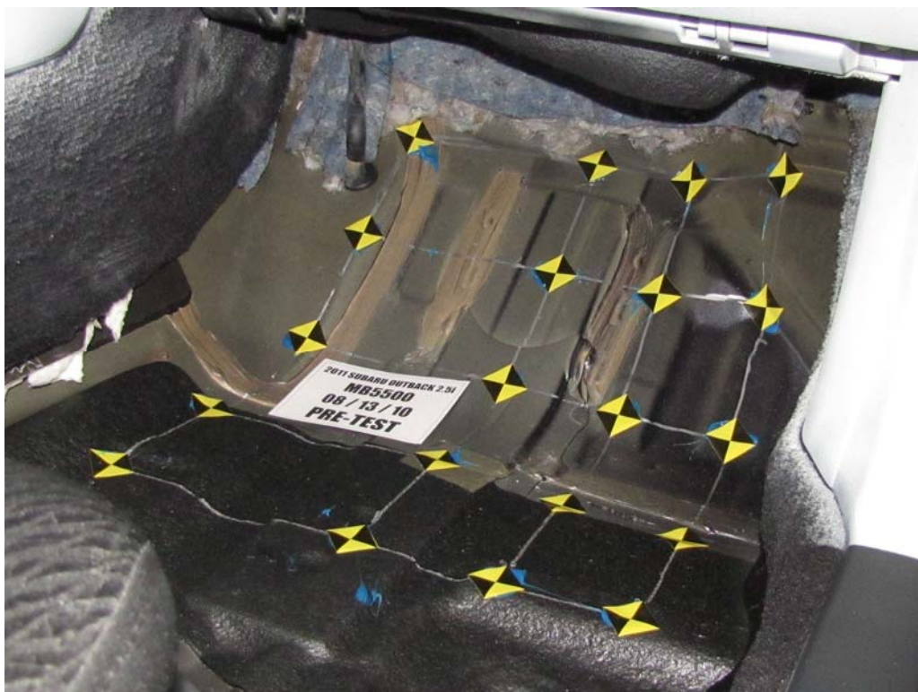
FIGURE 58. Pre-Test Passenger's Side Floorpan
