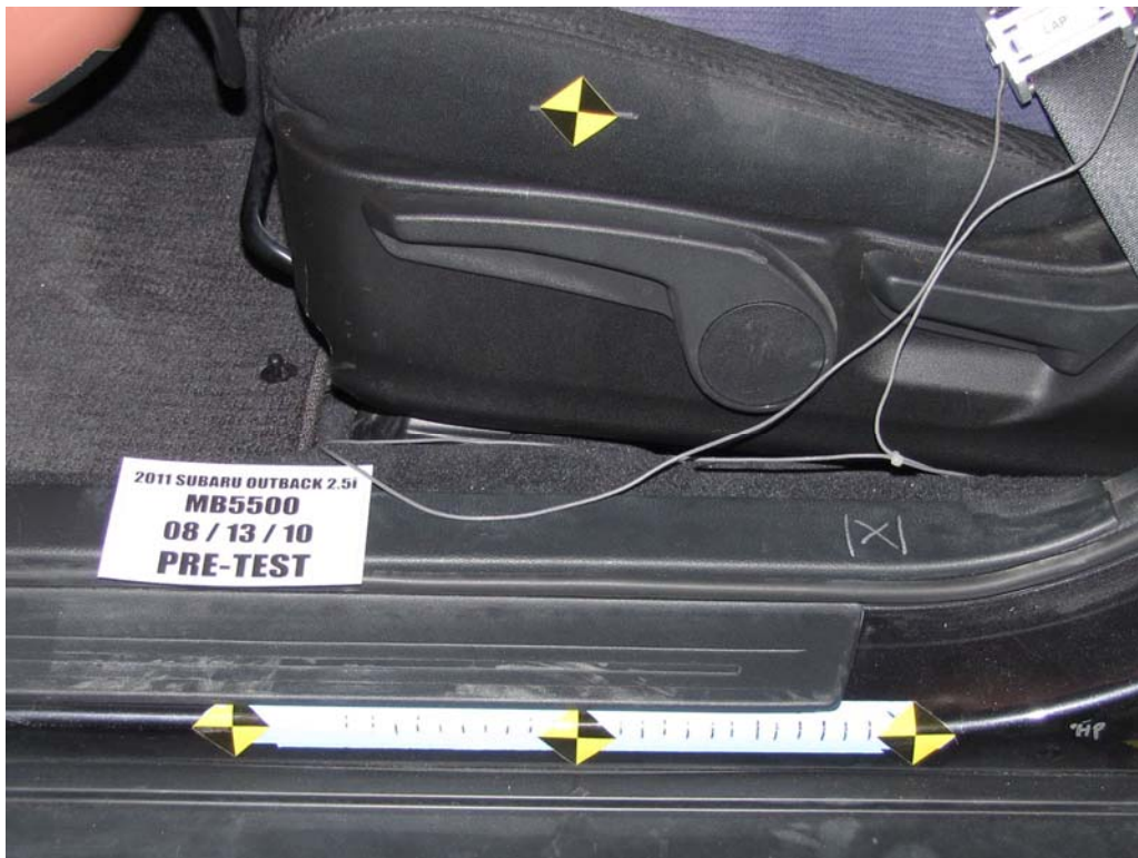
FIGURE 35. Pre-Test Driver's Seat Fore-Aft Markings
