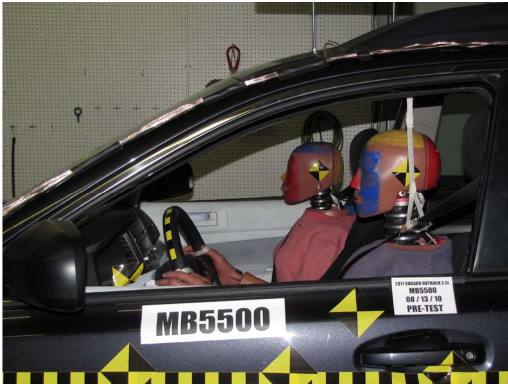
FIGURE 31. Pre-Test Driver Dummy Window View
