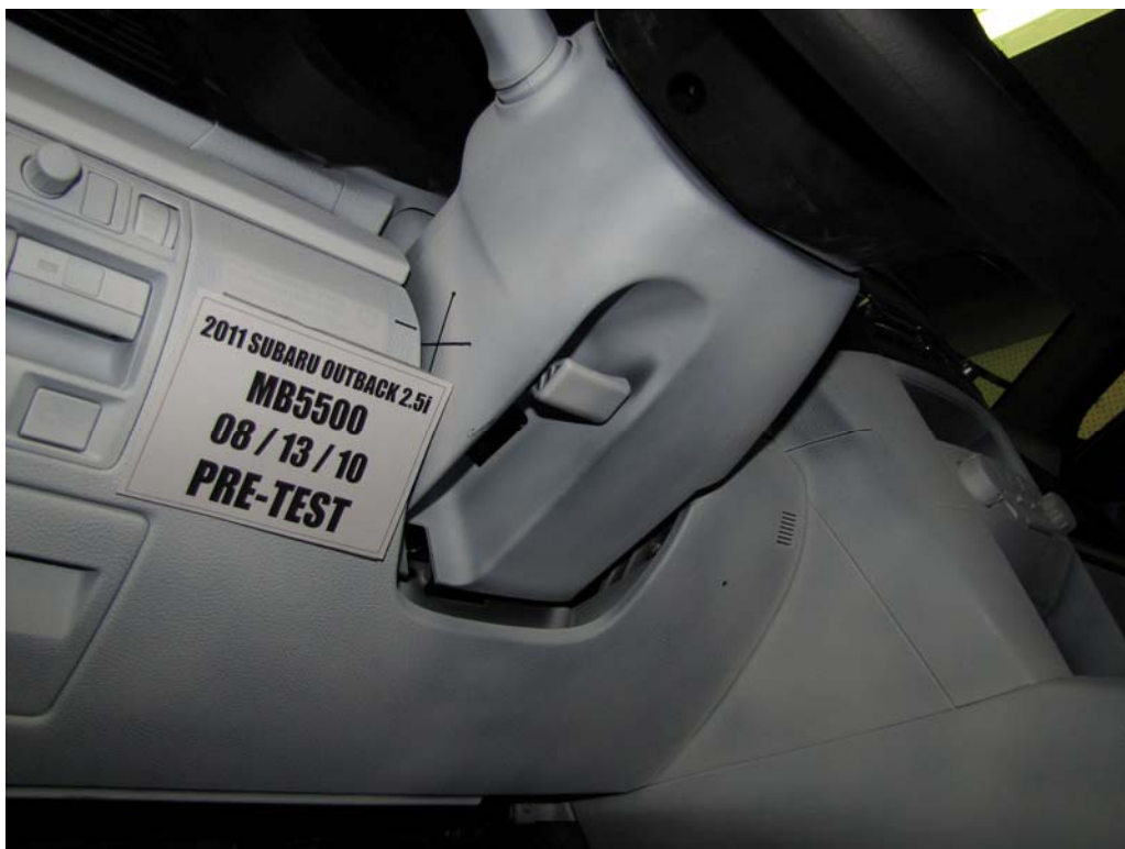
FIGURE 44. Pre-Test View of Steering Column Shear Capsule
