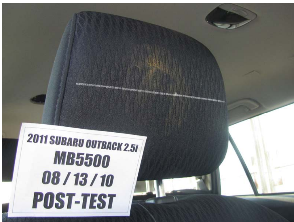
FIGURE 60a. Post-Test Passenger Dummy Contact With Headrest
