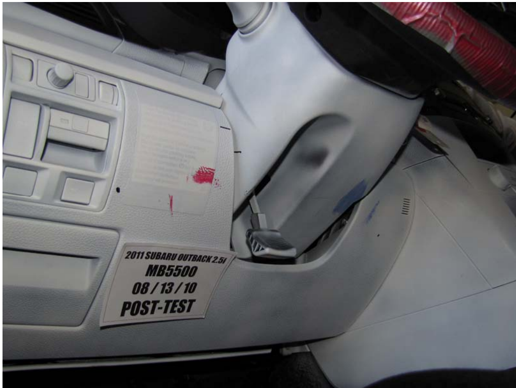
FIGURE 45. Post-Test View of Steering Column Shear Capsule
