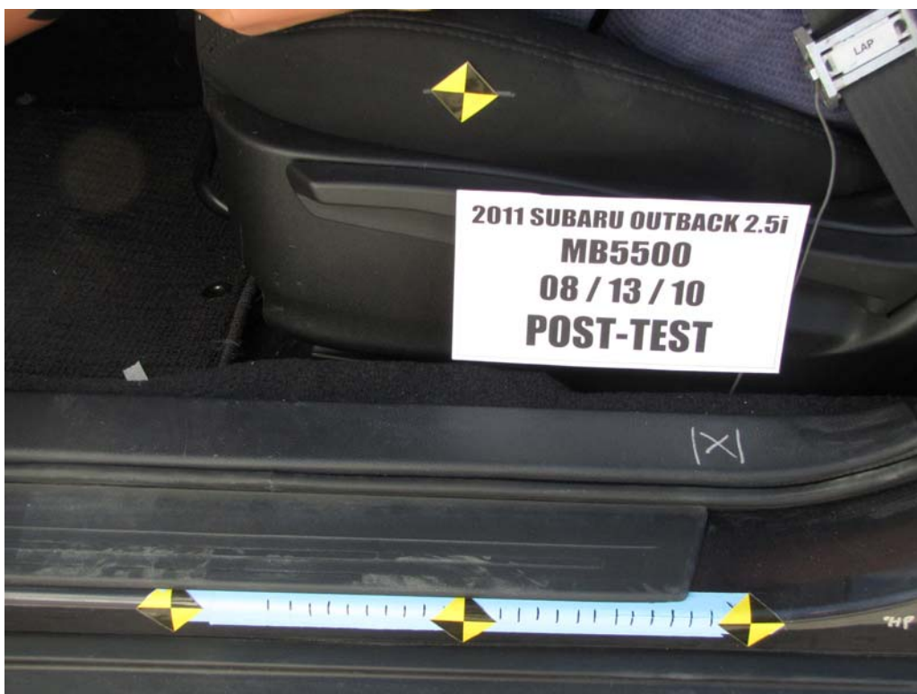
FIGURE 36. Post-Test Driver's Seat Fore-Aft Markings
