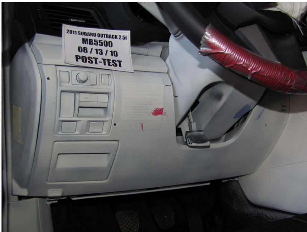
FIGURE 40. Post-Test Driver's Side Knee Bolster
