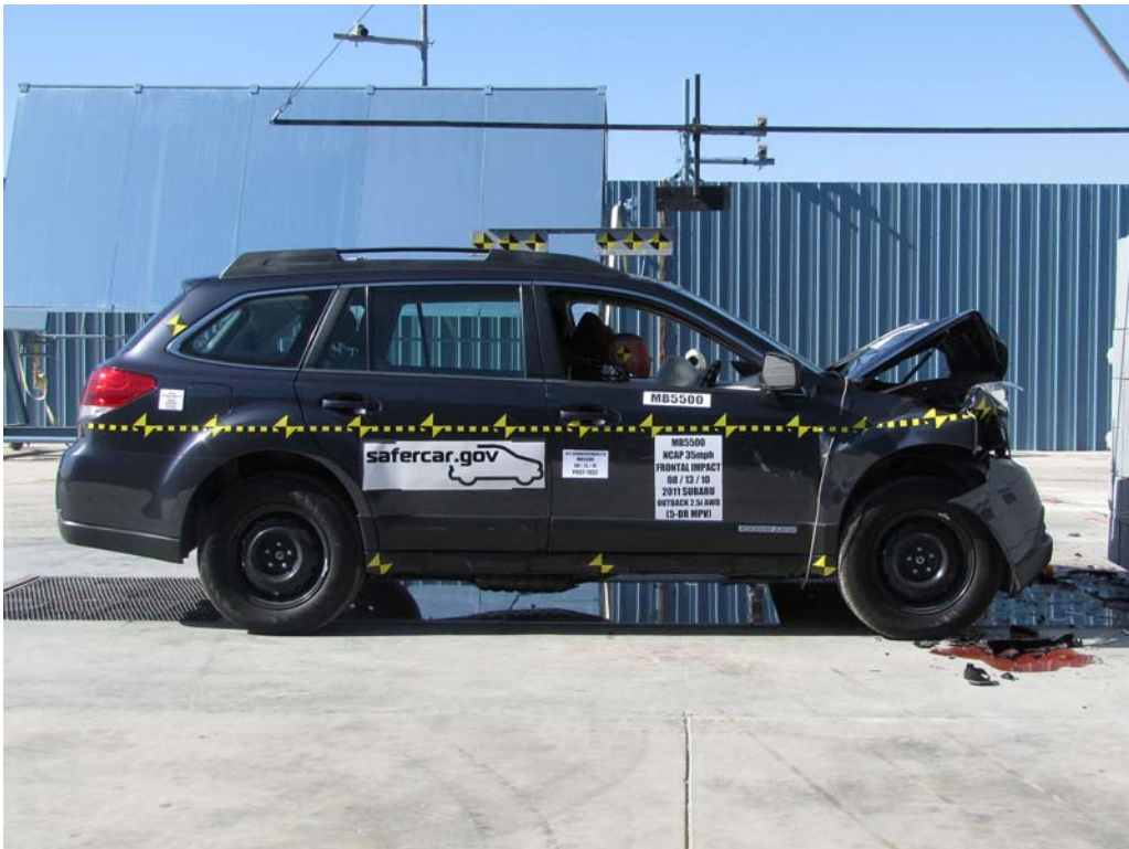
FIGURE 12. Post-Test Right View of Test Vehicle
