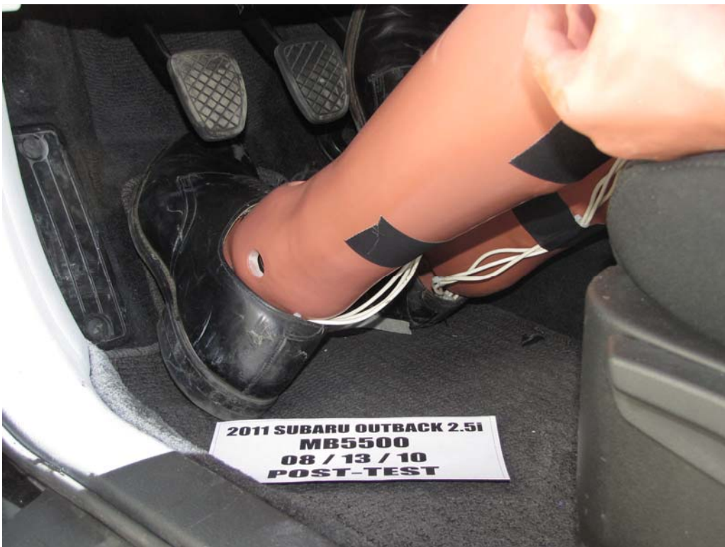
FIGURE 38. Post-Test Driver Dummy Feet
