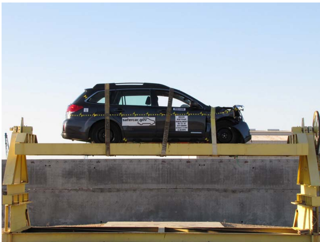
FIGURE 64. Vehicle at 0°on Static Rollover Device
