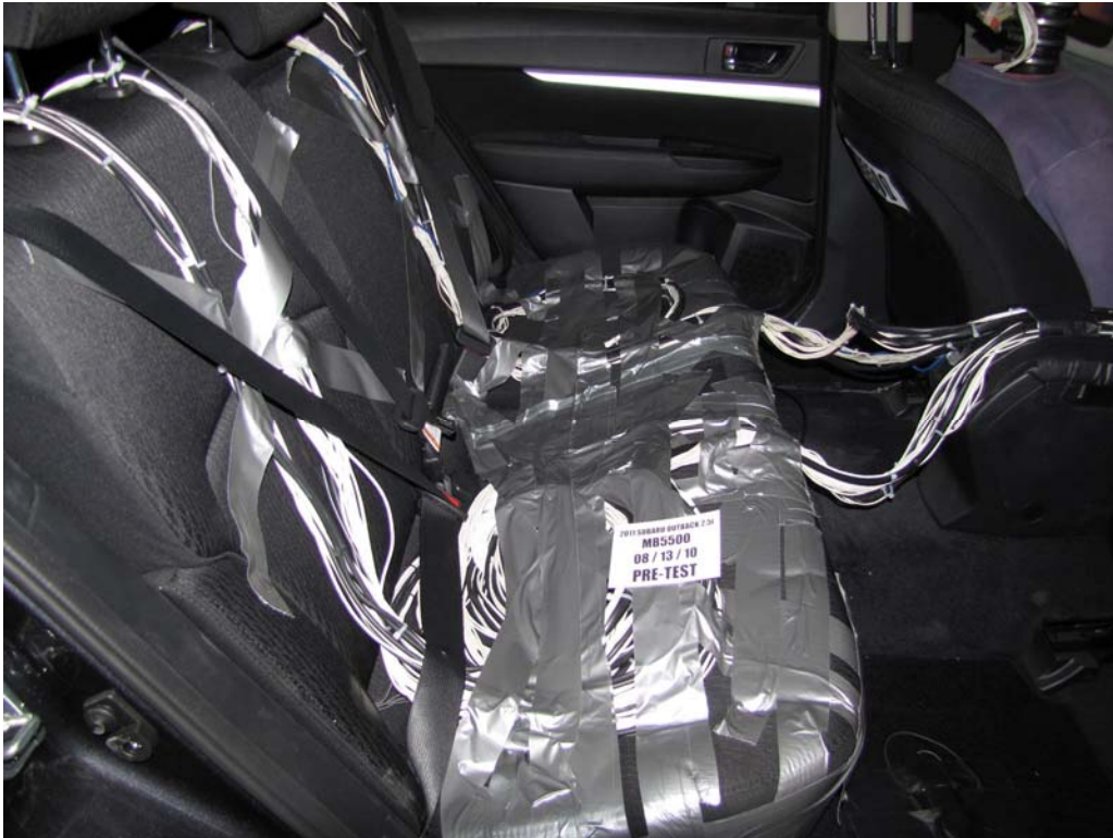
FIGURE 27. Pre-Test Dummy Cable Routing
