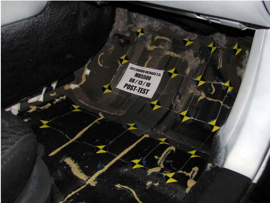
FIGURE 59. Post-Test Passenger's Side Floorpan
