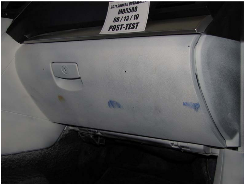
FIGURE 57. Post-Test Passenger's Side Knee Bolster
