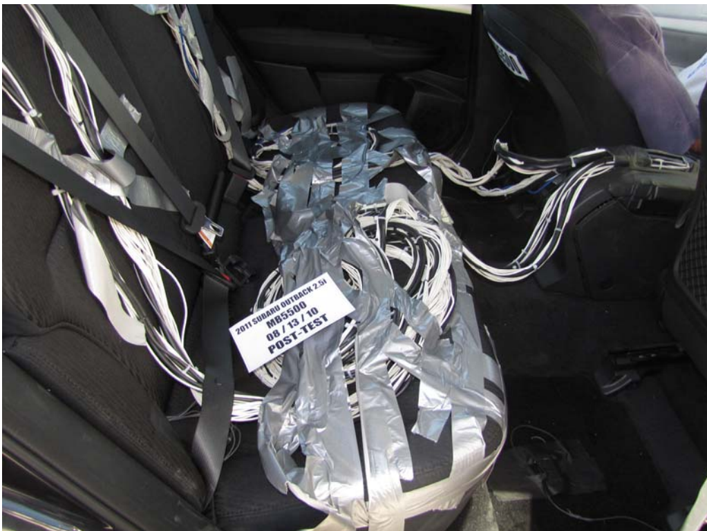
FIGURE 28. Post-Test Dummy Cable Routing
