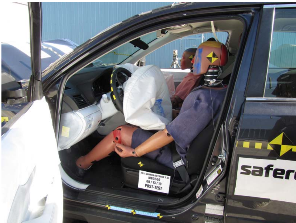
FIGURE 34. Post-Test Driver Dummy and Vehicle Interior View
