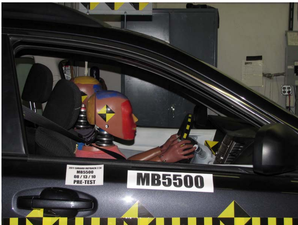
FIGURE 48. Pre-Test Passenger Dummy Window View
