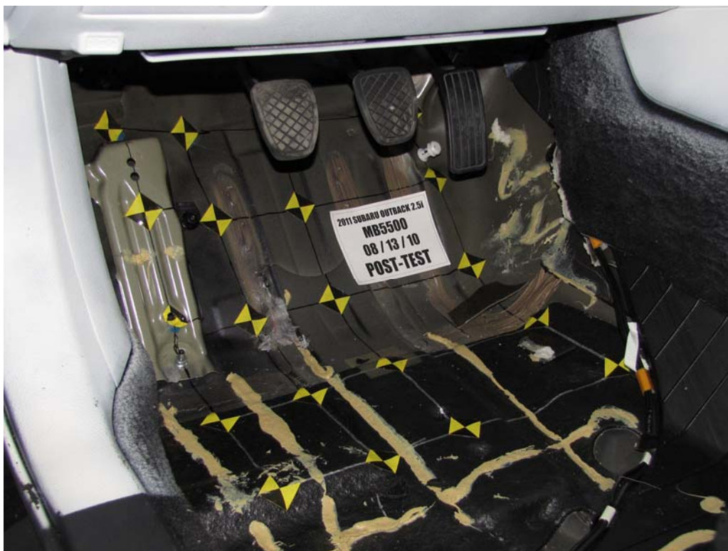
FIGURE 42. Post-Test Driver's Side Floorpan
