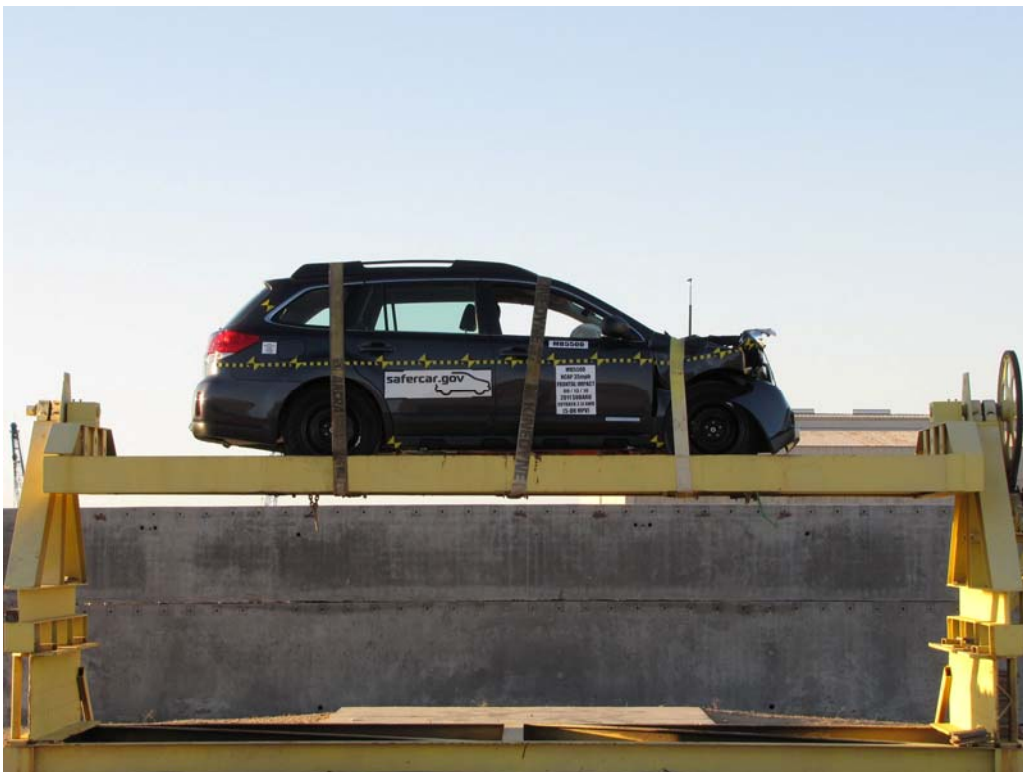
FIGURE 68. Vehicle at 360°on Static Rollover Device
