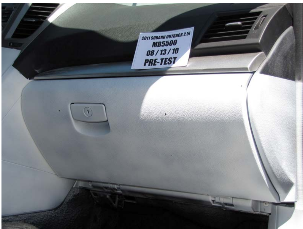
FIGURE 56. Pre-Test Passenger's Side Knee Bolster
