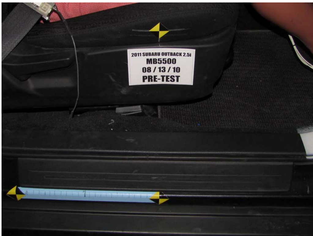
FIGURE 52. Pre-Test Passenger's Seat Fore-Aft Markings
