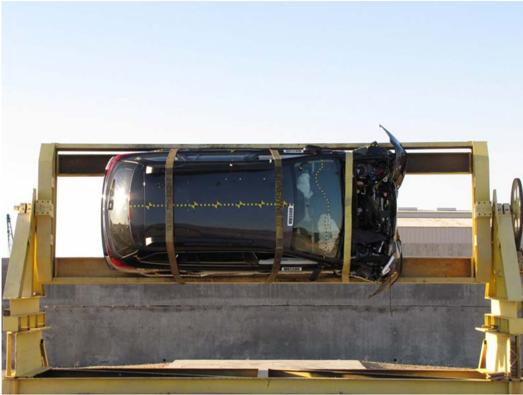
FIGURE 65. Vehicle at 90°on Static Rollover Device
