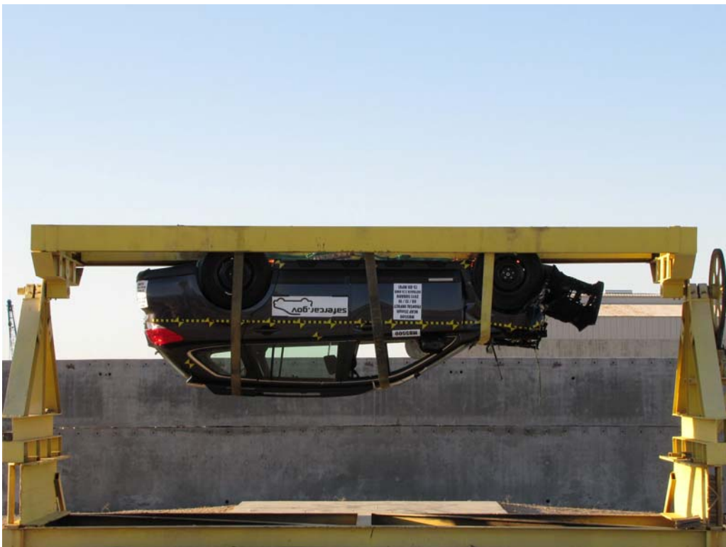
FIGURE 66. Vehicle at 180°on Static Rollover Device
