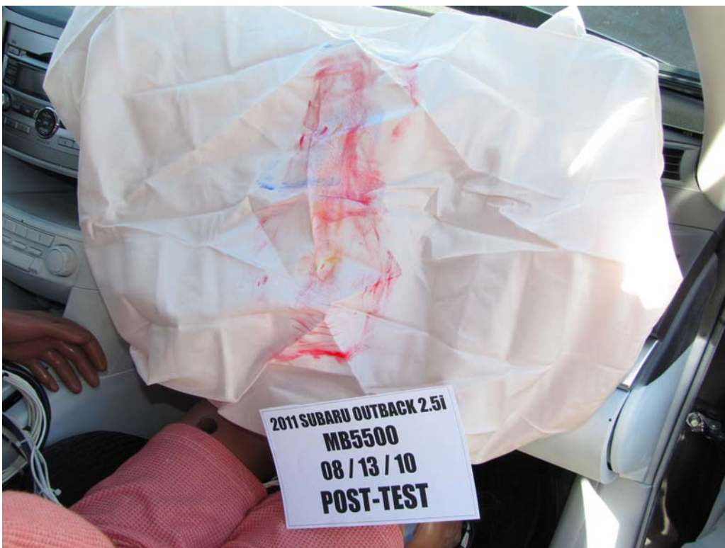
FIGURE 60. Post-Test Passenger Dummy Contact With Airbag
