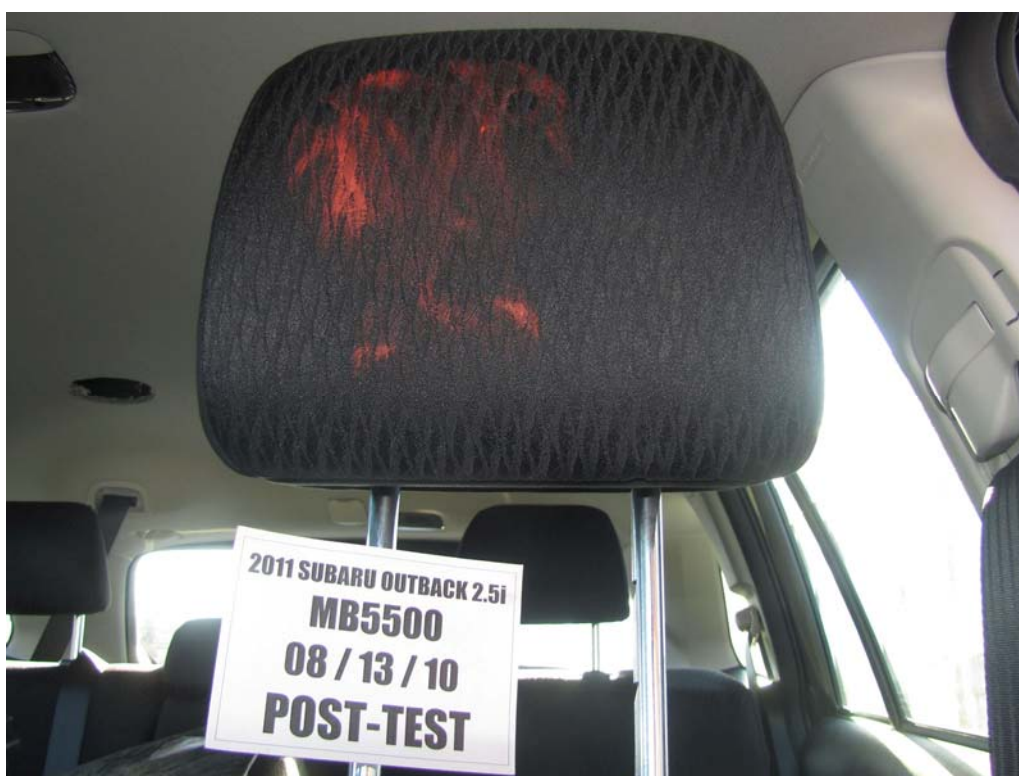
FIGURE 43a. Post-Test Driver Dummy Contact With Headrest
