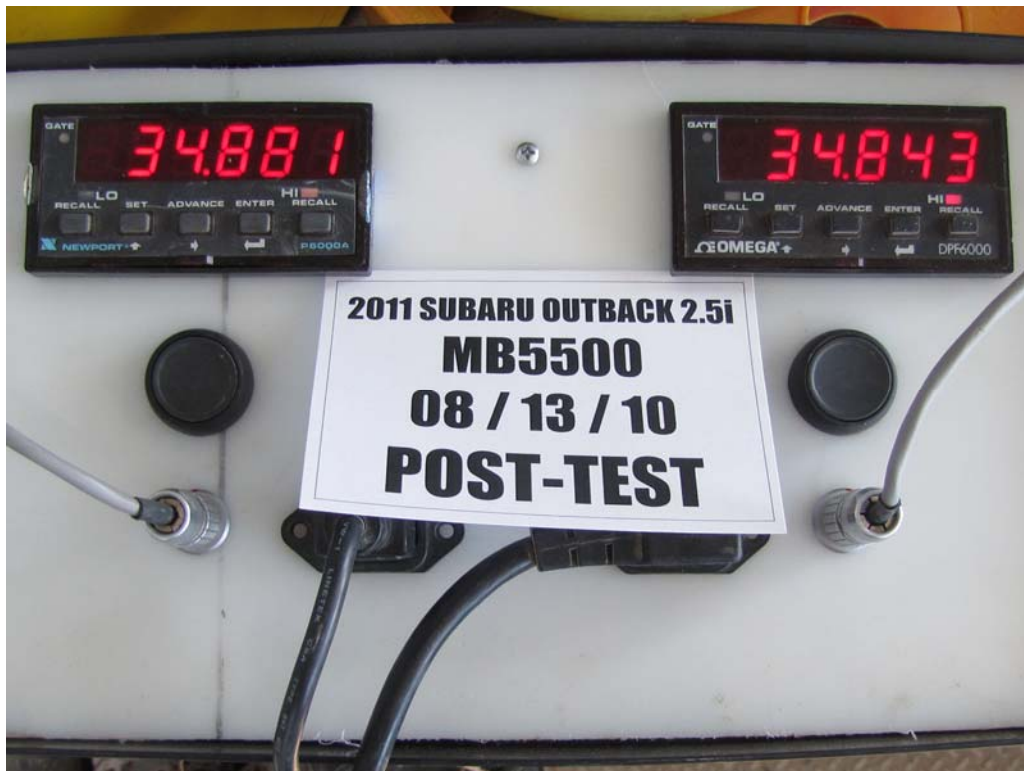
FIGURE 63. Post-Test Speed Trap Read Out
