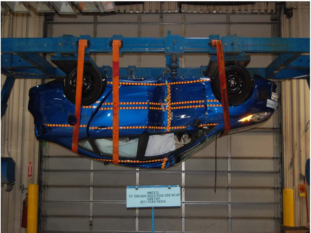
FMVSS No. 301/305 Rollover 180 Degrees
