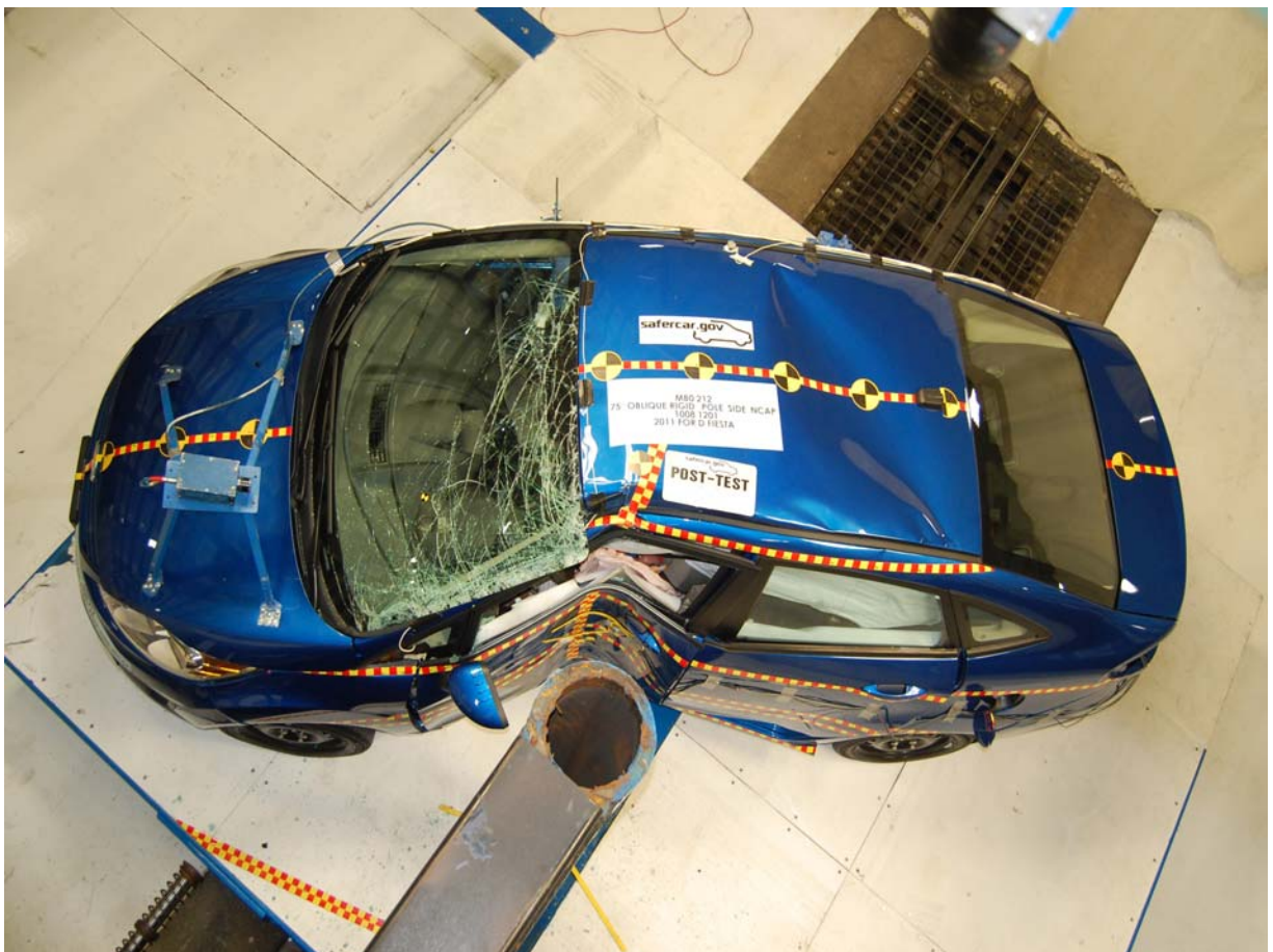
Post-Test Overhead View of Test Vehicle and Pole
