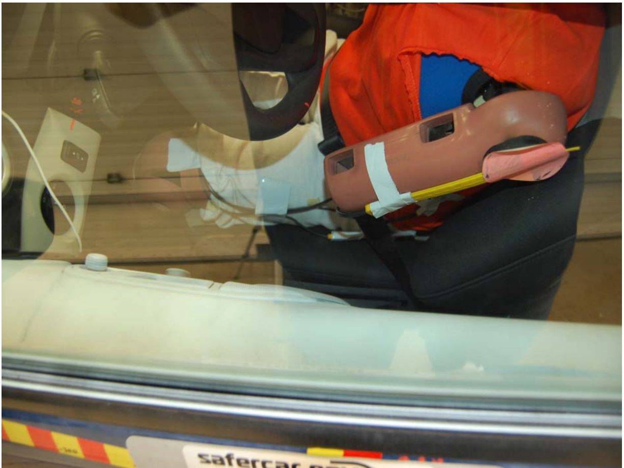
Pre-Test Dummy and Door Clearance View
