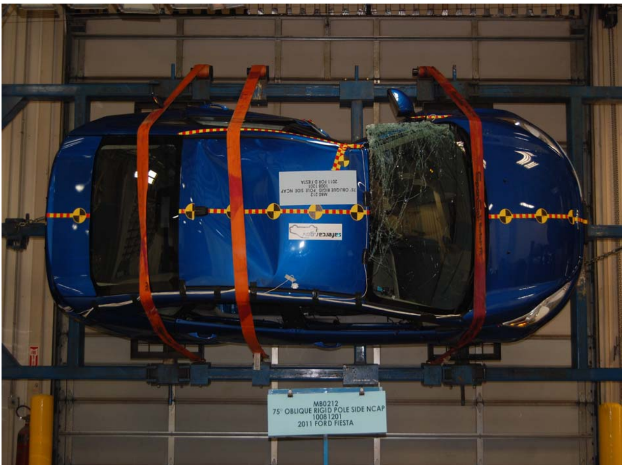
FMVSS No. 301/305 Rollover 270 Degrees
