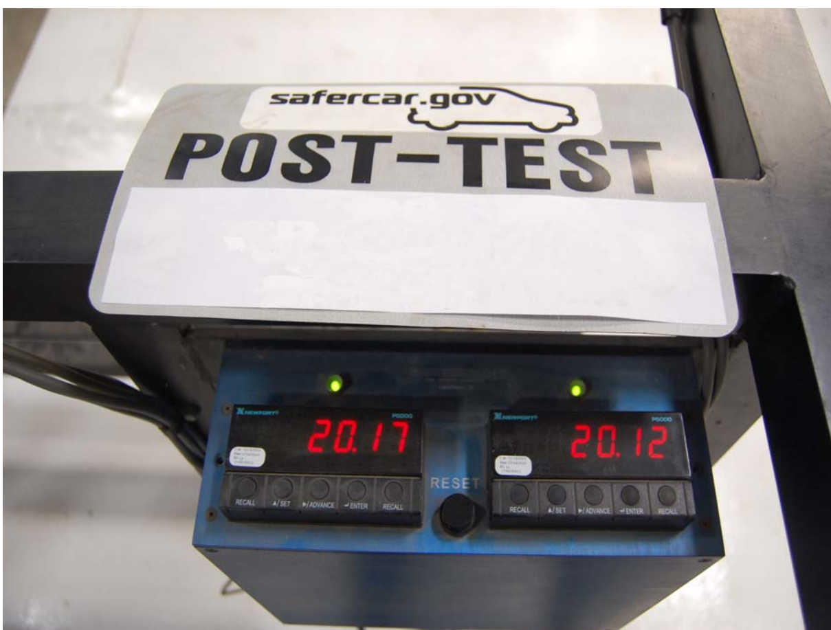
Post-Test Primary and Redundant Speed Trap Read-Out
