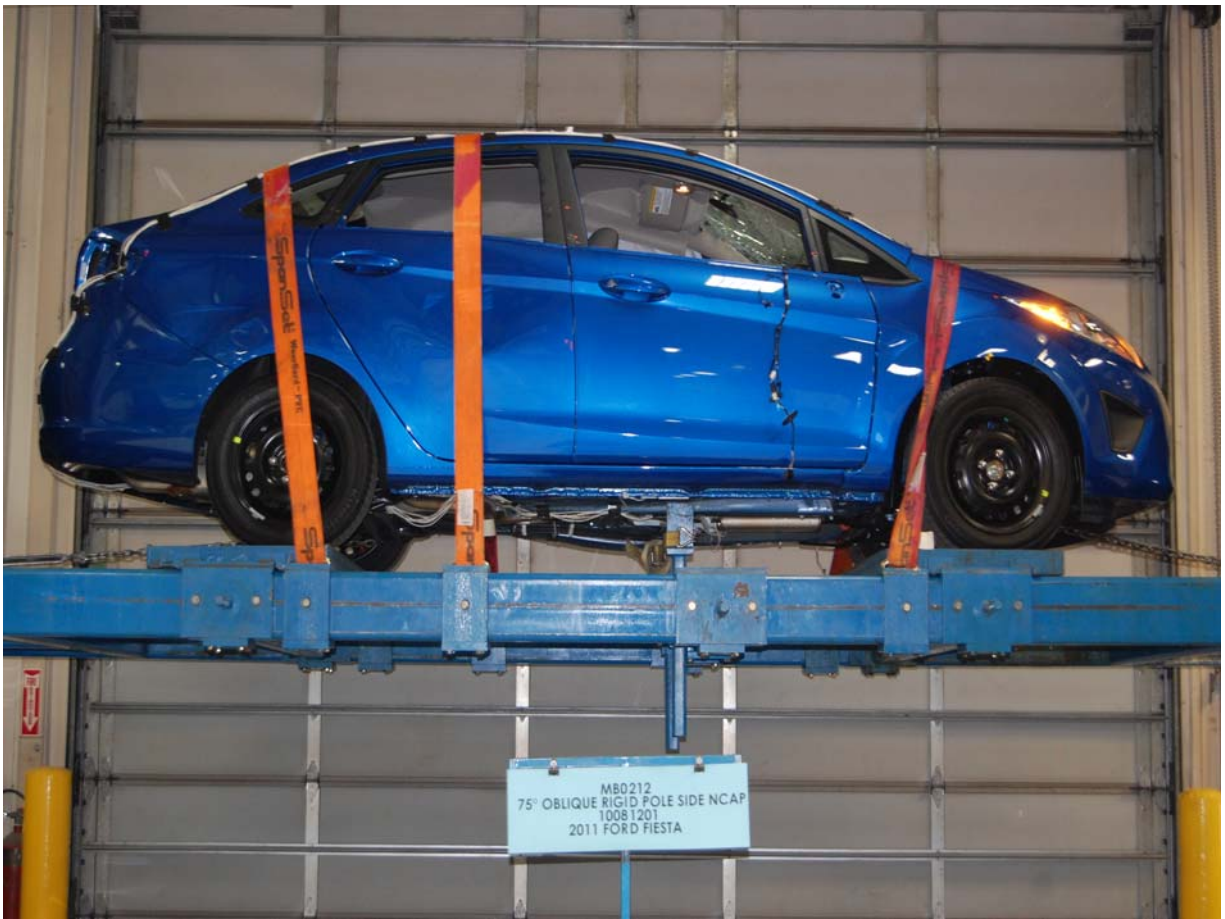
FMVSS No. 301/305 Rollover 360 Degrees
