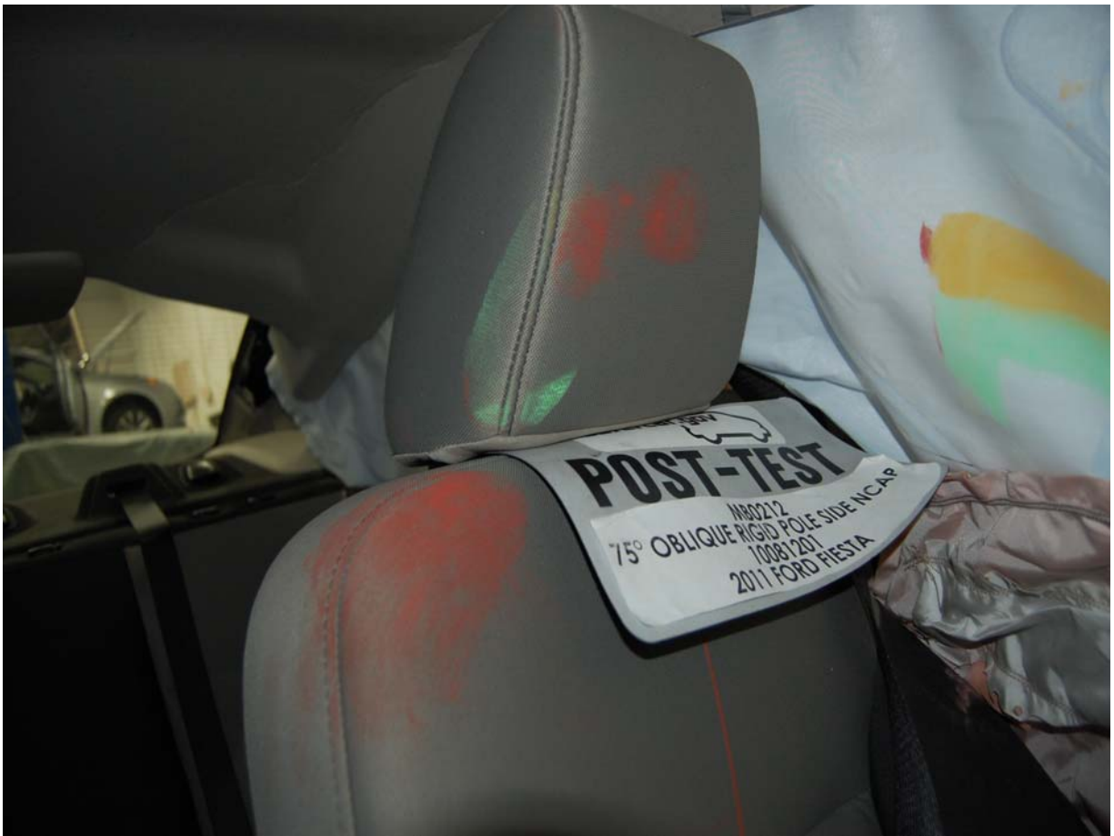
Post-Test Dummy Close-Up Head Contact with Vehicle View
