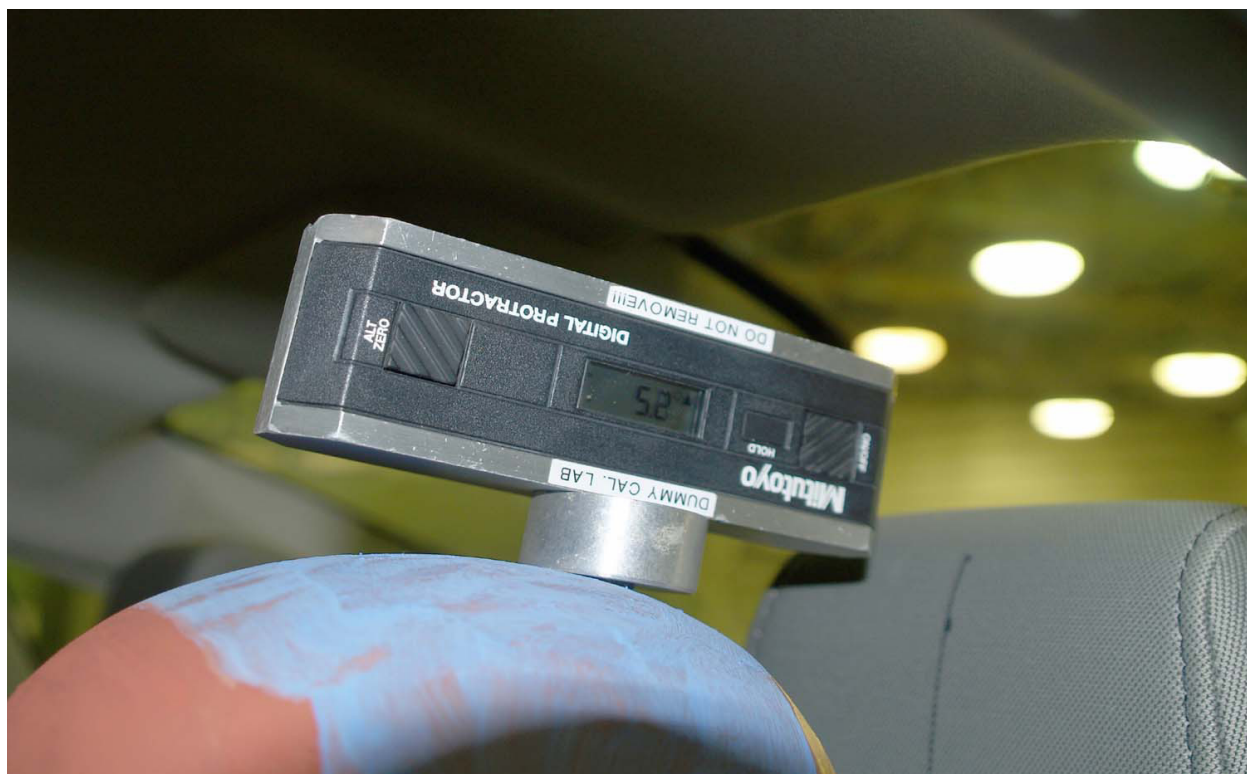
Figure A-61: Pre-Test View of Rear Passenger Dummy's Head Showing Dummy's Head is Level
