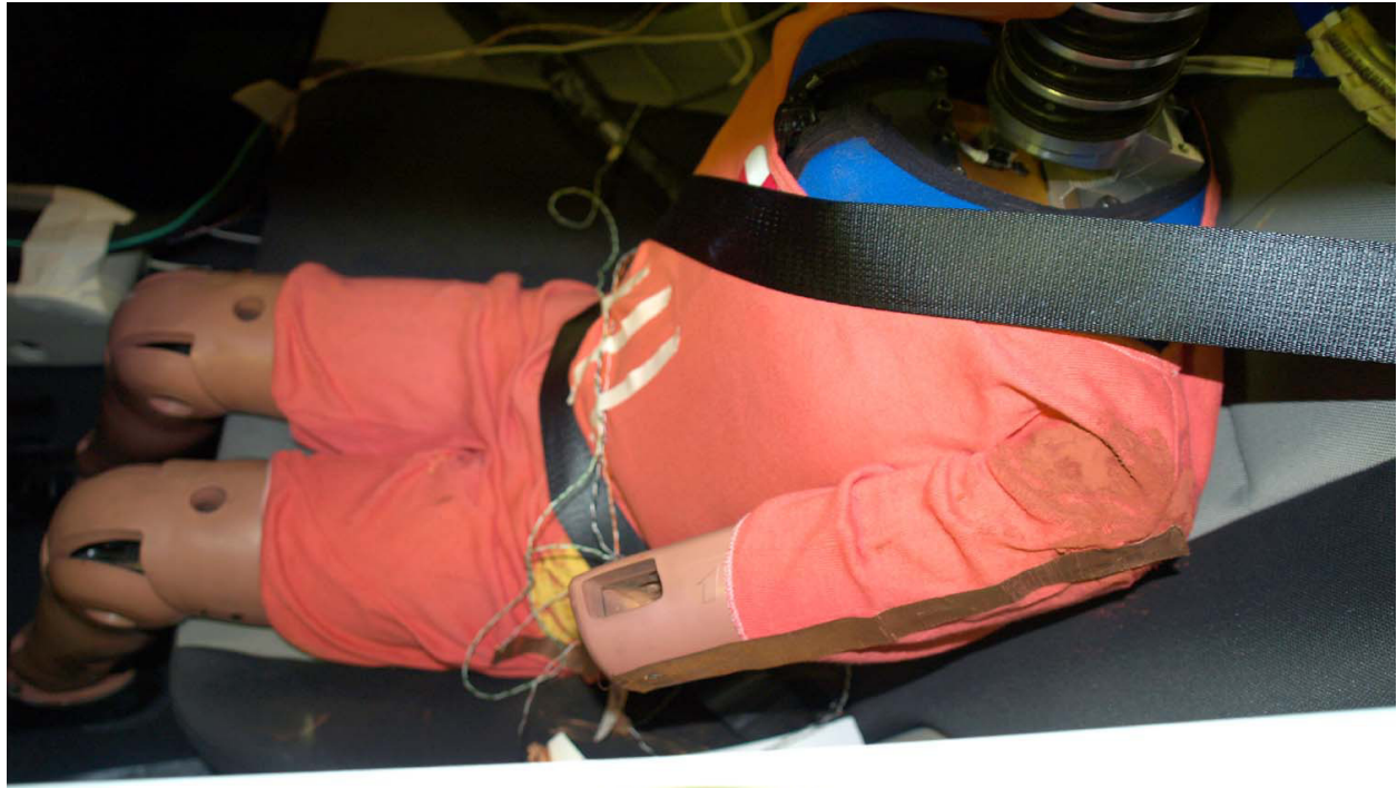
Figure A-67: Pre-Test Rear Passenger Dummy and Door Clearance View
