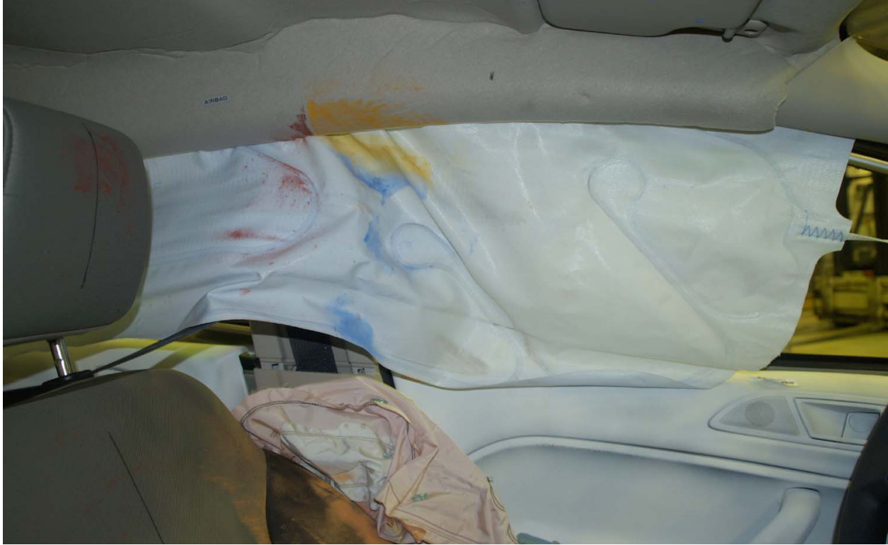
Figure A-47: Post-Test Driver Dummy Close-Up Head Contact with Vehicle View
