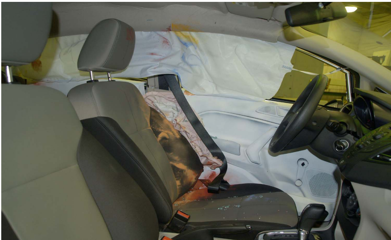
Figure A-46: Post-Test Driver Inner Door Panel Showing Driver Dummy Contact Locations
