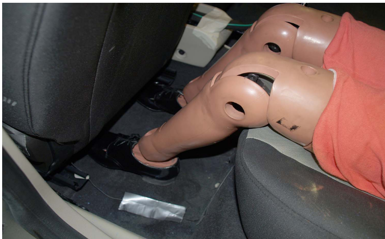
Figure A-62: Pre-Test Placement of Rear Passenger Dummy's Feet
