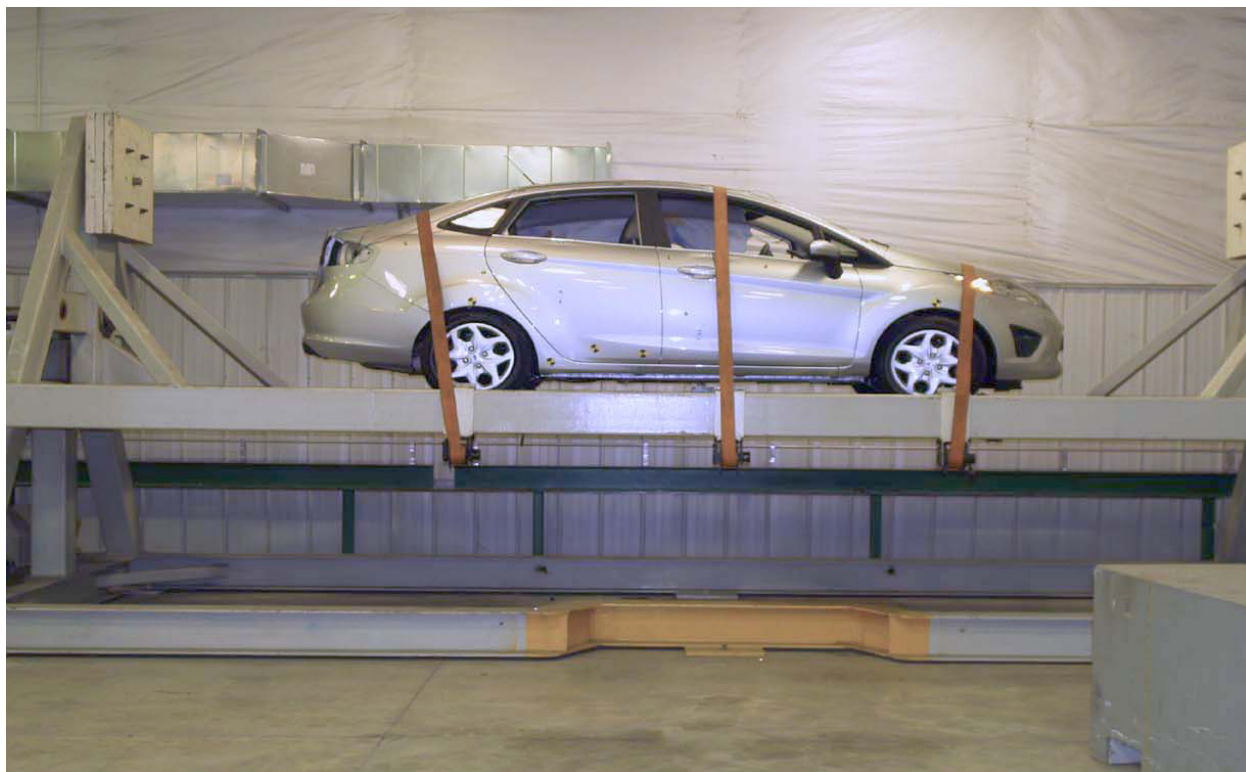
Figure A-97: FMVSS No. 301/305 Rollover 360°
