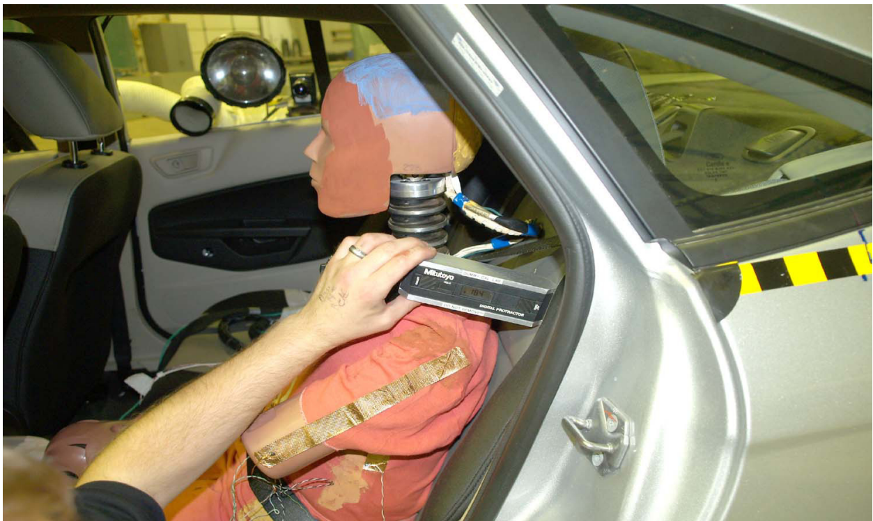
Figure A-66: Pre-Test Close-Up View of Rear Passenger Seat Back or Head Restraint
