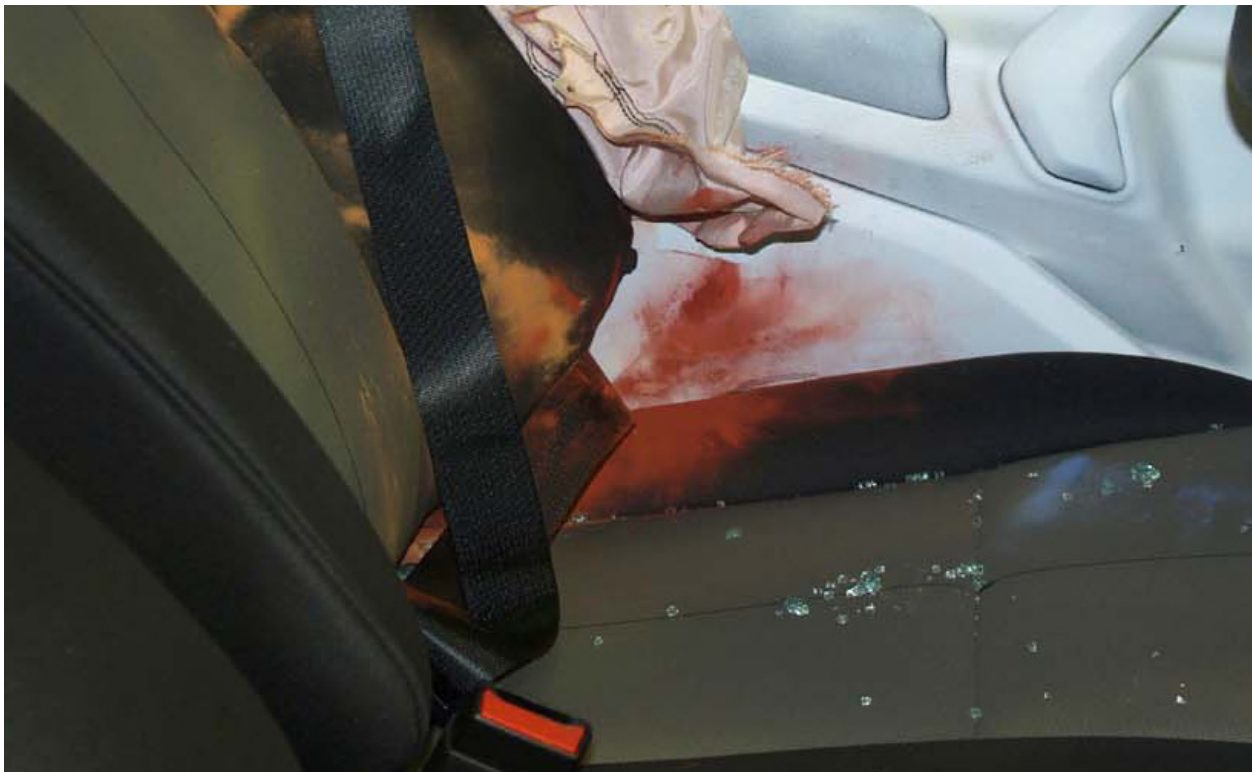
Figure A-52: Post-Test Driver Dummy Close-Up Pelvis Contact With Side Airbag View
