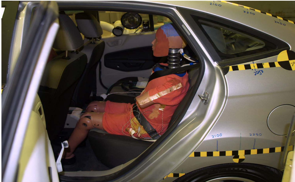
Figure A-53: Pre-Test Left Side View of Rear Passenger Dummy Showing Belt, Chalking, and Contact Switches
