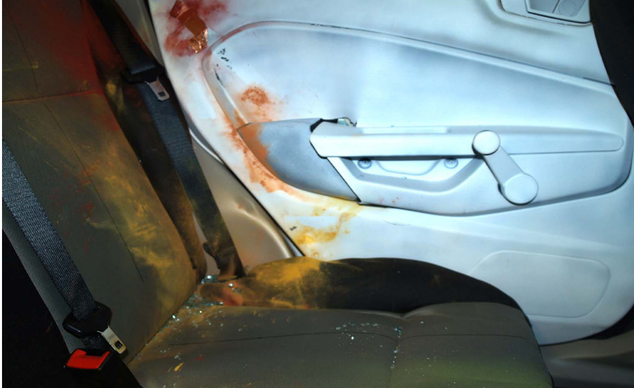
Figure A-77: Post-Test Rear Passenger Dummy Close-Up Pelvis Contact View
