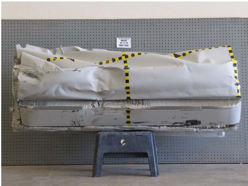
FIGURE 82. Post-Test Front View of MDB Impactor Face
