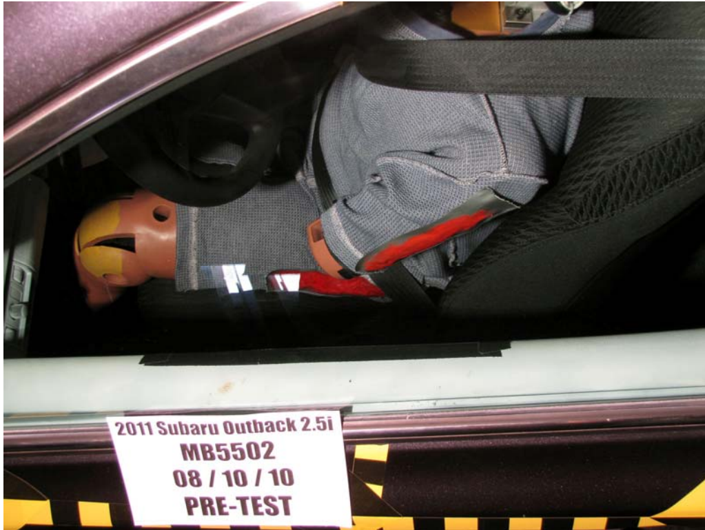
FIGURE 39. Pre-Test Driver Dummy and Door Clearance
