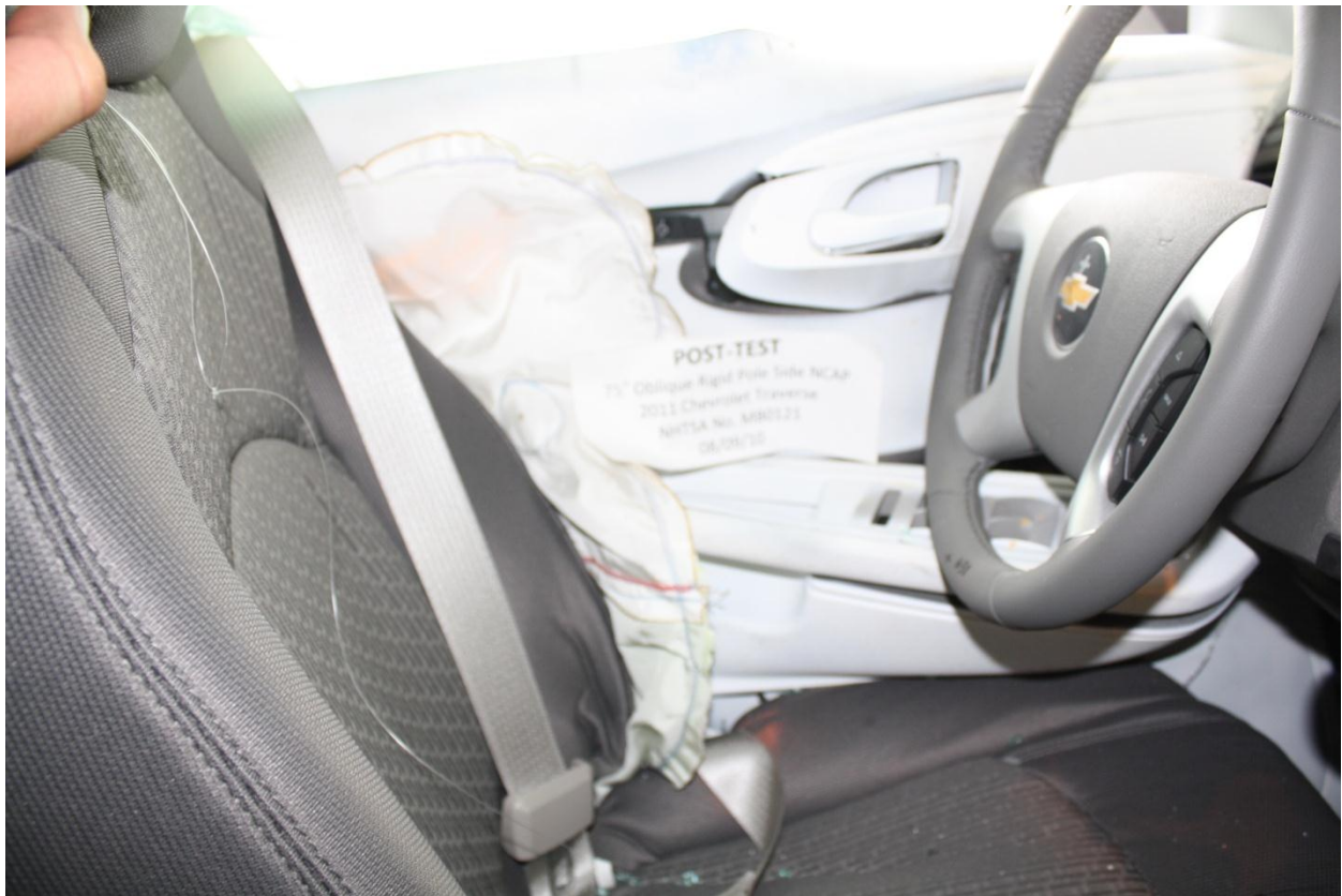
Figure A-48: Post-Test Dummy Close-Up Torso Contact with Side Airbag View
