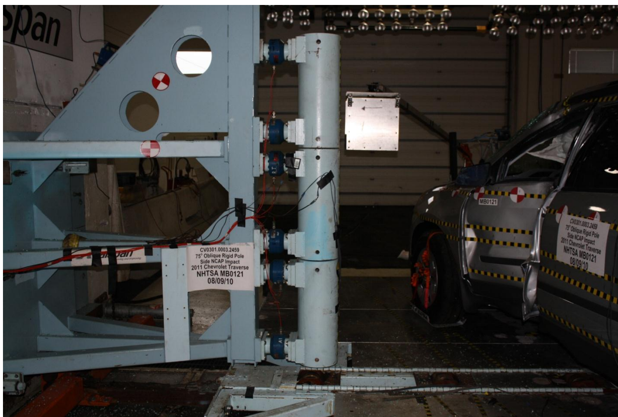
Figure A-58: Post-Test Pole Barrier Side View
