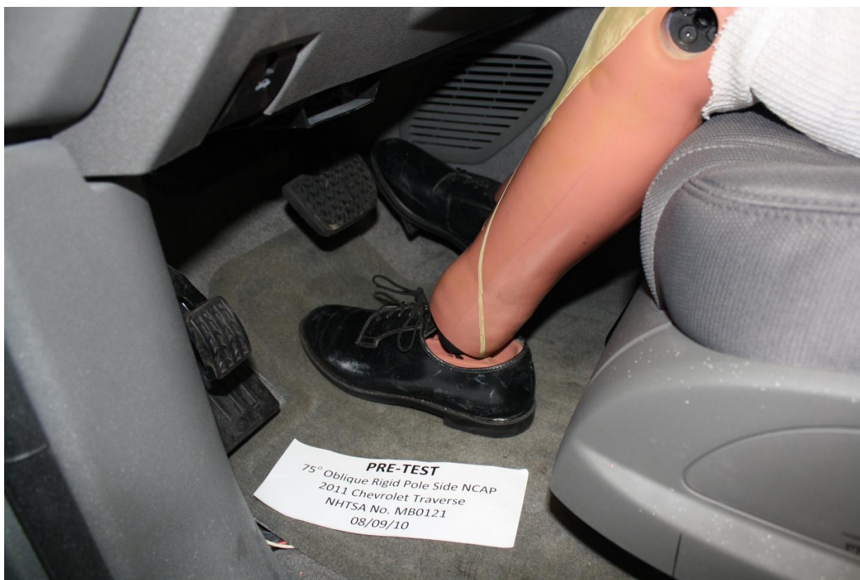
Figure A-32: Pre-Test Placement of Dummy's Feet
