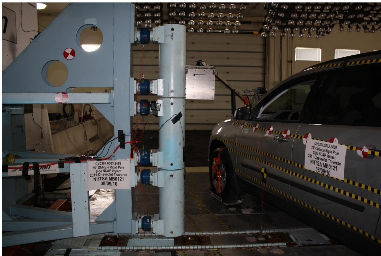
Figure A-57: Pre-Test Pole Barrier Side View
