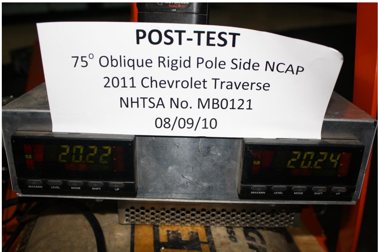
Figure A-60: Post-Test Primary and Redundant Speed Trap Read-Out
