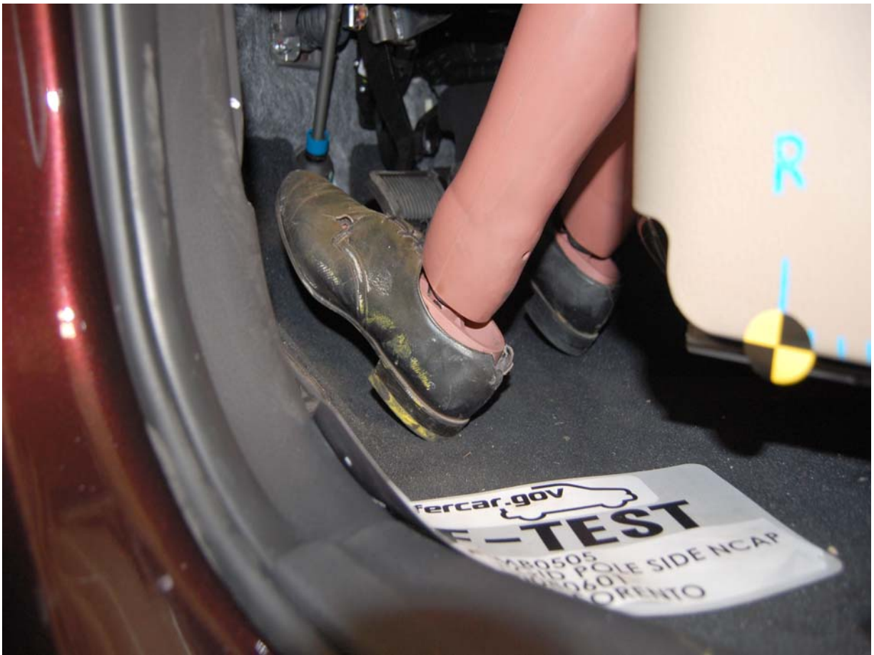
Pre-Test Placement of Dummy's Feet
