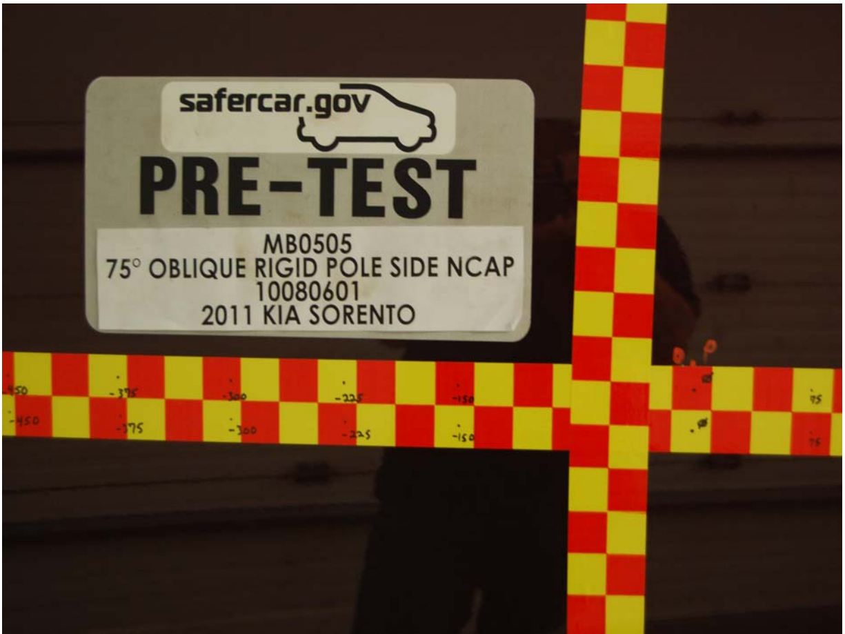
Pre-Test Close-Up View of Impact Point Target
