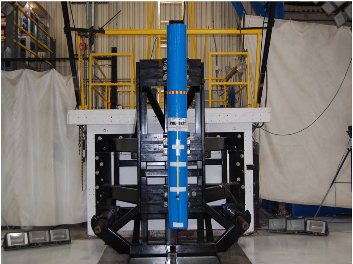
Pre-Test Pole Barrier Front View
