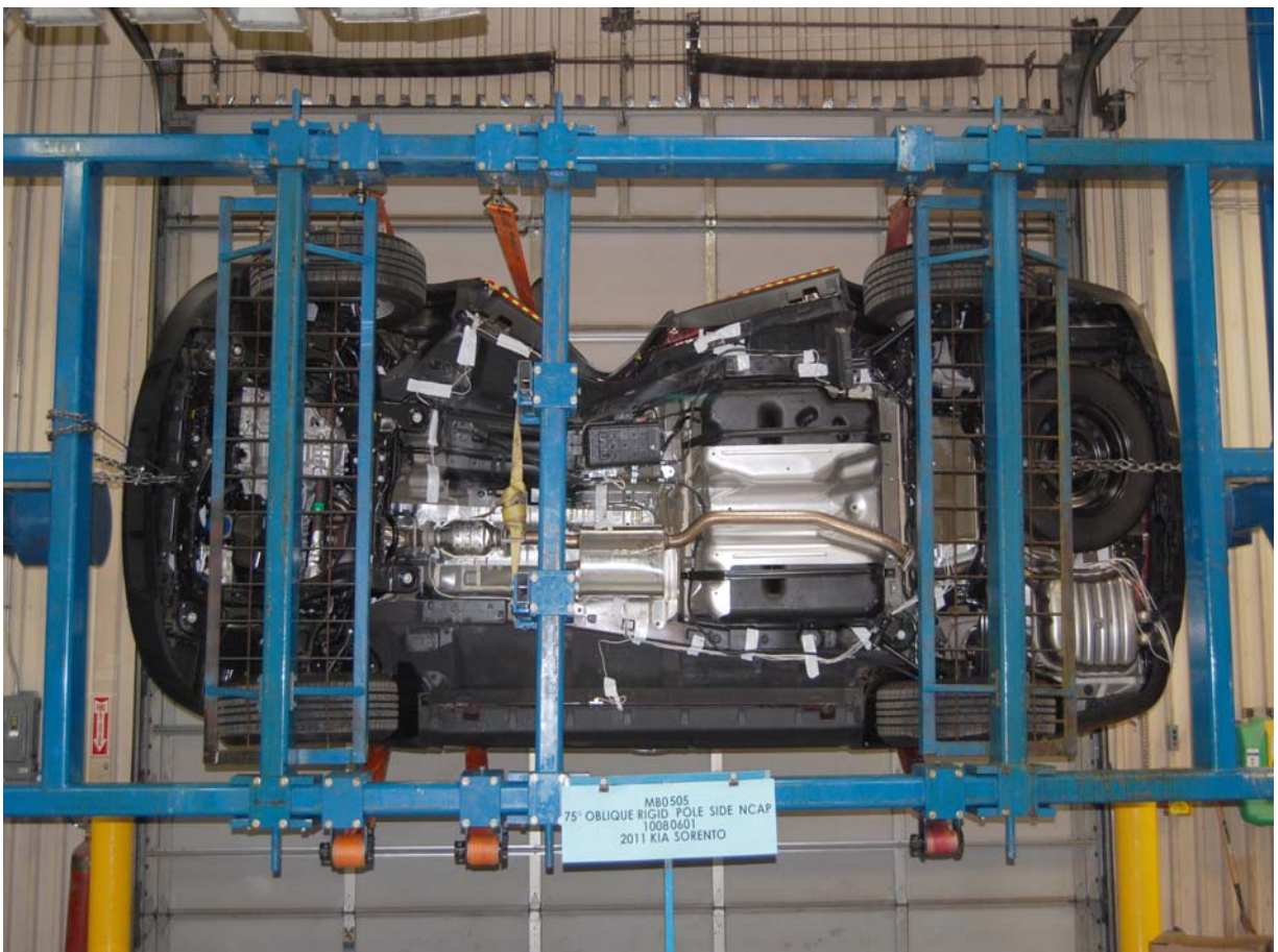
FMVSS No. 301/305 Rollover 270 Degrees
