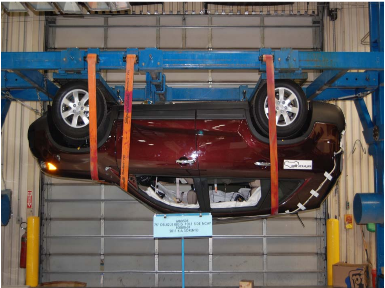
FMVSS No. 301/305 Rollover 180 Degrees
