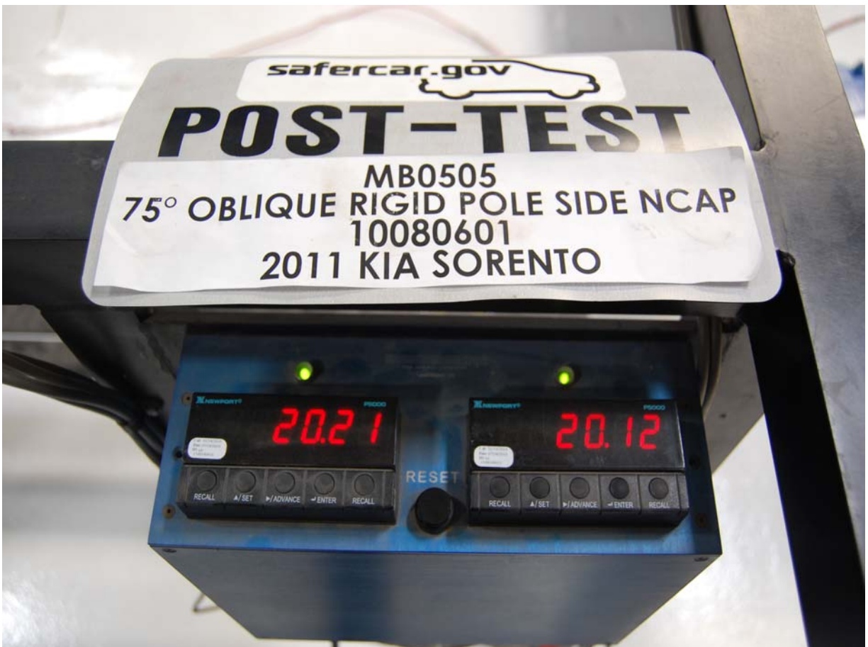
Post-Test Primary and Redundant Speed Trap Read-Out
