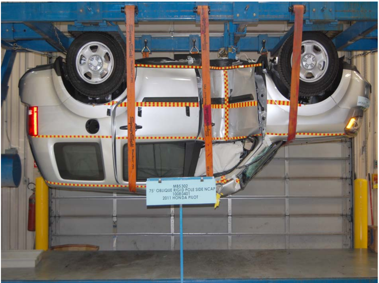
FMVSS No. 301/305 Rollover 180 Degrees
