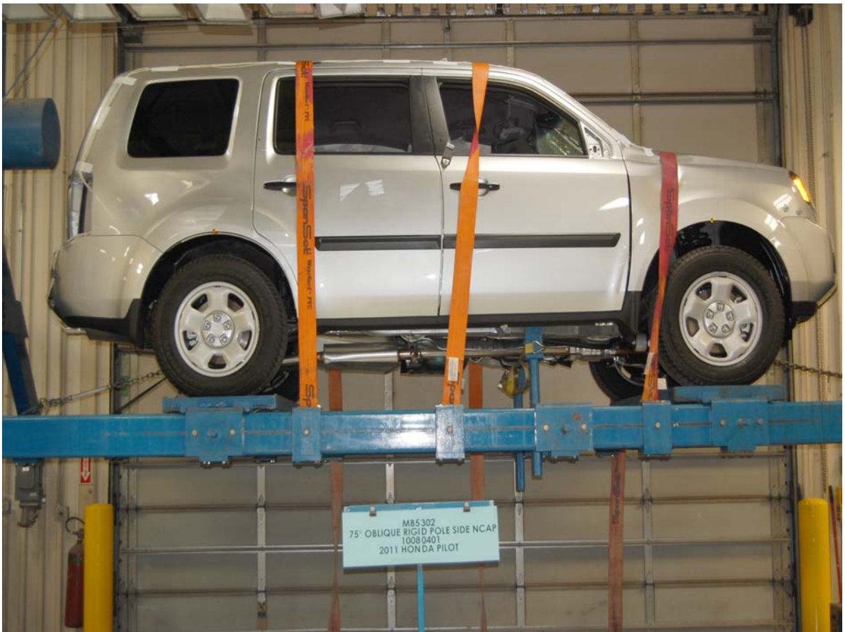
FMVSS No. 301/305 Rollover 360 Degrees
