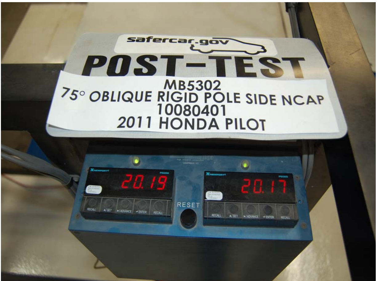
Post-Test Primary and Redundant Speed Trap Read-Out
