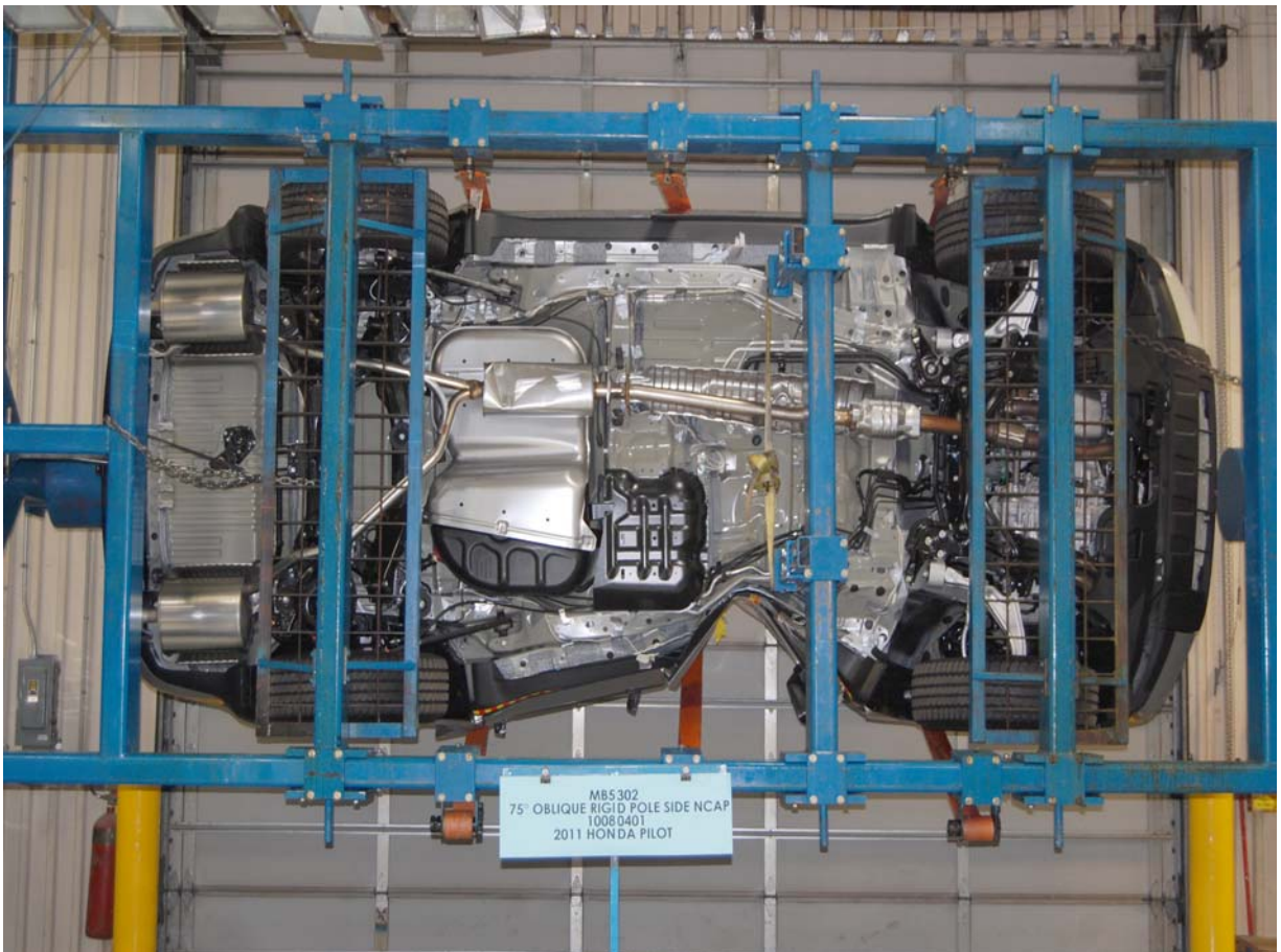
FMVSS No. 301/305 Rollover 90 Degrees
