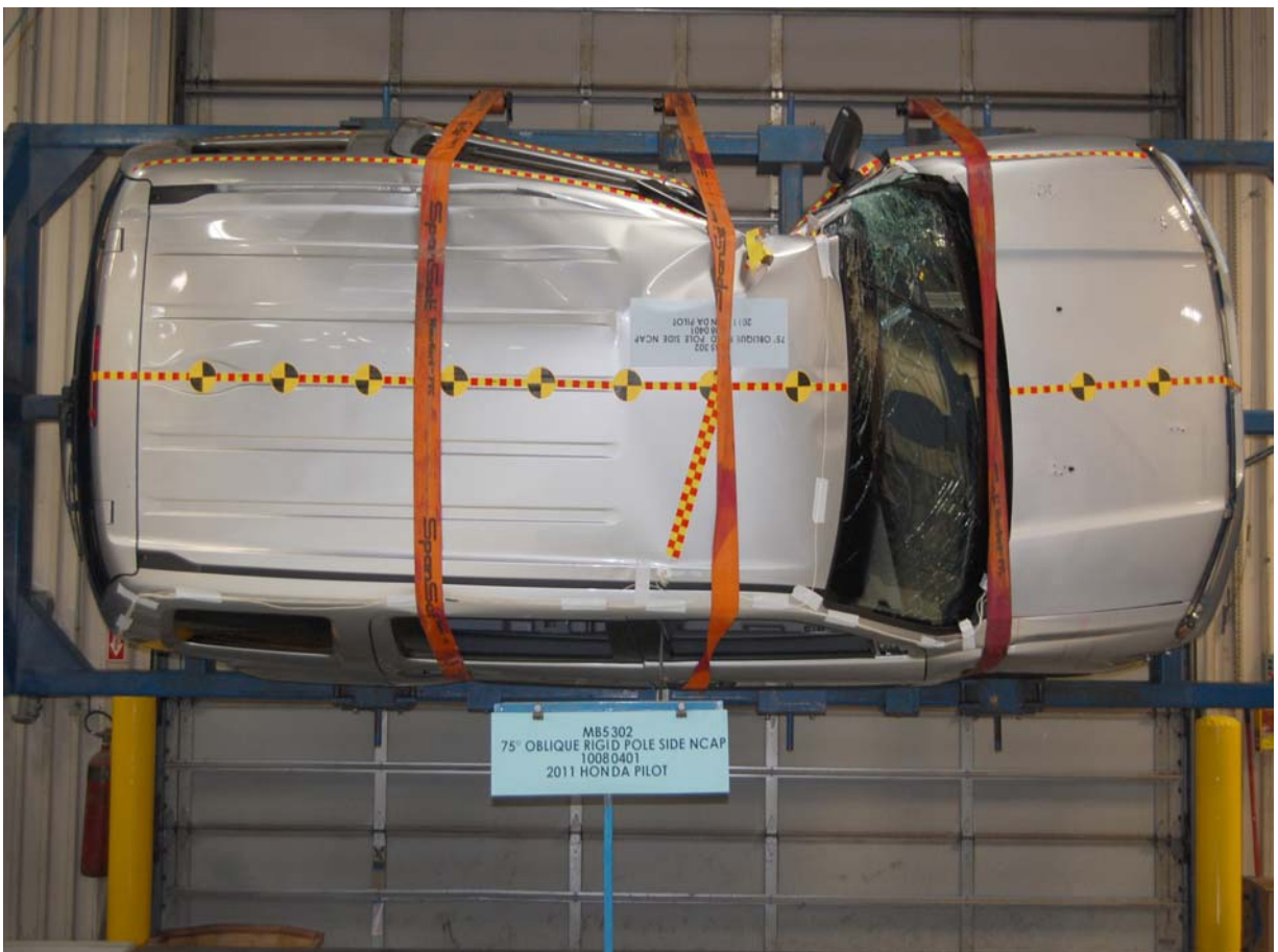
FMVSS No. 301/305 Rollover 270 Degrees
