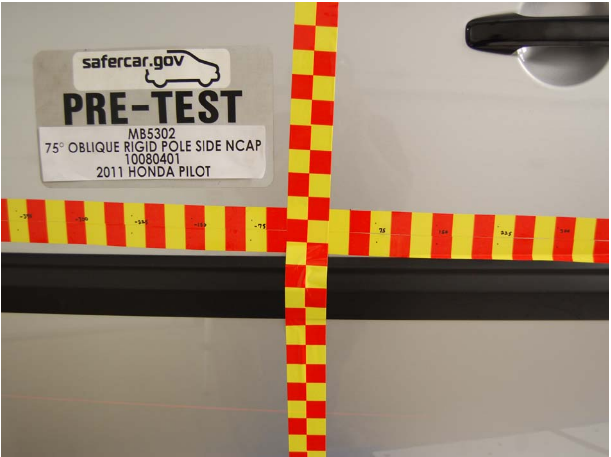
Pre-Test Close-Up View of Impact Point Target
