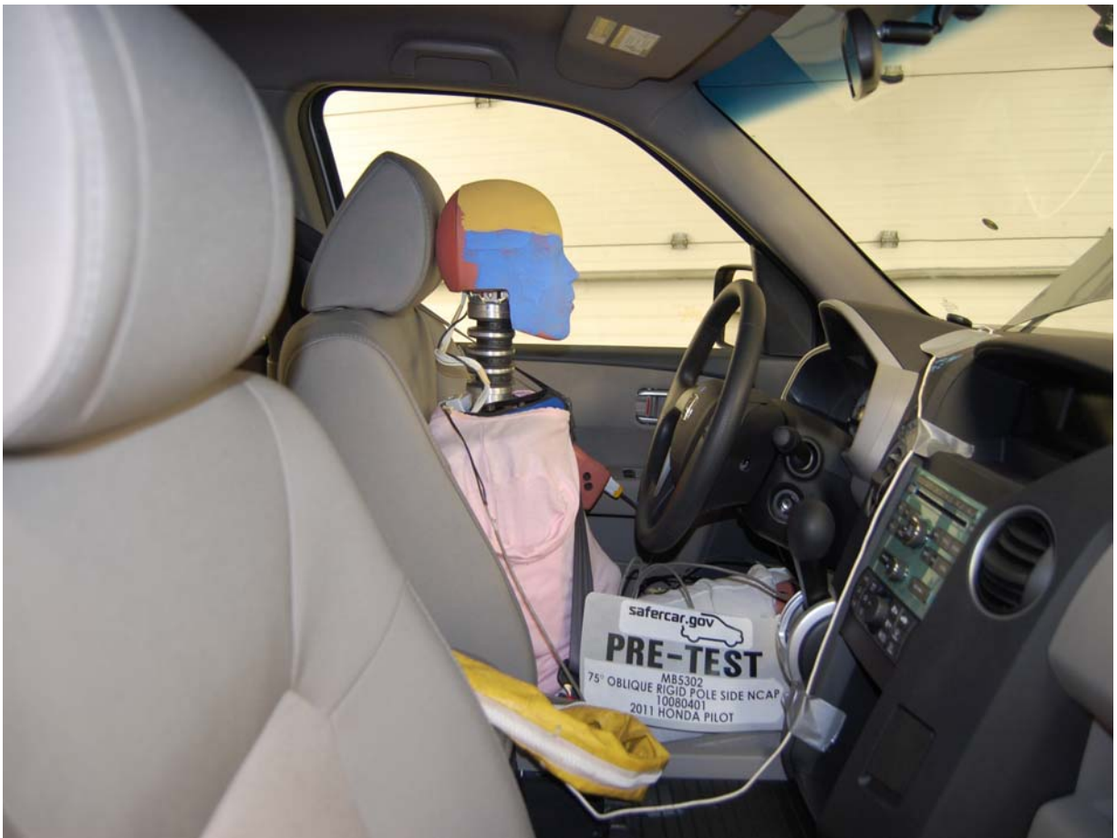
Pre-Test Right Side View of Dummy and Front Seat Occupant Compartment
