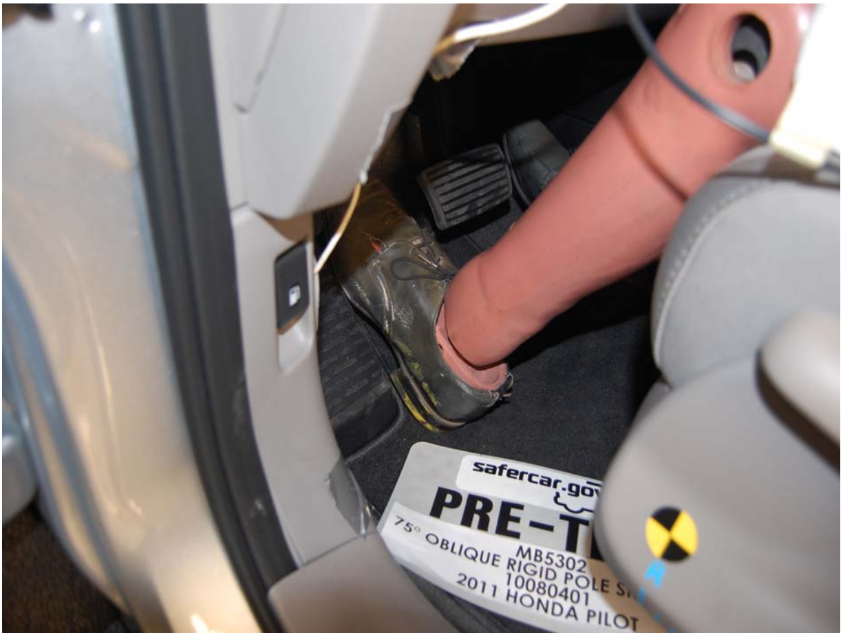
Pre-Test Placement of Dummy's Feet
