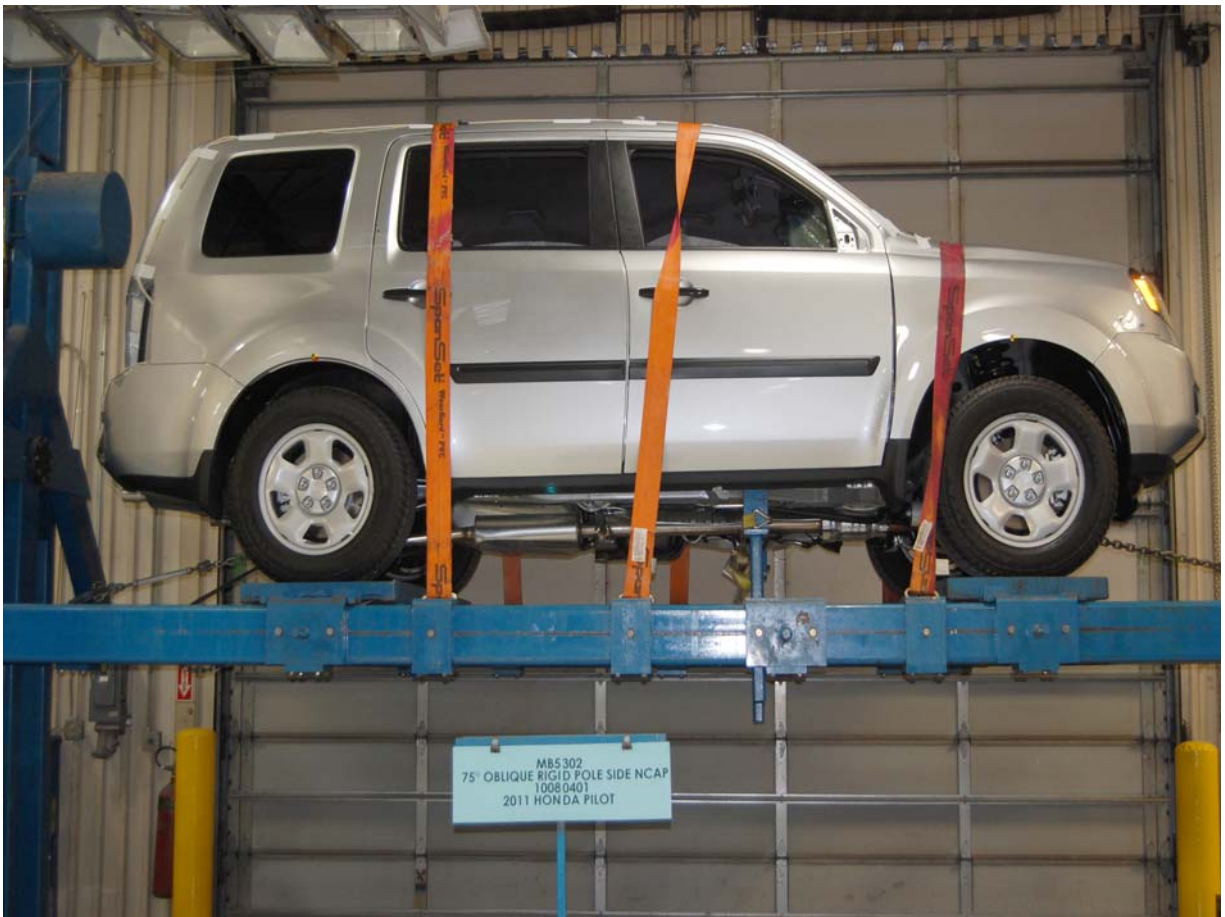
FMVSS No. 301/305 Rollover 0 Degrees
