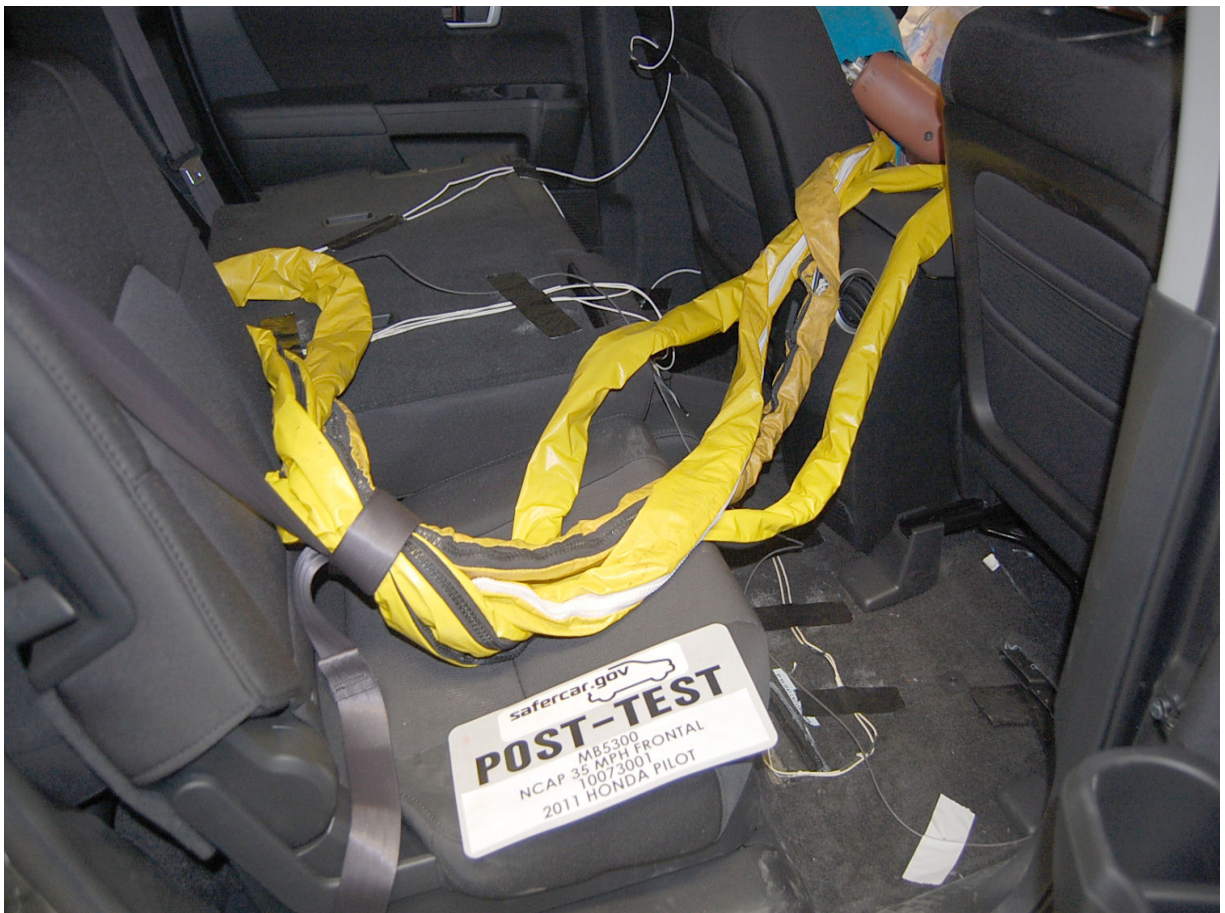
Post-Test Dummy Cable Routing
