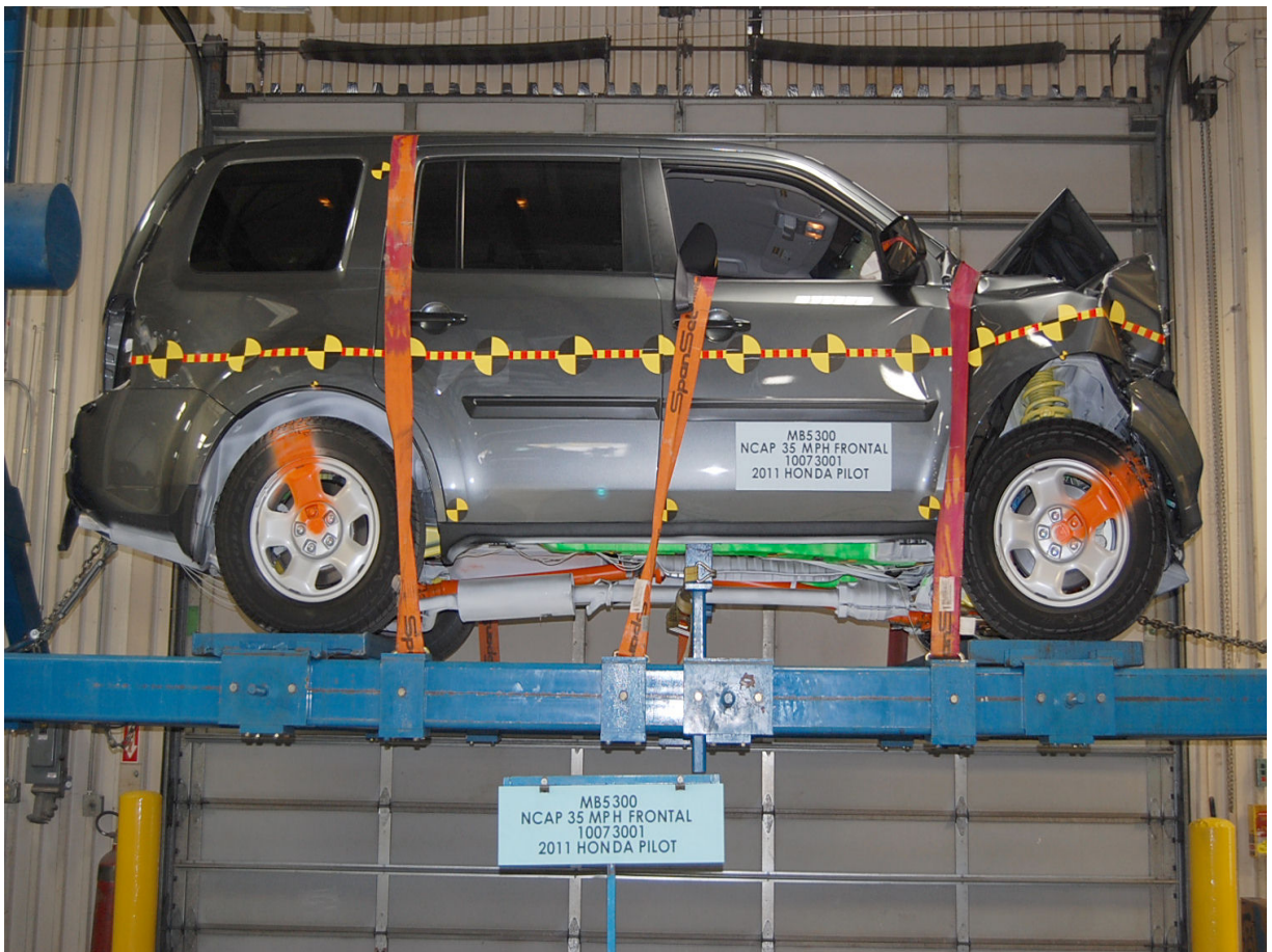
Vehicle at 360 Degrees on Static Rollover Device
