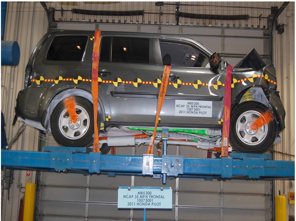
Vehicle at 0 Degrees on Static Rollover Device
