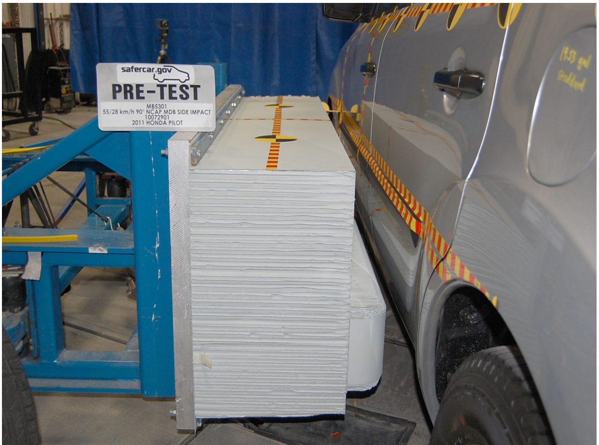
Pre-Test Right Side View of MDB Positioned Against Side of Target Vehicle at Ideal Impact Point
