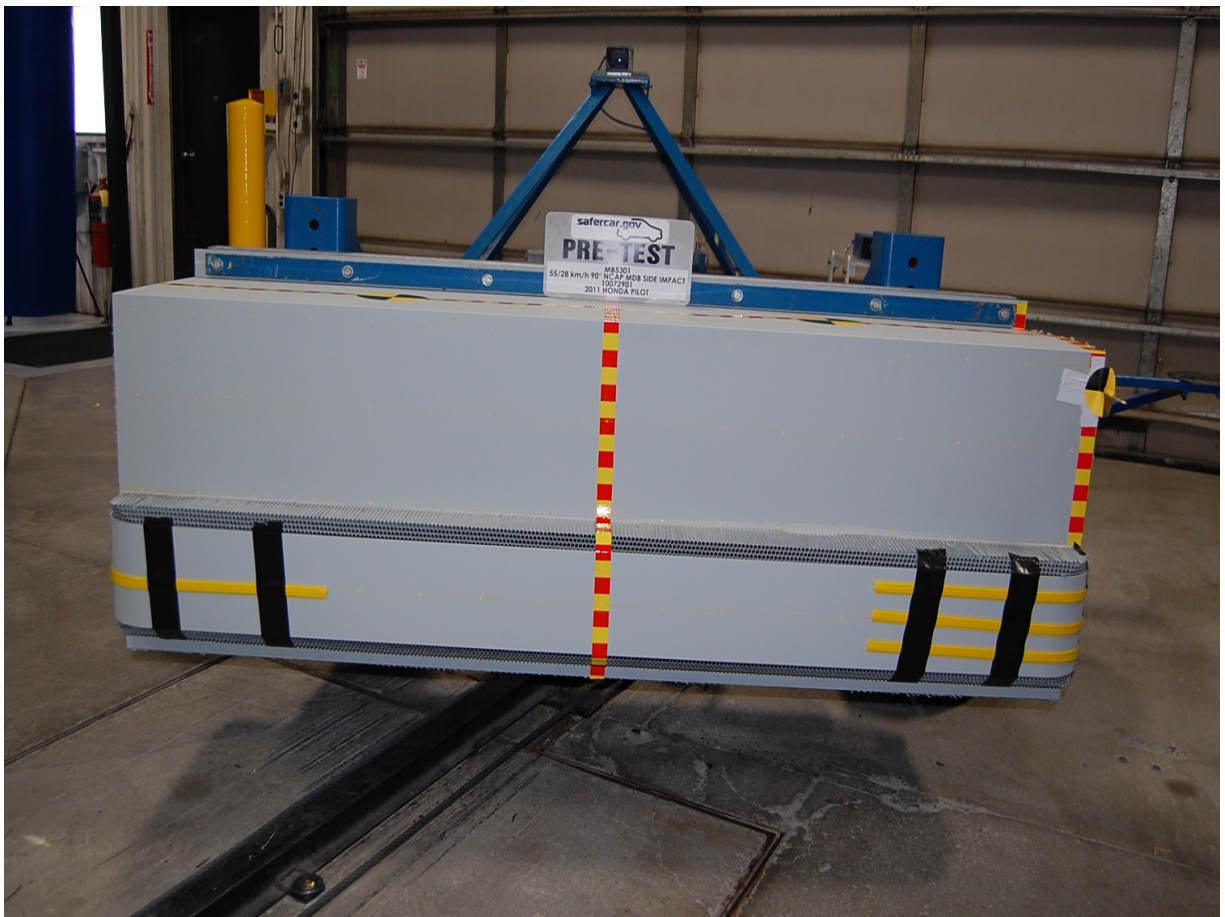
Pre-Test Front View of MDB Impactor Face
