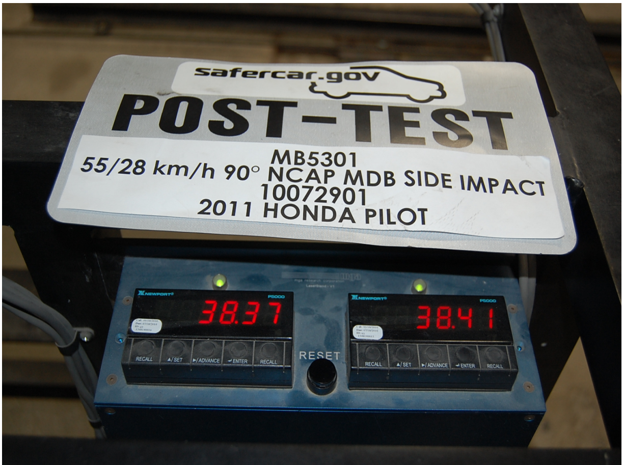
Post-Test Primary and Redundant Speed Trap Read-Out
