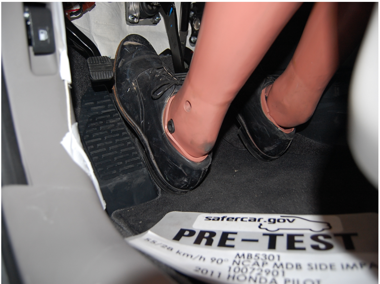
Pre-Test Placement of Driver Dummy's Feet
