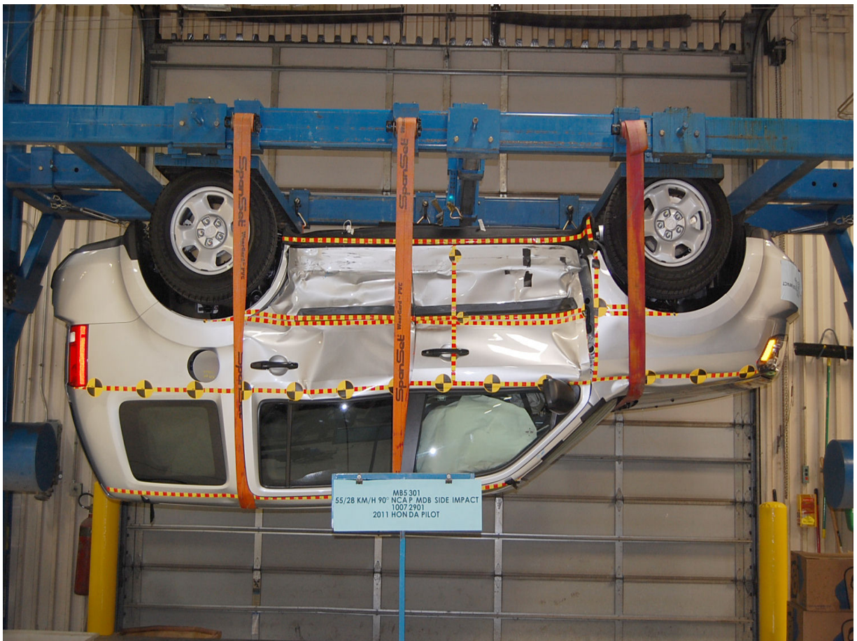
FMVSS No. 301/305 Rollover 180 Degrees
