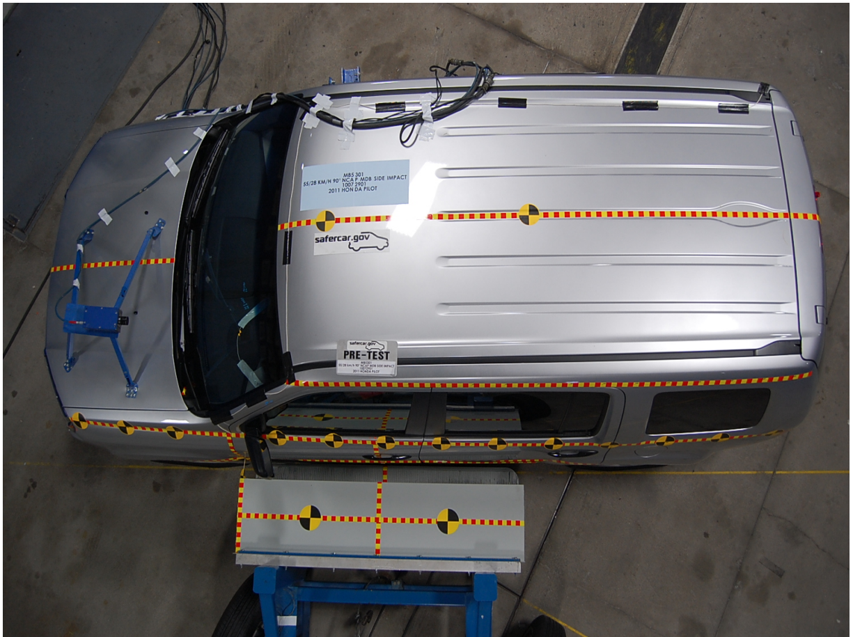
Pre-Test Overhead View of Test Vehicle with MDB Positioned Against Side of Target Vehicle at Ideal Impact Point
