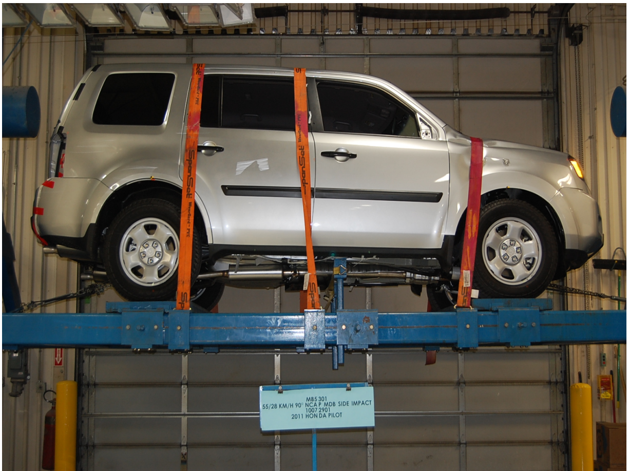
FMVSS No. 301/305 Rollover 0 Degrees
