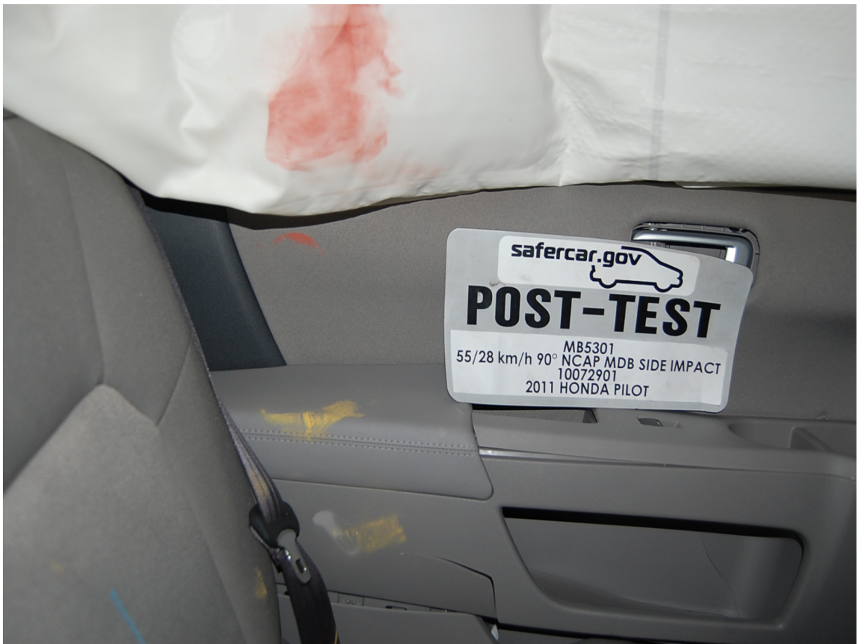
Post-Test Rear Passenger Dummy Close-up Torso Contact with Vehicle View
