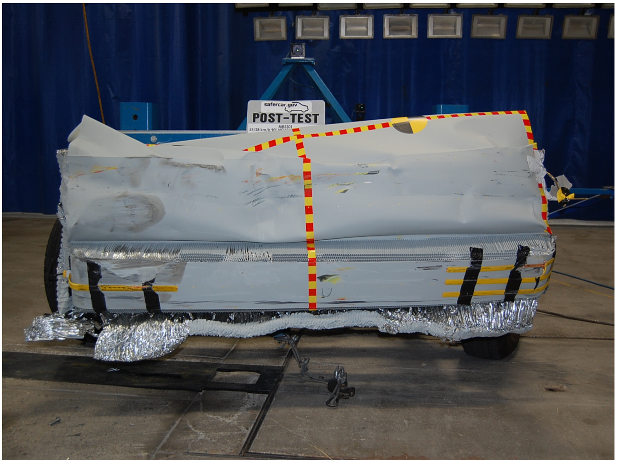
Post-Test Front View of MDB Impactor Face
