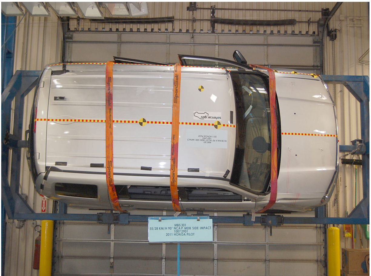
FMVSS No. 301/305 Rollover 270 Degrees
