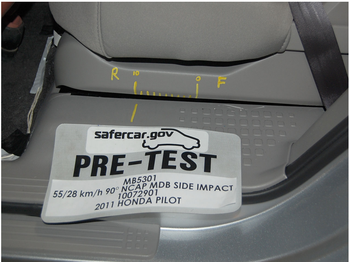
Pre-Test Close-Up Left Side View of Rear Passenger Seat Track Showing Test Position
