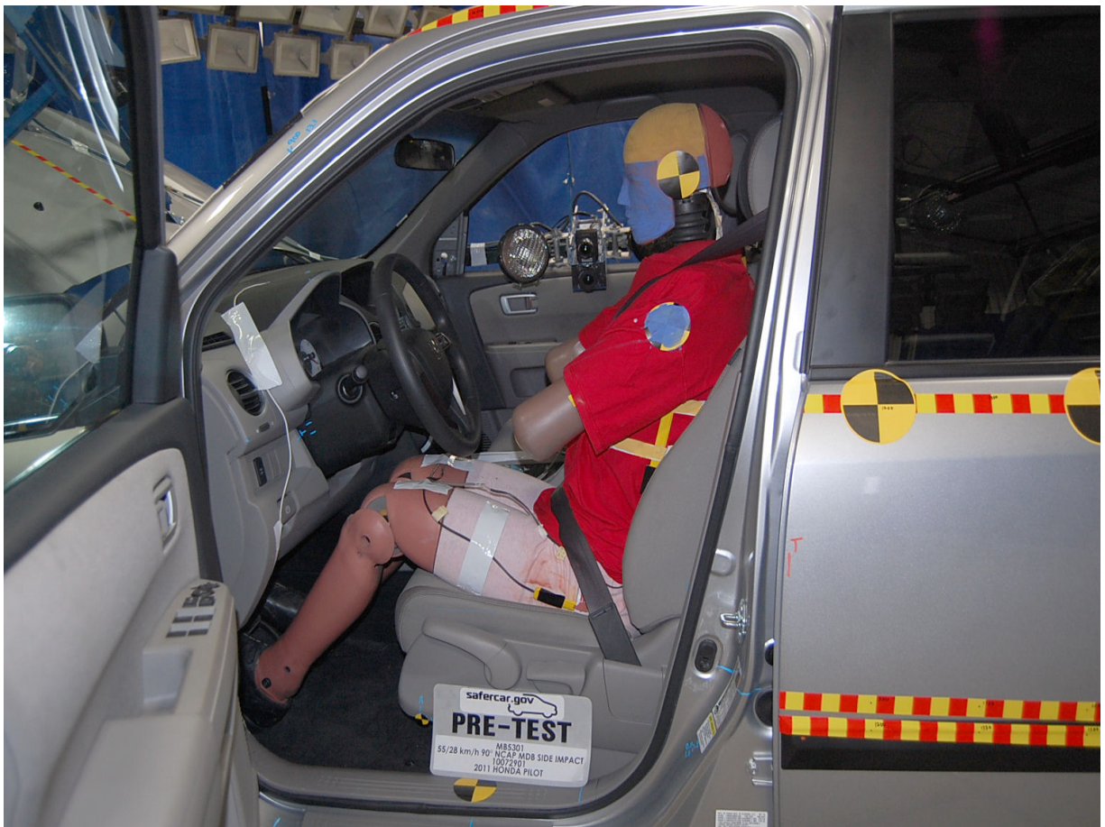
Pre-Test Left Side View of Driver Dummy Showing Belt, Chalking, and Contact Switches (Door Open)
