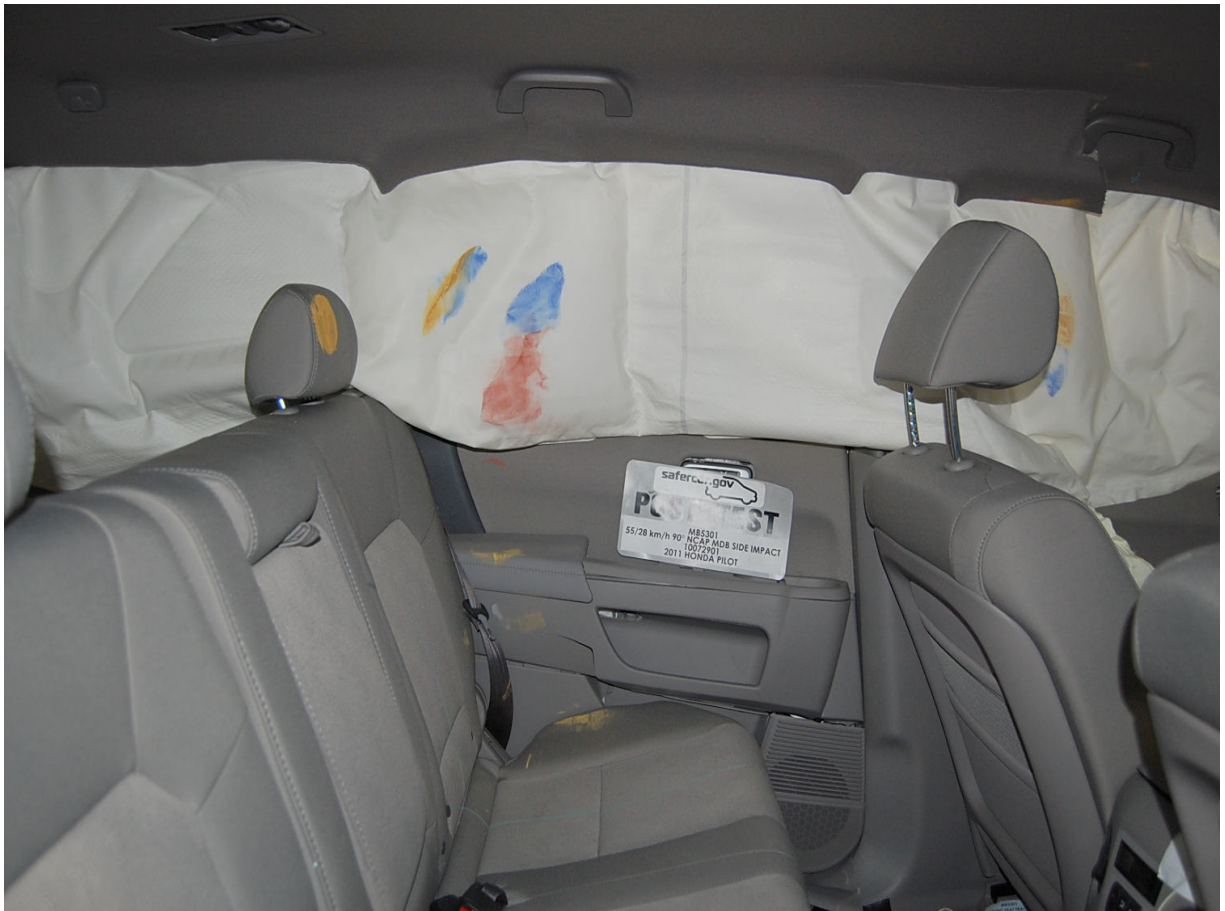
Post-Test Rear Passenger Inner Door Panel View Showing Rear Passenger Dummy Contact Locations
