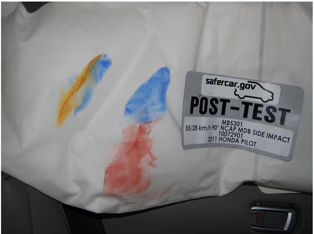
Post-Test Rear Passenger Dummy Close-up Head Contact with Side Airbag View
