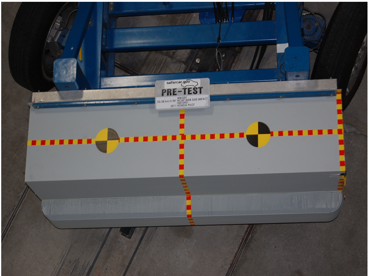
Pre-Test Top View of MDB Impactor Face
