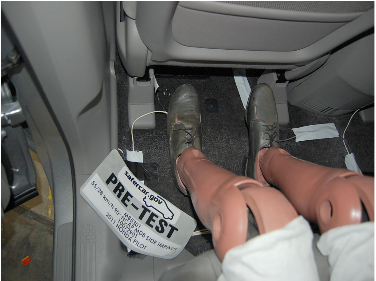
Pre-Test Placement of Rear Passenger Dummy's Feet
