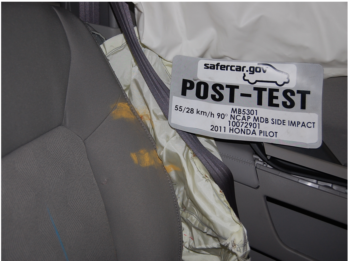
Post-Test Driver Dummy Close-up Torso Contact with Vehicle View
