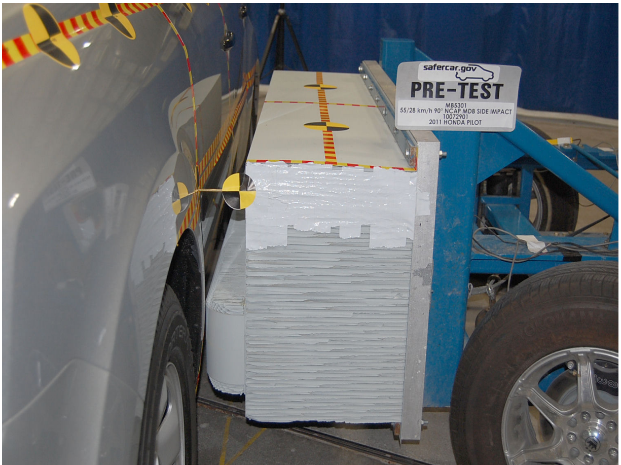
Pre-Test Left Side View of MDB Positioned Against Side of Target Vehicle at Ideal Impact Point
