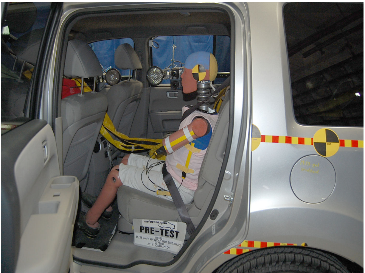
Pre-Test Left Side View of Passenger Dummy Showing Belt, Chalking, and Contact Switches (Door Open)
