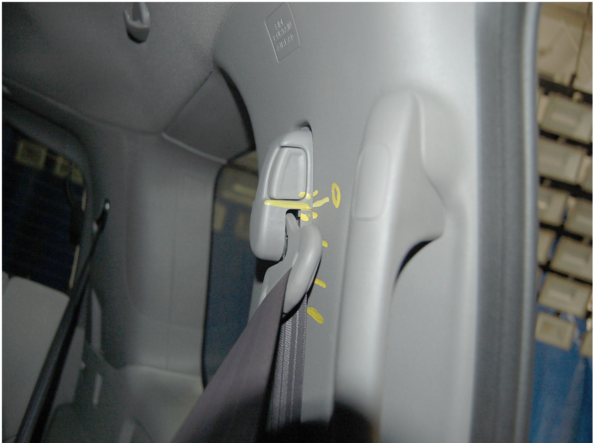
Pre-Test View of Belt Anchorage for Rear Passenger Dummy to Show Position
