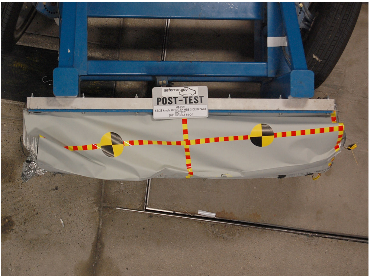
Post-Test Top View of MDB Impactor Face
