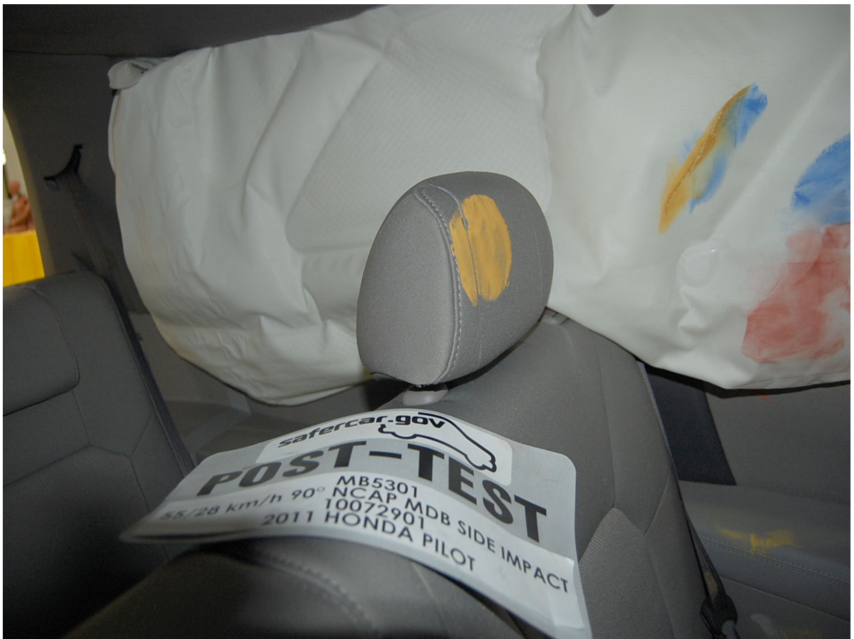
Post-Test Rear Passenger Dummy Close-up Head Contact with Vehicle View
