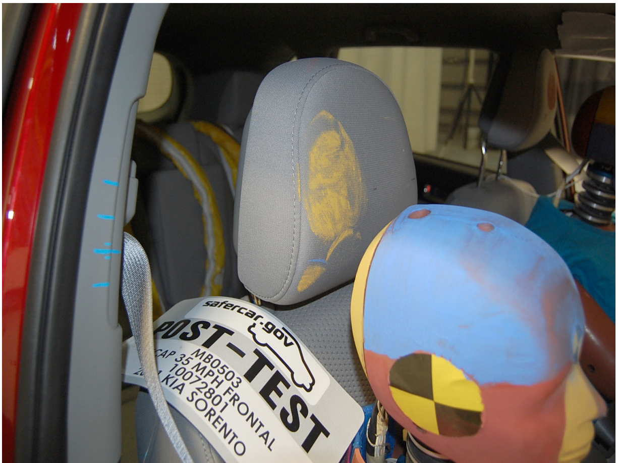
Post-Test Passenger Dummy Contact with Headrest
