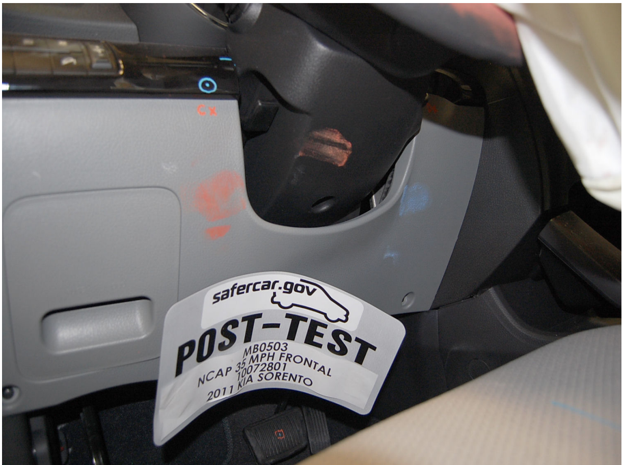
Post-Test Driver Dummy Contact with Knee Bolster
