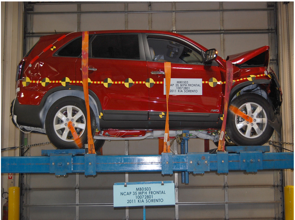
Vehicle at 0 Degrees on Static Rollover Device
