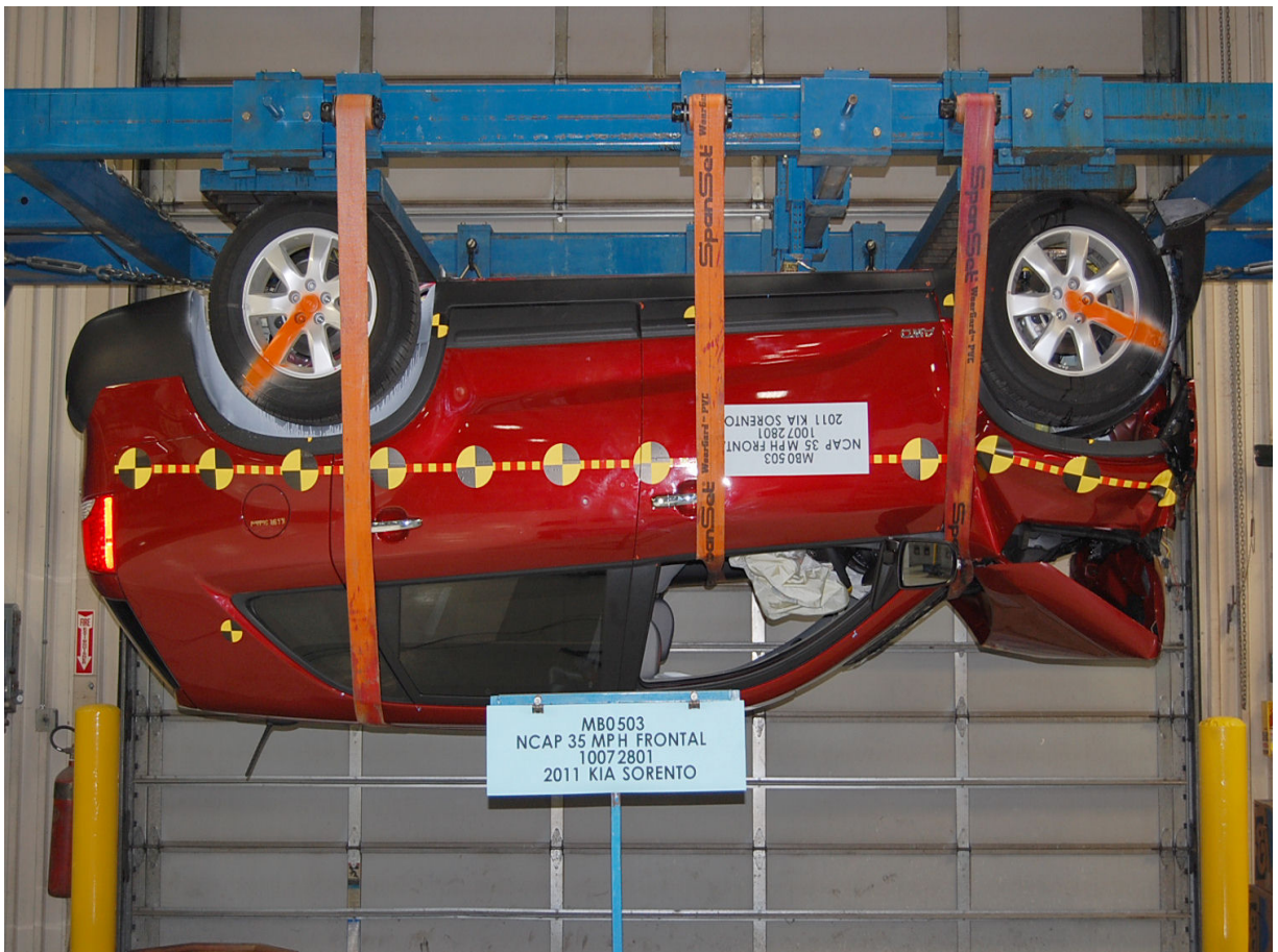
Vehicle at 180 Degrees on Static Rollover Device
