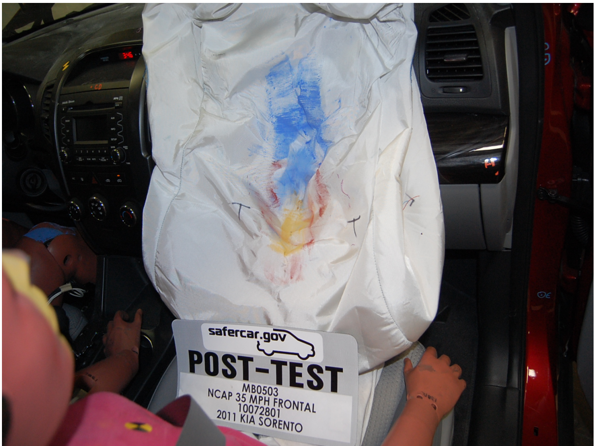
Post-Test Passenger Dummy Contact with Airbag
