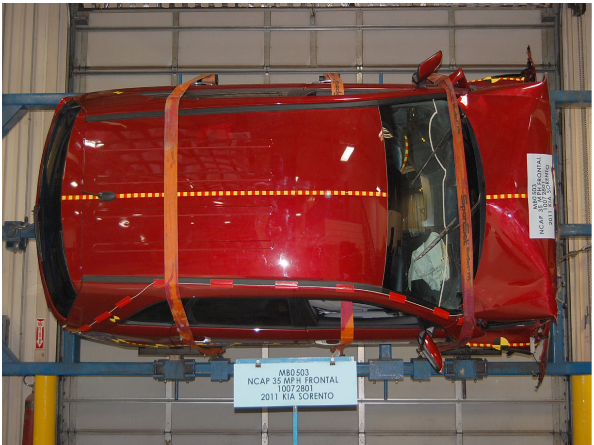
Vehicle at 270 Degrees on Static Rollover Device
