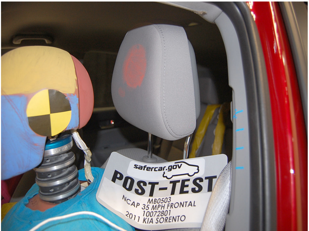
Post-Test Driver Dummy Contact with Headrest
