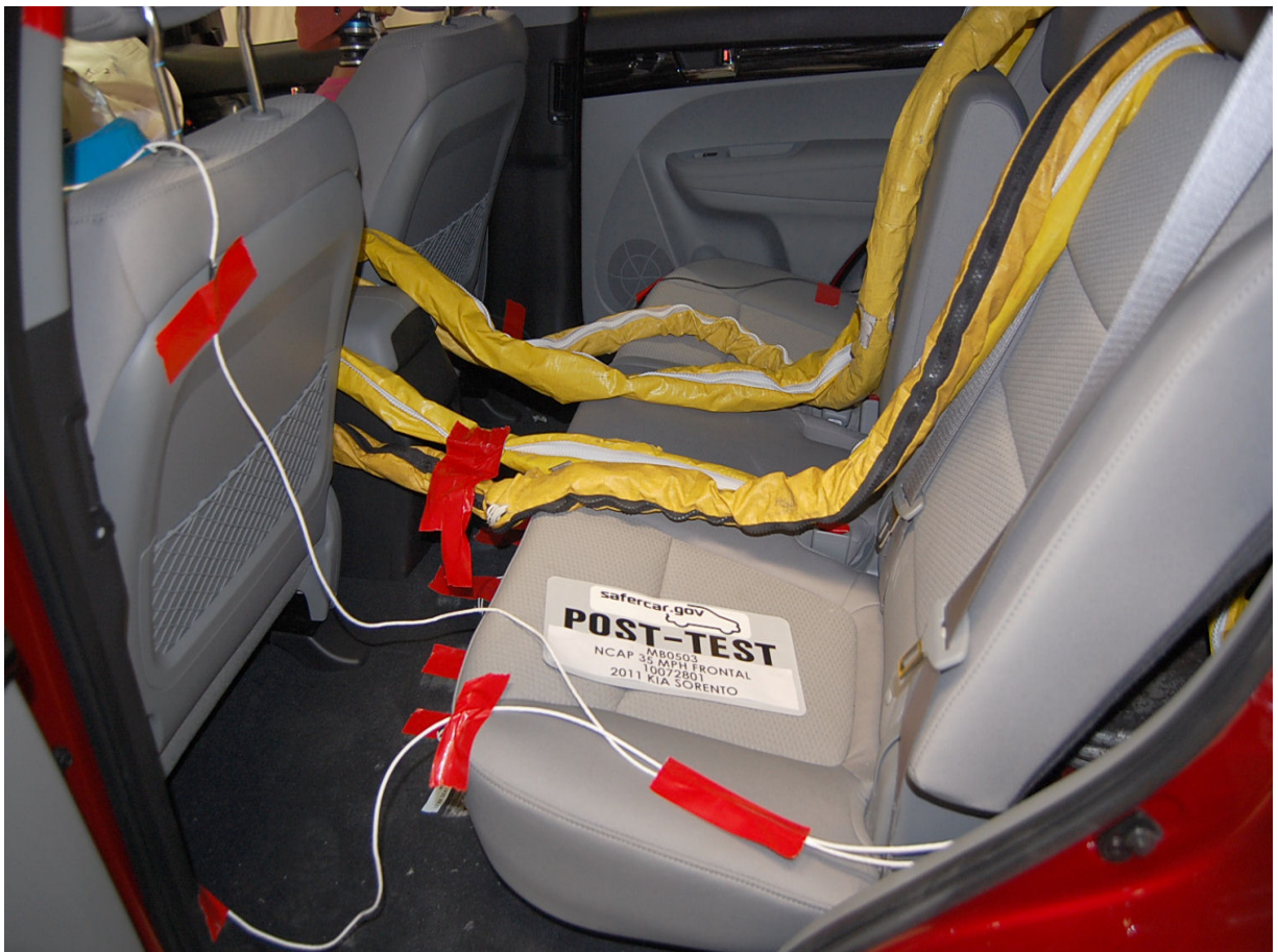
Post-Test Dummy Cable Routing
