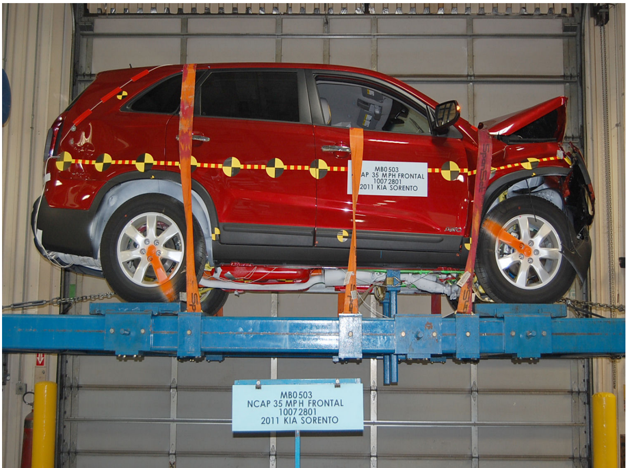
Vehicle at 360 Degrees on Static Rollover Device
