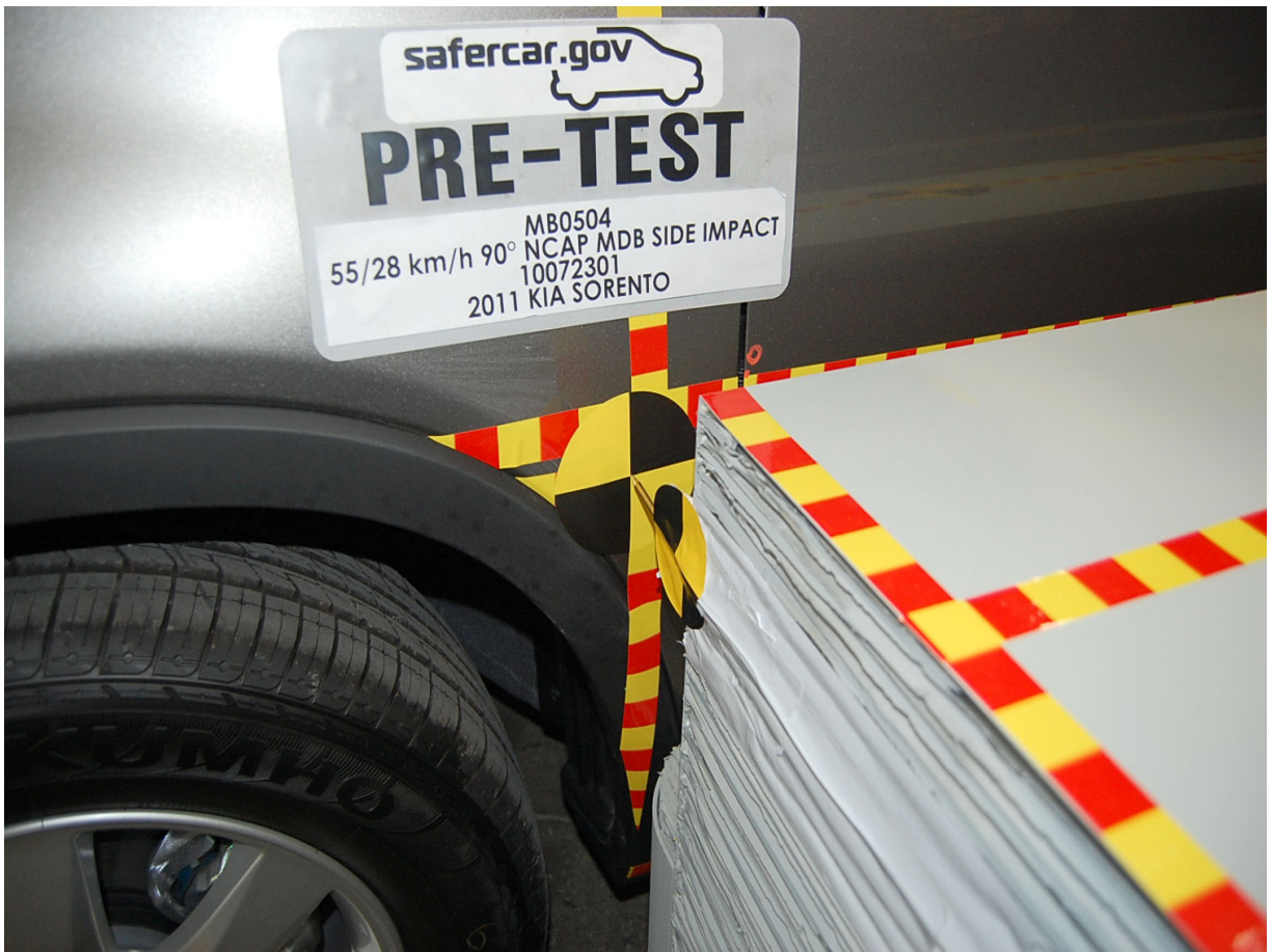
Pre-Test Close-Up View of Impact Point Target
