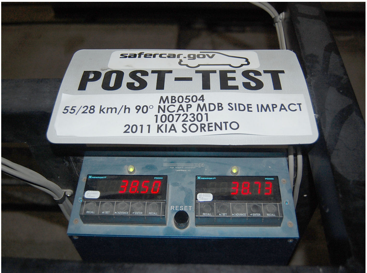
Post-Test Primary and Redundant Speed Trap Read-Out
