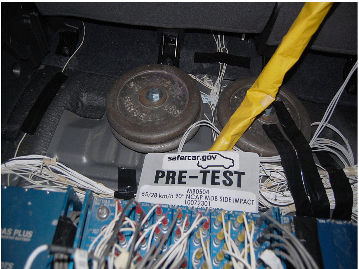
Pre-Test Ballast View
