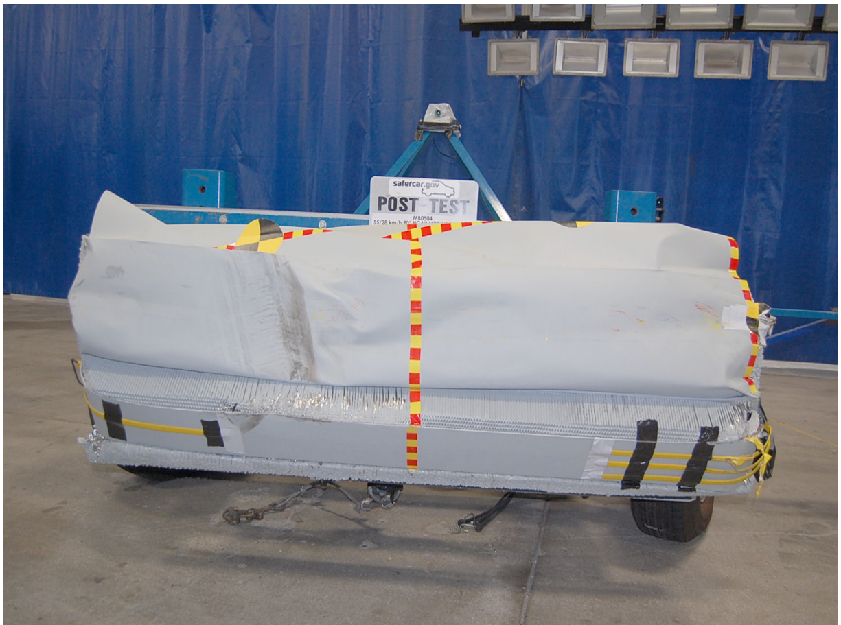
Post-Test Front View of MDB Impactor Face
