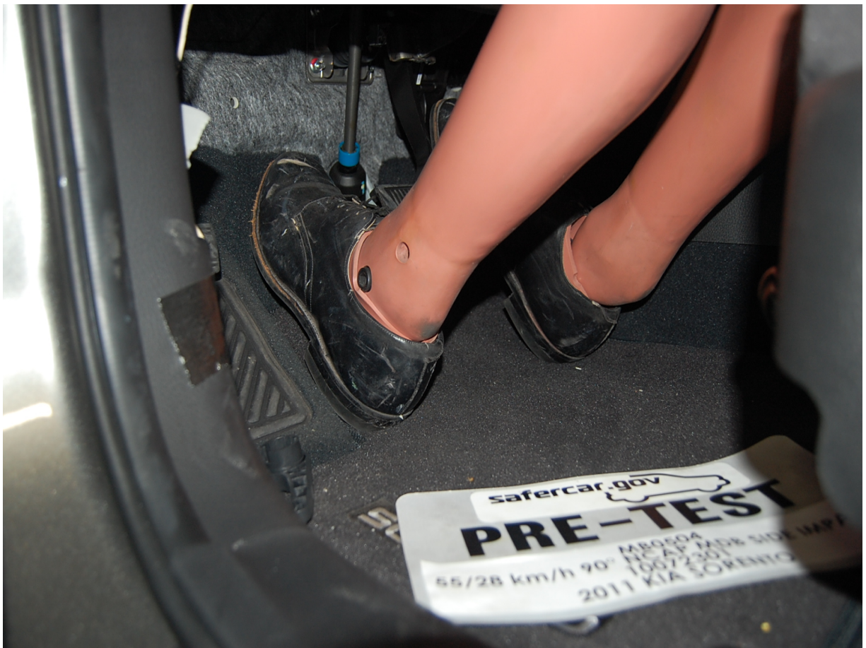
Pre-Test Placement of Driver Dummy's Feet
