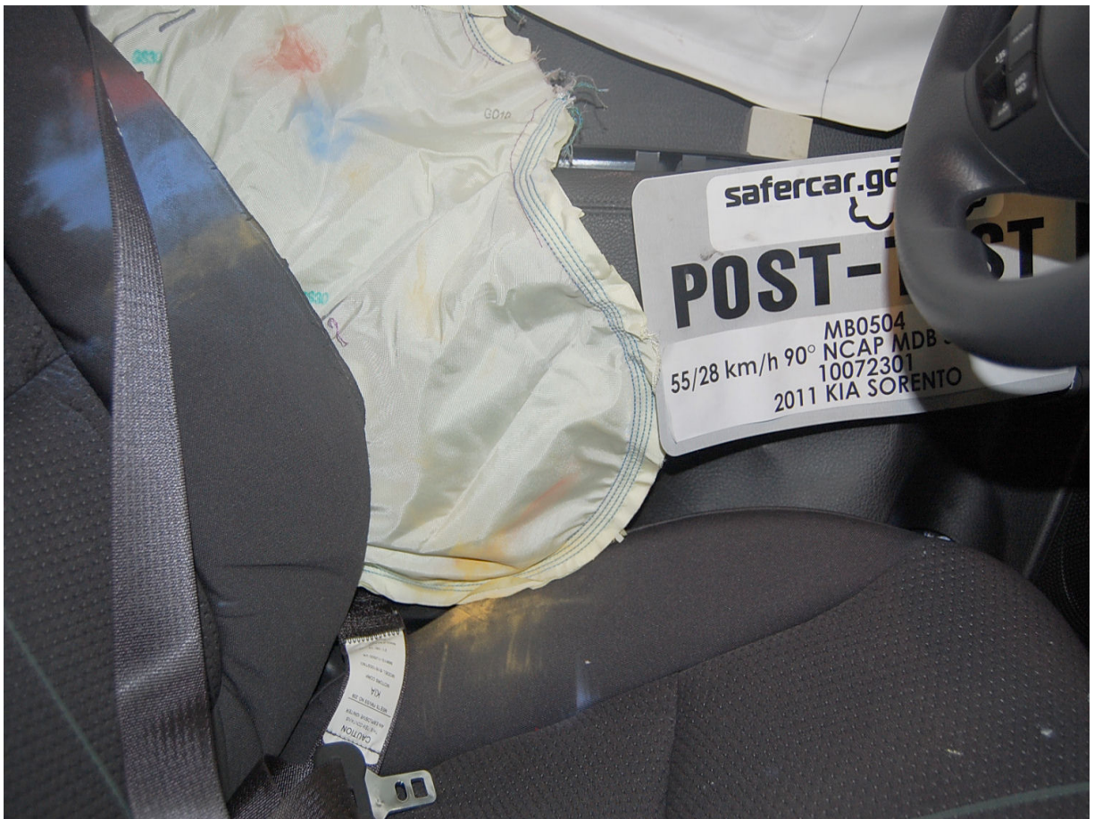
Post-Test Driver Dummy Close-up Pelvis Contact View
