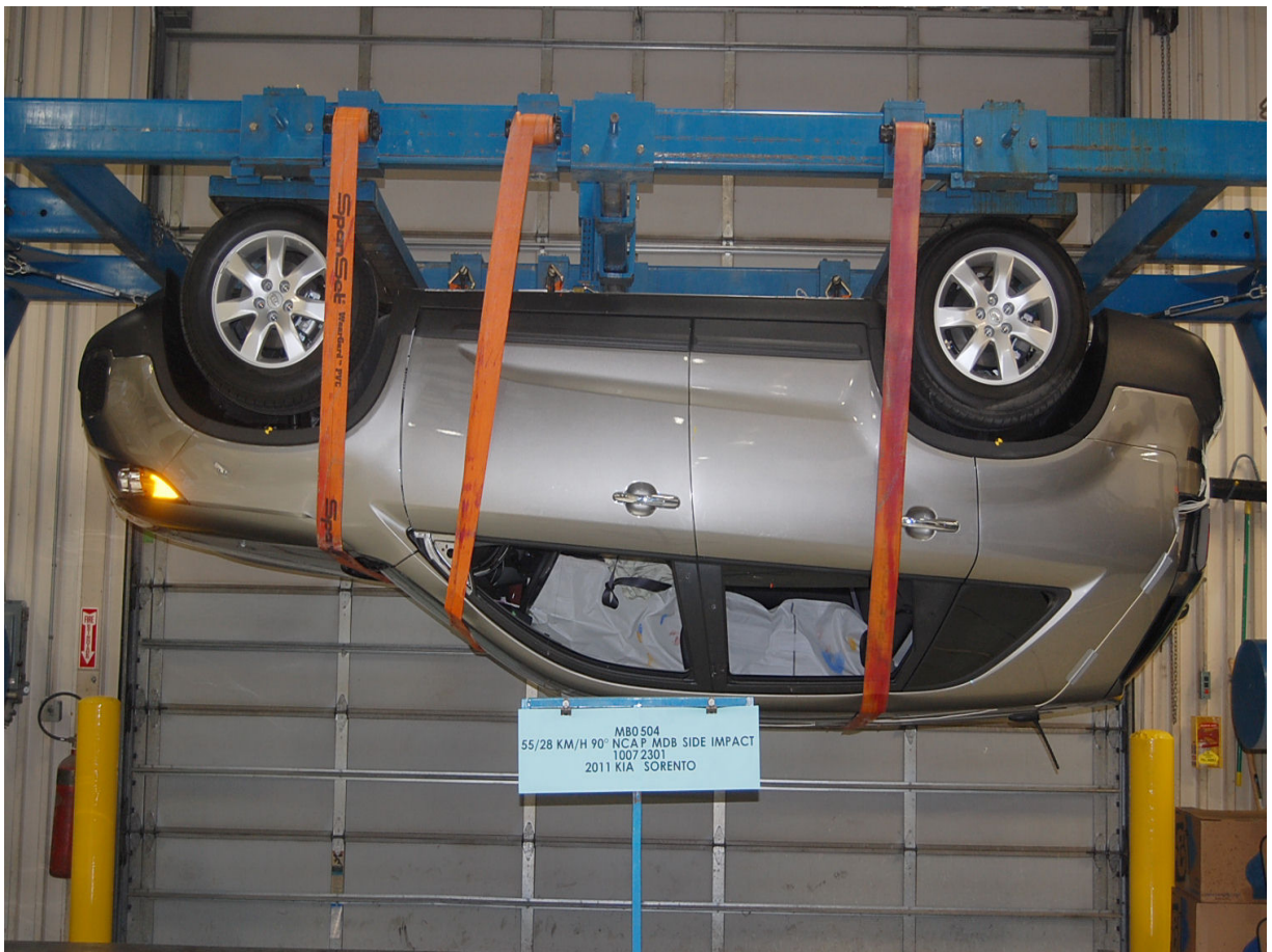
FMVSS No. 301/305 Rollover 180 Degrees
