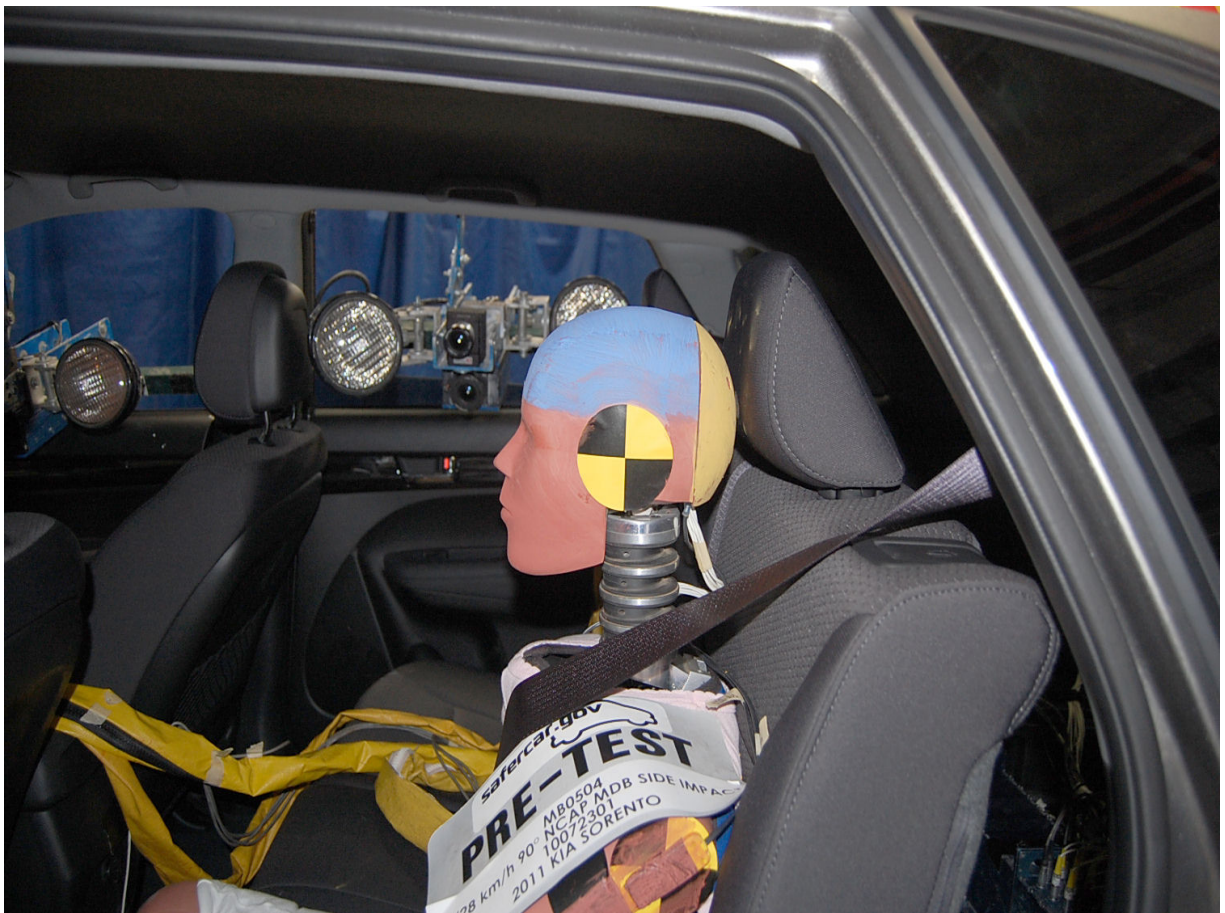
Pre-Test Close-Up Left Side View of Rear Passenger Seat Back Showing Test Position
