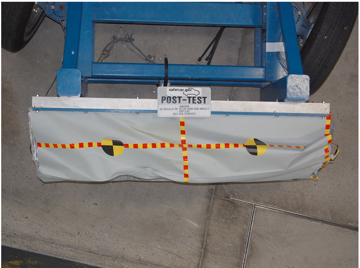
Post-Test Top View of MDB Impactor Face
