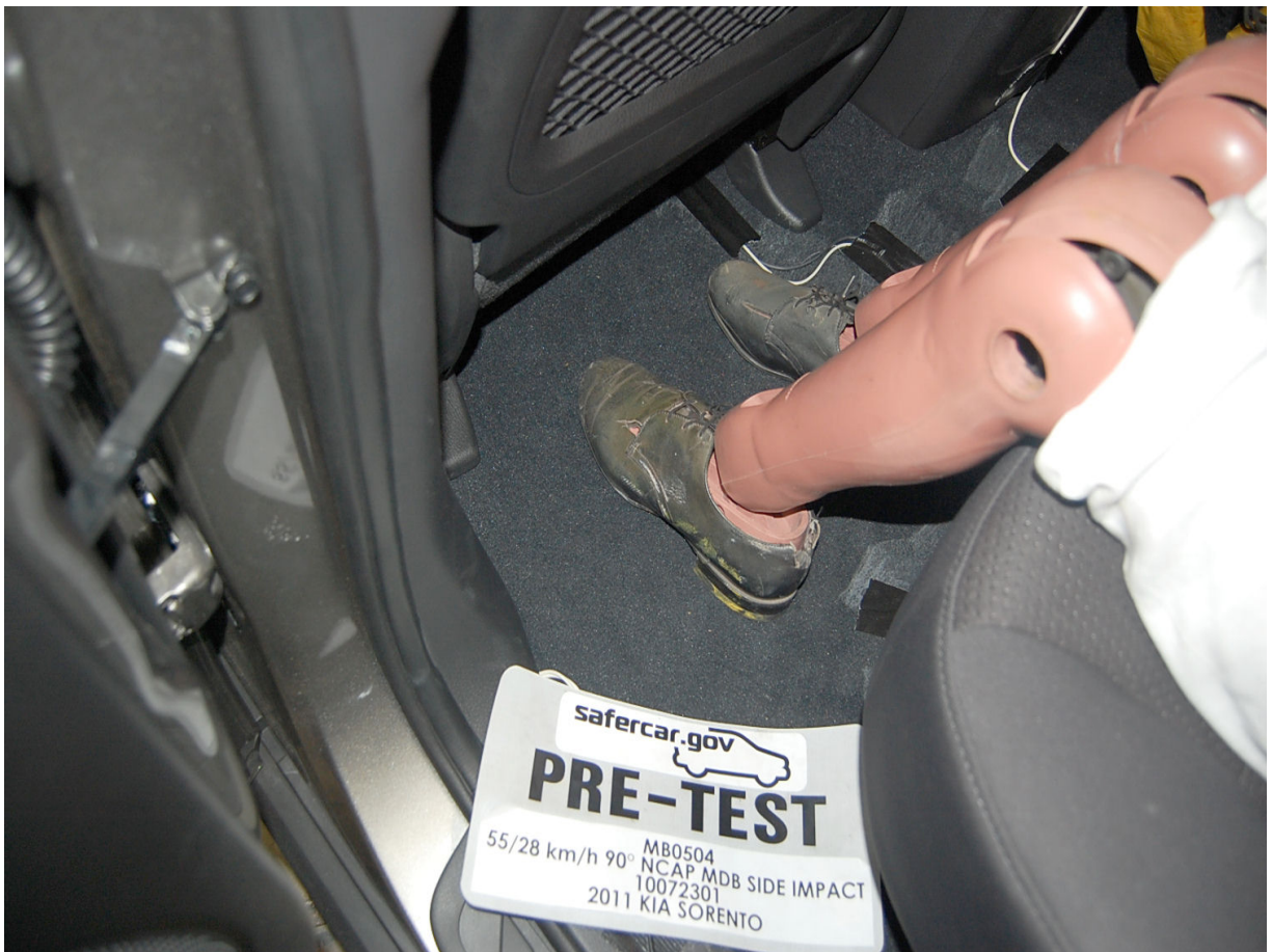
Pre-Test Placement of Rear Passenger Dummy's Feet
