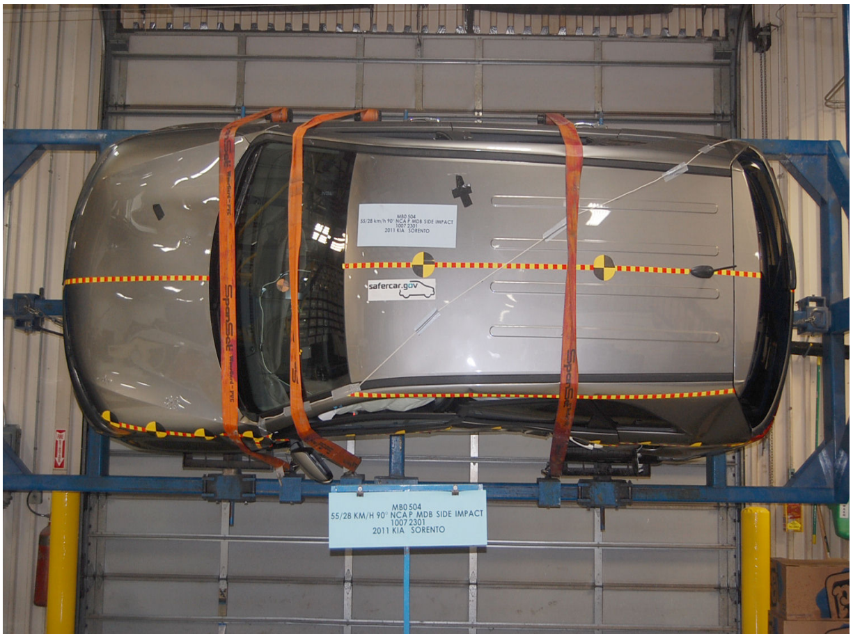
FMVSS No. 301/305 Rollover 90 Degrees
