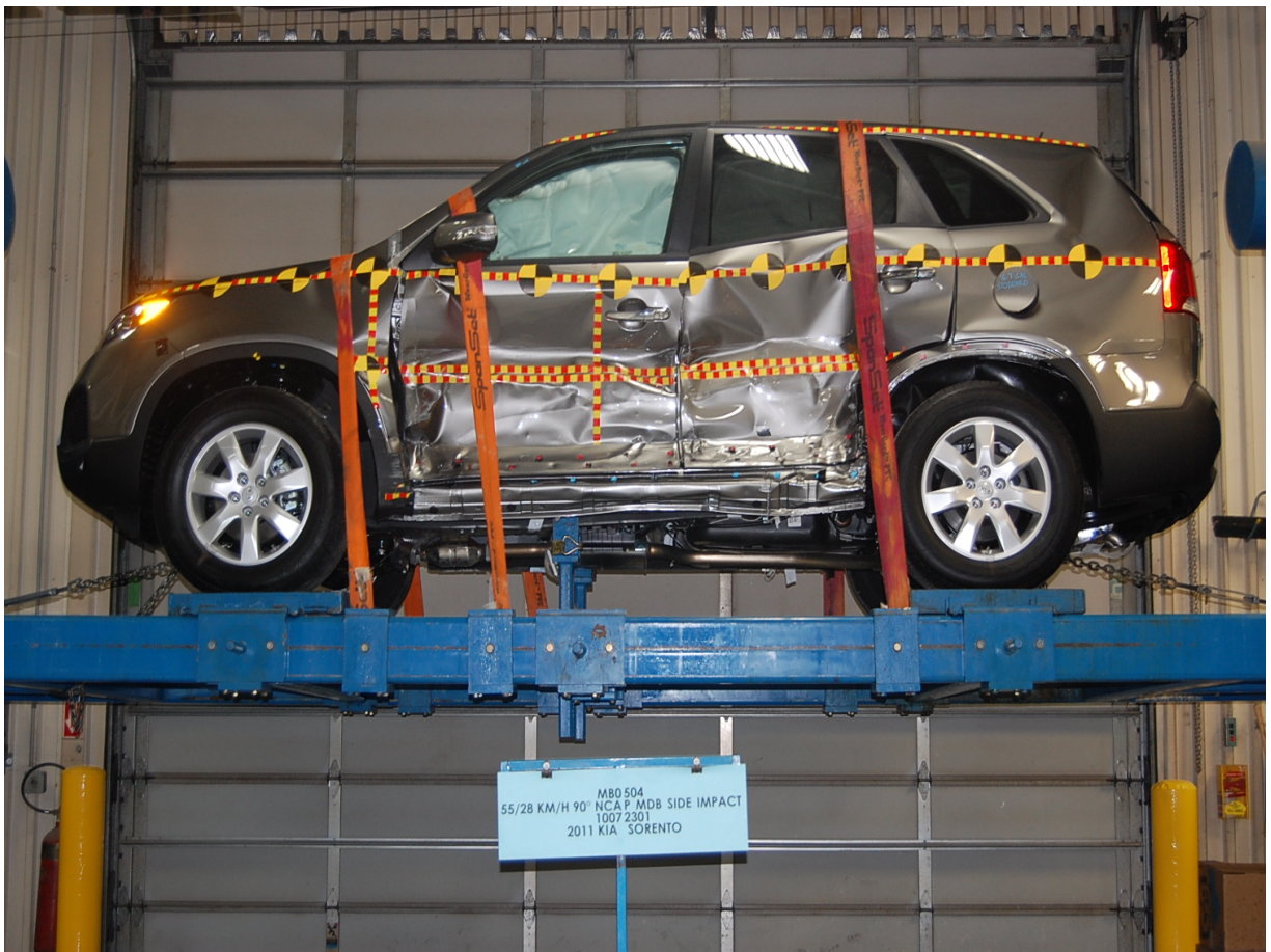
FMVSS No. 301/305 Rollover 0 Degrees
