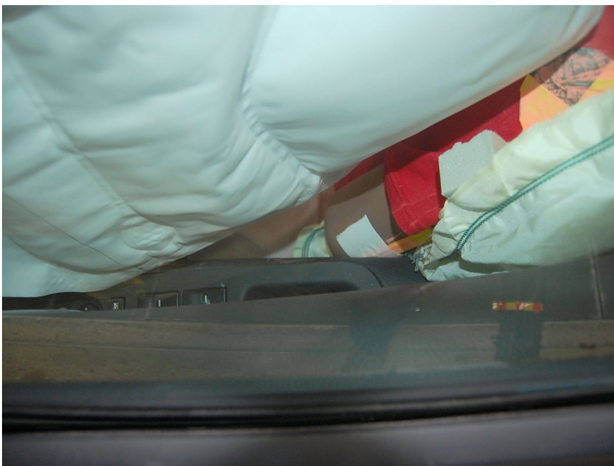
Post-Test Driver Dummy and Door Clearance View
