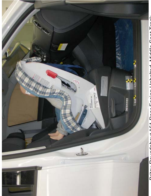
Britax Roundabout 161 Rear Facing Unbelated, Middle Seat Track
