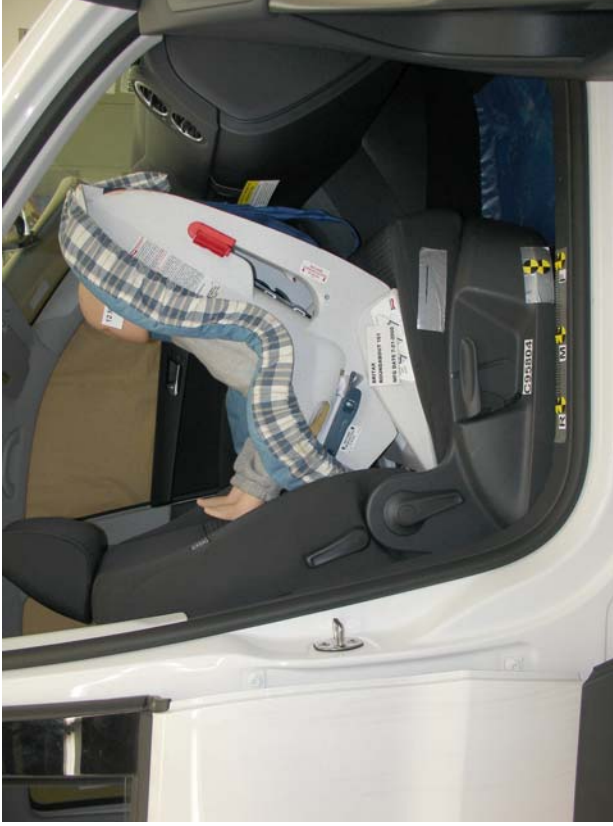
Britax Roundabout 161 Rear Facing Unbelated, Forward Seat Track
