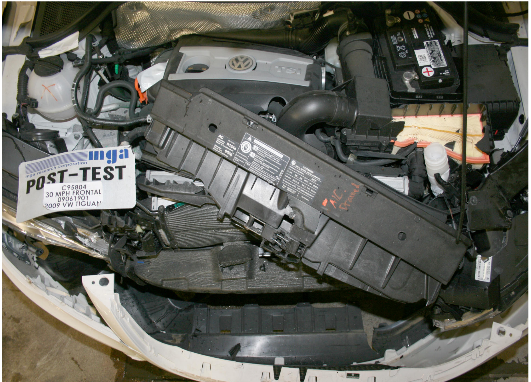
Post-Test Engine Compartment View
