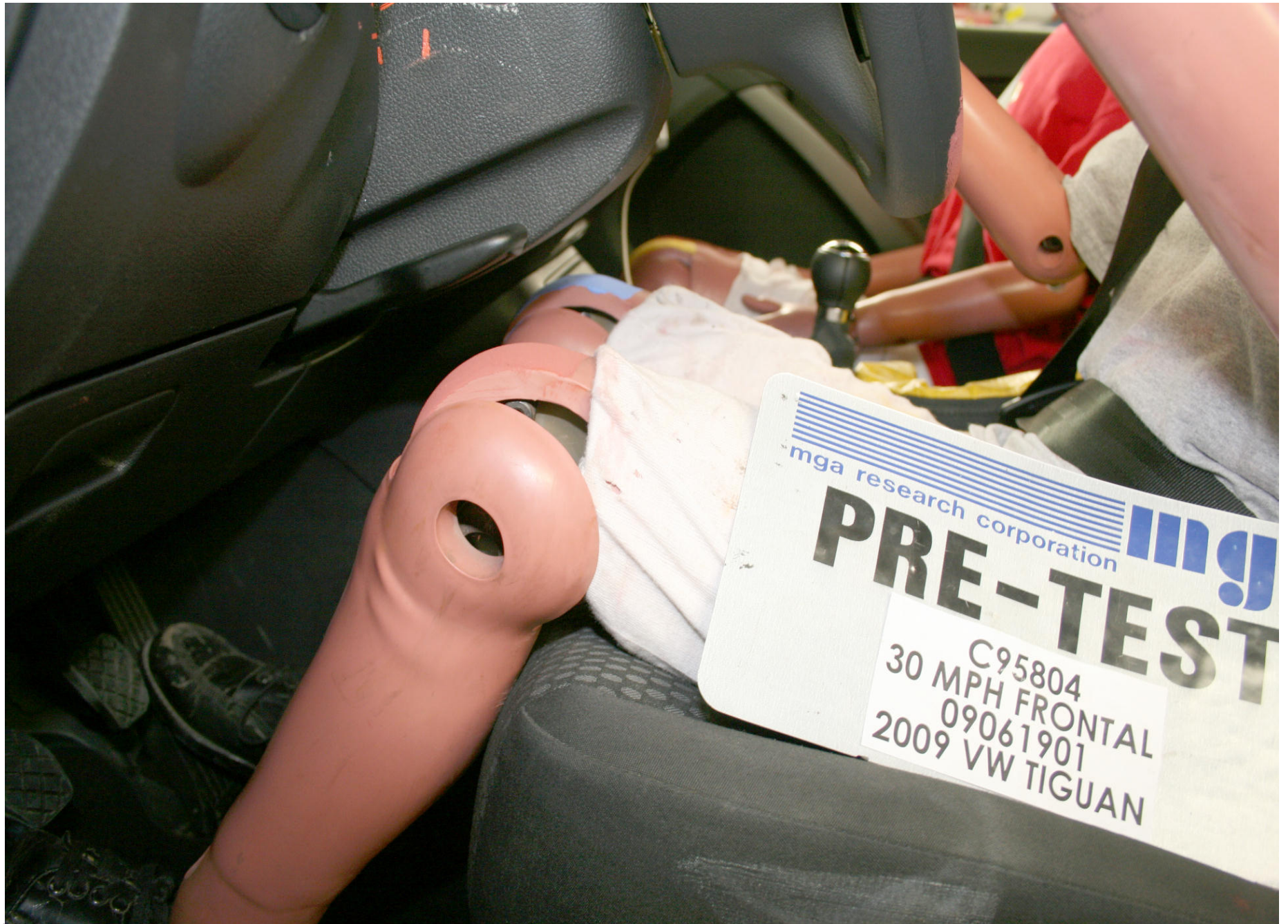
Pre-Test Driver Side Knee Bolster View
