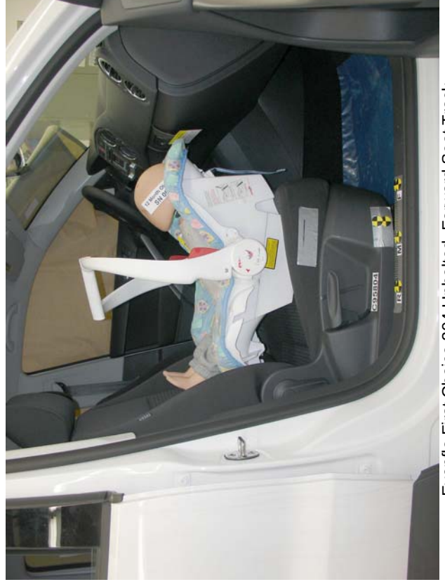
Evenflo First Choice 204 Unbelted, Forward Seat Track
