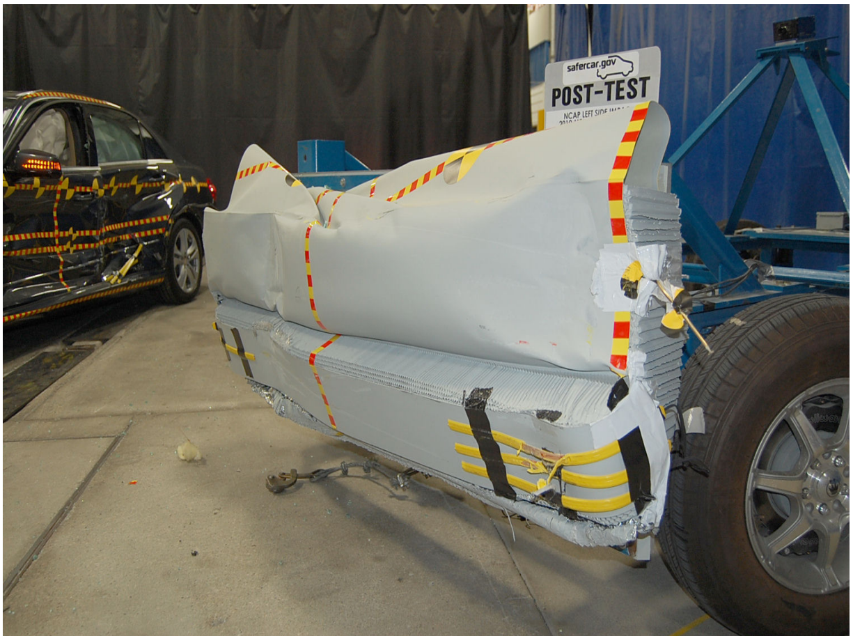
Post-Test Right Side View of Deformable Barrier
