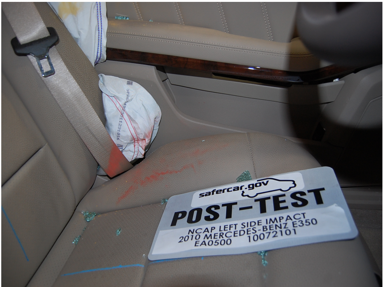
Post-Test Driver Dummy Lower Torso Contact
