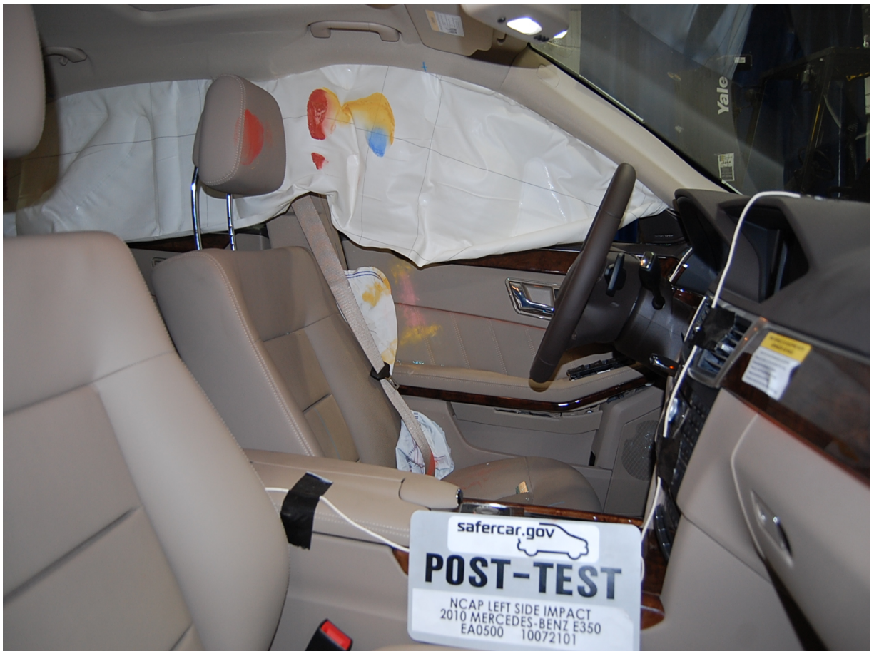
Post-Test Driver Dummy Contact
