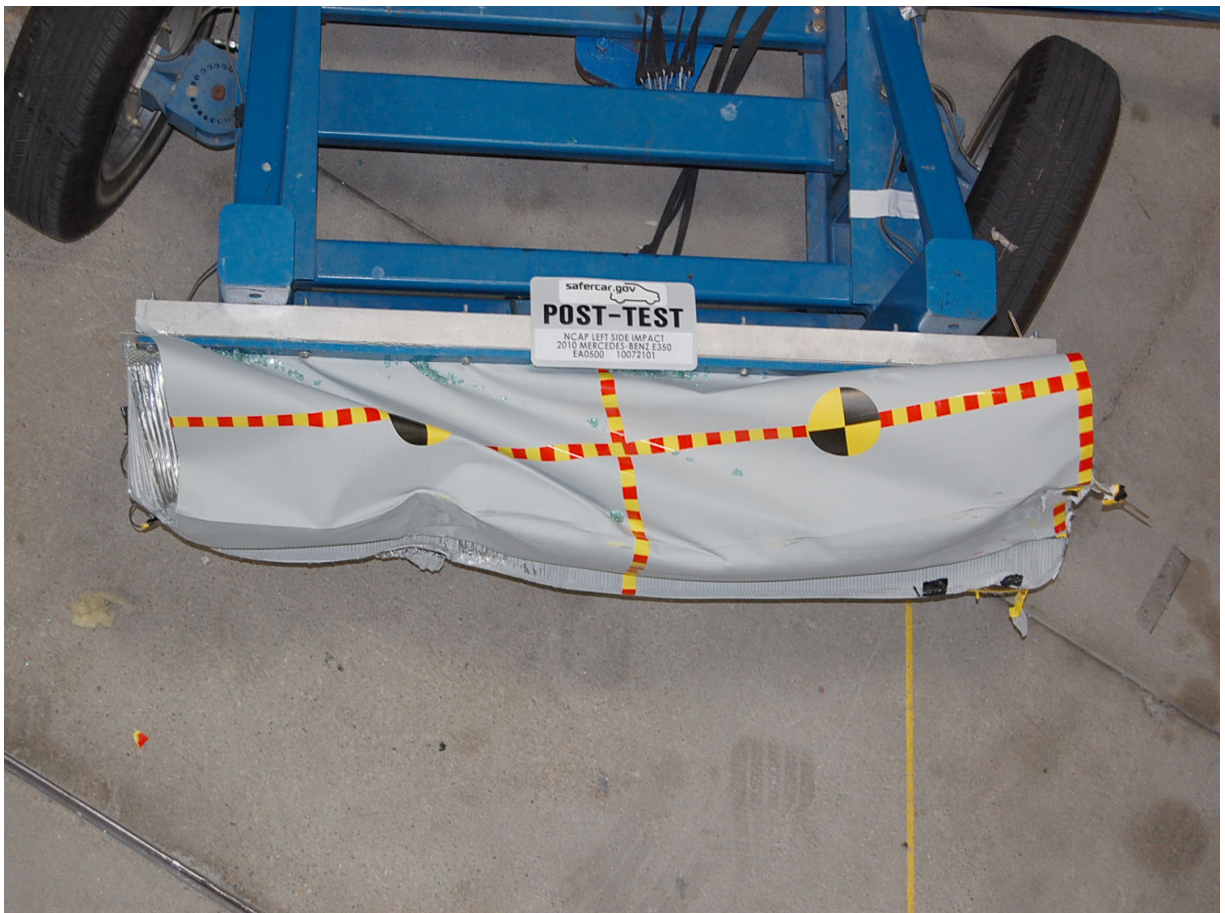
Post-Test Top View of Deformable Barrier
