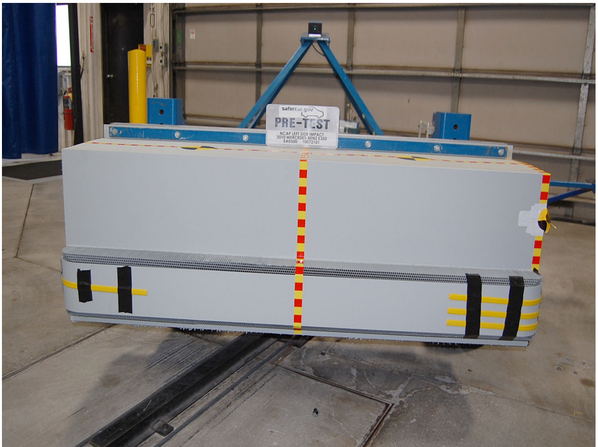
Pre-Test Front View of Deformable Barrier
