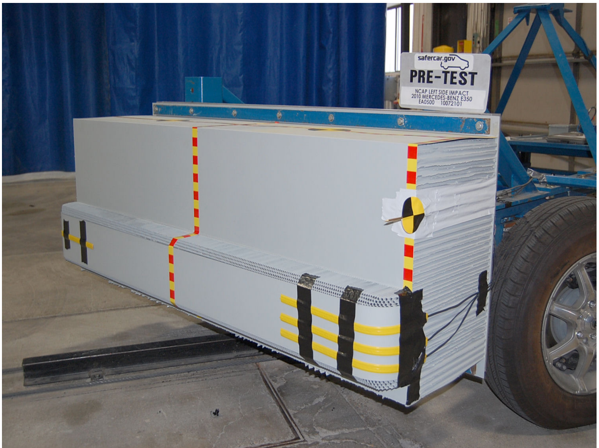
Pre-Test Right Side View of Deformable Barrier
