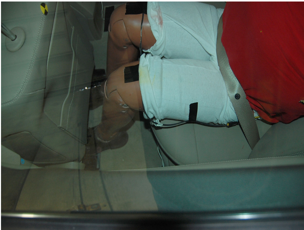
Pre-Test Passenger Dummy Clearance From Door
