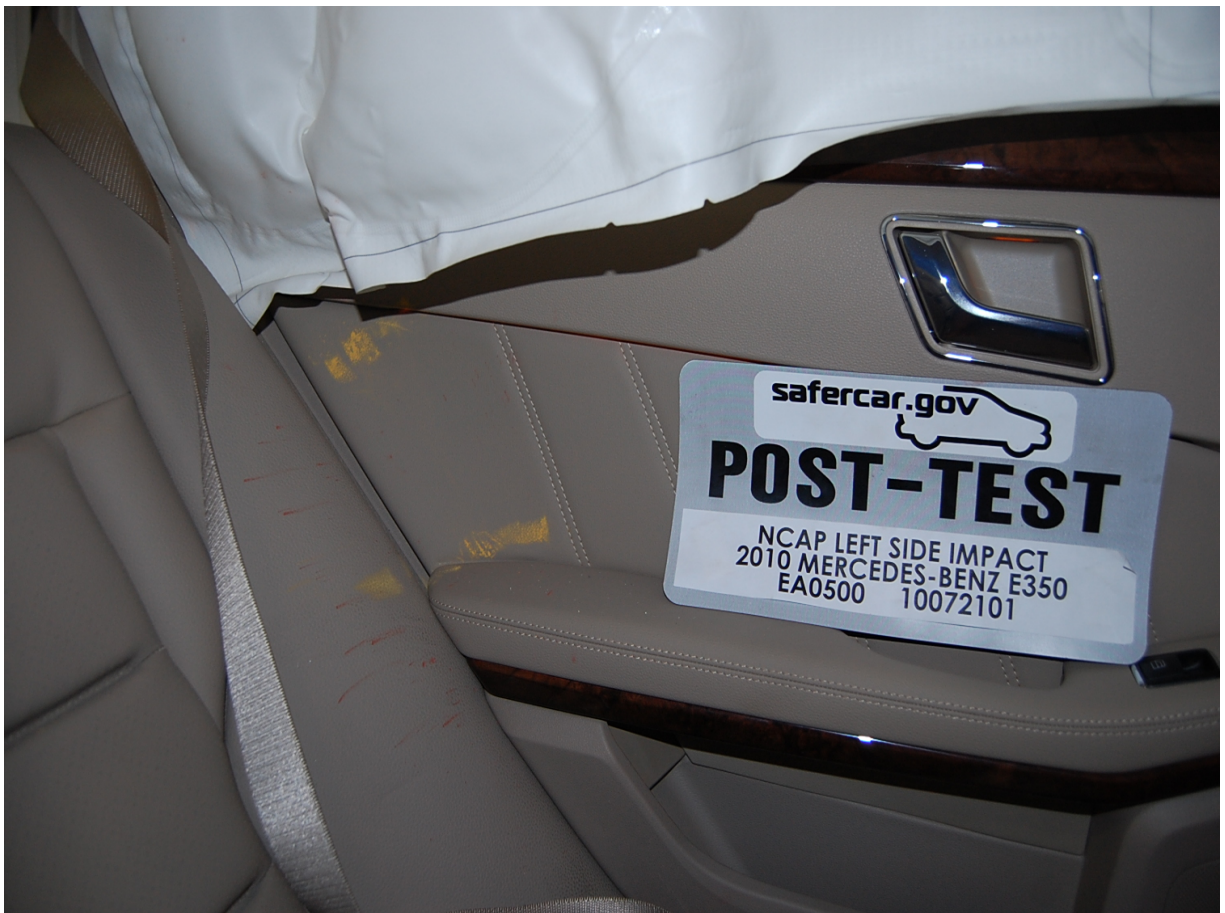
Post-Test Passenger Dummy Upper Torso Contact
