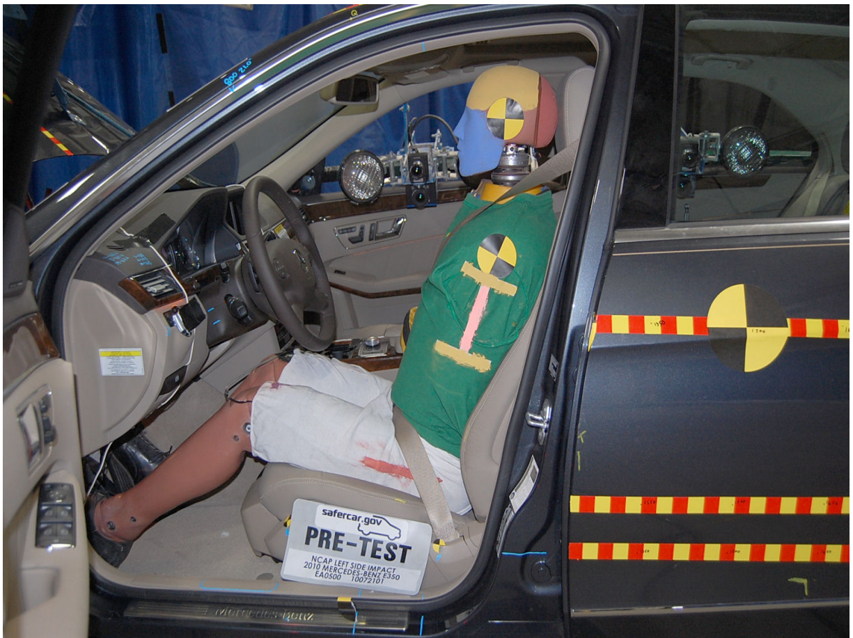
Pre-Test Driver Dummy (Door Open)
