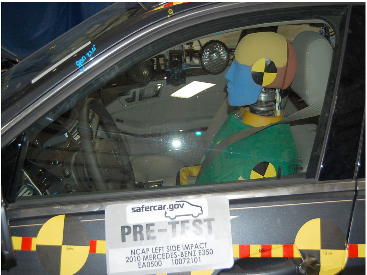
Pre-Test Driver Dummy (Through Window)
