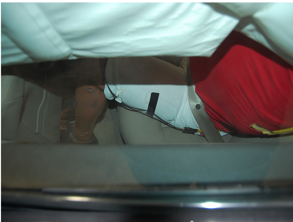
Post-Test Passenger Dummy Clearance From Door
