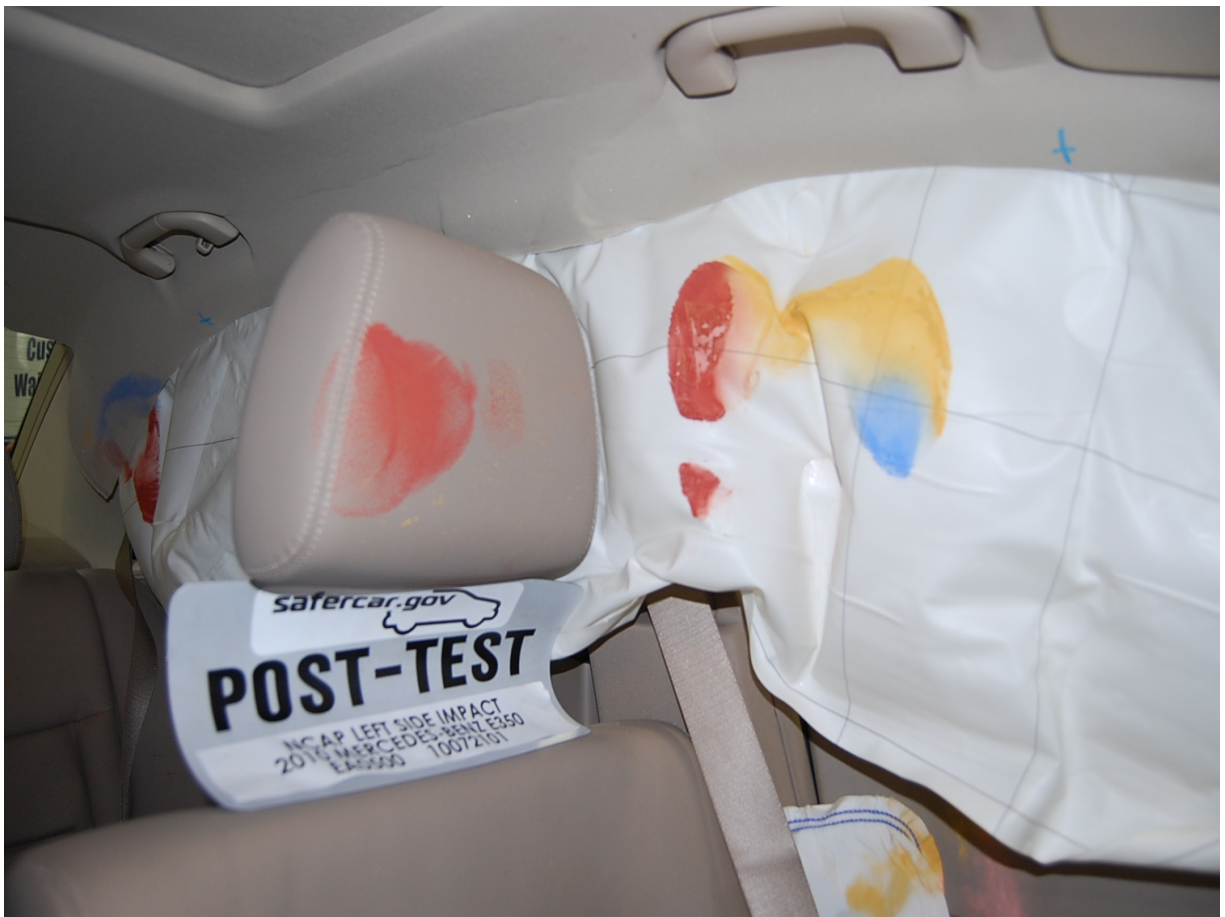
Post-Test Driver Dummy Head Contact View
