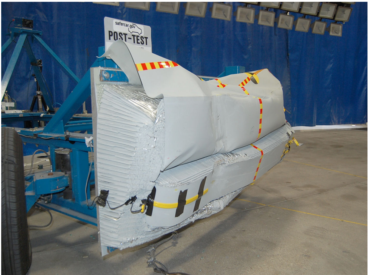
Post-Test Left Side View of Deformable Barrier
