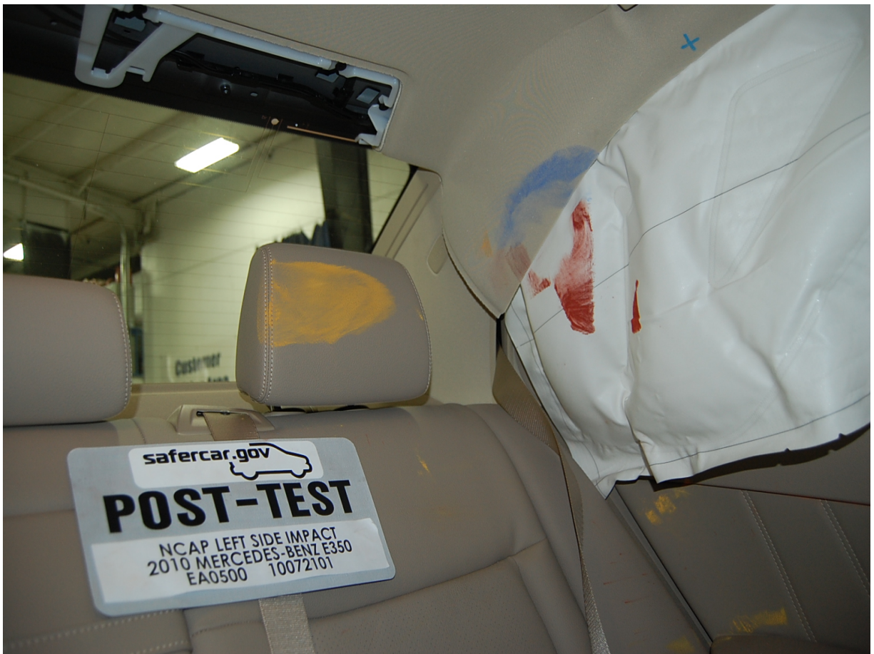
Post-Test Passenger Dummy Head Contact View
