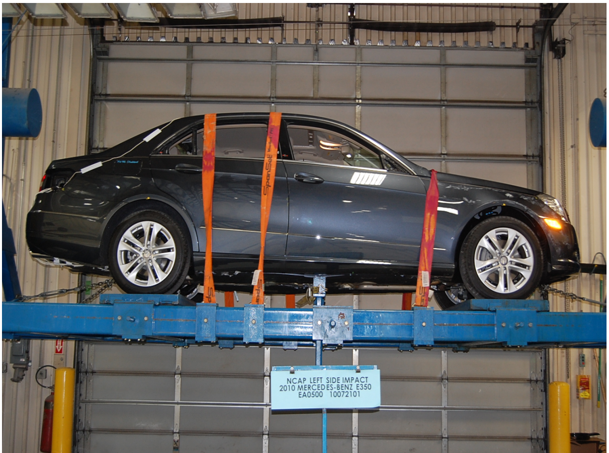
Vehicle on Rollover Device (360 Degrees)
