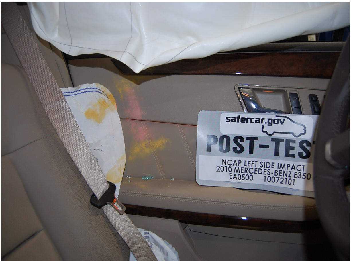
Post-Test Driver Dummy Upper Torso Contact
