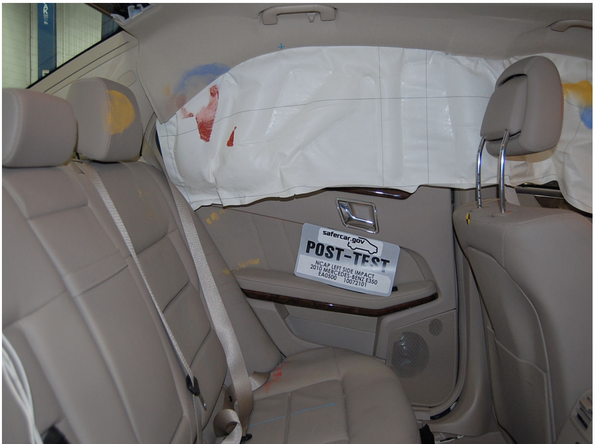
Post-Test Passenger Dummy Contact
