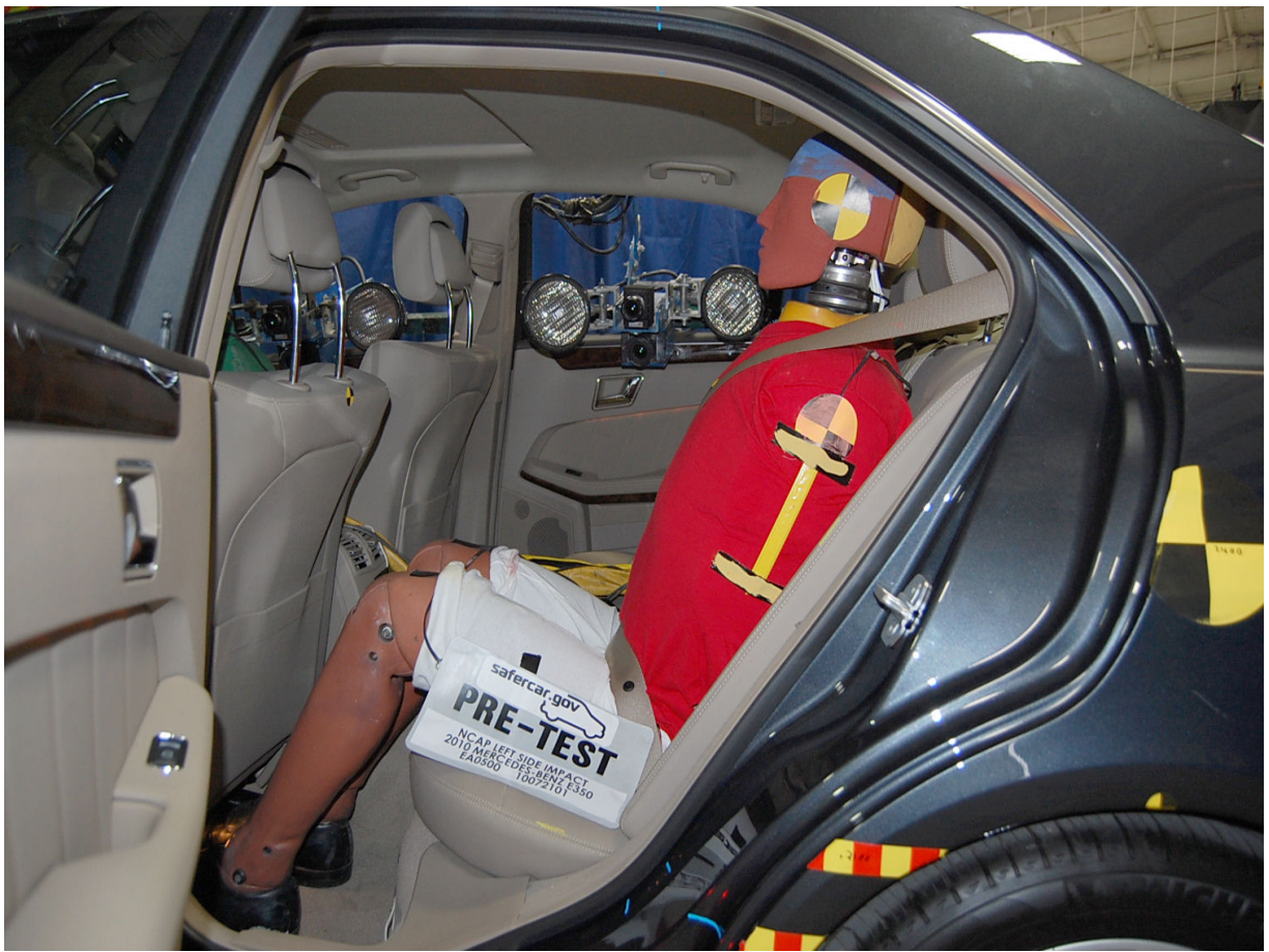
Pre-Test Passenger Dummy (Door Open)
