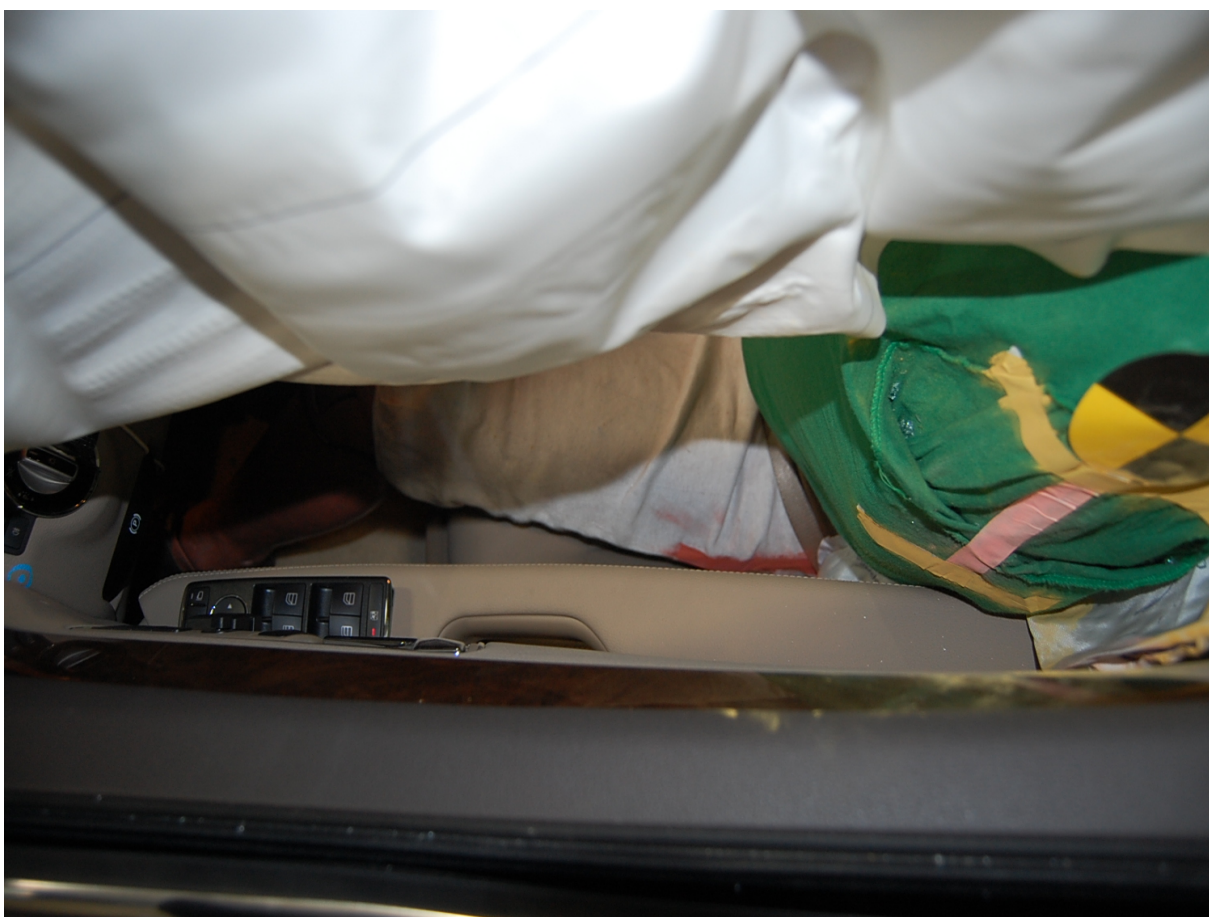
Post-Test Driver Dummy Clearance From Door
