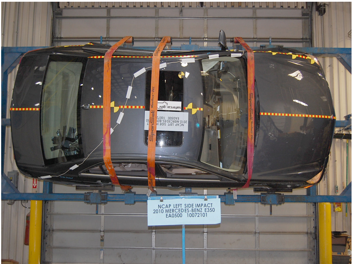
Vehicle on Rollover Device (90 Degrees)
