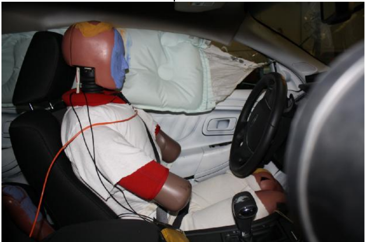
Figure A-44: Post-test Right Side View of Driver Dummy and Front Seat of Occupant Compartment
