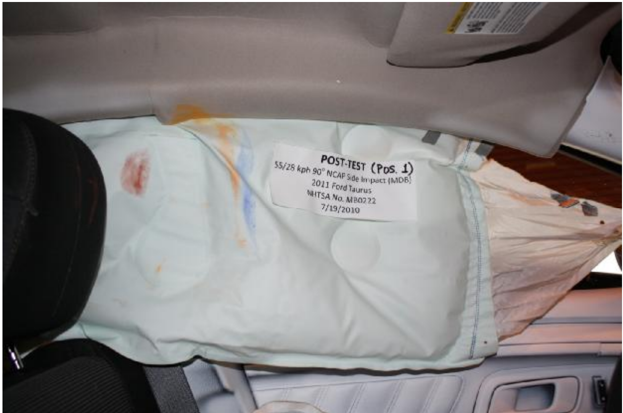
Figure A-48: Post-test Driver Dummy Close-Up Head Contact with Side Airbag View
