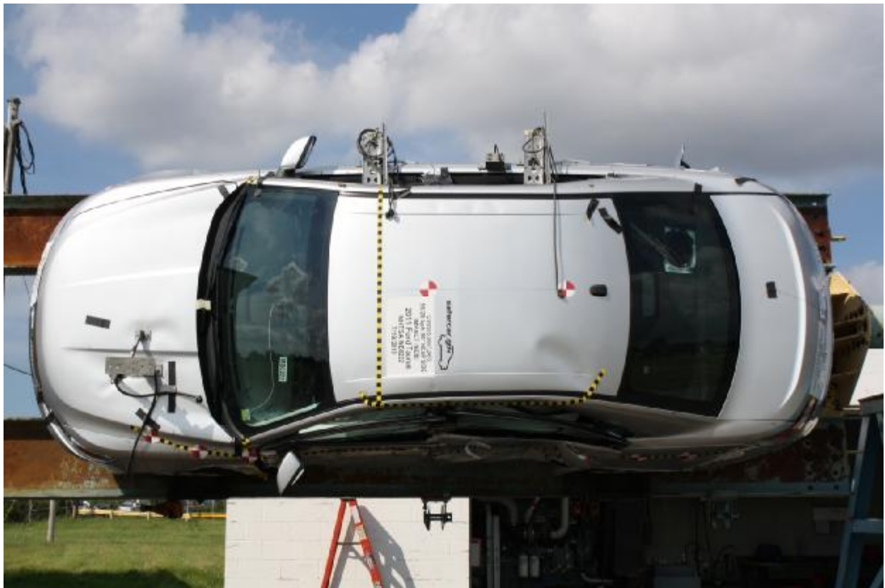
Figure A-94: FMVSS No. 301 Rollover 90°
