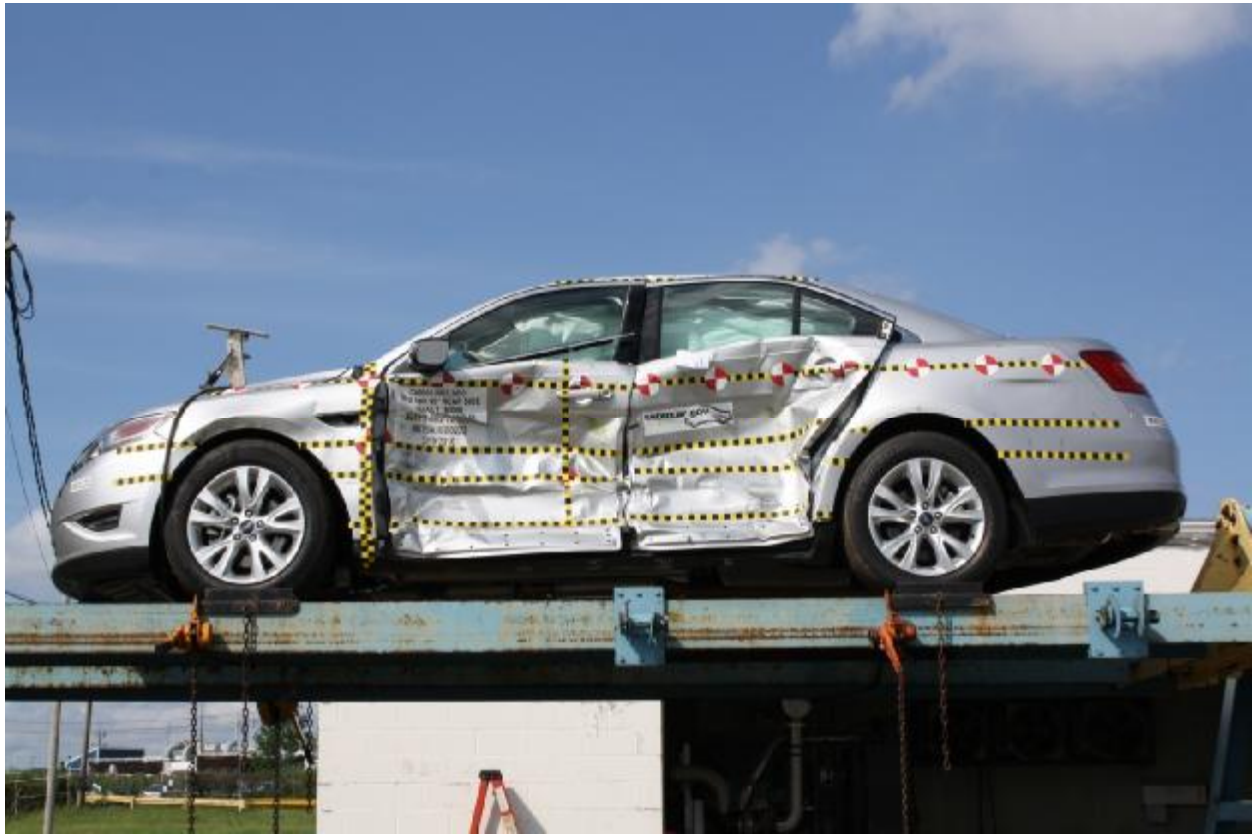
Figure A-93: FMVSS No. 301 Rollover 0°
