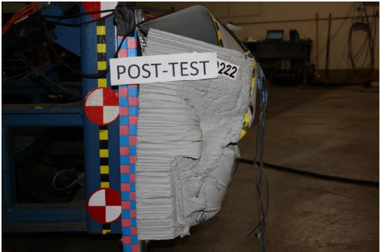
Figure A-88: Post-Test Right Side View of MDB Impactor Face
