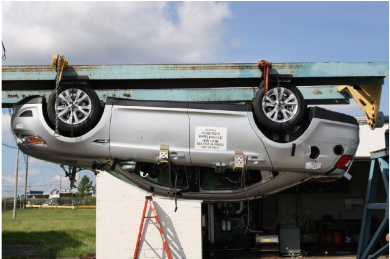
Figure A-95: FMVSS No. 301 Rollover 180°
