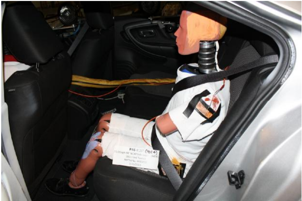
Figure A-53: Pre-test Left Side View of Passenger Dummy Showing Belt, Chalking, and Contact Switches
