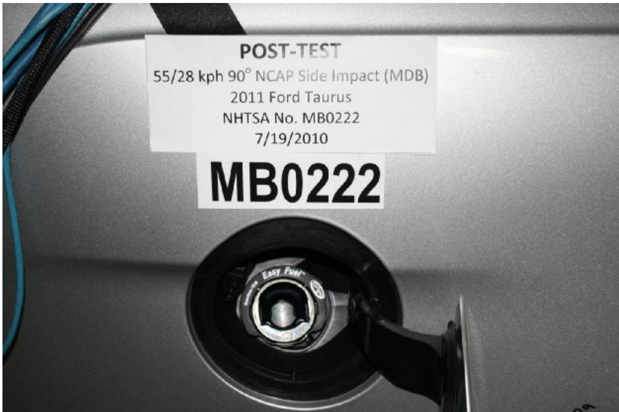
Figure A-80: Post-Test View of Fuel Filler Cap or Fuel Filler Neck
