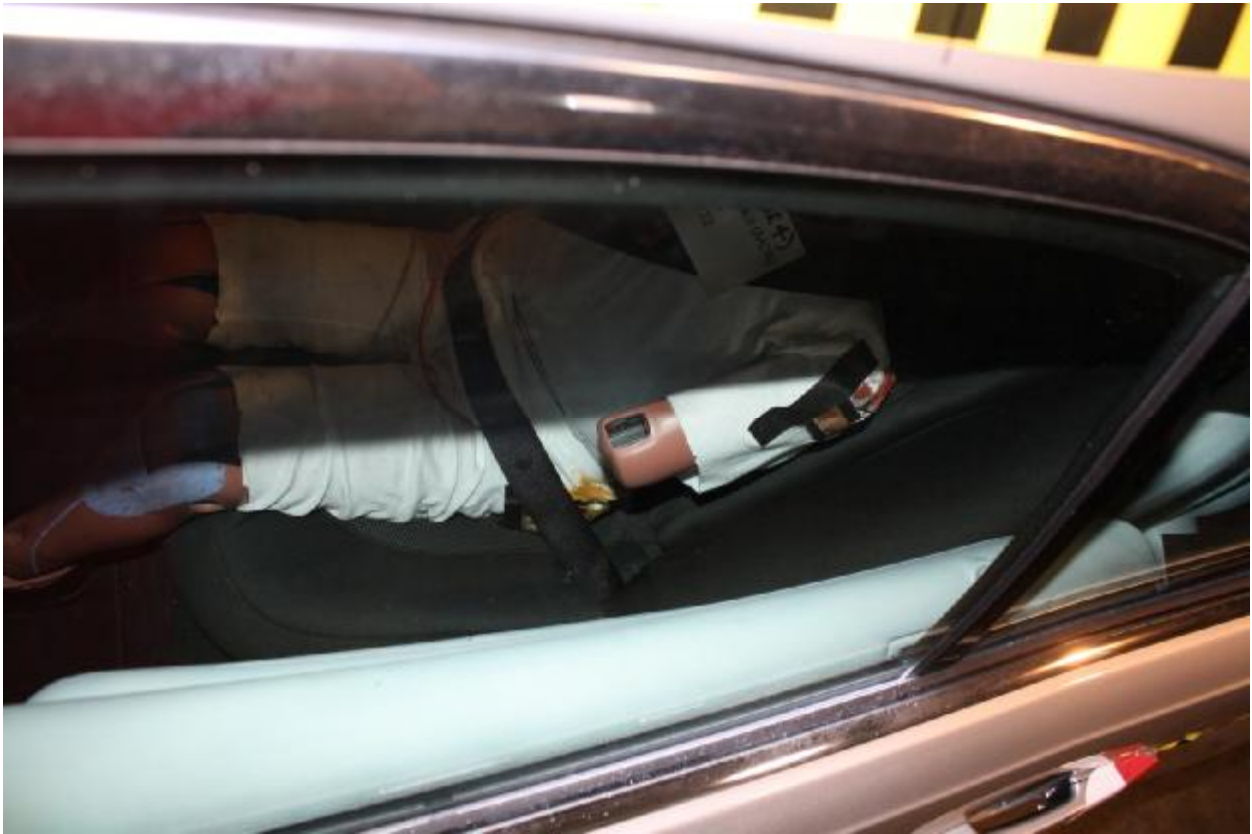
Figure A-67: Pre-Test Passenger Dummy and Door Clearance View
