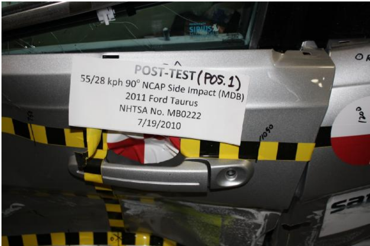
Figure A-22: Post-Test Left Front Door Lath Close-up
