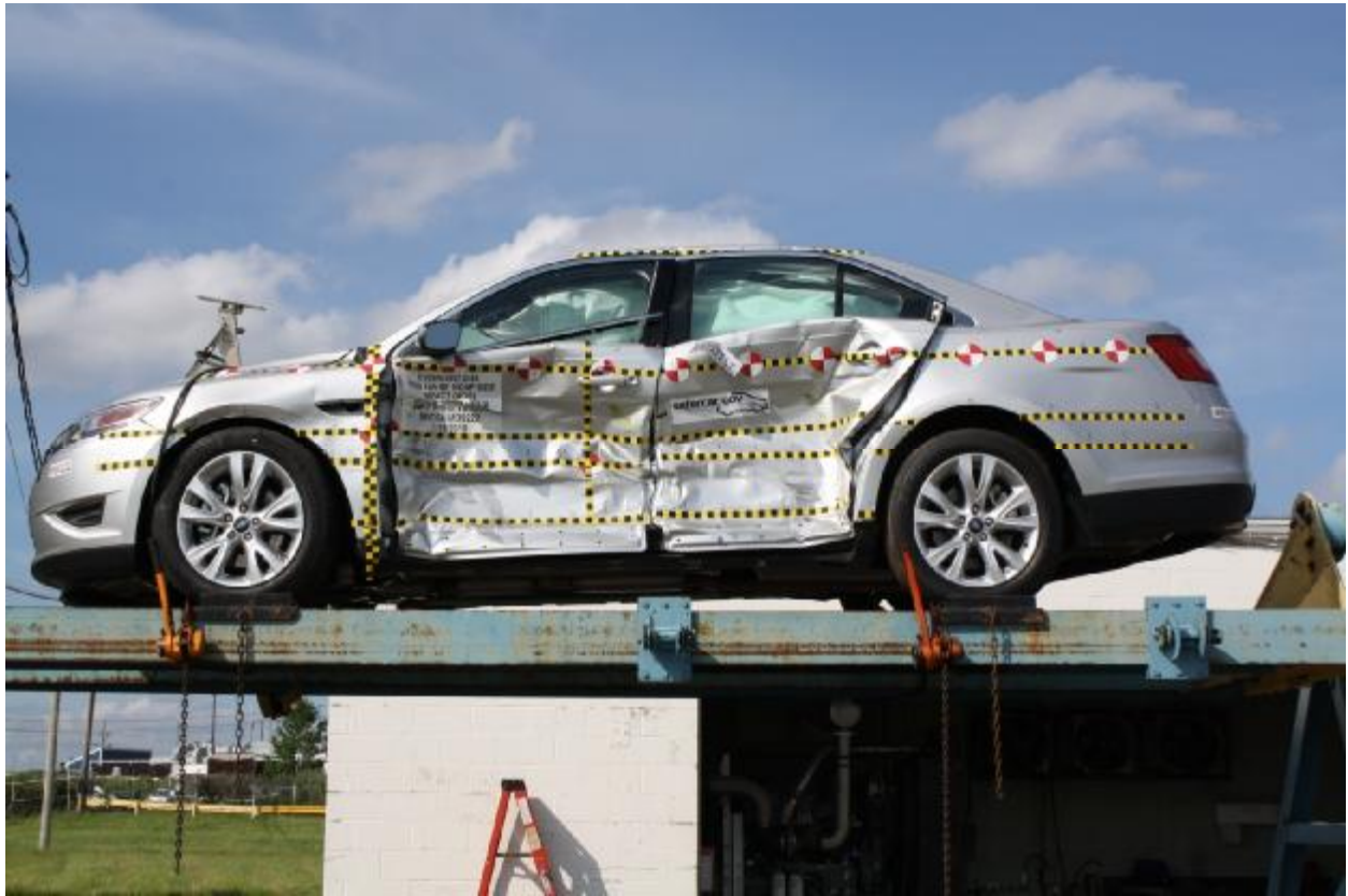
Figure A-97: FMVSS No. 301 Rollover 360°
