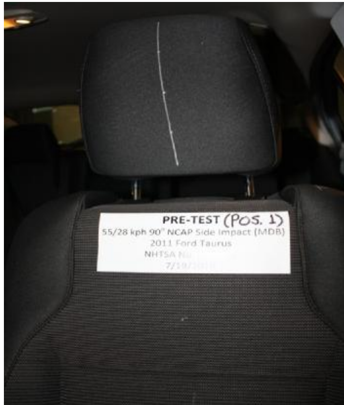
Figure A-30: Pre-Test Frontal View of Driver Seat Back Prior to Dummy Positioning
