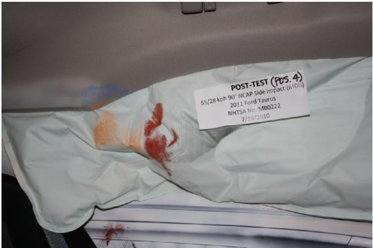
Figure A-74: Post-test Rear Passenger Dummy Close-Up Head Contact with Side Airbag View
