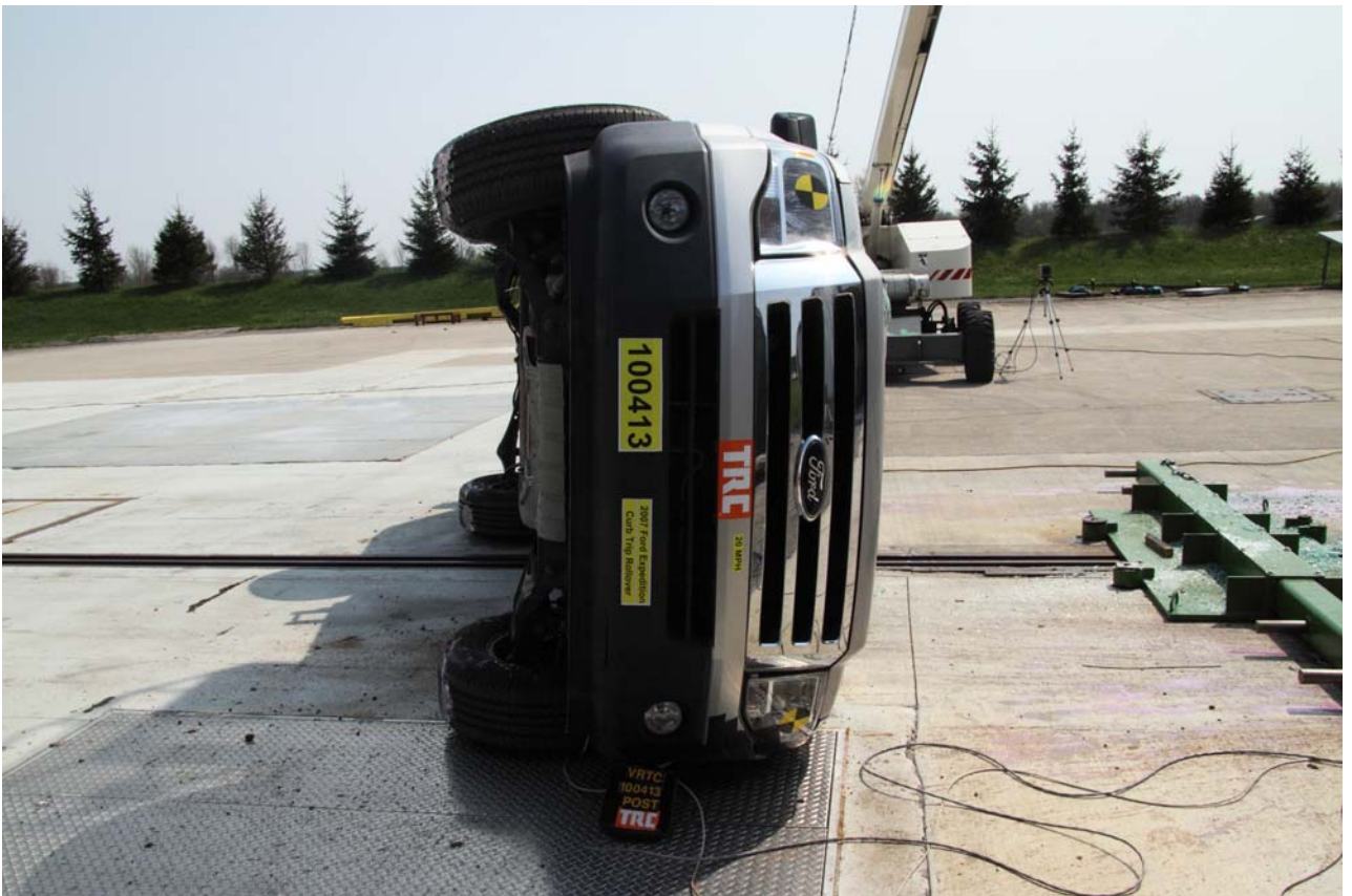
Figure A-58 Post-Test Vehicle Resting Position – Front
