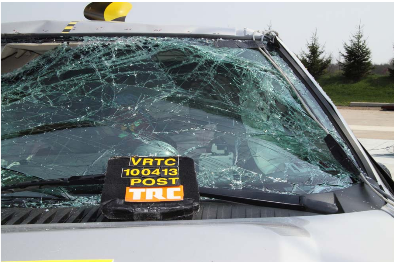
Figure A-24 Post-Test Windshield View – Driver Dummy
