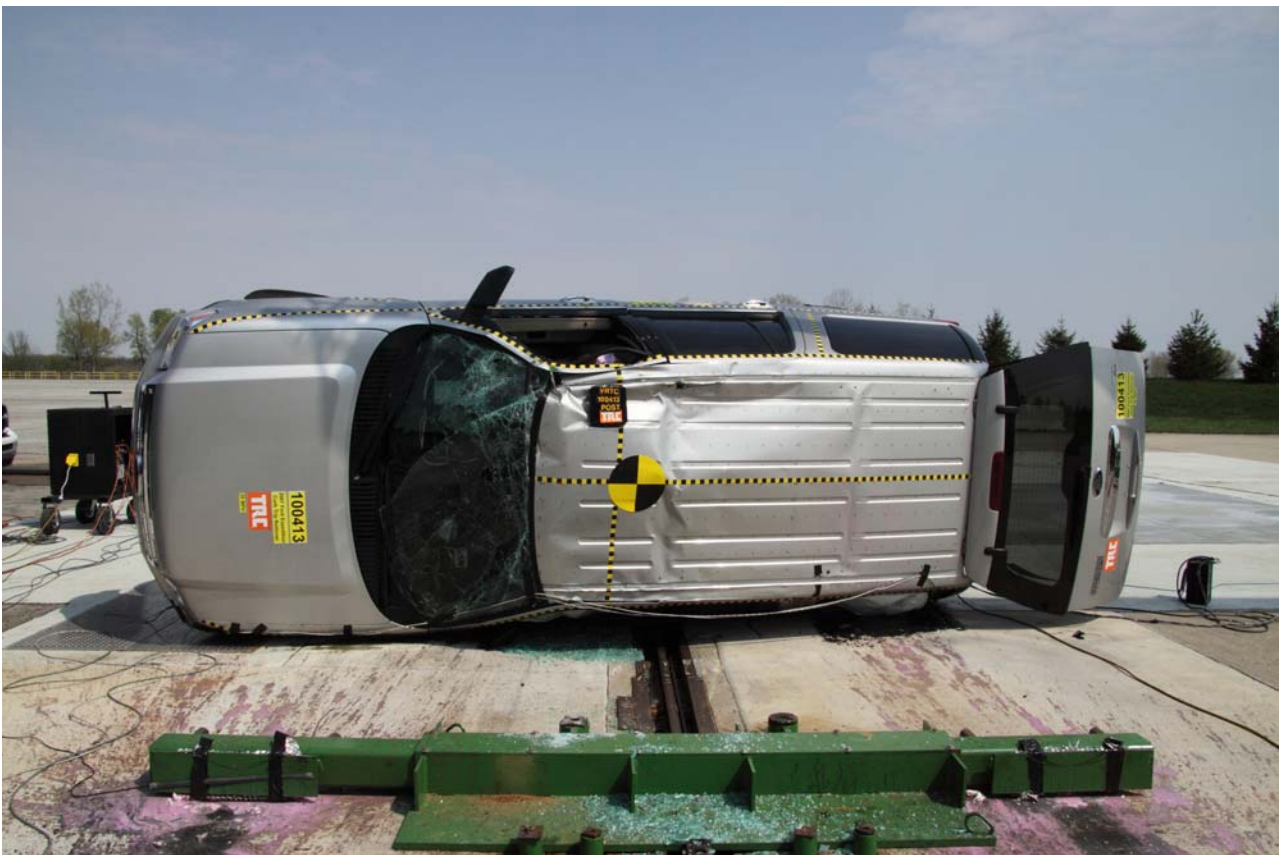
Figure A-59 Post-Test Vehicle Resting Position – Left Side
