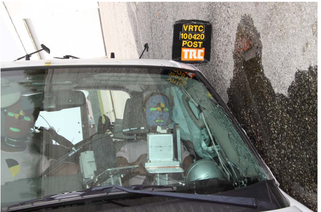
Figure A-24 Post-Test Windshield View – Driver Dummy
