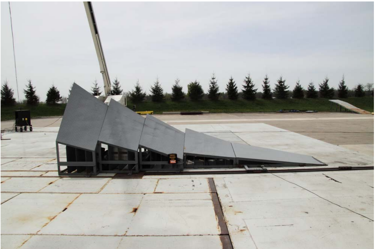
Figure A-81 Pre-Test Corkscrew Ramp – Left Side View
