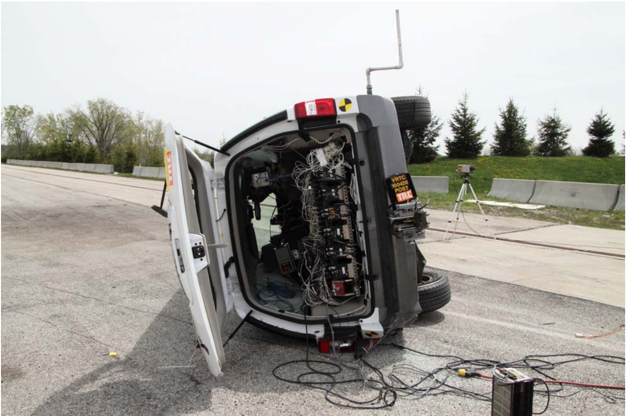
Figure A-78 Post-Test Vehicle Resting Position – Rear View
