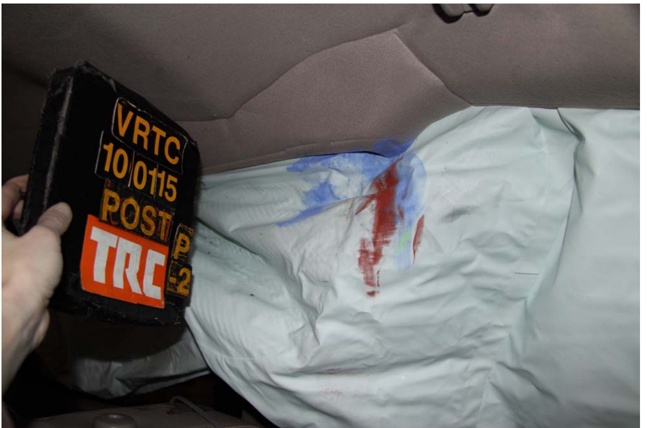
Figure A-58 Post-Test Left Rear Passenger Dummy Contact View
