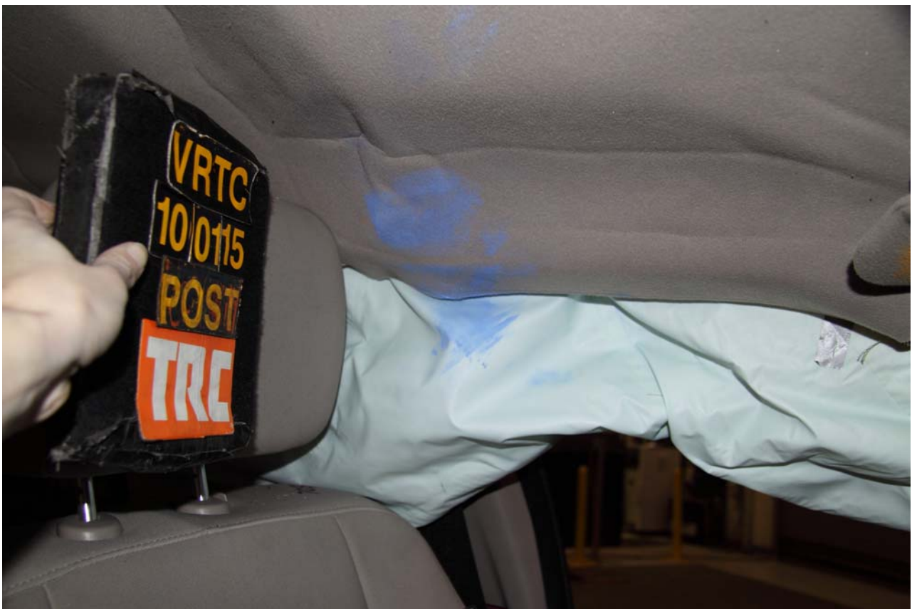
Figure A-54 Post-Test Driver Dummy Contact - View 1
