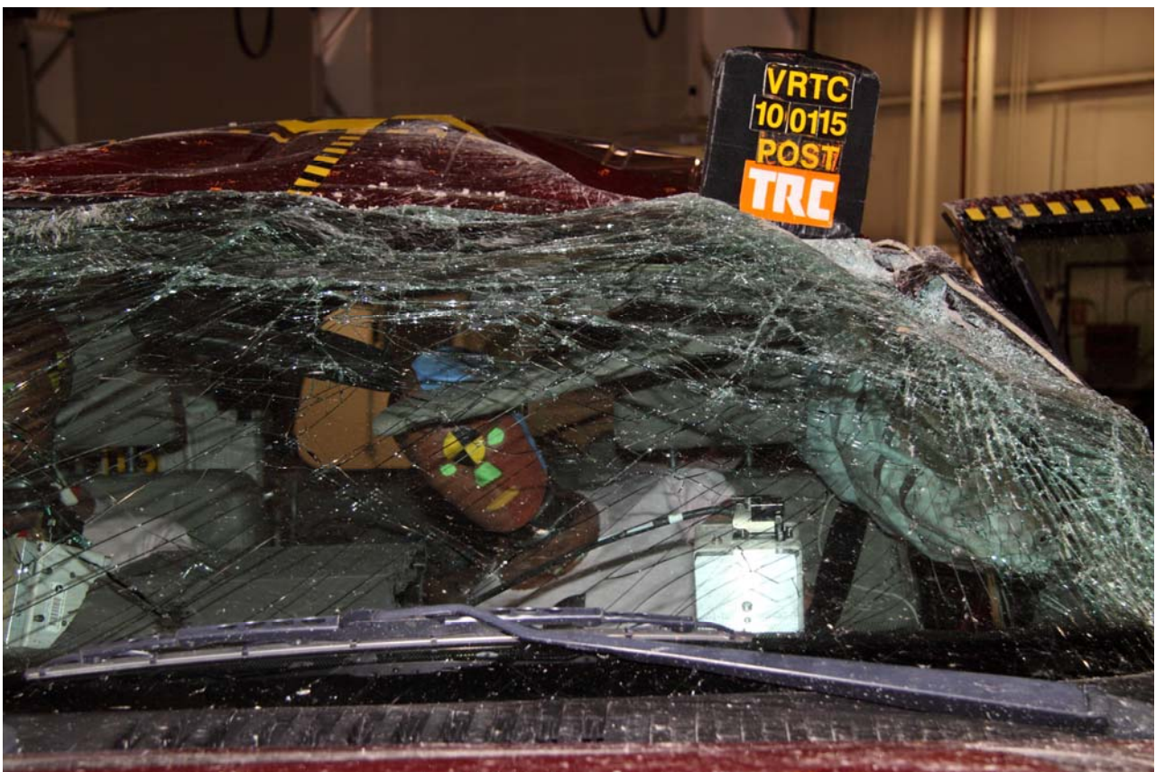
Figure A-24 Post-Test Windshield View – Driver Dummy
