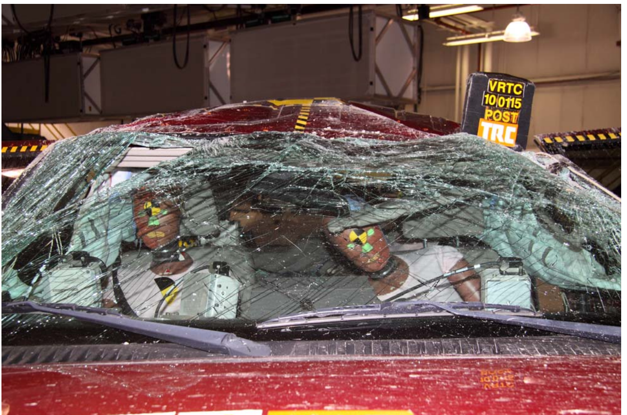
Figure A-22 Post-Test Windshield View
