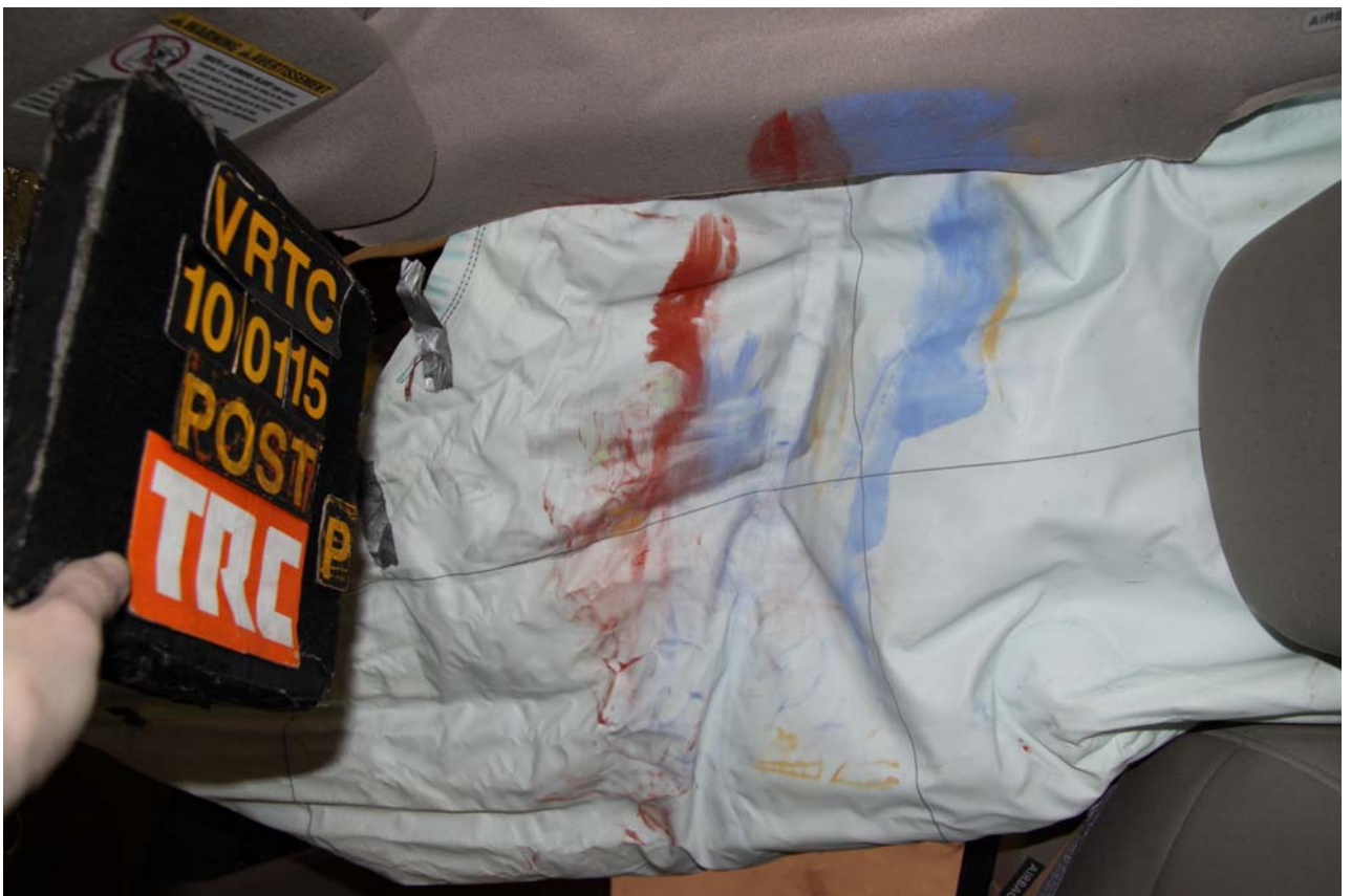
Figure A-56 Post-Test Right Front Passenger Dummy Contact - View 1
