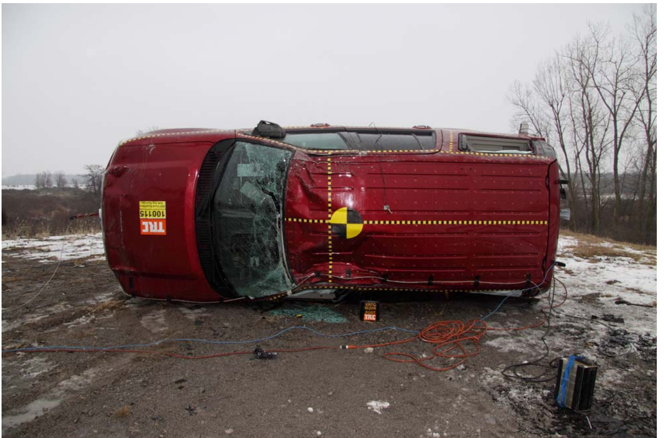
Figure A-66 Post-Test Vehicle Resting Position – Left Side
