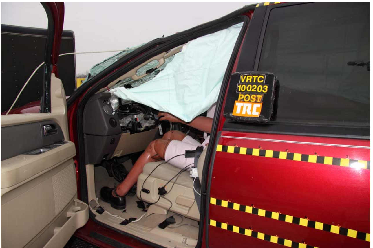
Figure A-28 Post-Test Driver Dummy - View 2
