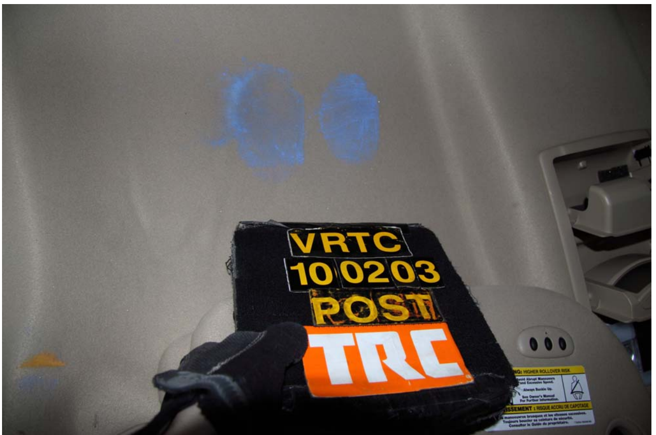
Figure A-51 Post-Test Driver Dummy Contact - View 1
