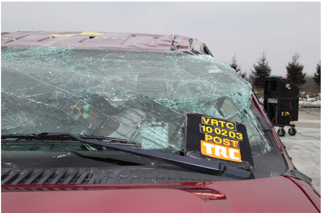
Figure A-24 Post-Test Windshield View – Driver Dummy
