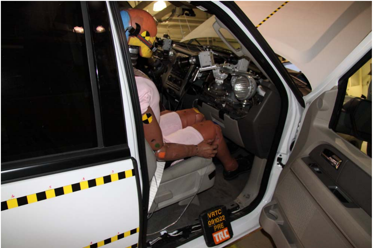
Figure A-40 Pre-Test Right Front Passenger Dummy - View 3
