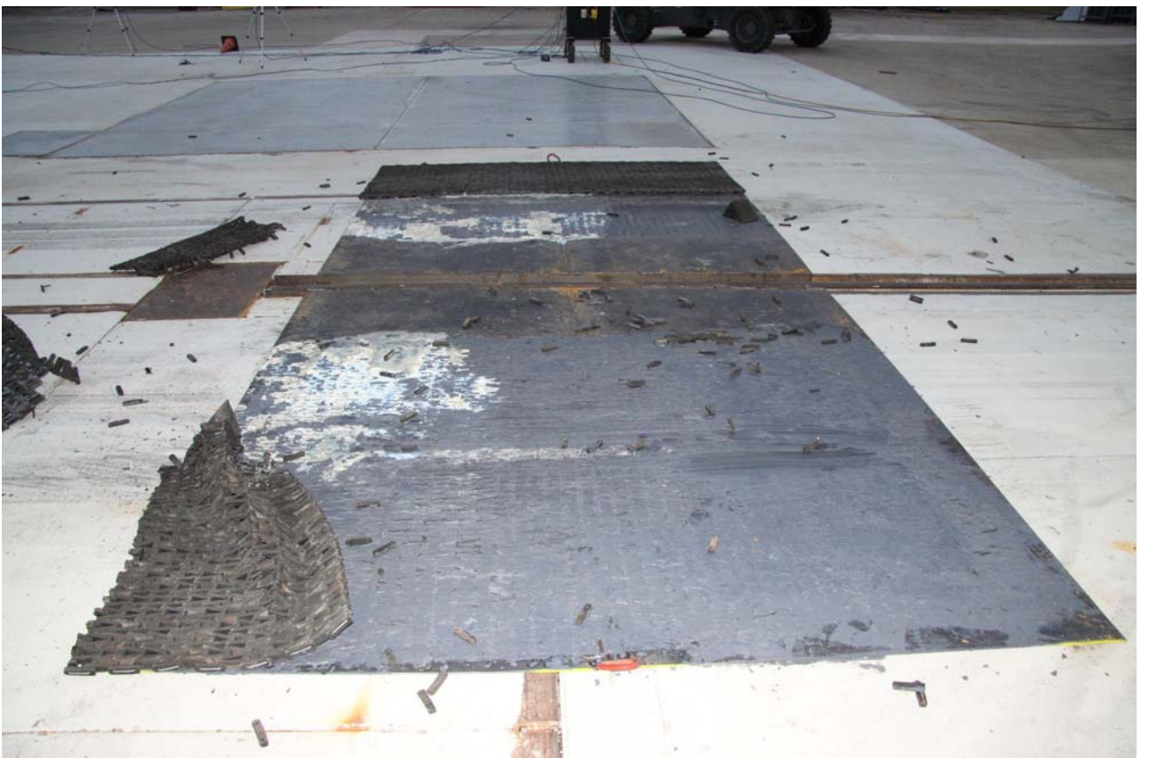
Figure A-67 Post-Test Mat Displacement – View 4
