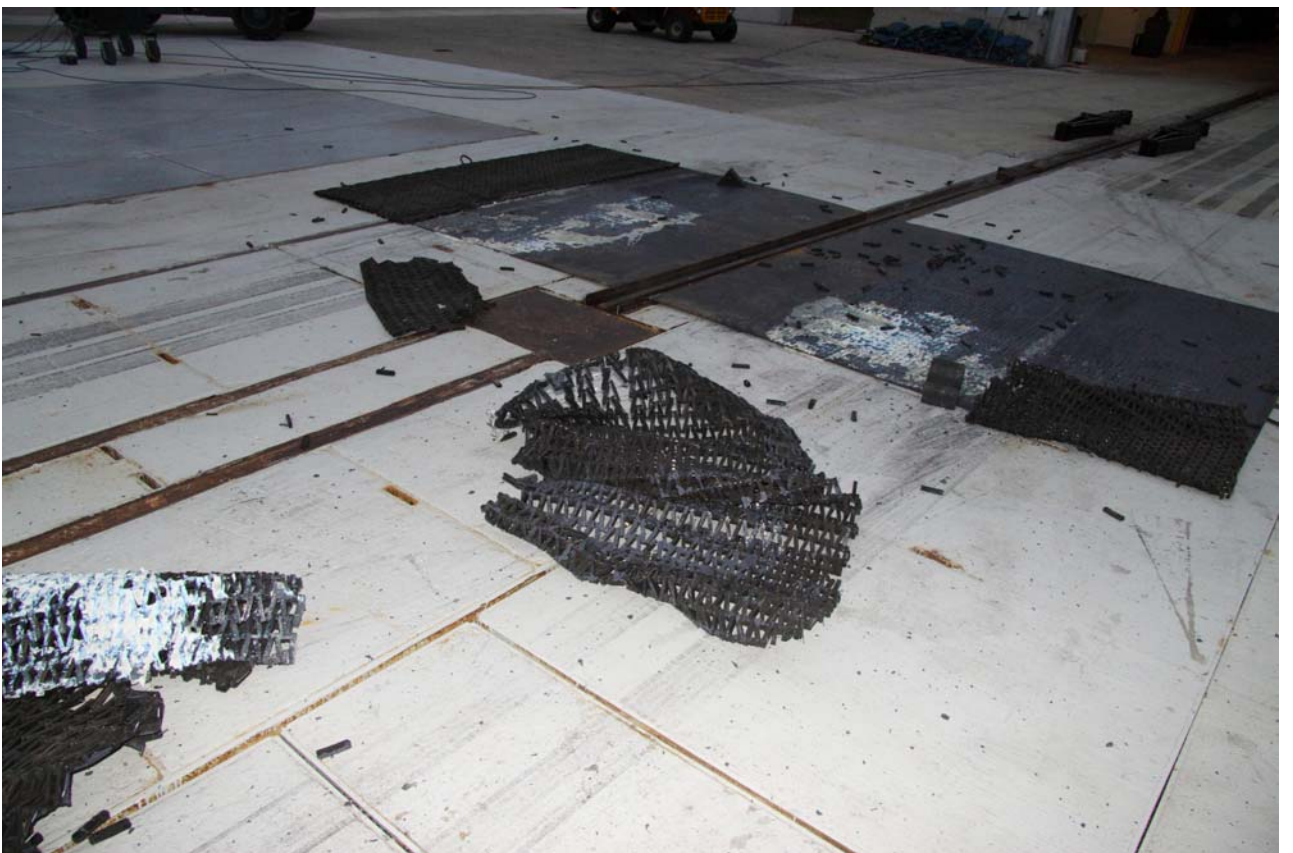
Figure A-69 Post-Test Mat Displacement – View 6
