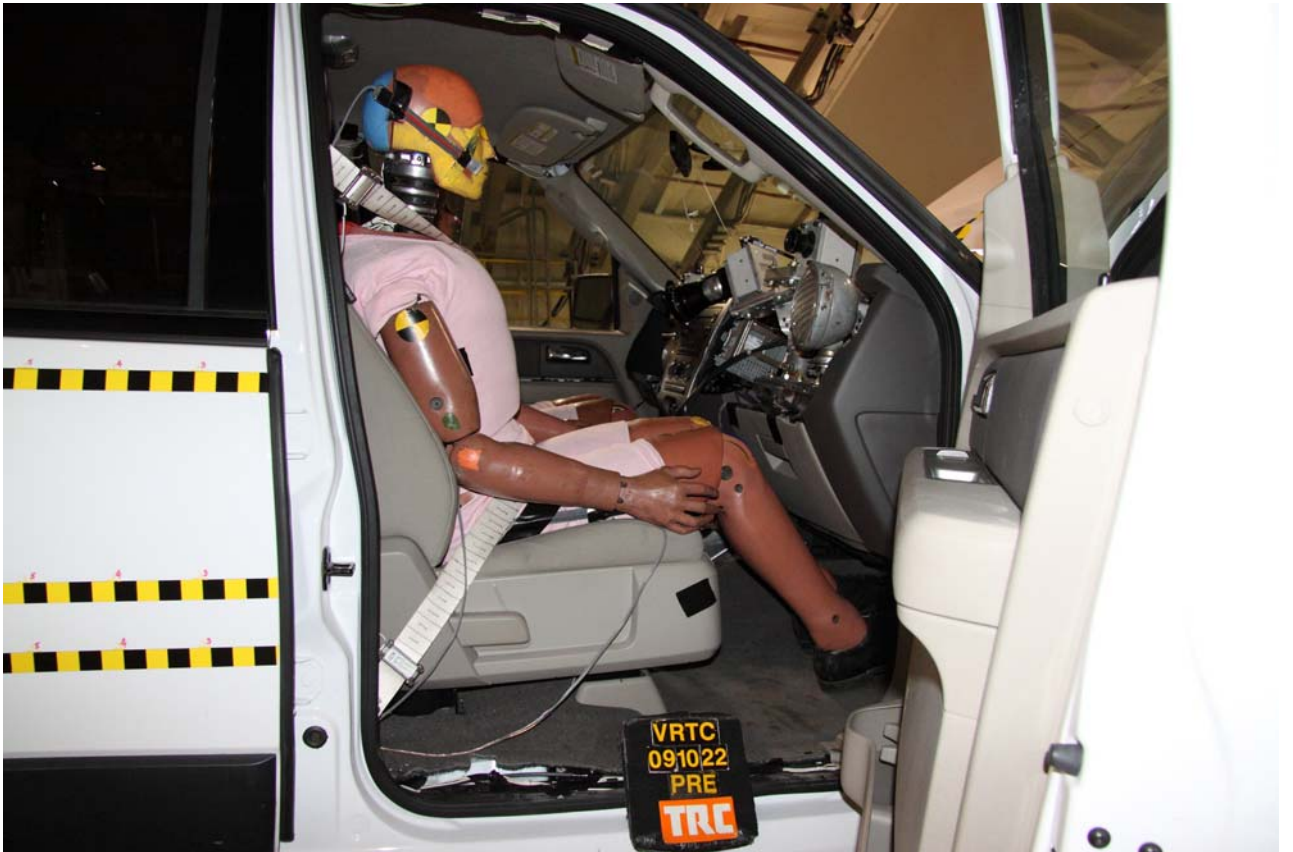
Figure A-38 Pre-Test Right Front Passenger Dummy - View 2
