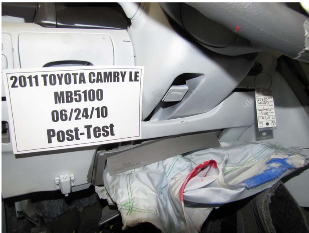
FIGURE 45. Post-Test View of Steering Column Shear Capsule
