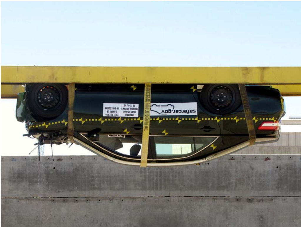
FIGURE 66. Vehicle at 180°on Static Rollover Device
