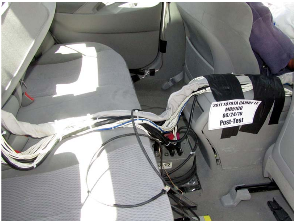
FIGURE 28. Post-Test Dummy Cable Routing
