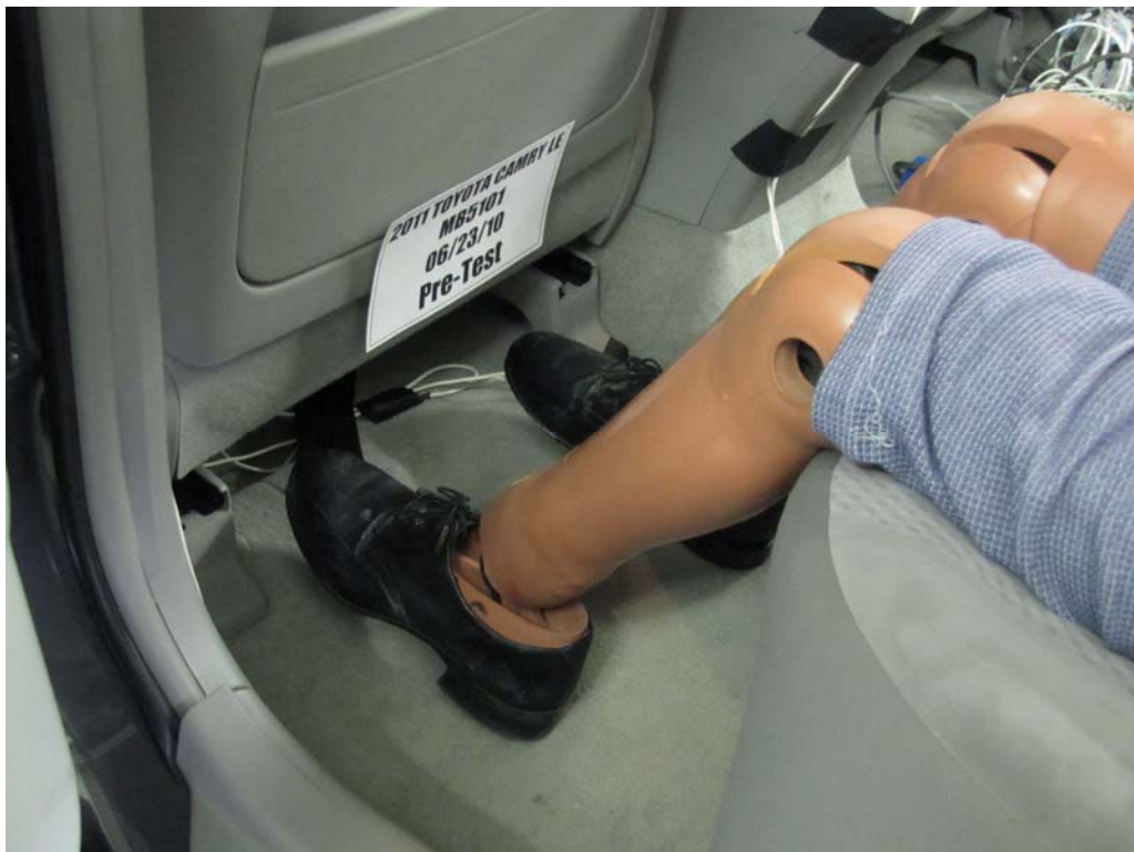
FIGURE 62. Pre-Test Placement of Rear Passenger Dummy's Feet
