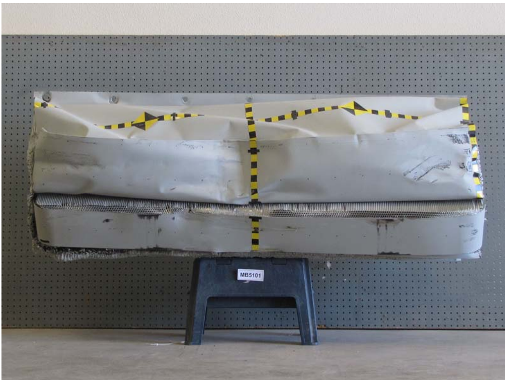
FIGURE 82. Post-Test Front View of MDB Impactor Face
