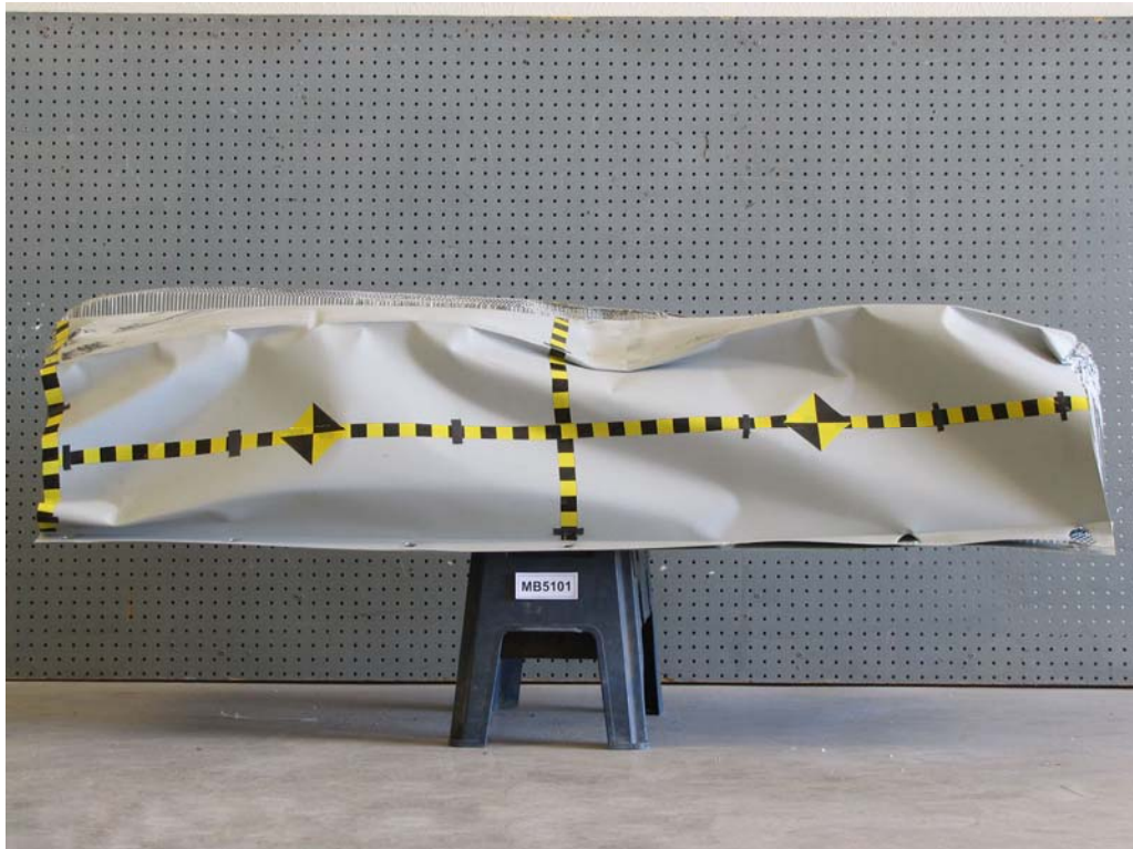
FIGURE 84. Post-Test Top View of MDB Impactor Face
