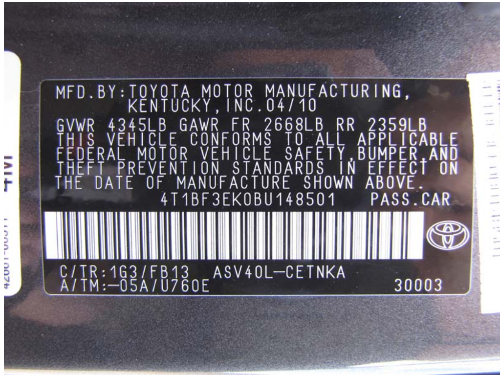
FIGURE 89. Close-Up View of Vehicle's Certification Label
