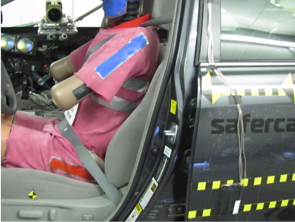
FIGURE 39. Pre-Test Close-Up Left Side View of Driver Seat Back Showing Test Position
