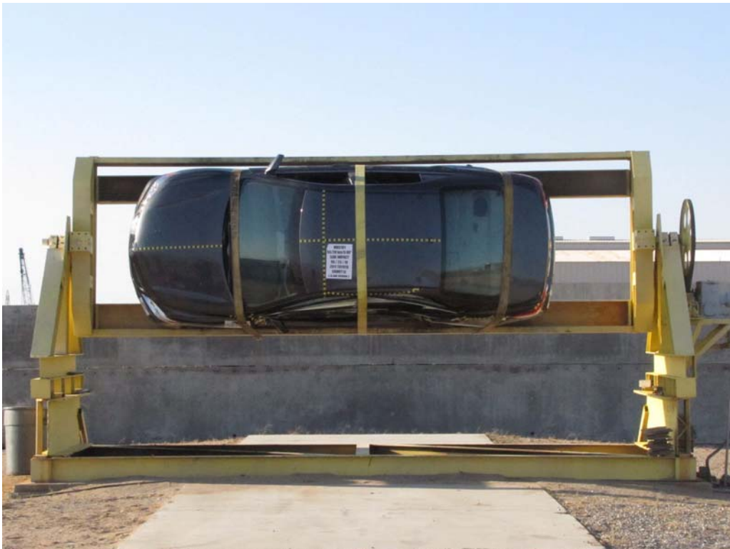
FIGURE 94. FMVSS No. 301/305 Rollover 90°
