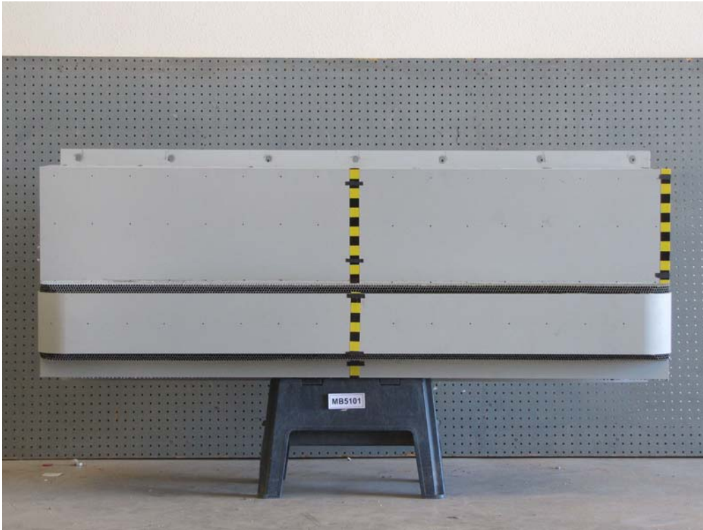
FIGURE 81. Pre-Test Front View of MDB Impactor Face
