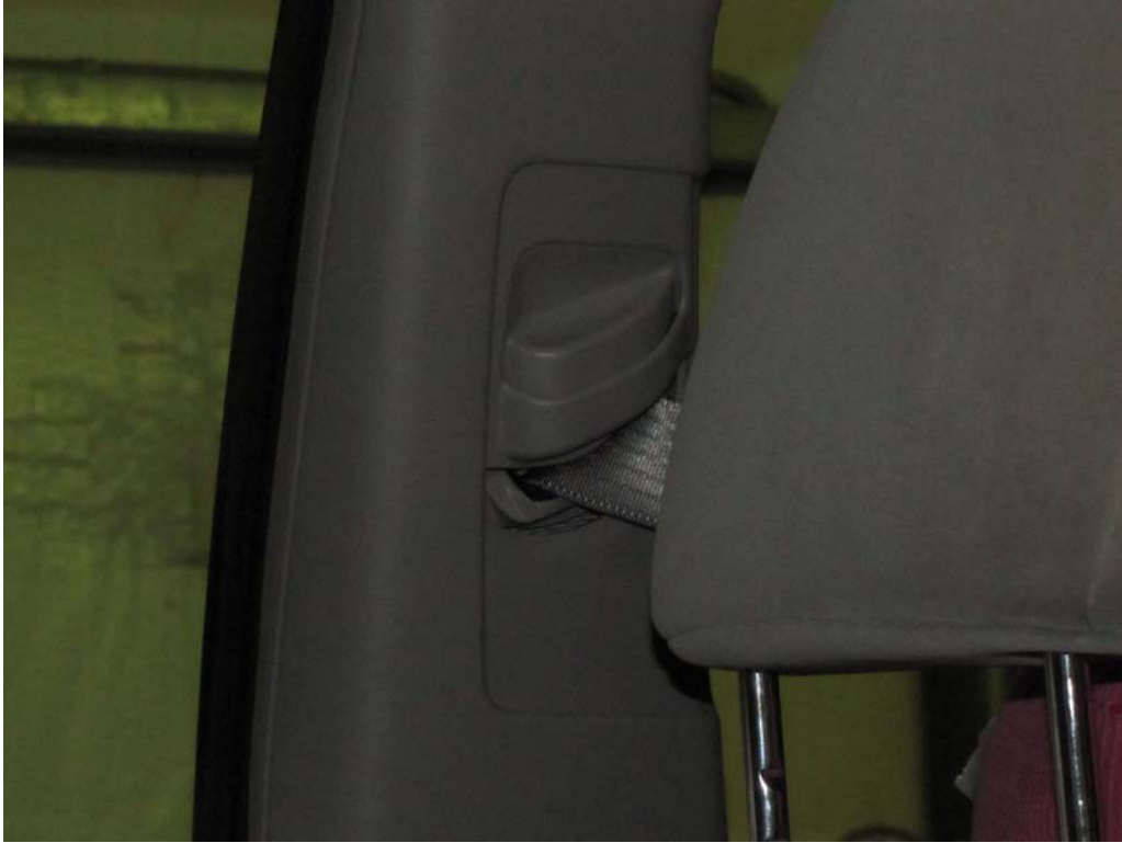
FIGURE 35. Pre-Test View of Belt Anchorage for Driver Dummy to Show Position
