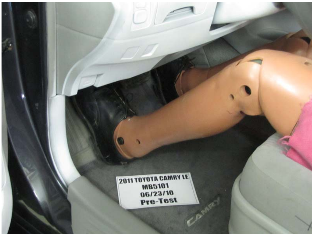
FIGURE 34. Pre-Test Placement of Driver Dummy's Feet
