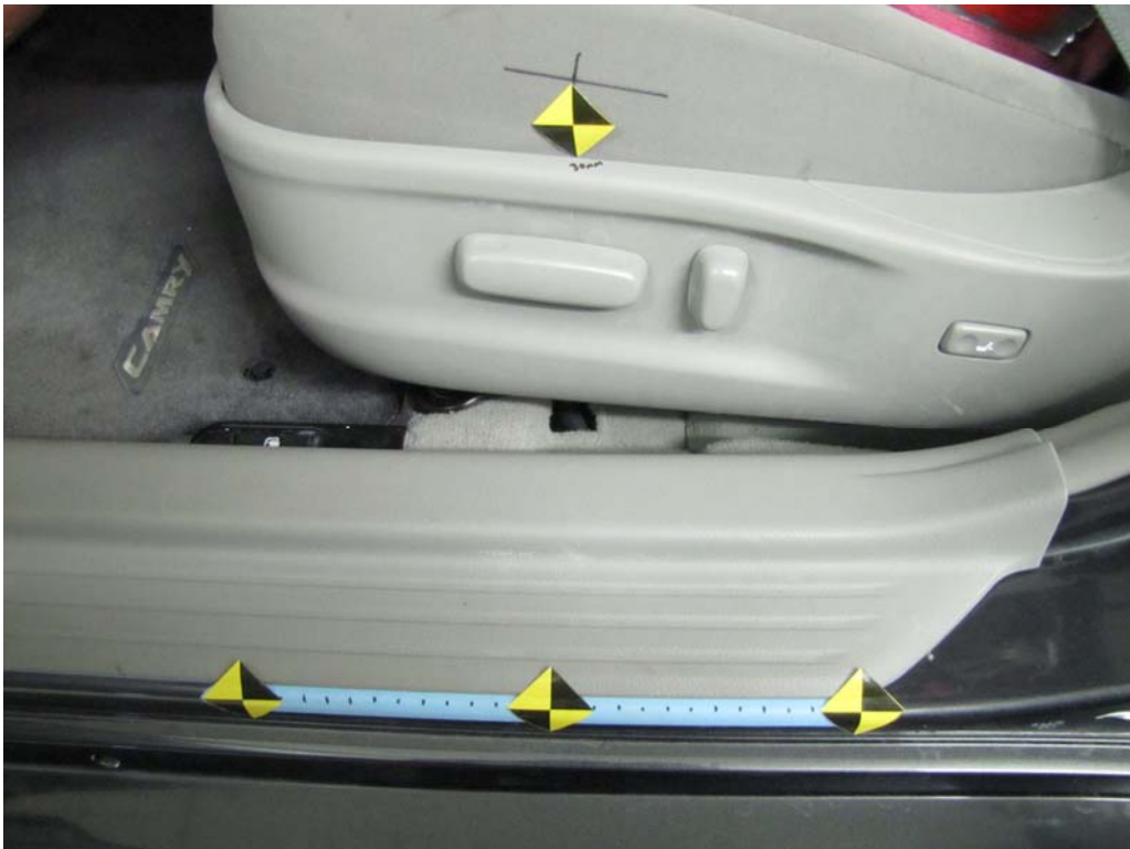
FIGURE 38. Pre-Test Close-Up Left Side View of Driver Seat Track Showing Test Position
