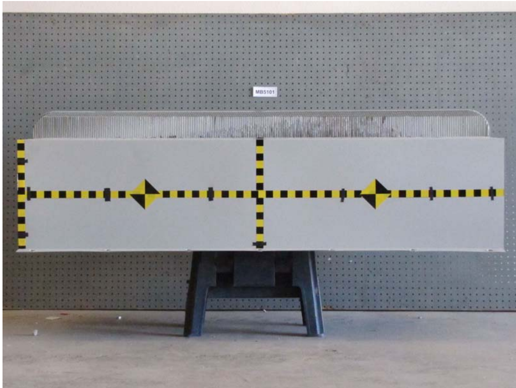
FIGURE 83. Pre-Test Top View of MDB Impactor Face
