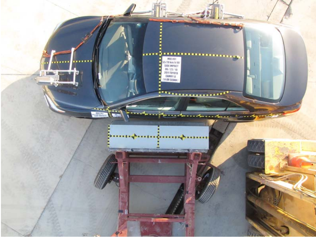
FIGURE 15. Pre-Test Overhead View of Test Vehicle with MDB Positioned Against Side of Target Vehicle at Ideal Impact Point
