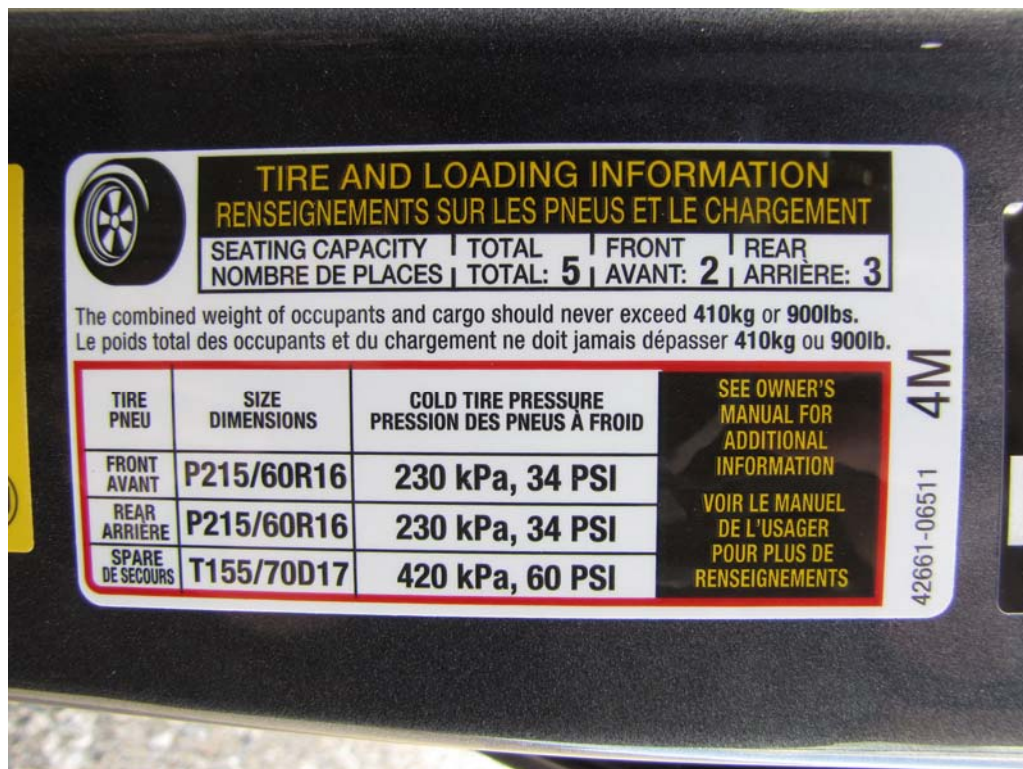
FIGURE 90. Close-Up View of Vehicle's Tire Information Placard
