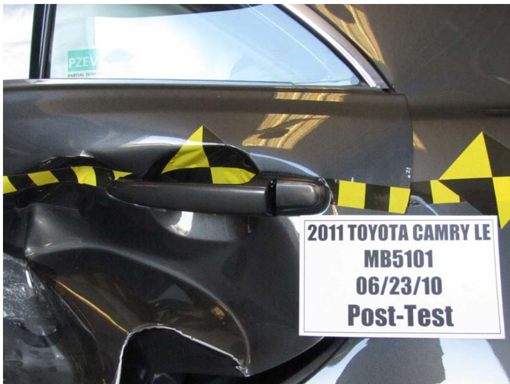
FIGURE 24. Post-Test Left Rear Door Latch Close-Up
