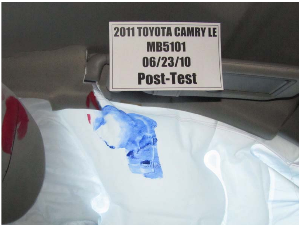
FIGURE 48. Post-Test Driver Dummy Close-Up Head Contact with Side Airbag View
