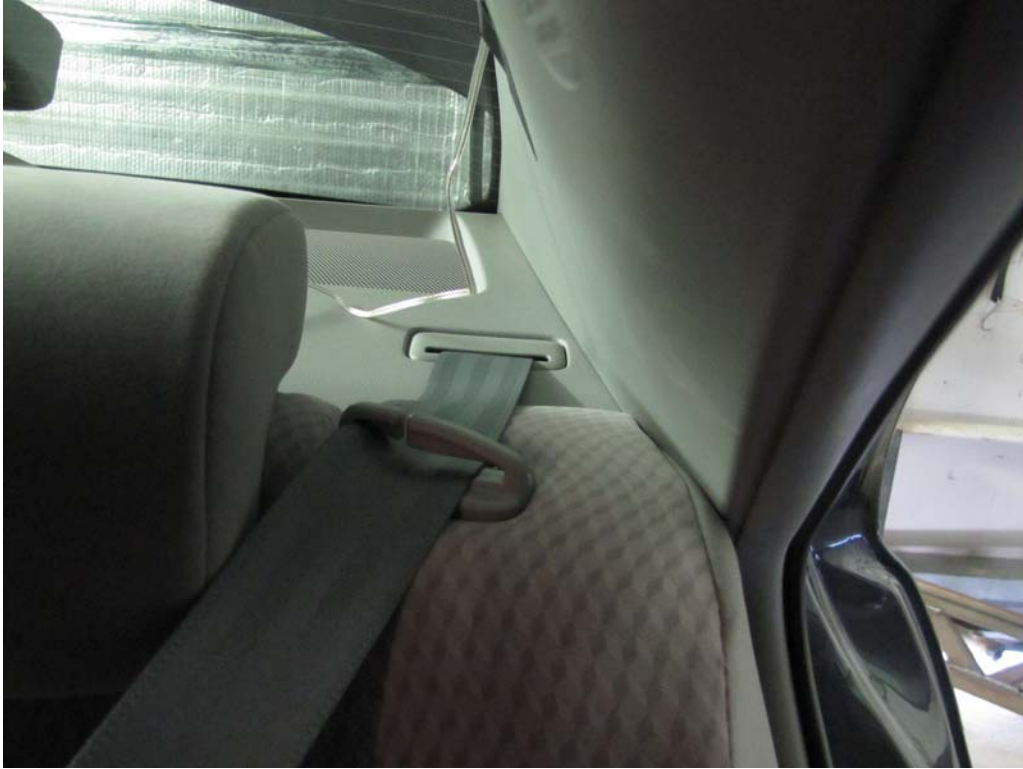
FIGURE 63. Pre-Test View of Belt Anchorage for Rear Passenger Dummy to Show Position
