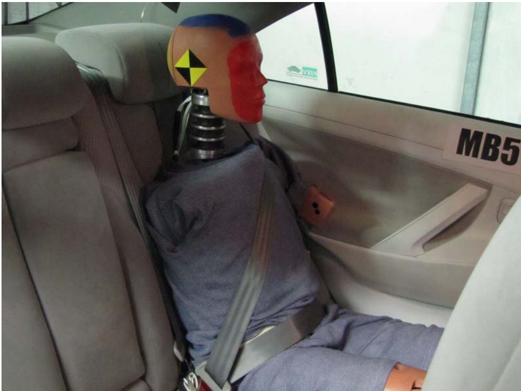
FIGURE 66. Pre-Test Close-Up View of Rear Passenger Seat Back or Head Restraint Showing Seat Back Test Position
