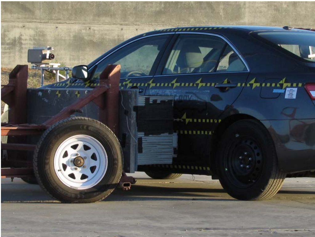
FIGURE 18. Pre-Test Right Side View of MDB Positioned Against Side of Target Vehicle at Ideal Impact Point
