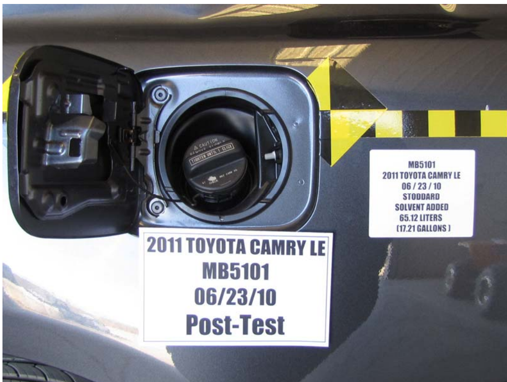
FIGURE 80. Post-Test View of Fuel Filler Cap
