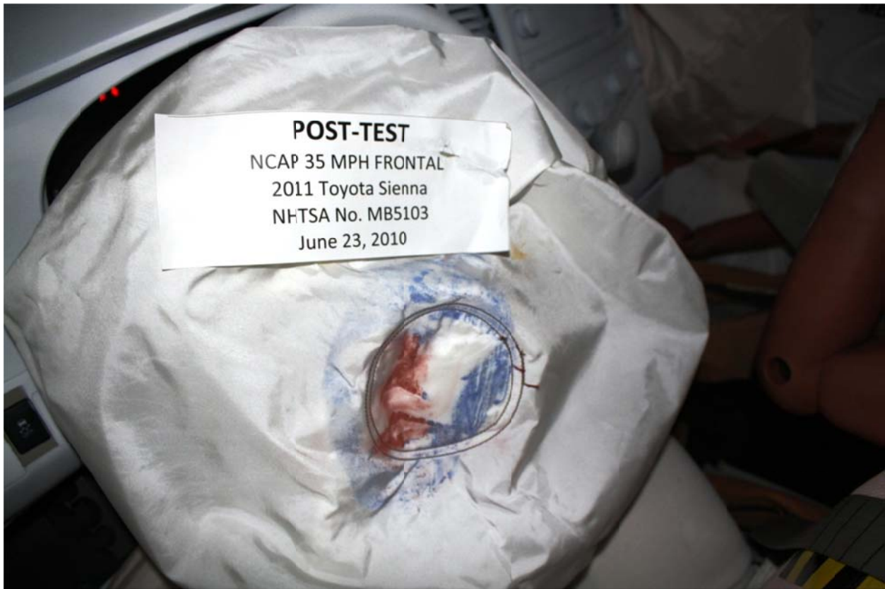
Figure A-43a: Post-Test Diver Dummy Contact with Airbag
