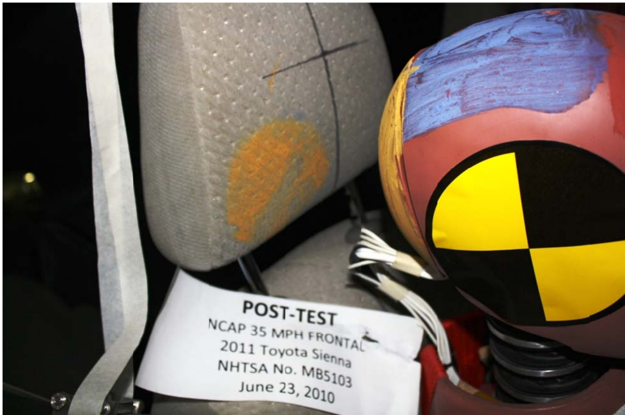
Figure A-60b: Post-Test Passenger Dummy Contact with Head Restraint
