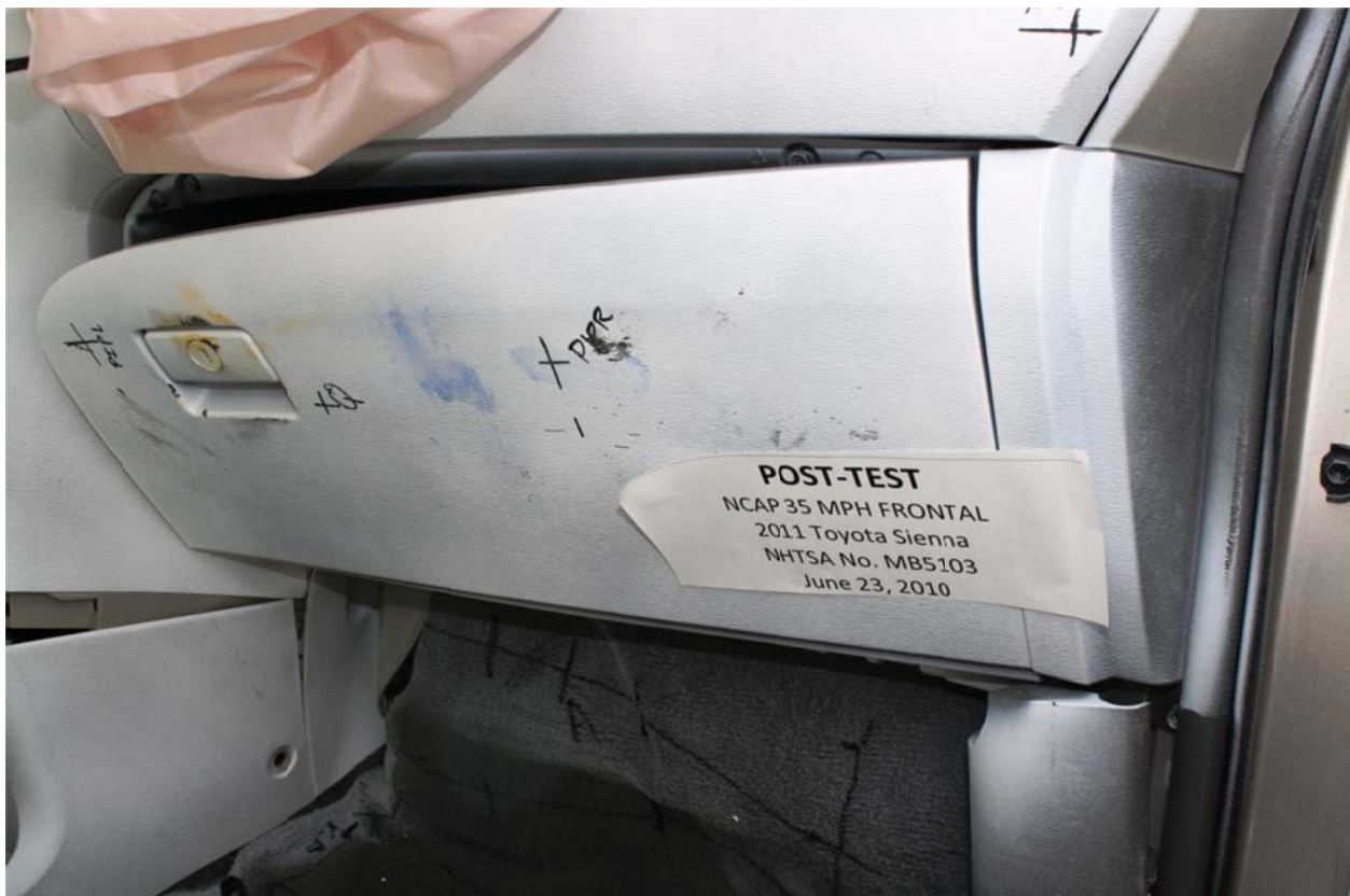
Figure A-57: Post-Test Passenger's Side Knee Bolster
