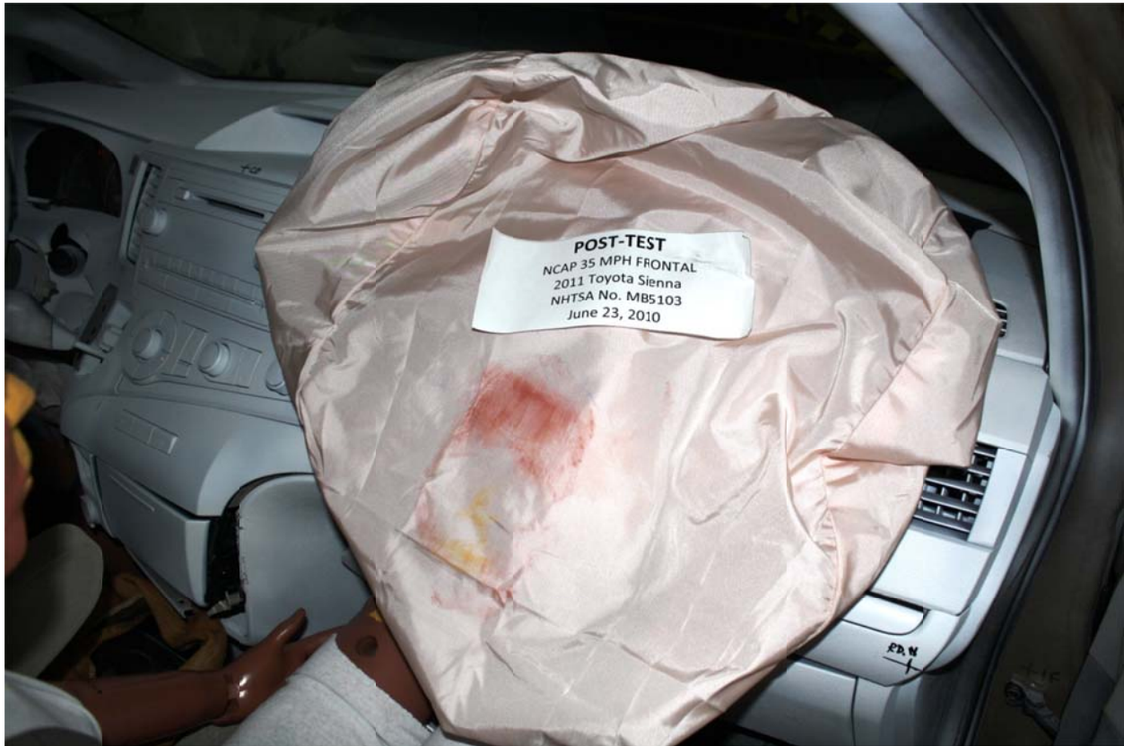
Figure A-60a: Post-Test Passenger Dummy Conatact with Airbag
