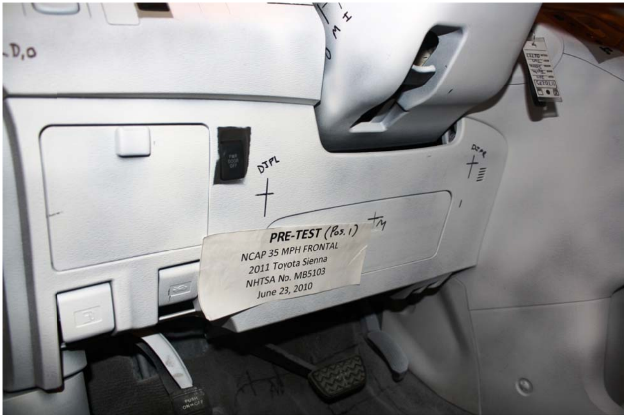
Figure A-39: Pre-Test Driver's Side Knee Bolster
