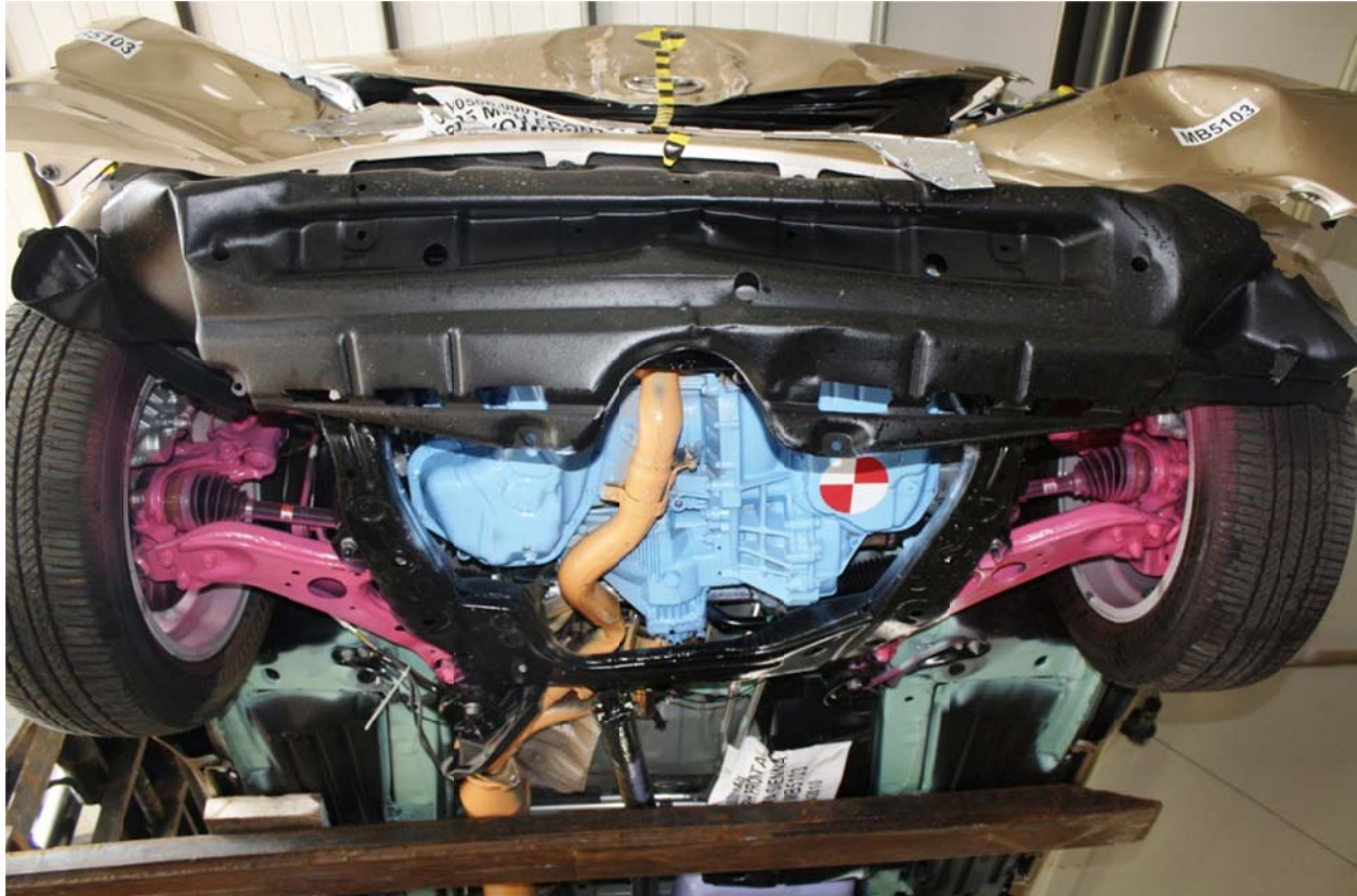
Figure A-24: Post-Test Front Underbody View
