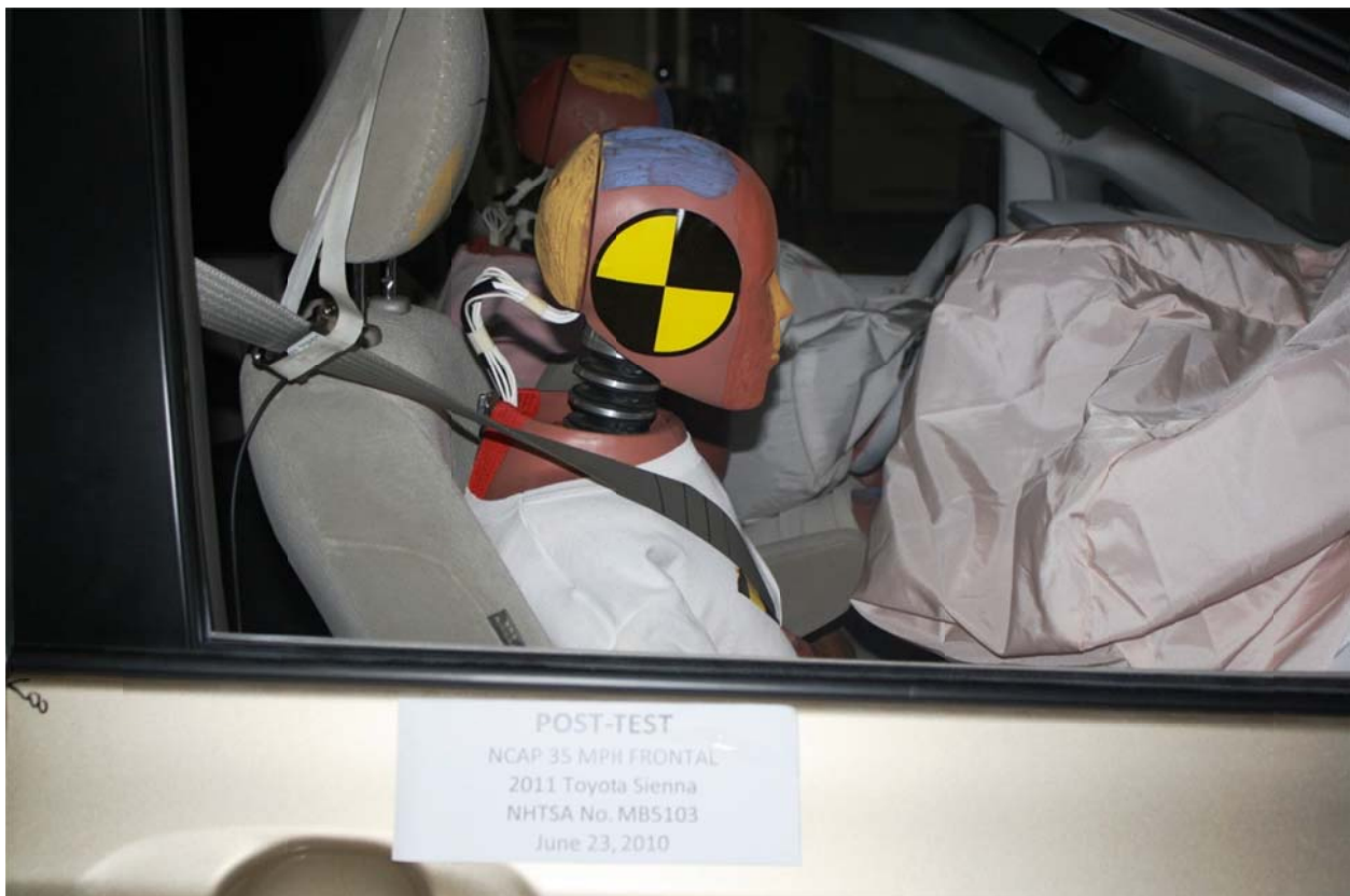
Figure A-49: Post-Test Passenger Dummy Window View
