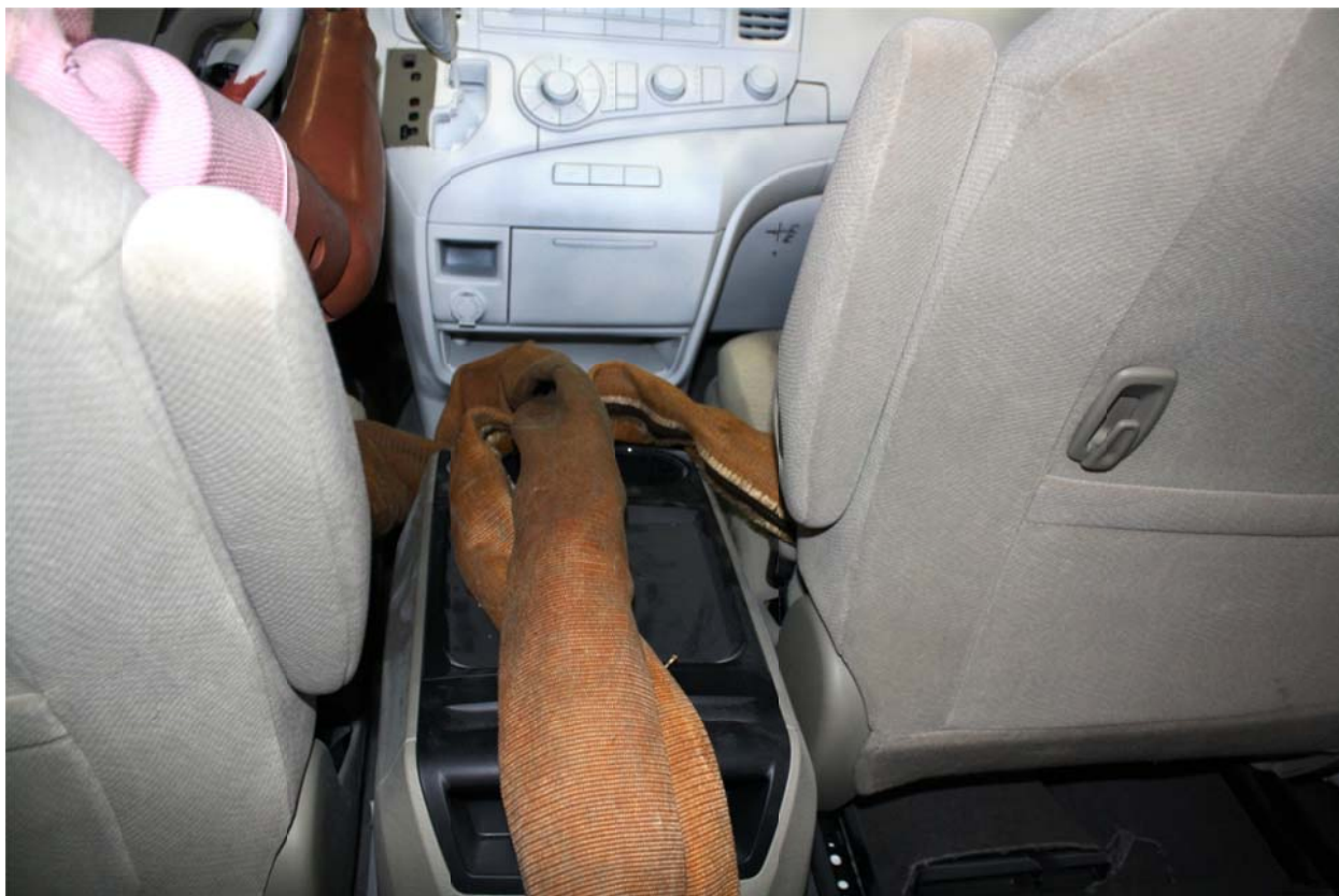
Figure A-27: Pre-Test Dummy Cable Routing
