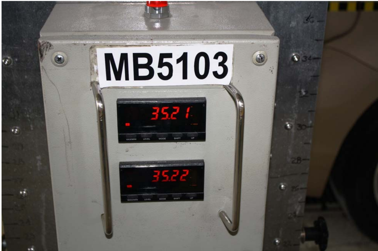
Figure A-63: Post-Test Speed Trap Read Out
