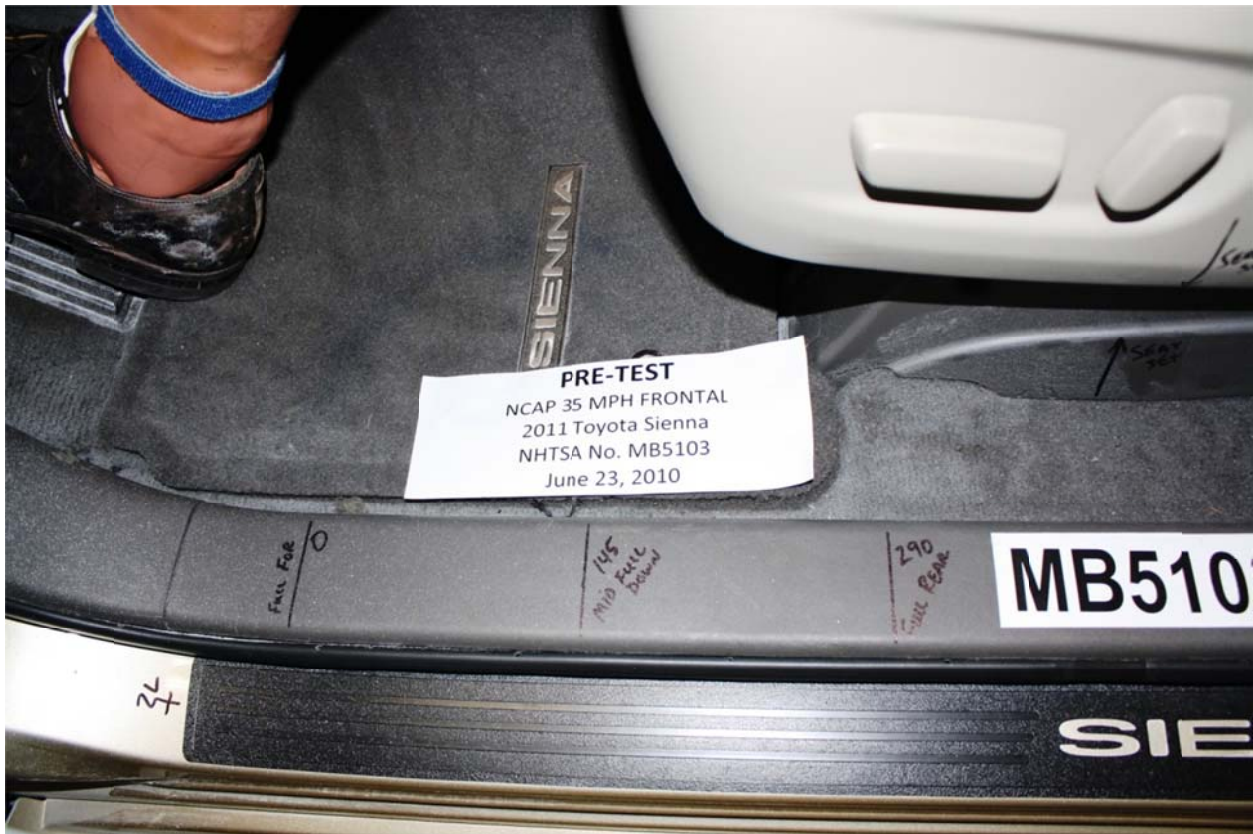
Figure A-35: Pre-Test Driver's Seat Fore-Aft Markings
