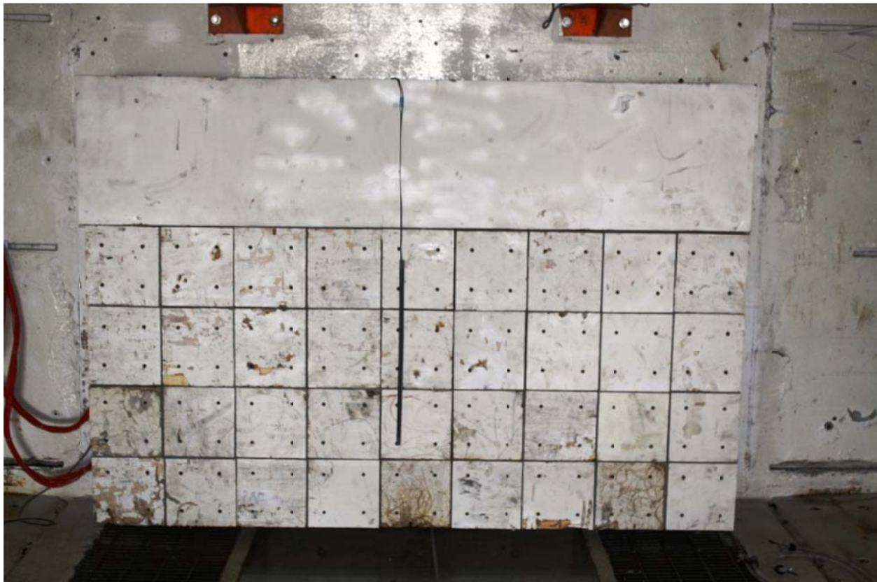
Figure A-2: Load Cell Wall
