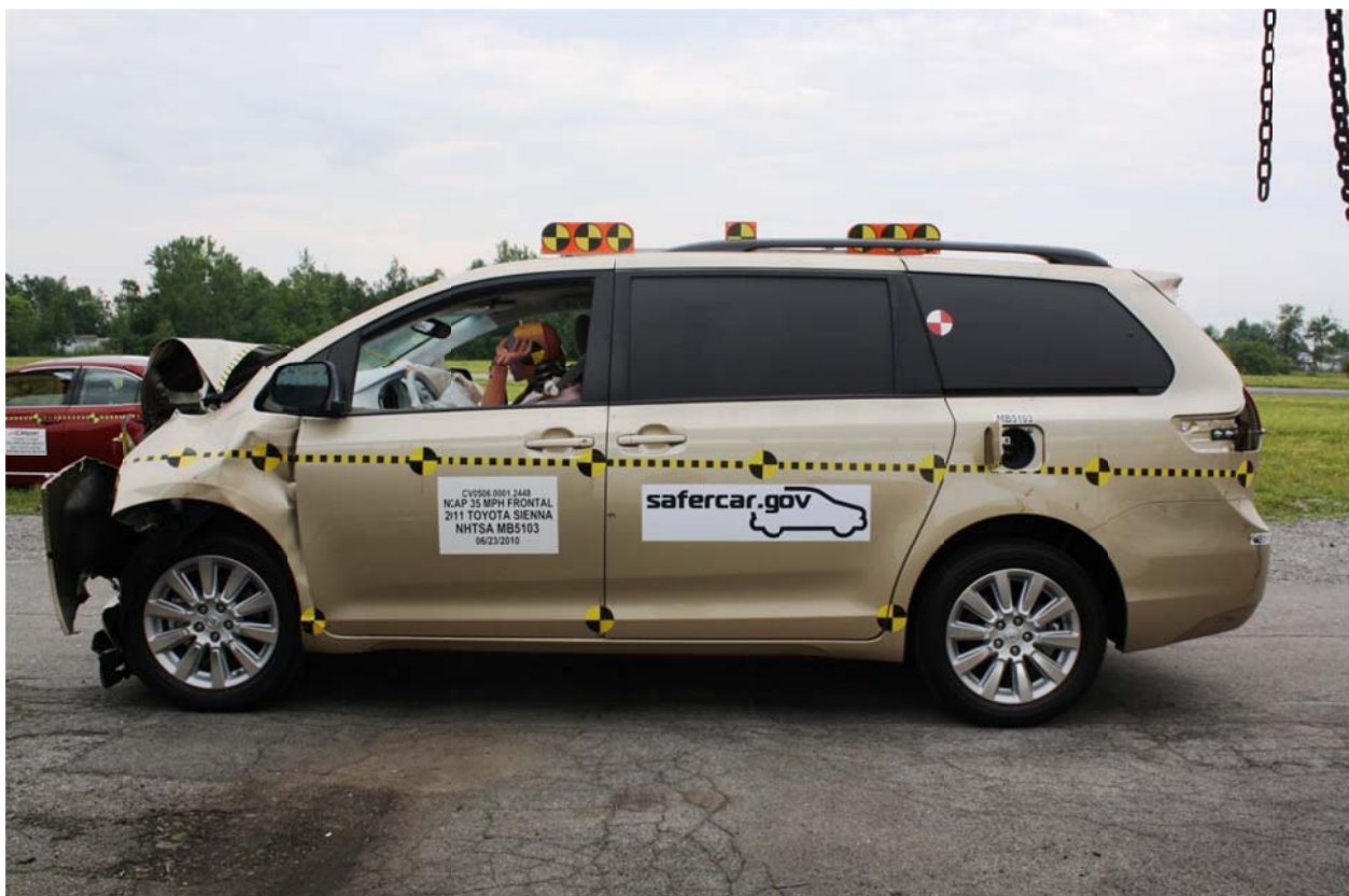
Figure A-10 – Post-Test Left View of Vehicle
