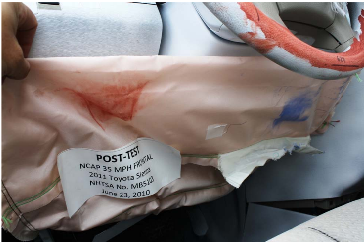
Figure A-40: Post-Test Driver's Side Knee Bolster
