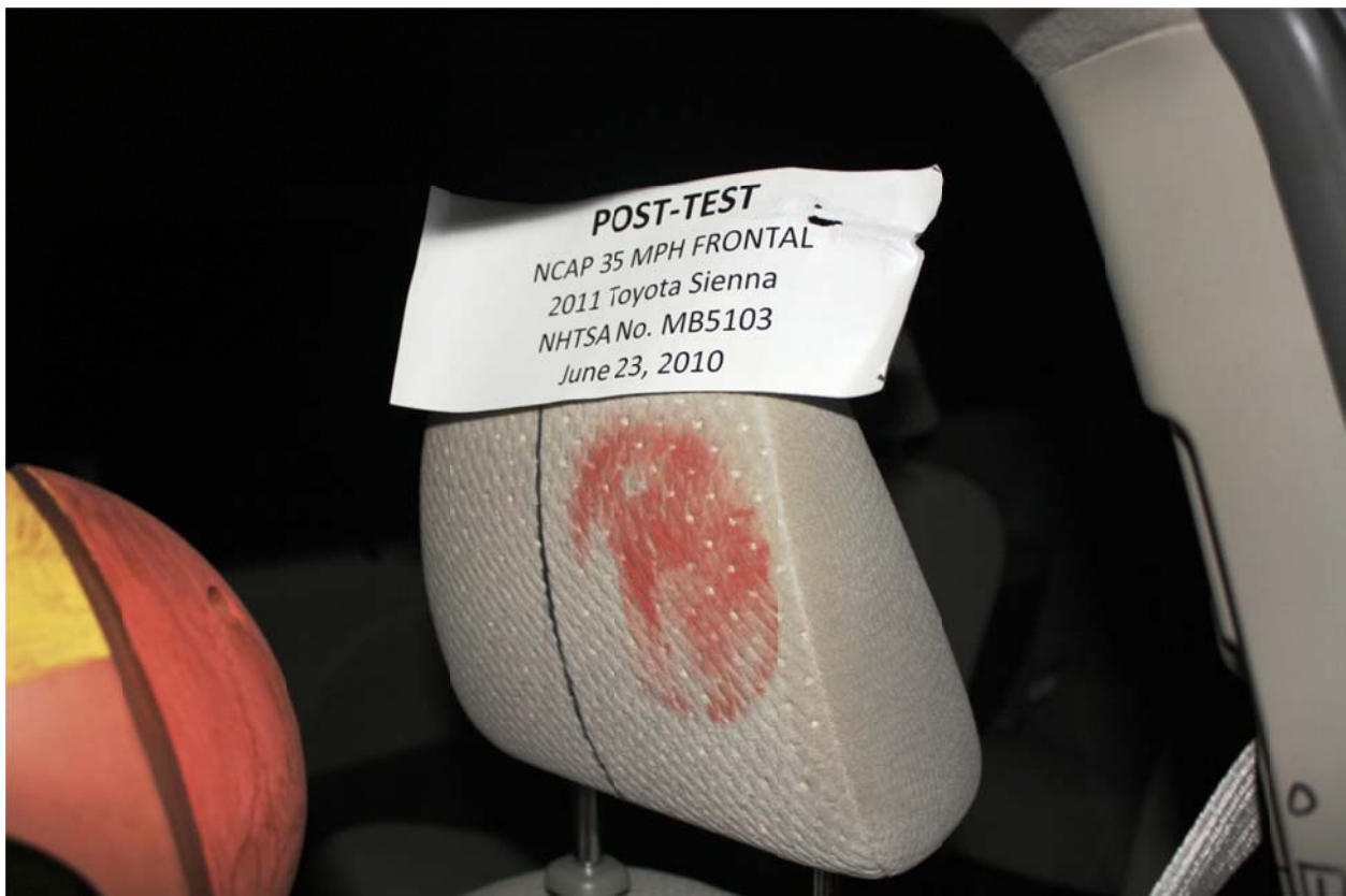
Figure A-43b: Post-Test Driver Dummy Contact with Head Restraint
