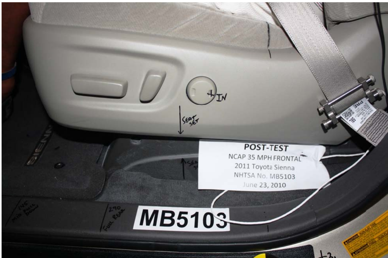
Figure A-36: Post-Test Driver's Seat Fore-Aft Markings
