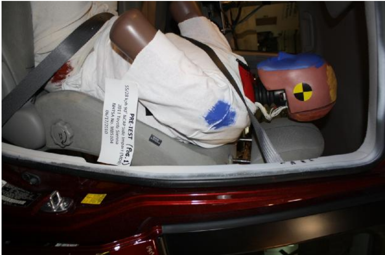
Figure A-53: Pre-Test Left Side View of Rear Passenger Dummy Showing Belt, Chalking, and Contact Switches
