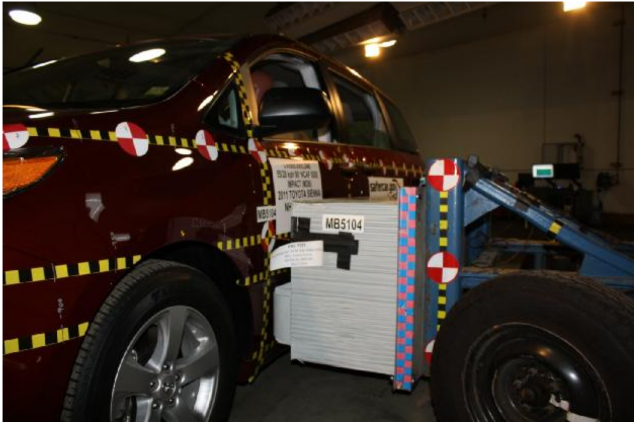
Figure A-17: Pre-Test Left Side View of MDB Positioned against Side of Target Vehicle at Ideal Impact Point
