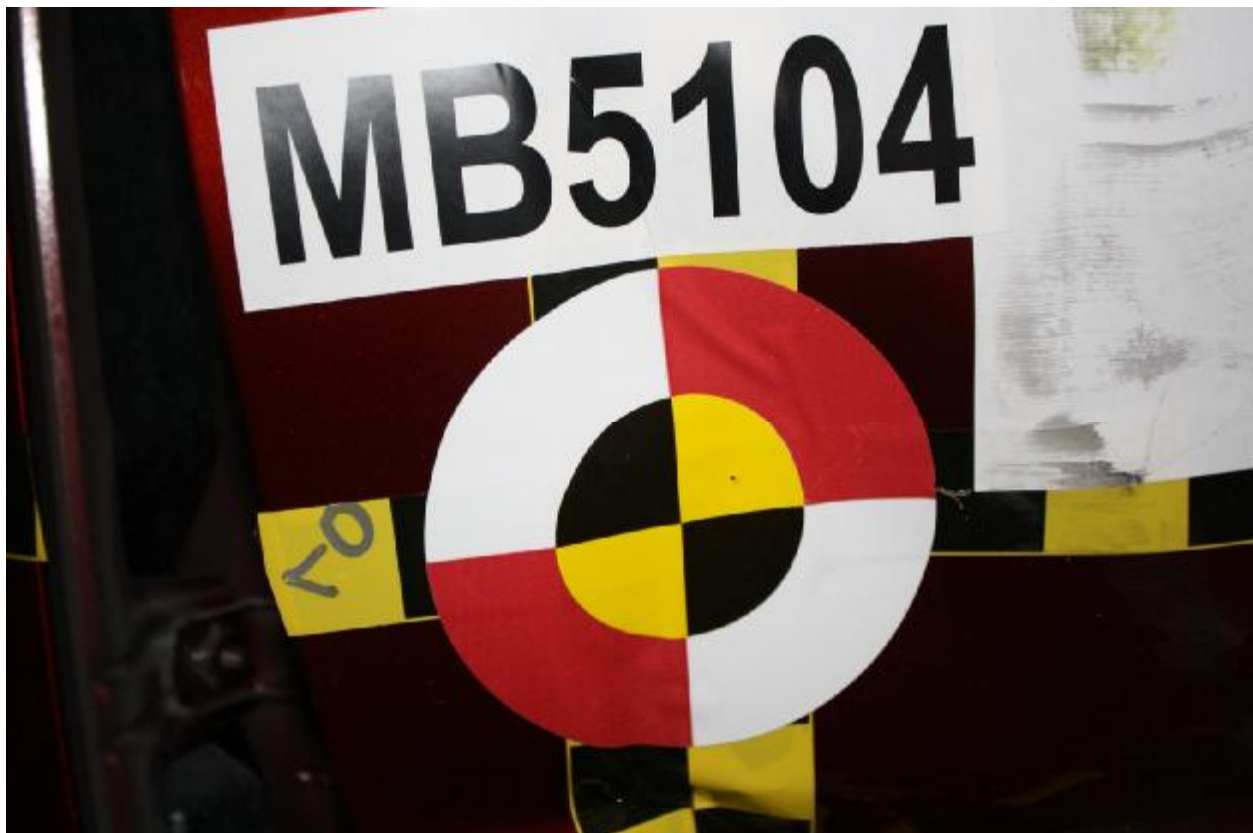
Figure A-20: Post-Test Close-Up View of Impact Target Point
