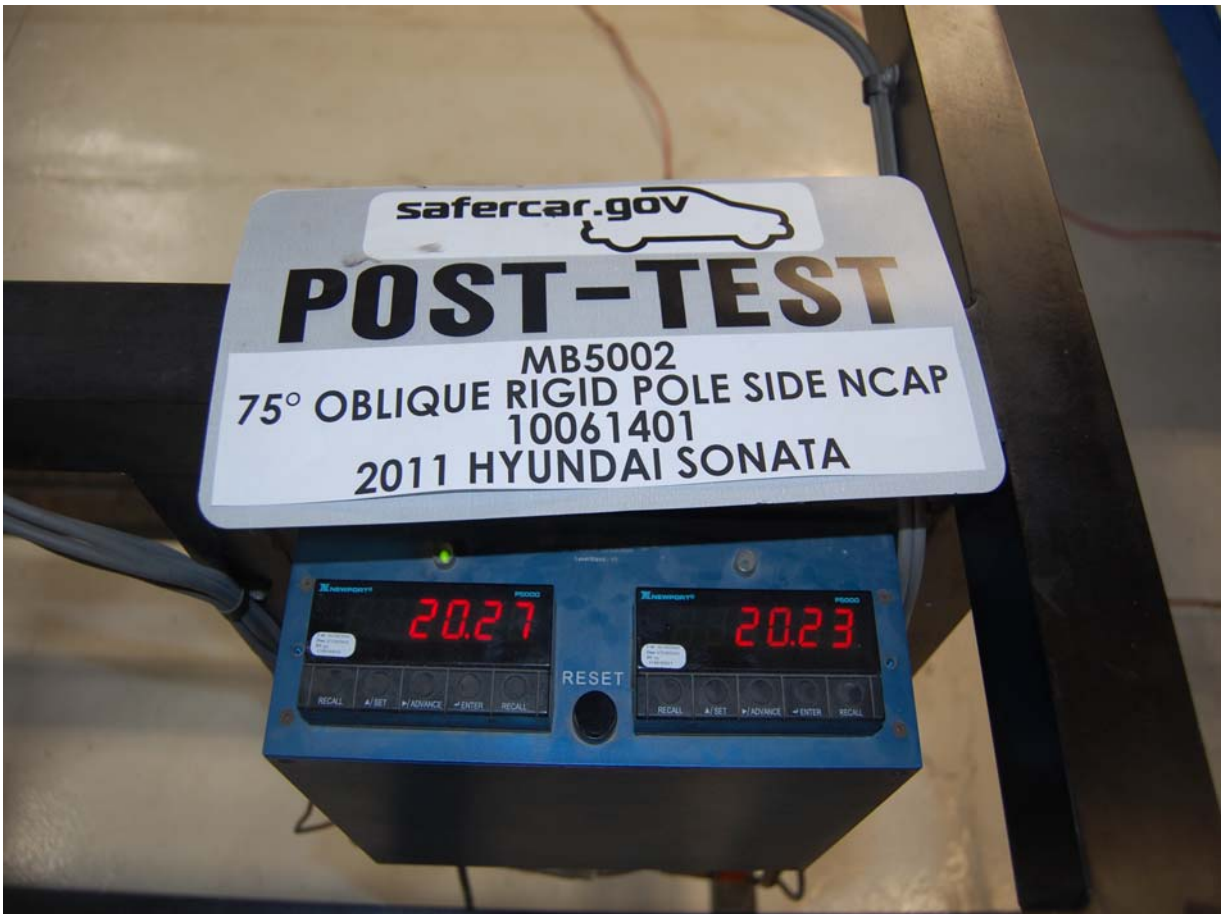
Post-Test Primary and Redundant Speed Trap Read-Out
