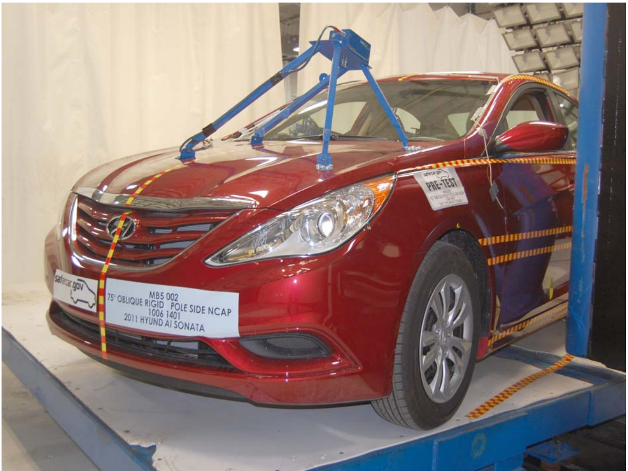
Pre-Test Left Side View of Pole Positioned Against Side of Vehicle at Ideal Impact Point
