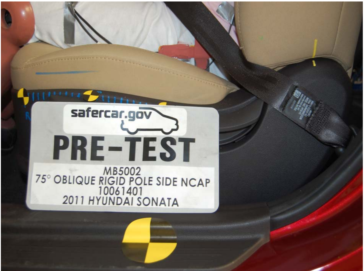
Pre-Test Close-Up Left Side View of Driver Seat Back Showing Test Position
