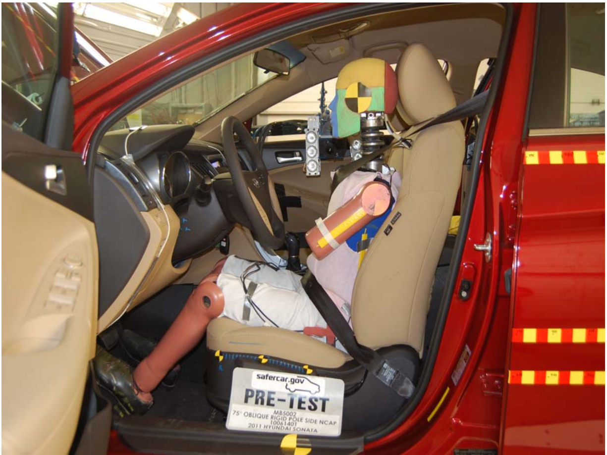
Pre-Test Left Side View of Dummy Showing Belts, Chalking, and Contact Switches (Door Open)
