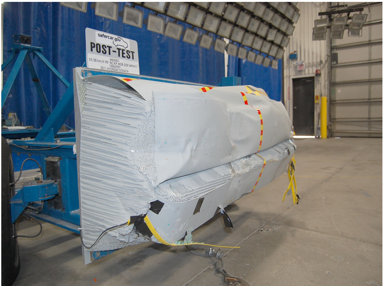
Post-Test Left Side View of MDB Impactor Face
