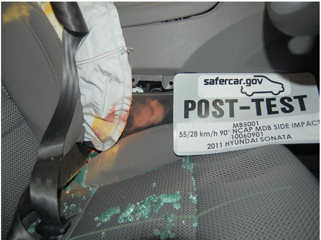
Post-Test Driver Dummy Pelvis Contact with Vehicle Interior View
