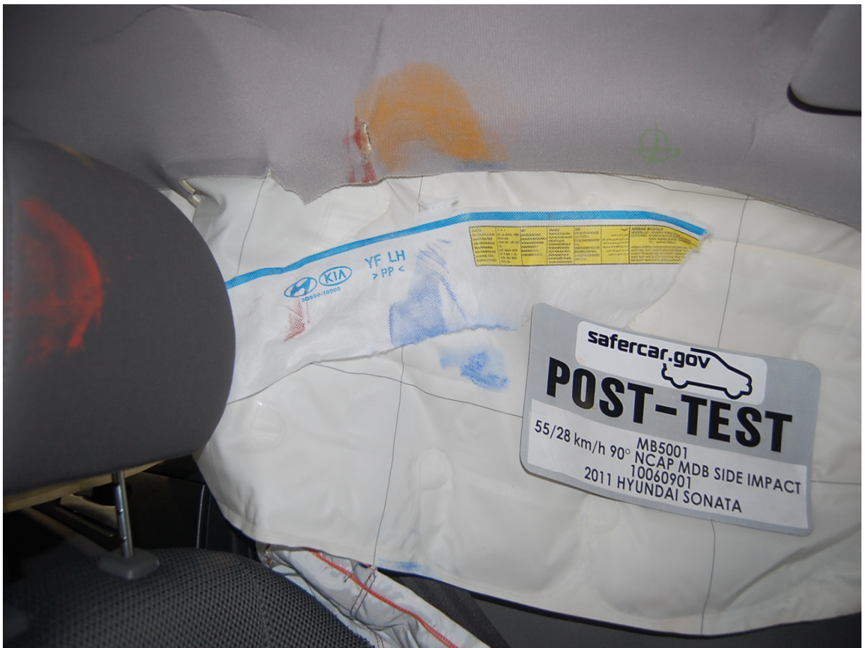
Post-Test Driver Dummy Head Contact with Vehicle View
