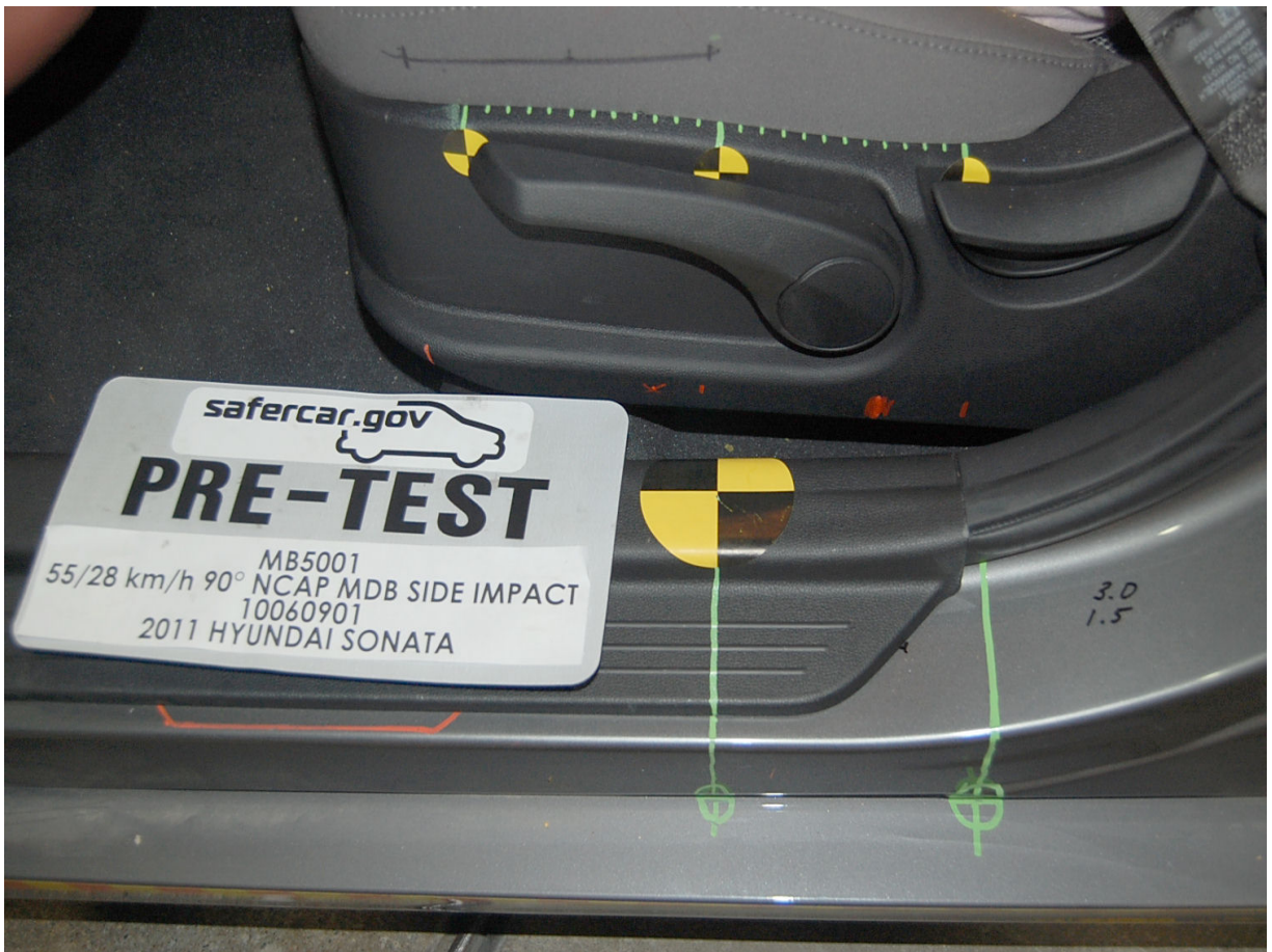
Pre-Test Close-Up Left Side View of Driver Seat Track Showing Seat Positioning
