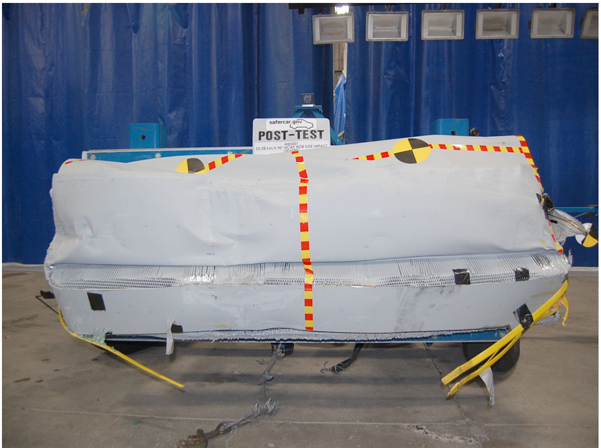
Post-Test Front View of MDB Impactor Face
