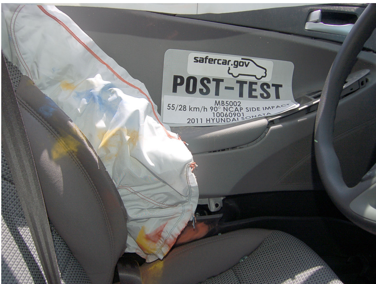
Post-Test Driver Dummy Torso Contact with Side Airbag View
