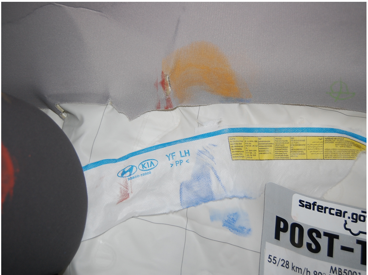
Post-Test Driver Dummy Head Contact with Side Airbag View
