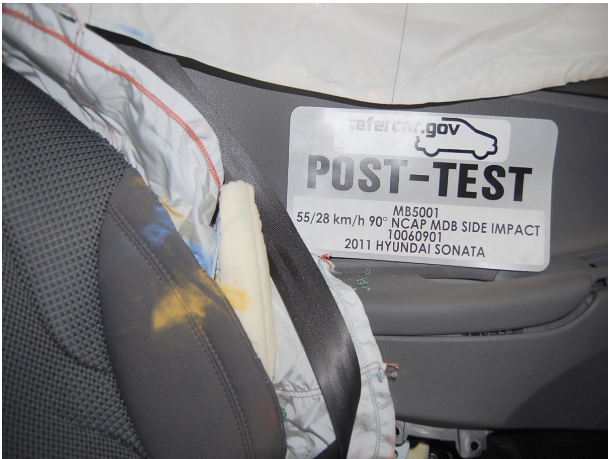
Post-Test Driver Dummy Torso Contact with Vehicle View
