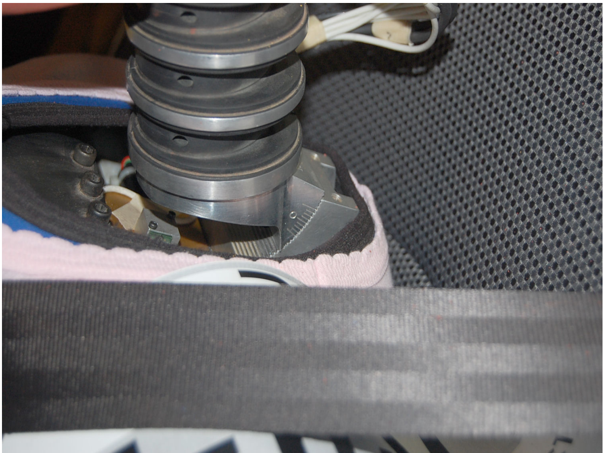
Pre-Test View of Passenger Dummy's Neck Showing Position of Adjustable Neck Bracket
