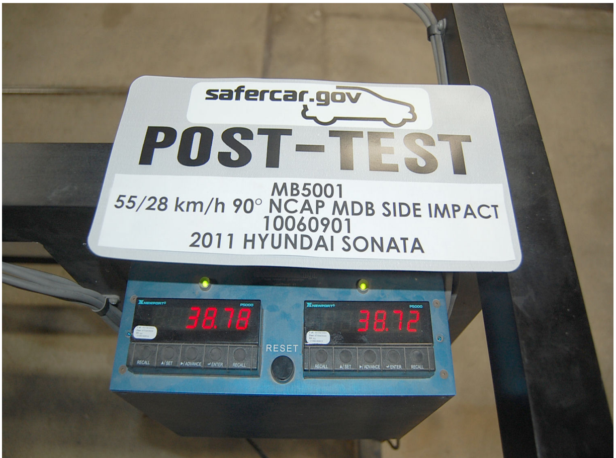
Post-Test Speed Trap Velocity Read-Out with Placard Showing NHTSA Number
