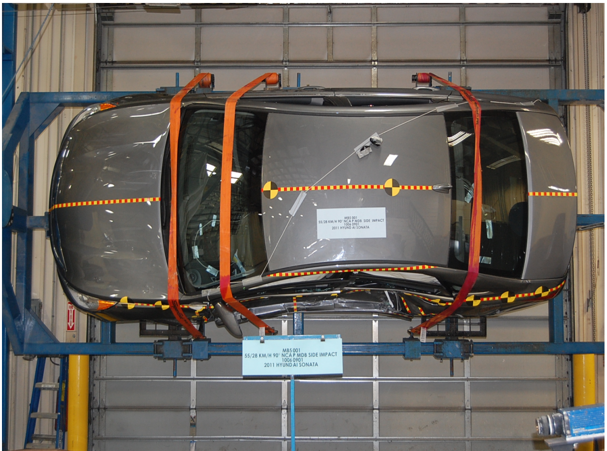
FMVSS No. 301/305 Rollover 90 Degrees
