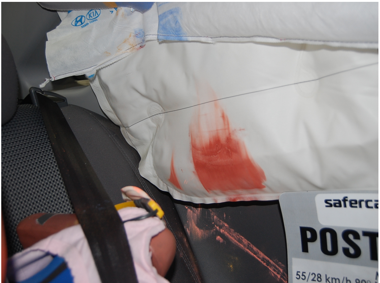
Post-Test Passenger Dummy Head Contact with Side Airbag View
