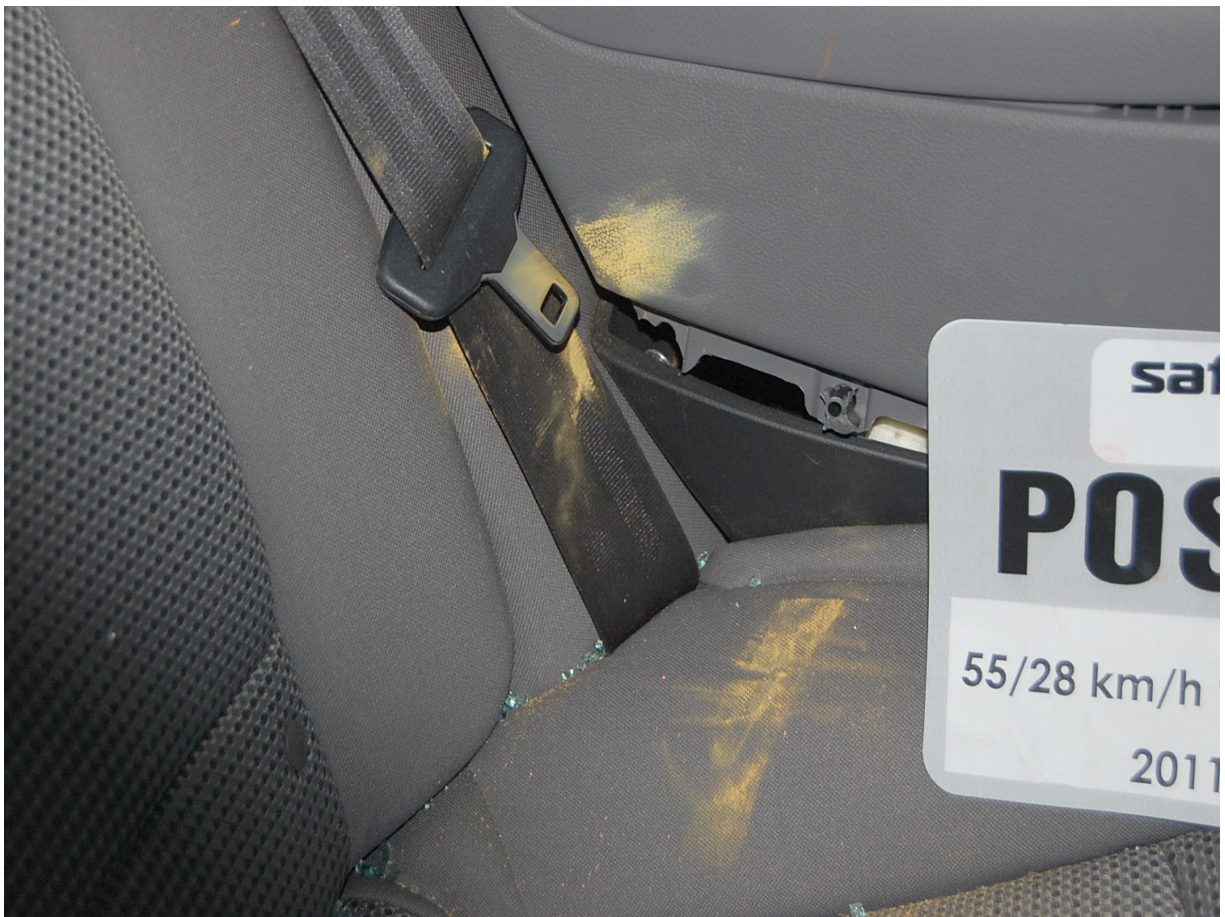
Post-Test Passenger Dummy Pelvis Contact with Vehicle Interior View
