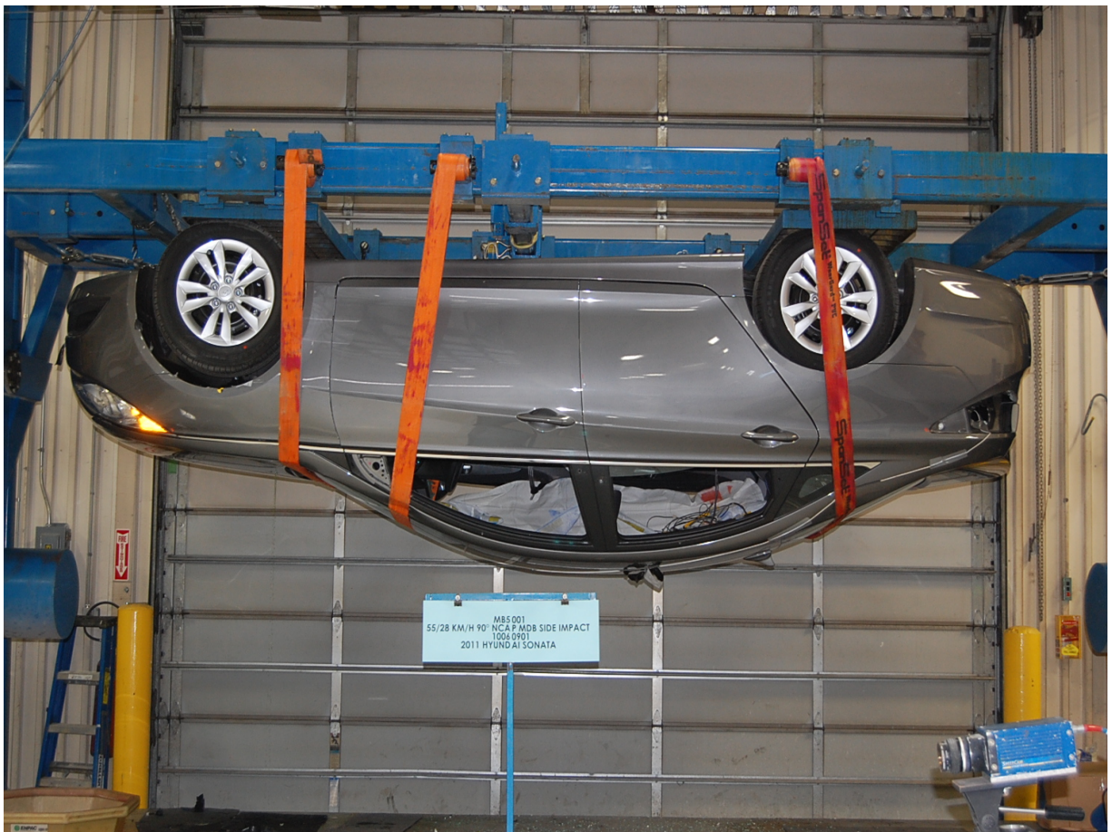
FMVSS No. 301/305 Rollover 180 Degrees
