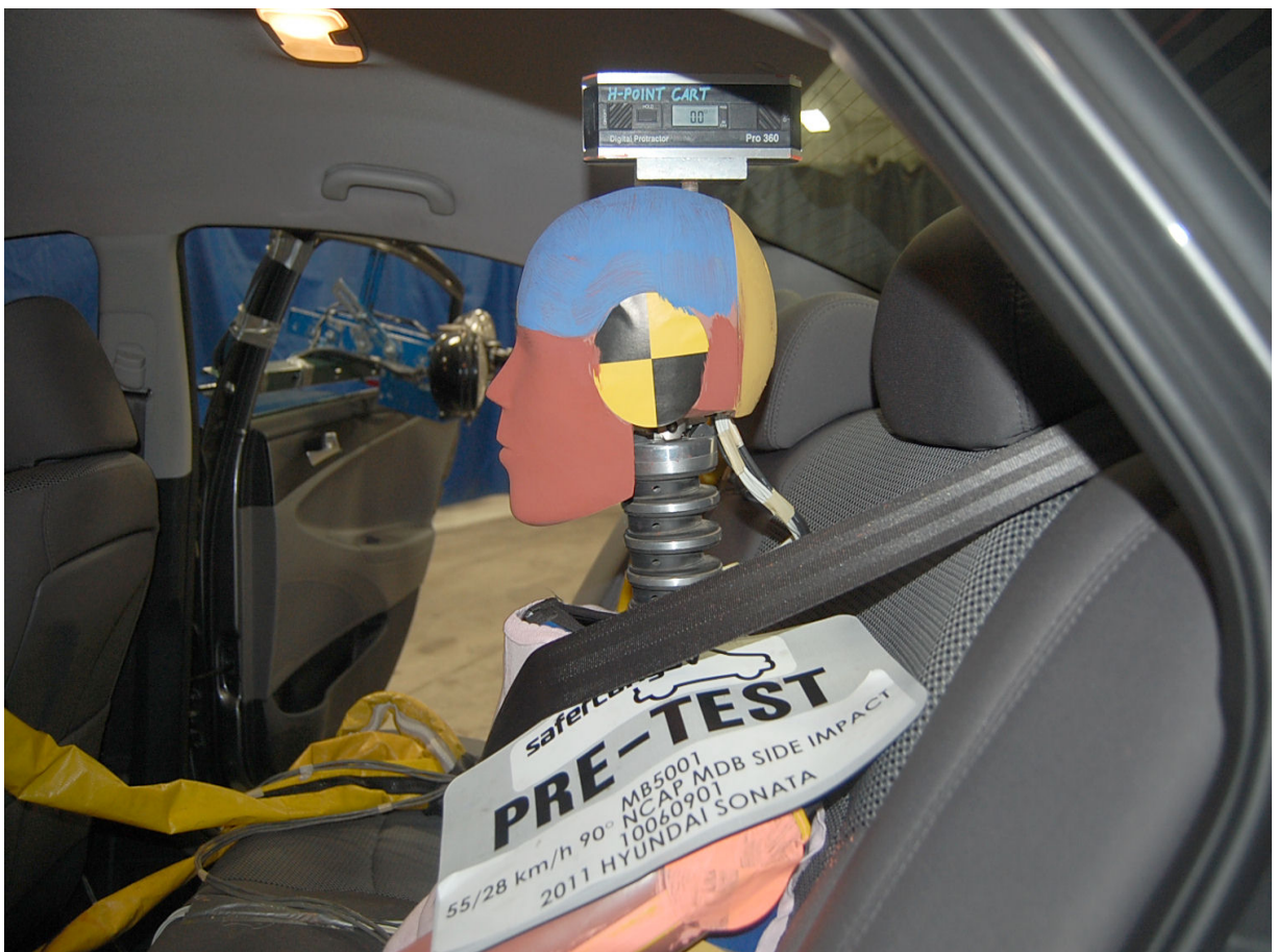
Pre-Test View of Passenger Dummy's Head Showing Dummy's Head is Level
