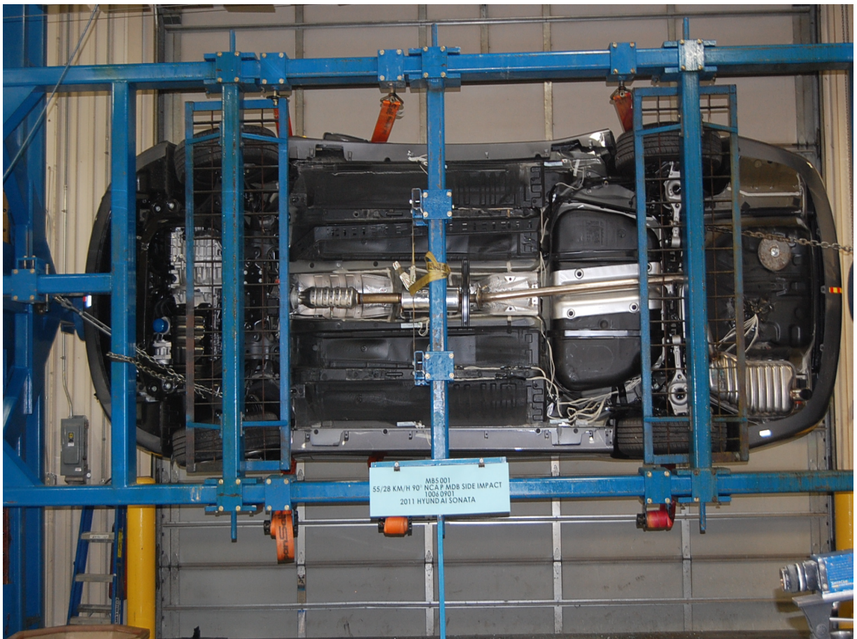
FMVSS No. 301/305 Rollover 270 Degrees
