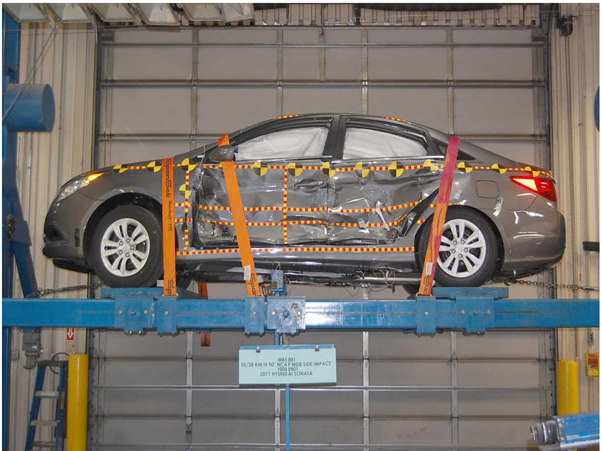
FMVSS No. 301/305 Rollover 0 Degrees
