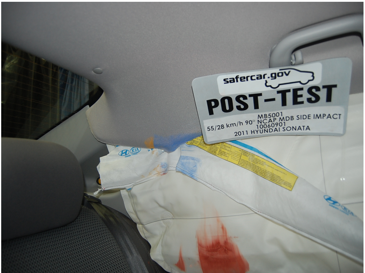
Post-Test Passenger Dummy Head Contact with Vehicle View
