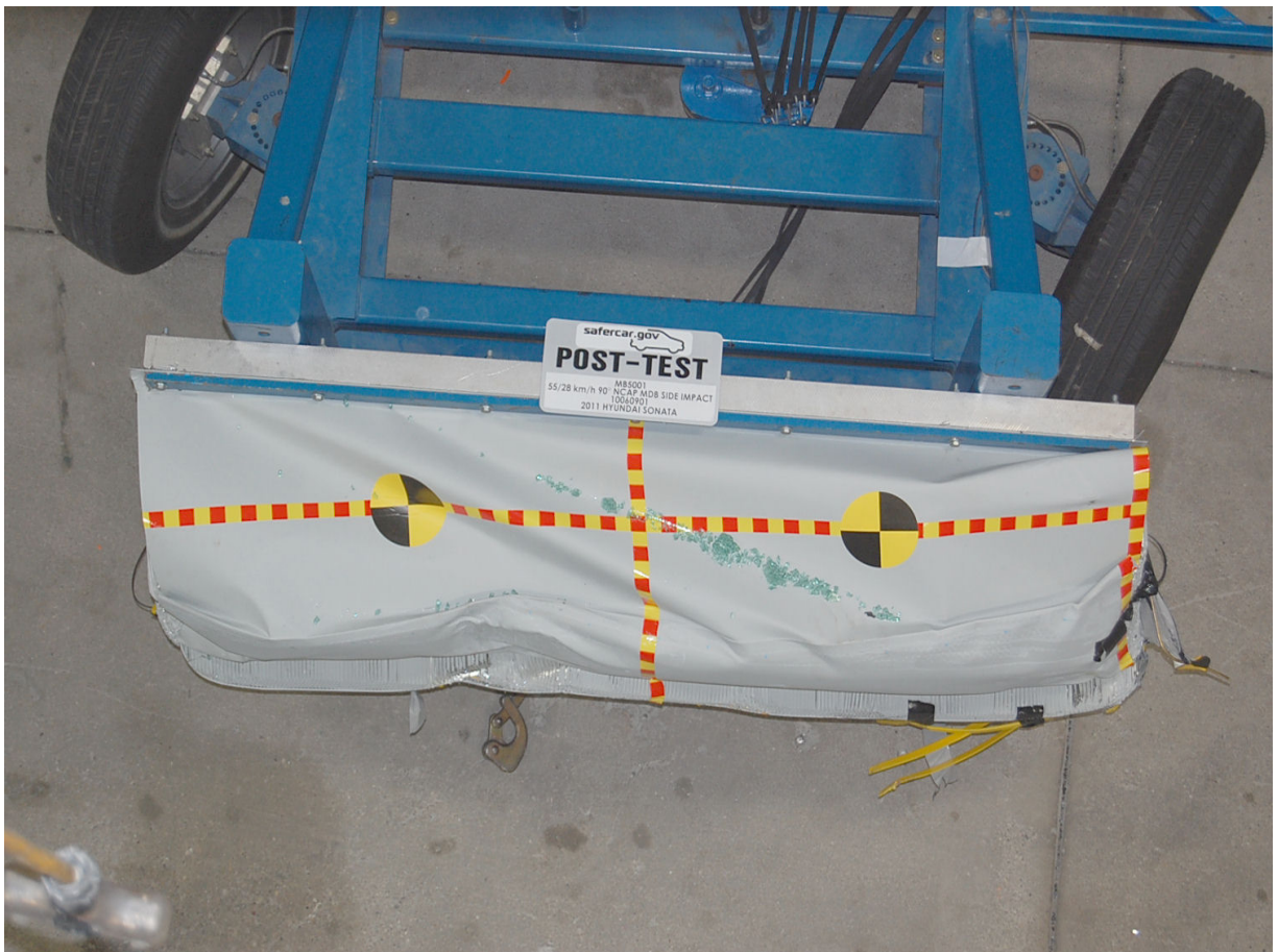
Post-Test Top View of MDB Impactor Face
