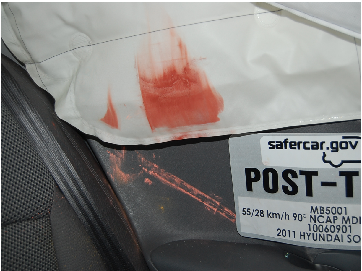
Post-Test Passenger Dummy Torso Contact with Vehicle View
