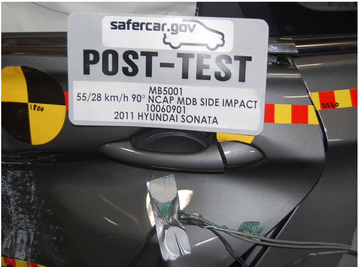
Post-Test Left Rear Door Latch Close-Up
