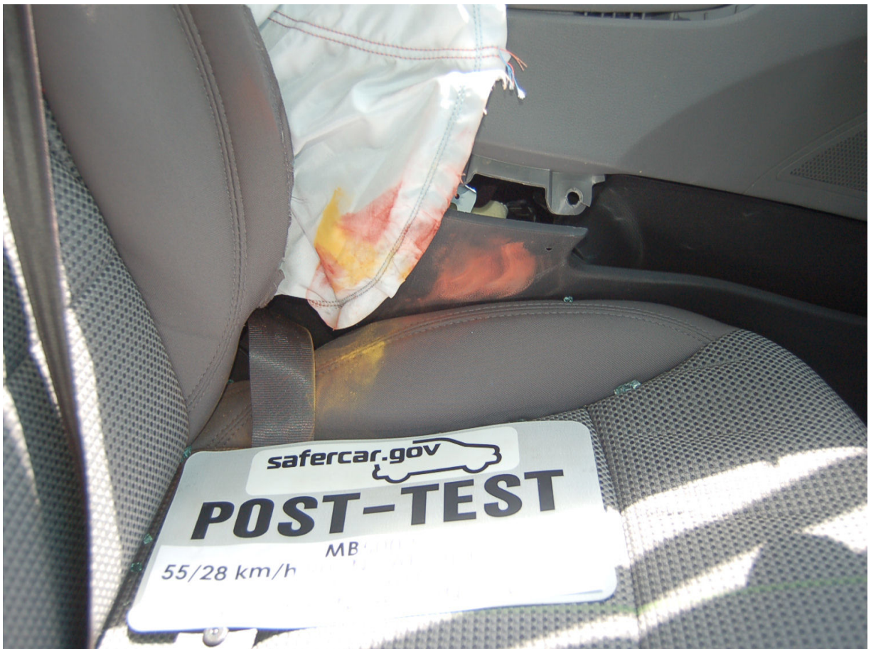
Post-Test Driver Dummy Pelvis Contact with Side Airbag View
