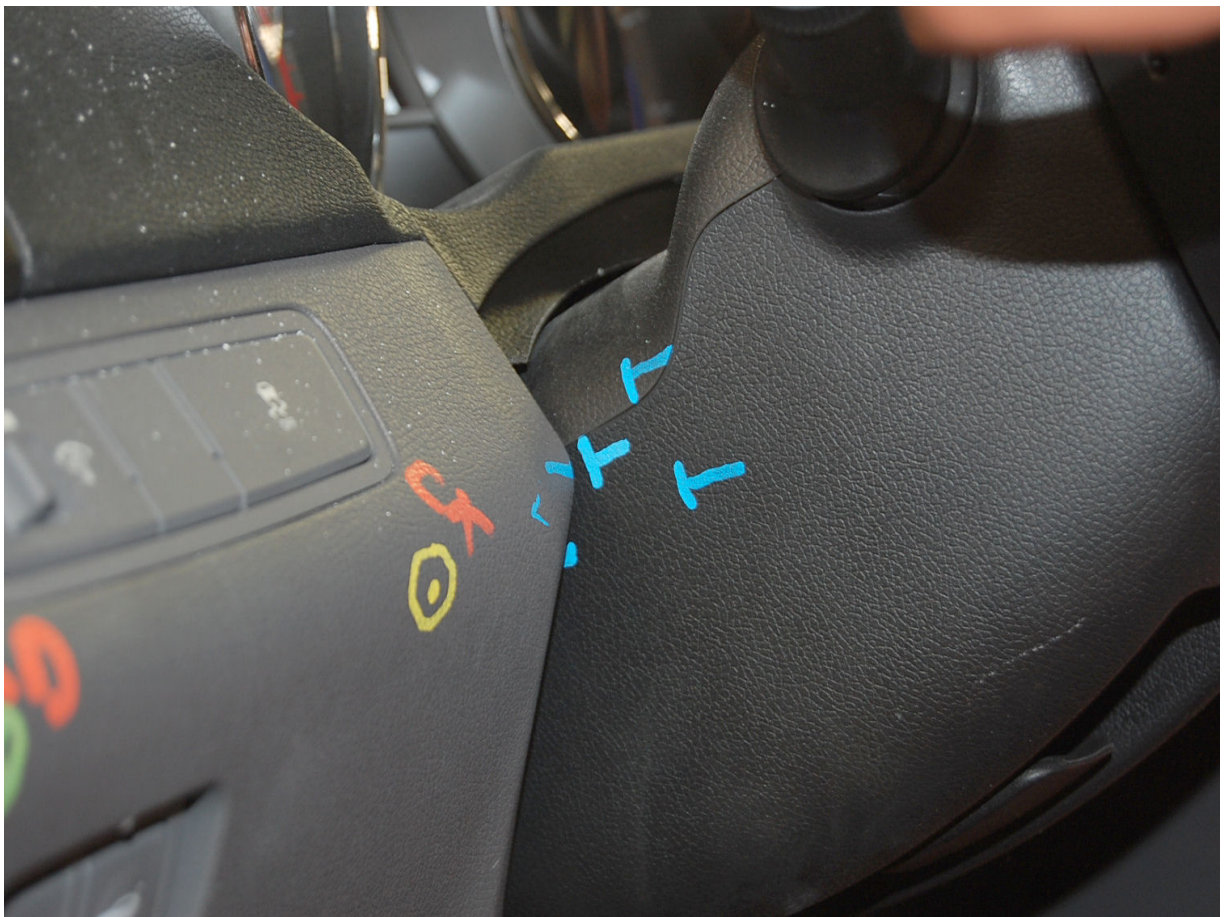
Pre-Test View of Steering Column Shear Capsule
