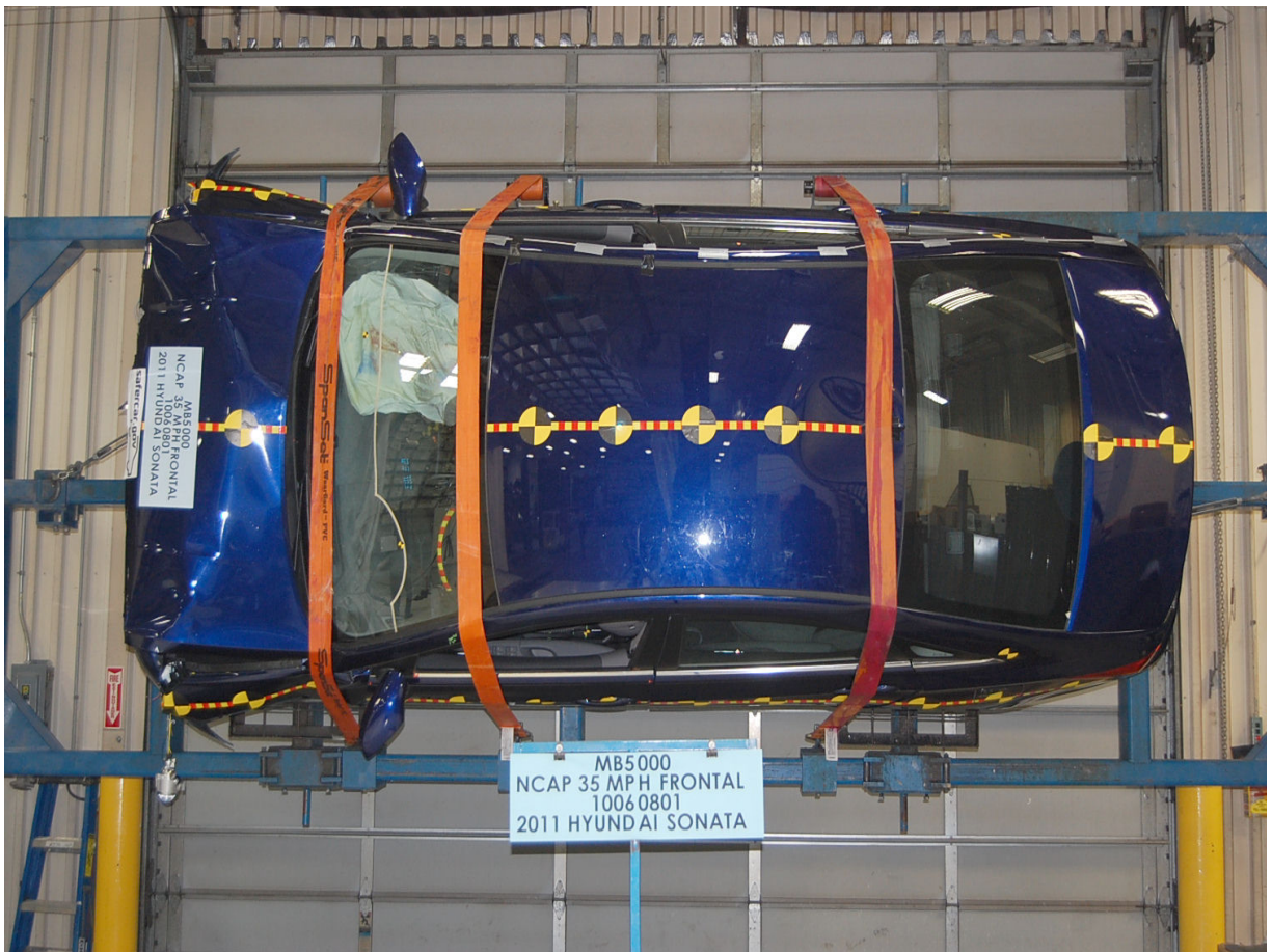
Vehicle at 90 Degrees on Static Rollover Device
