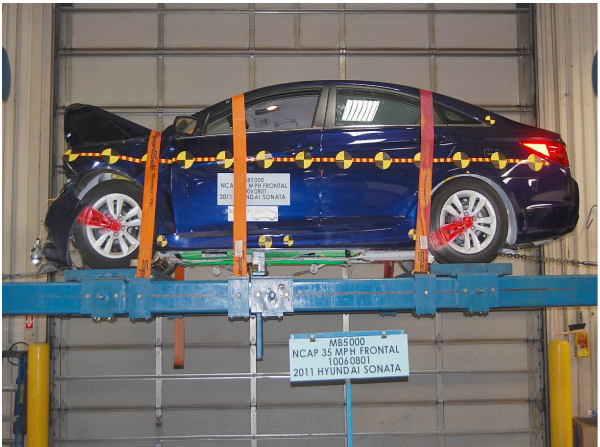
Vehicle at 0 Degrees on Static Rollover Device
