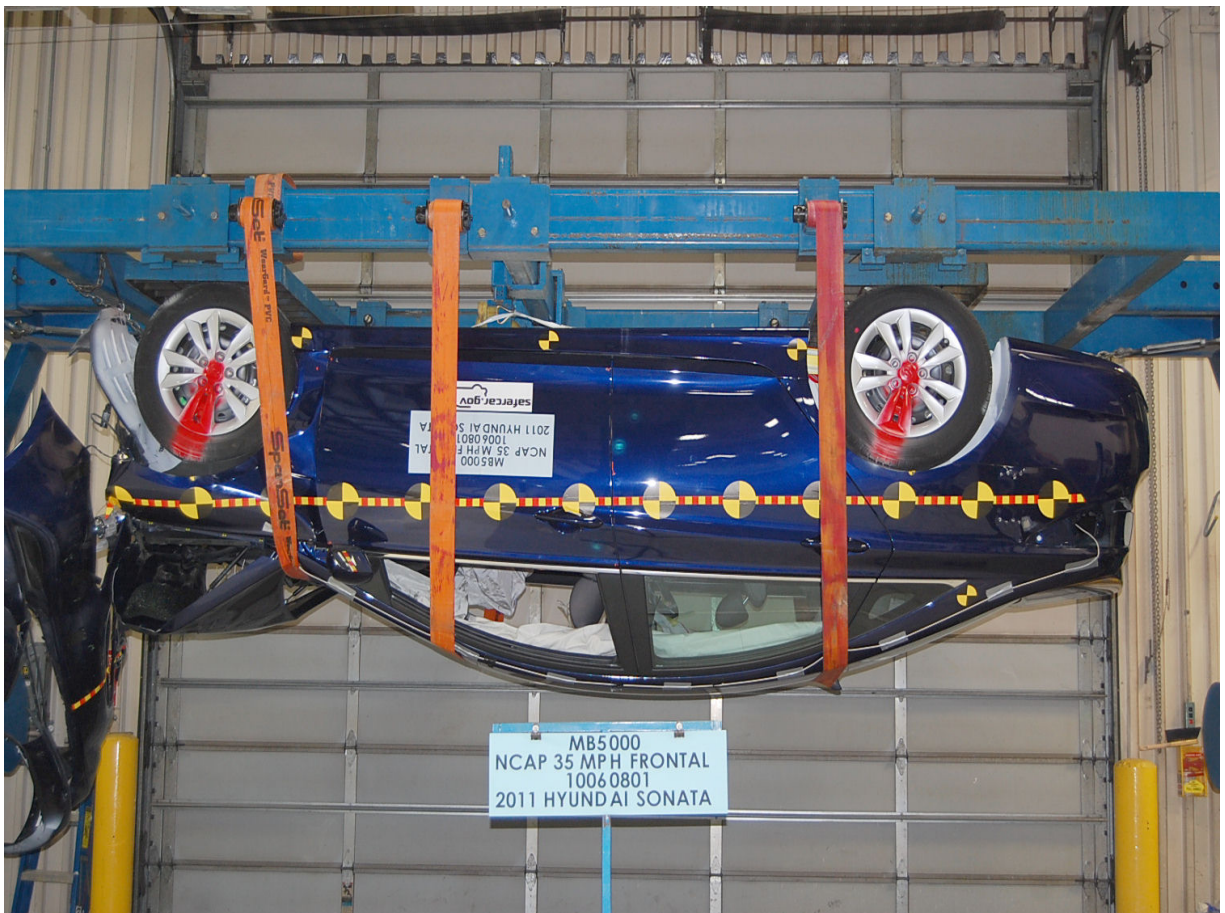
Vehicle at 180 Degrees on Static Rollover Device
