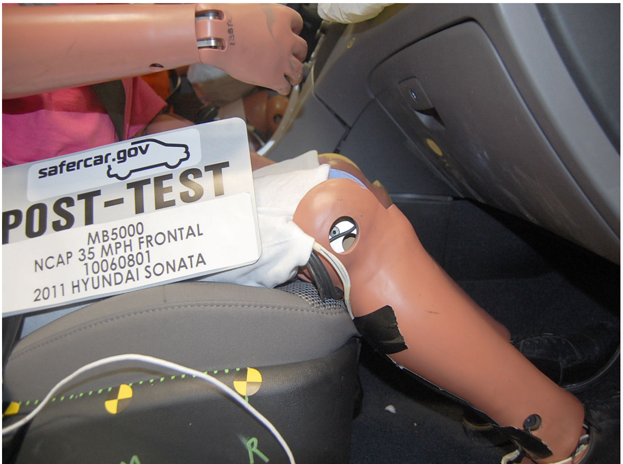
Post-Test Passenger's Side Knee Bolster
