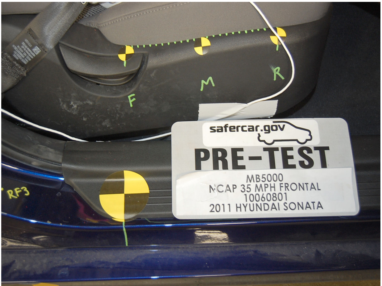
Pre-Test Passenger's Seat Fore-Aft Markings
