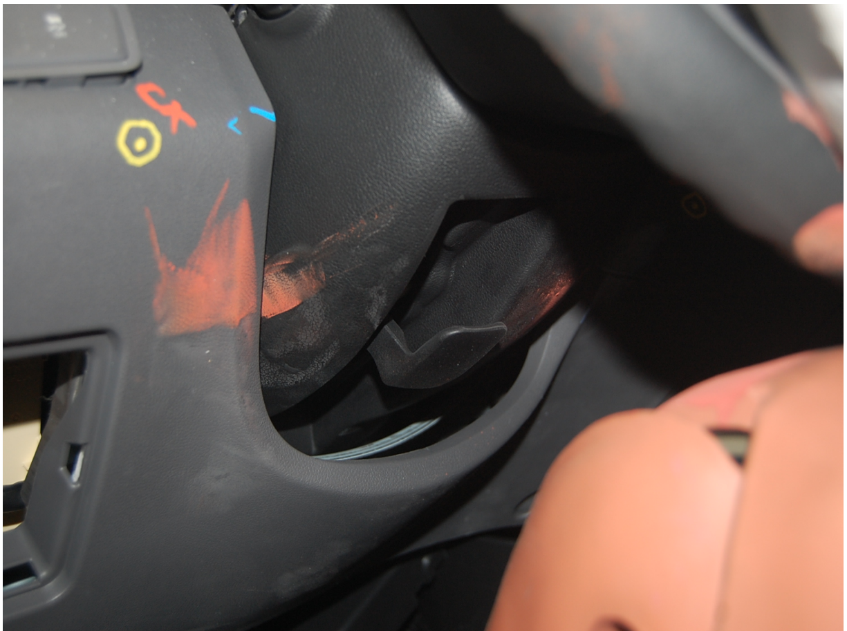
Post-Test View of Steering Column Shear Capsule
