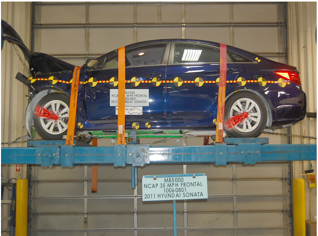
Vehicle at 360 Degrees on Static Rollover Device
