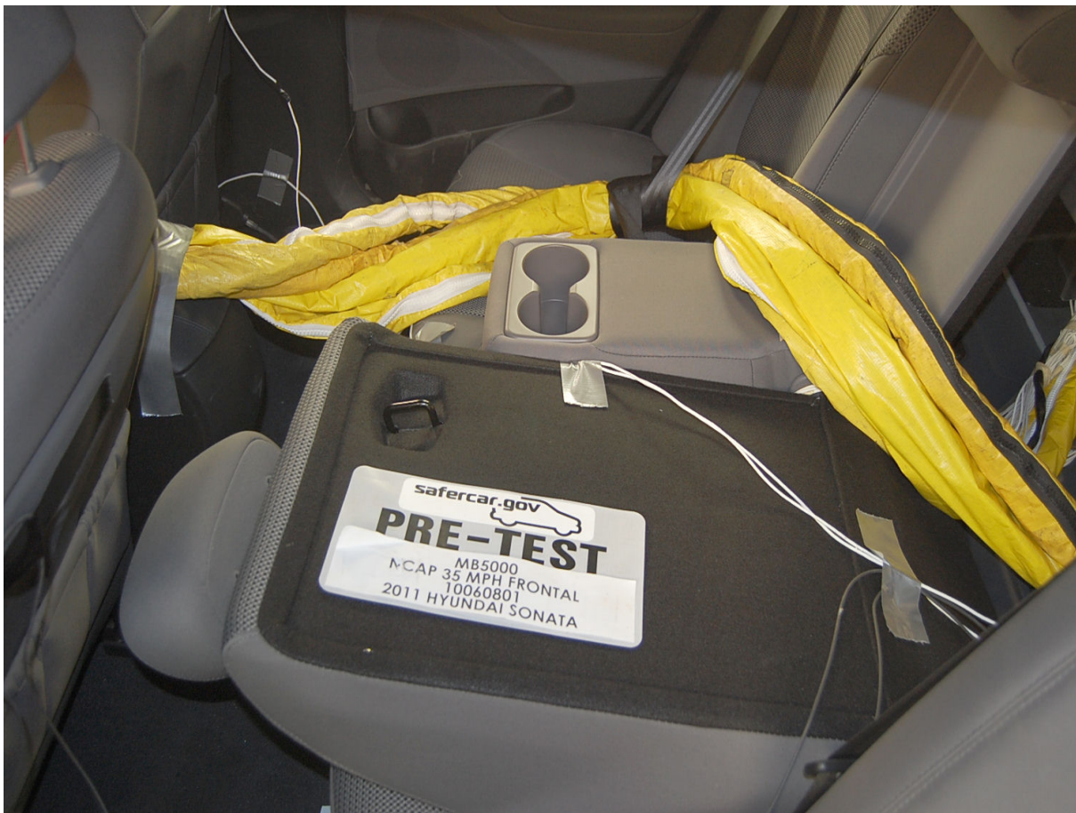
Pre-Test Dummy Cable Routing
