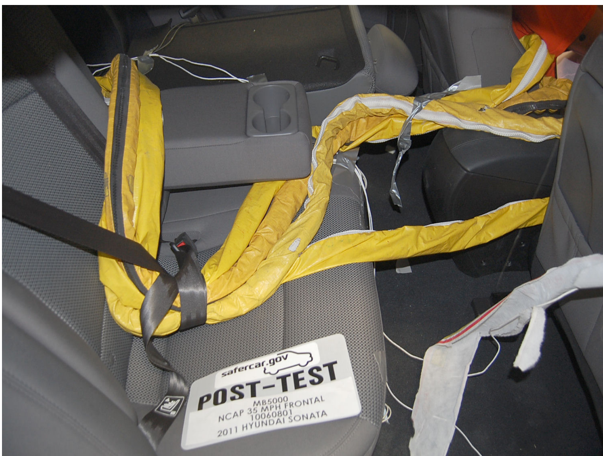
Post-Test Dummy Cable Routing
