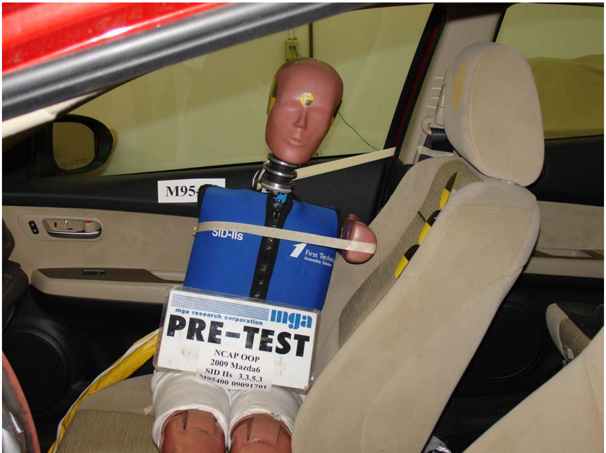
Pre-Test SID-IIs Dummy Left Side Closeup View
