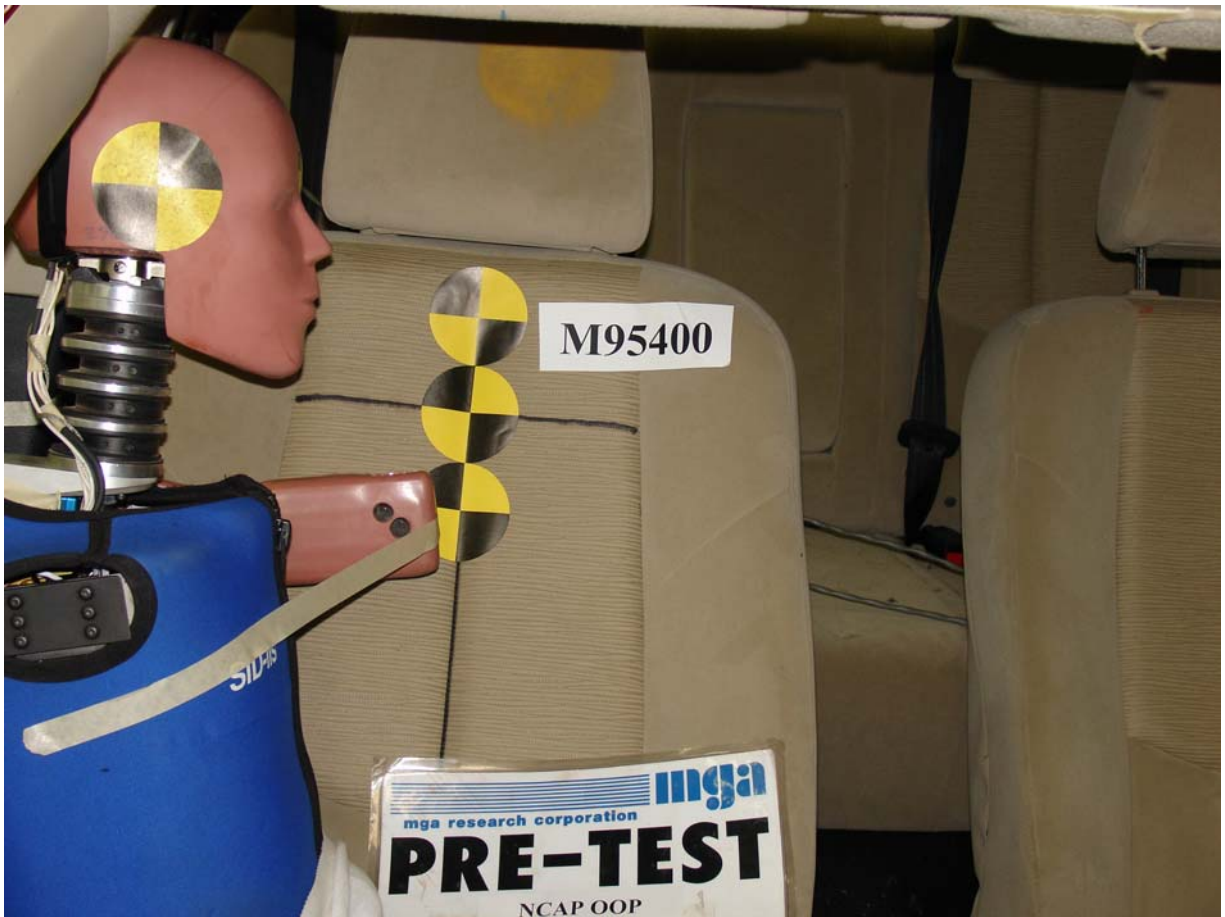
Pre-Test SID-IIs Dummy Front Closeup View
