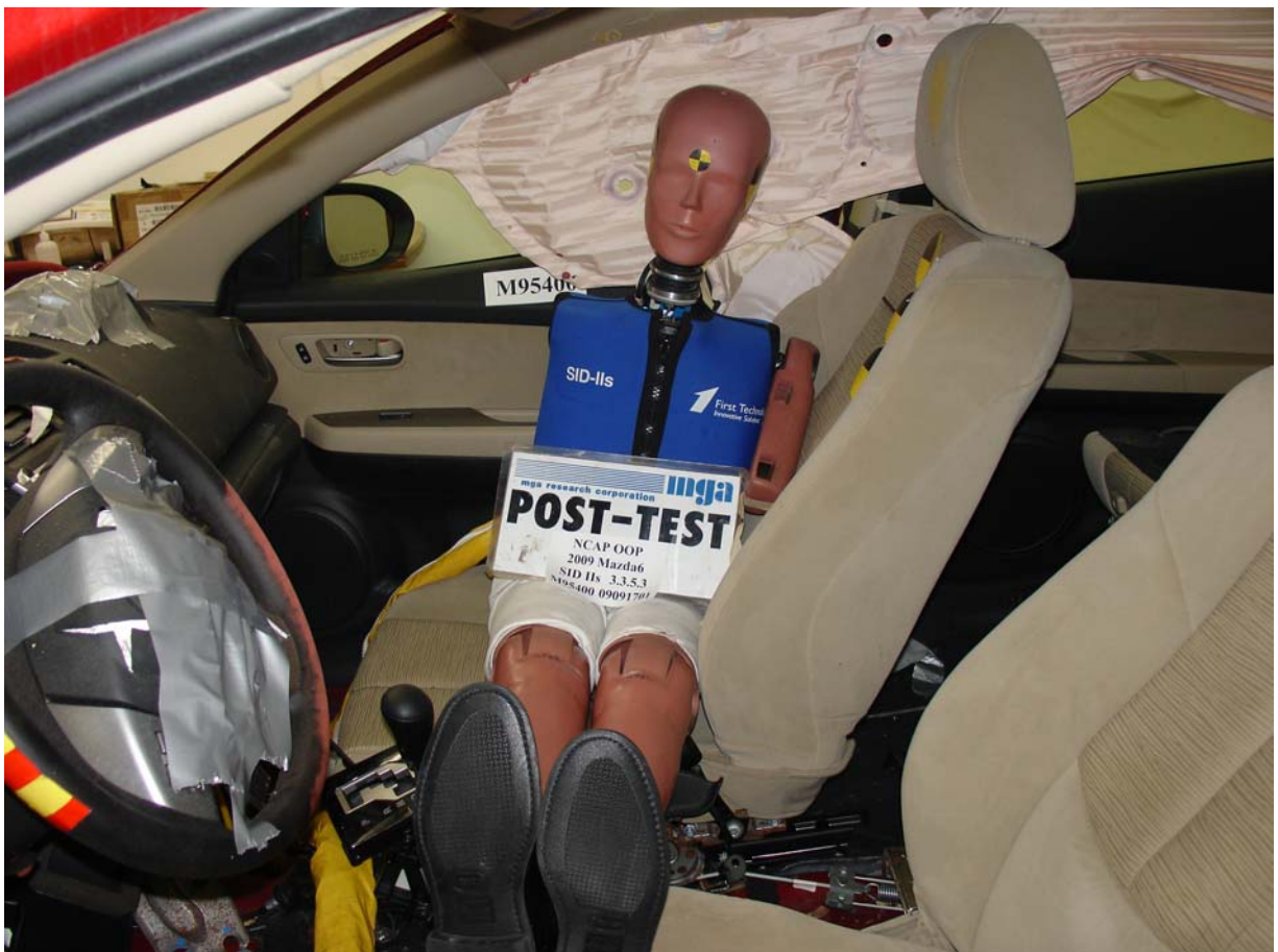
Post-Test SID-IIs Dummy Left Side View
