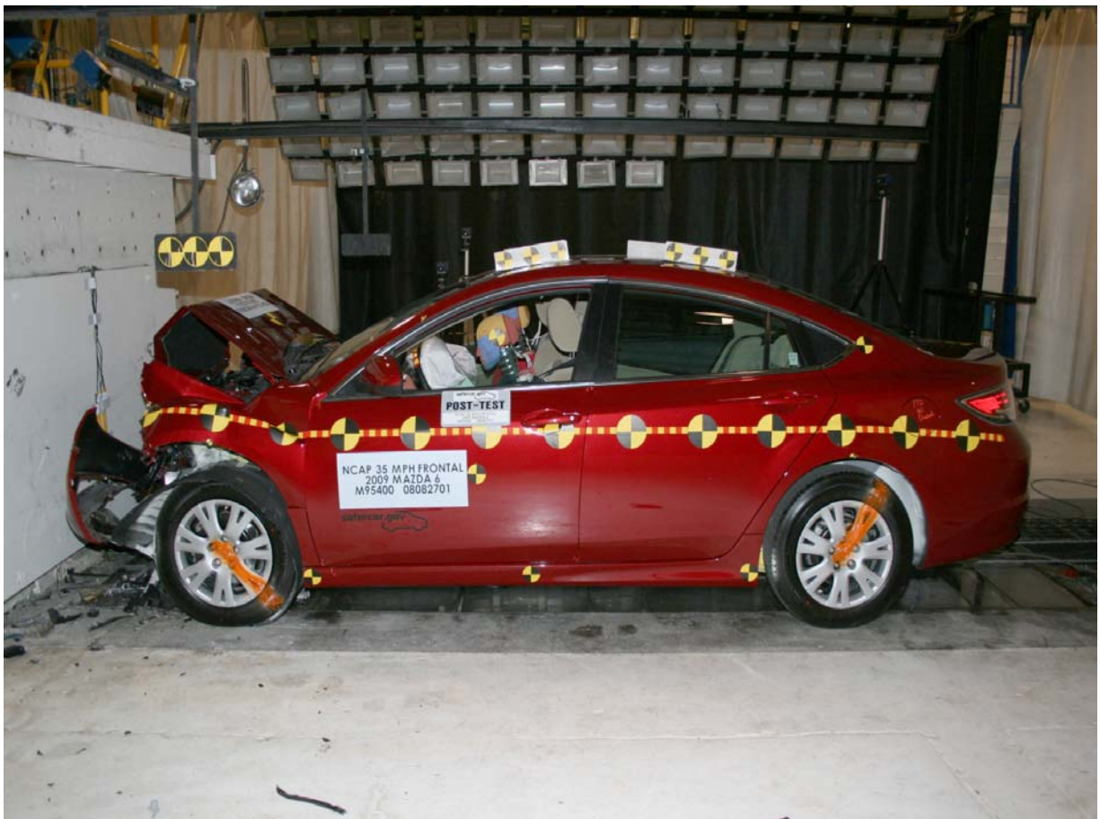
Post-Test Vehicle Left Side View
