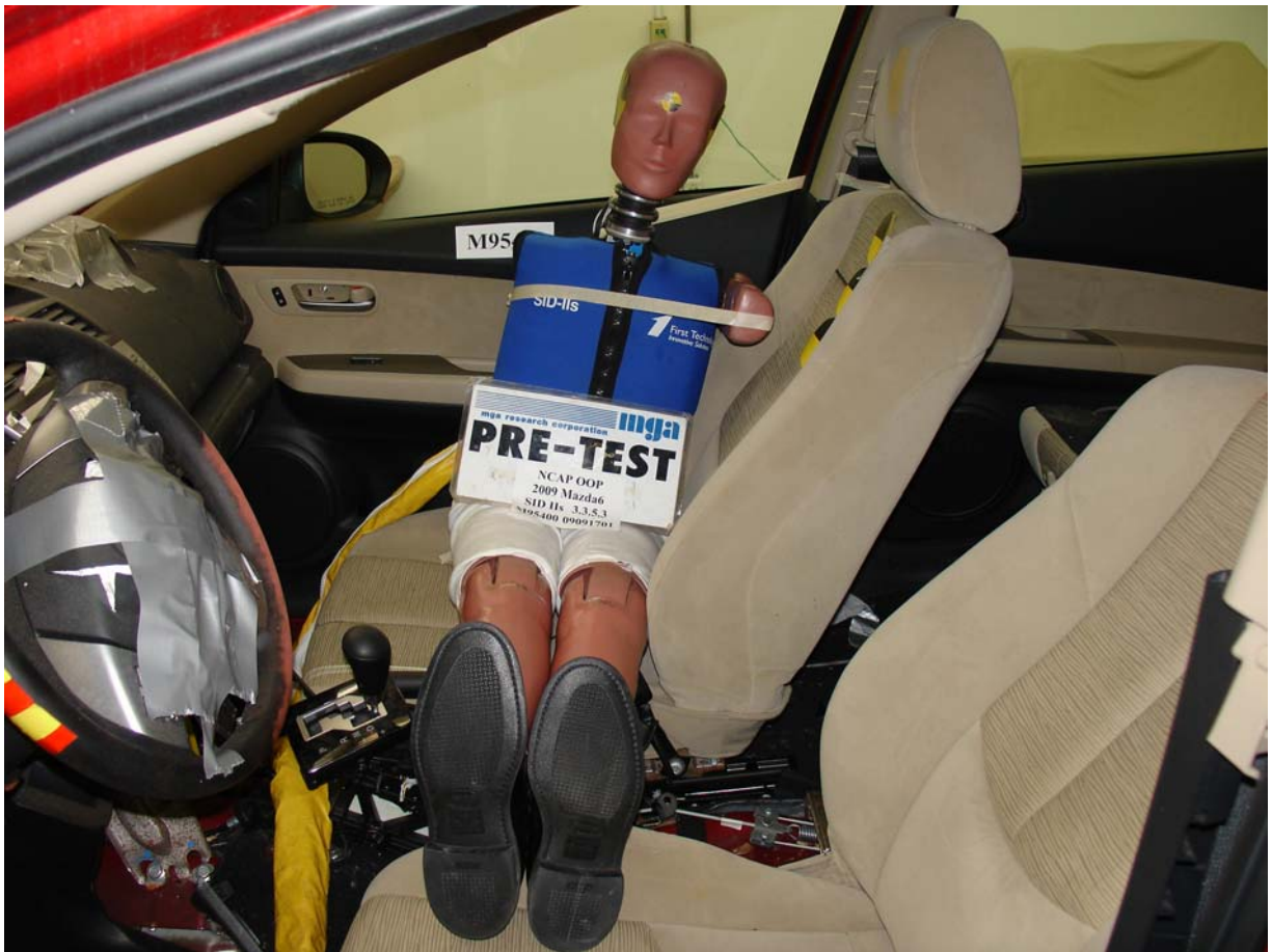
Pre-Test SID-IIs Dummy Left Side View
