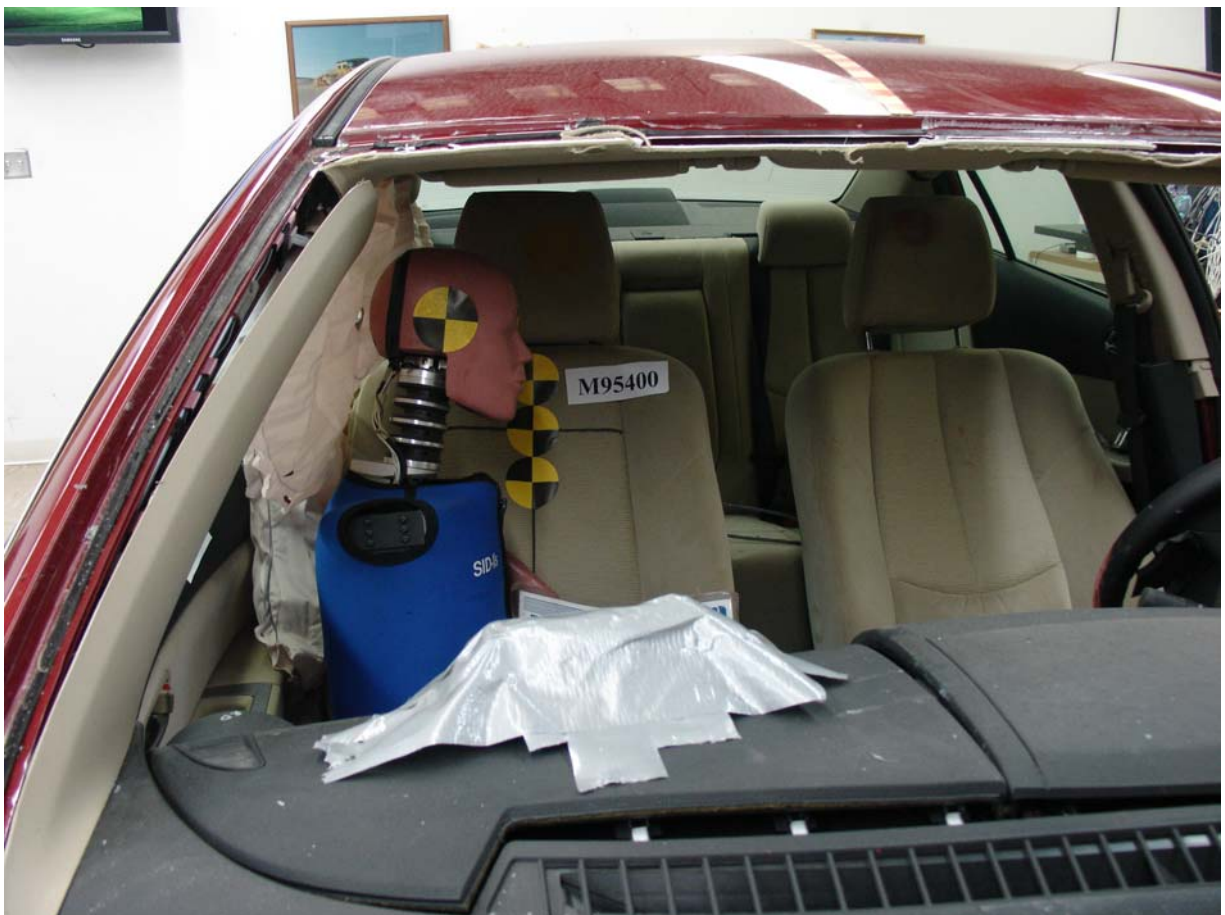
Post-Test SID-IIs Dummy Front View
