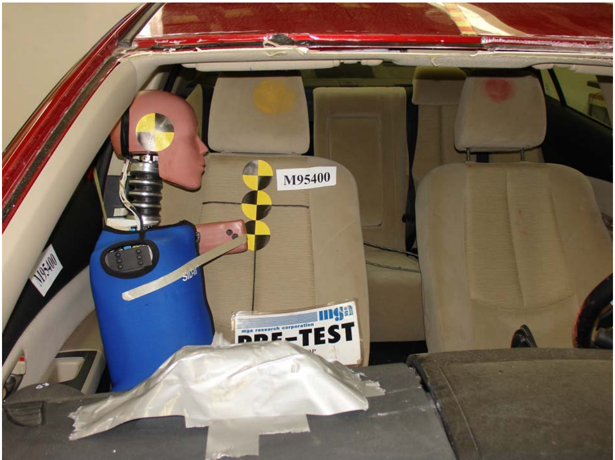
Pre-Test SID-IIs Dummy Front View
