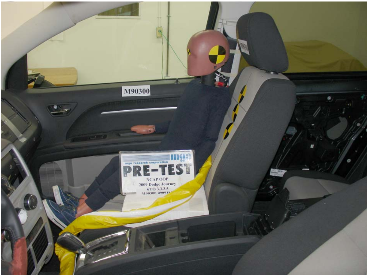
Pre-Test 6-Year-Old Child Dummy Left Side View
