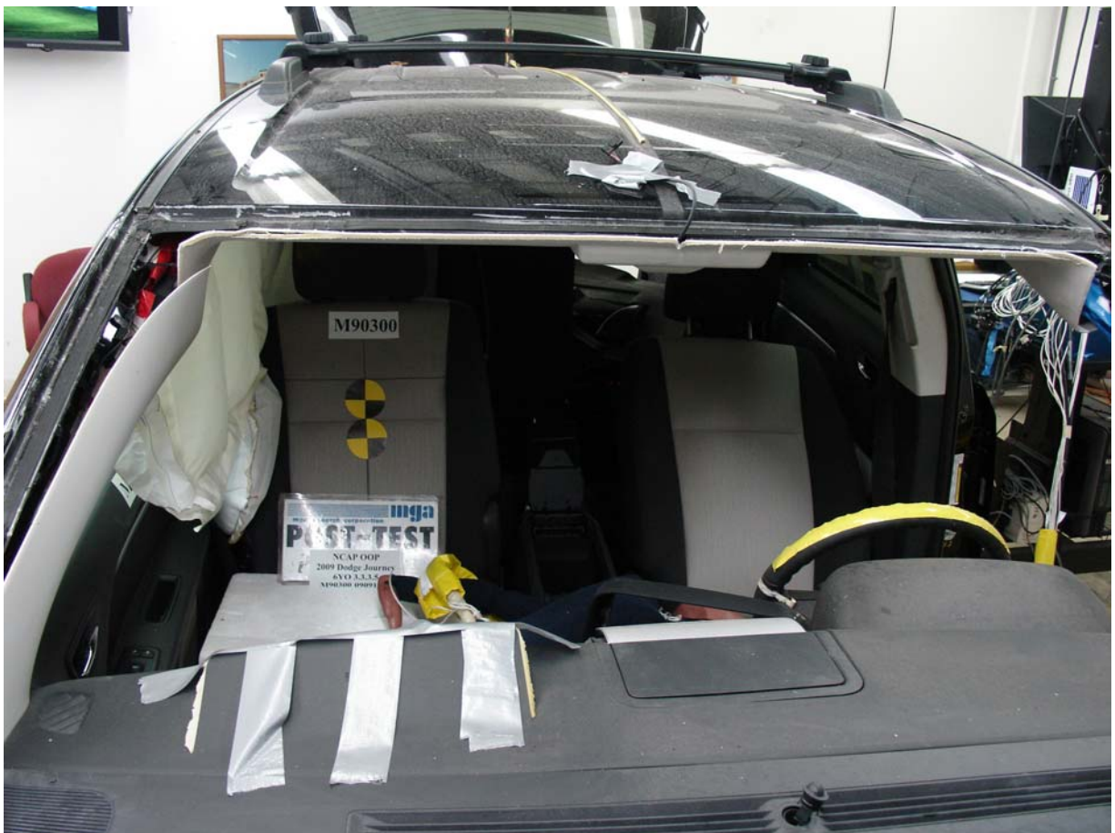
Post-Test 6-Year-Old Child Dummy Front View
