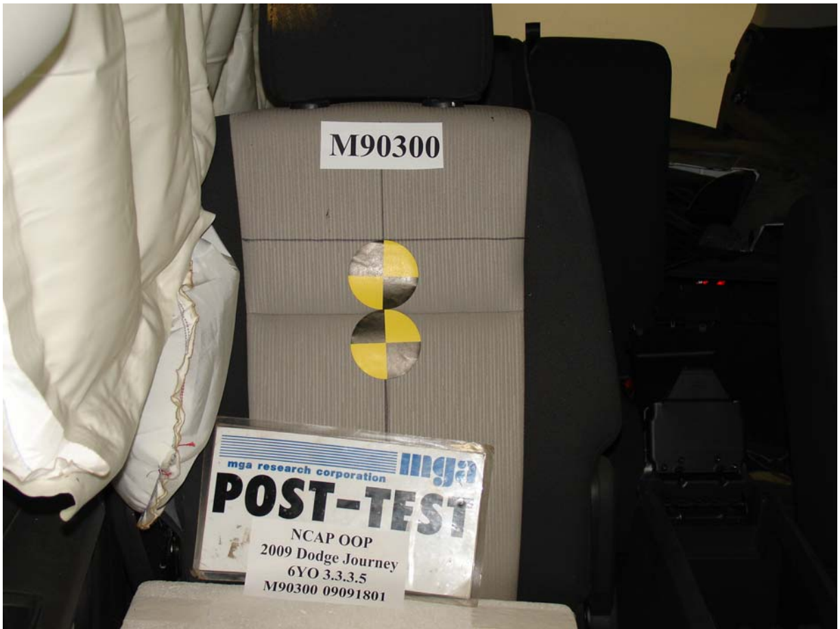
Post-Test Curtain and Torso Airbag Front View
