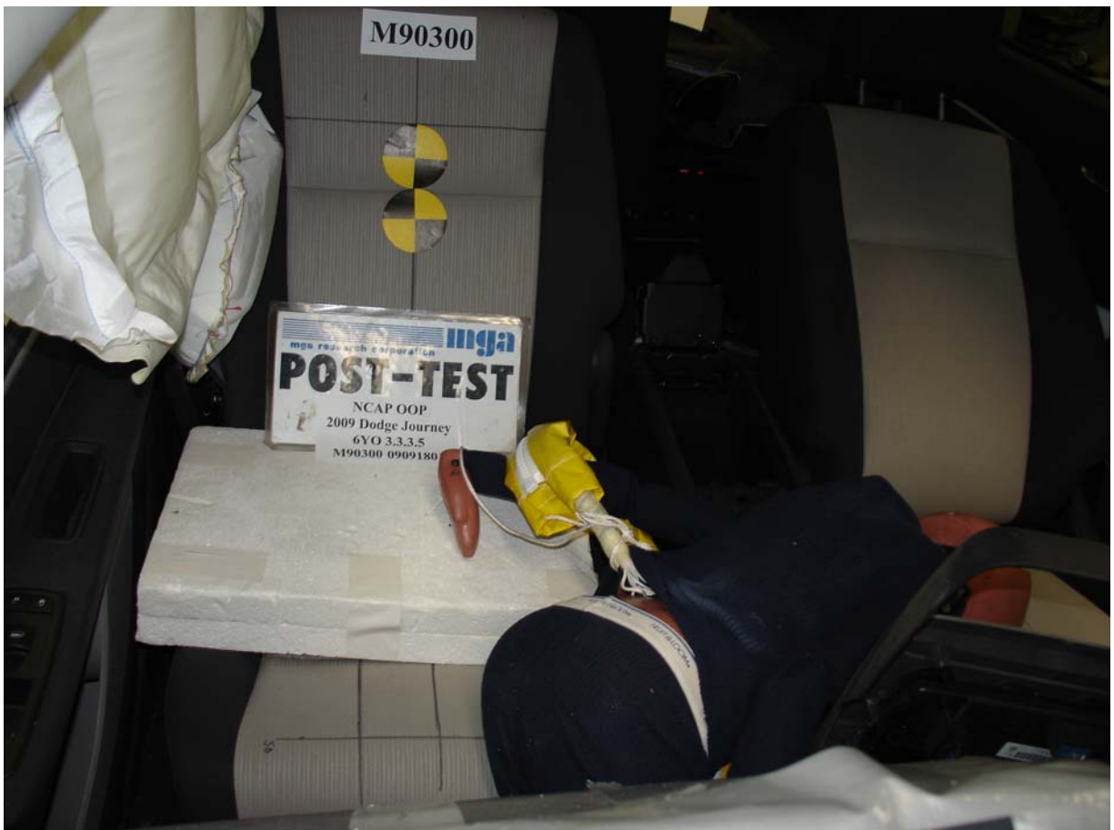
Post-Test 6-Year-Old Child Dummy Front Closeup View
