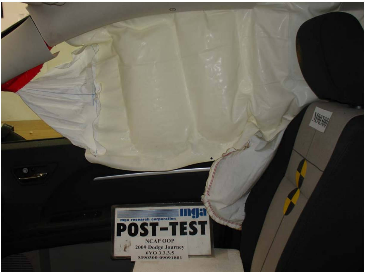
Post-Test Right Front Passenger Compartment View
