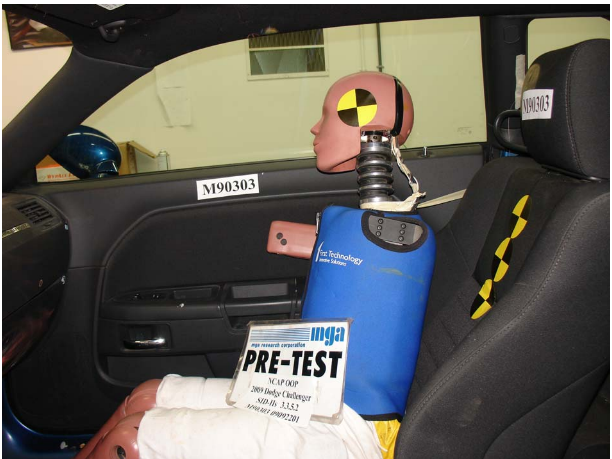
Pre-Test SID-IIs Dummy Left Side Closeup View
