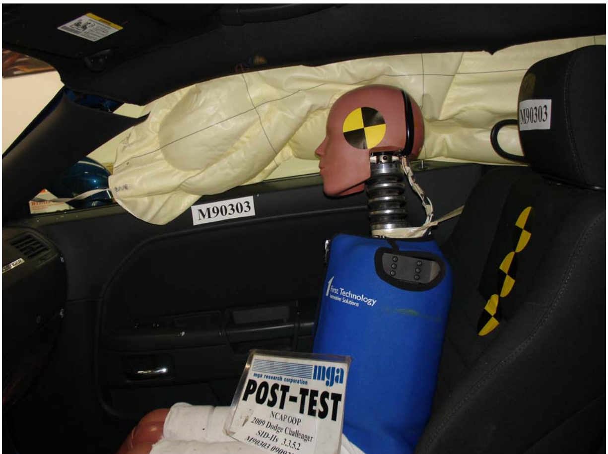
Post-Test SID-IIs Dummy Left Side Closeup View
