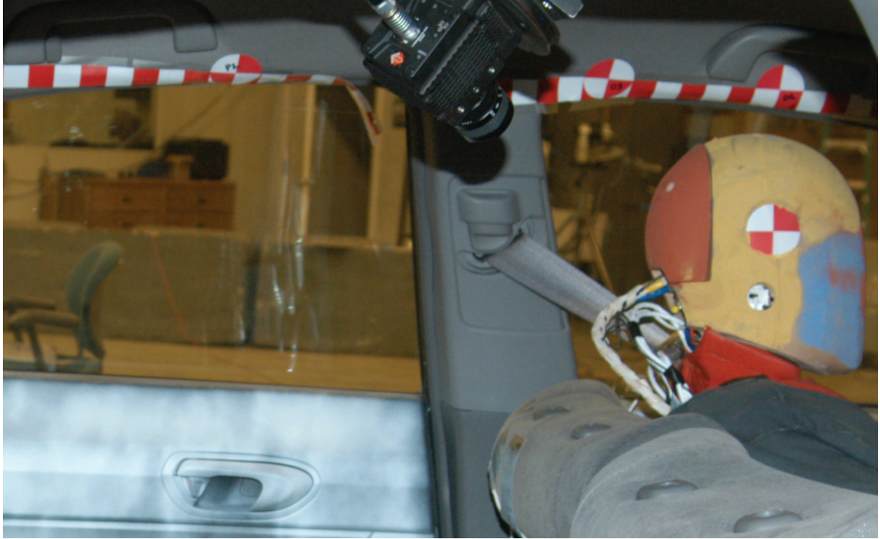
Figure A-49: Post test driver head contact (b-pillar)
