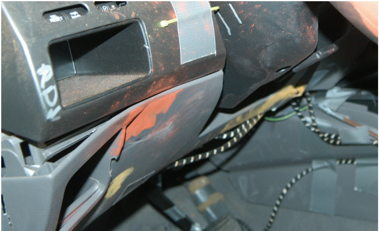
Figure A-46: Post test driver knee bolster
