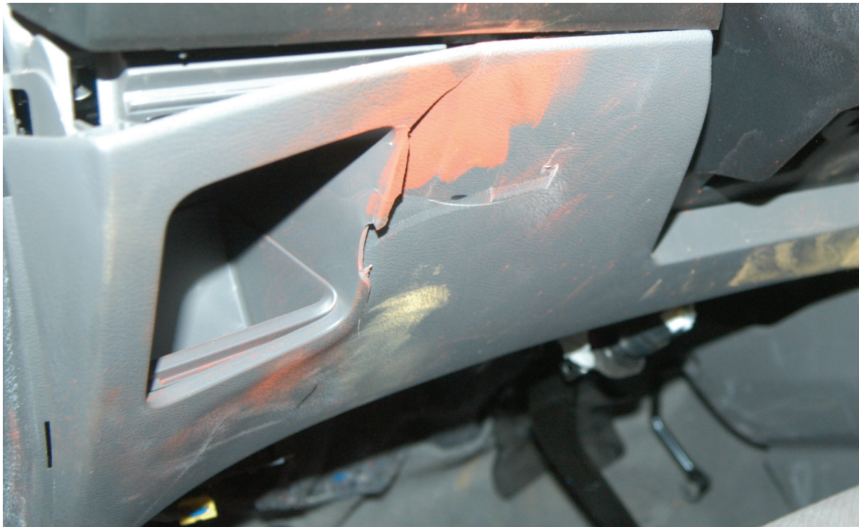
Figure A-50: Post test driver knee contact
