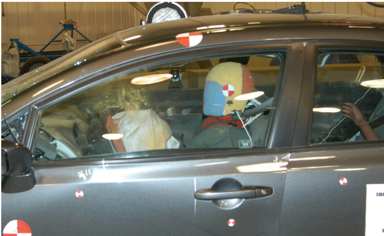
Figure A-36: Post test driver through window
