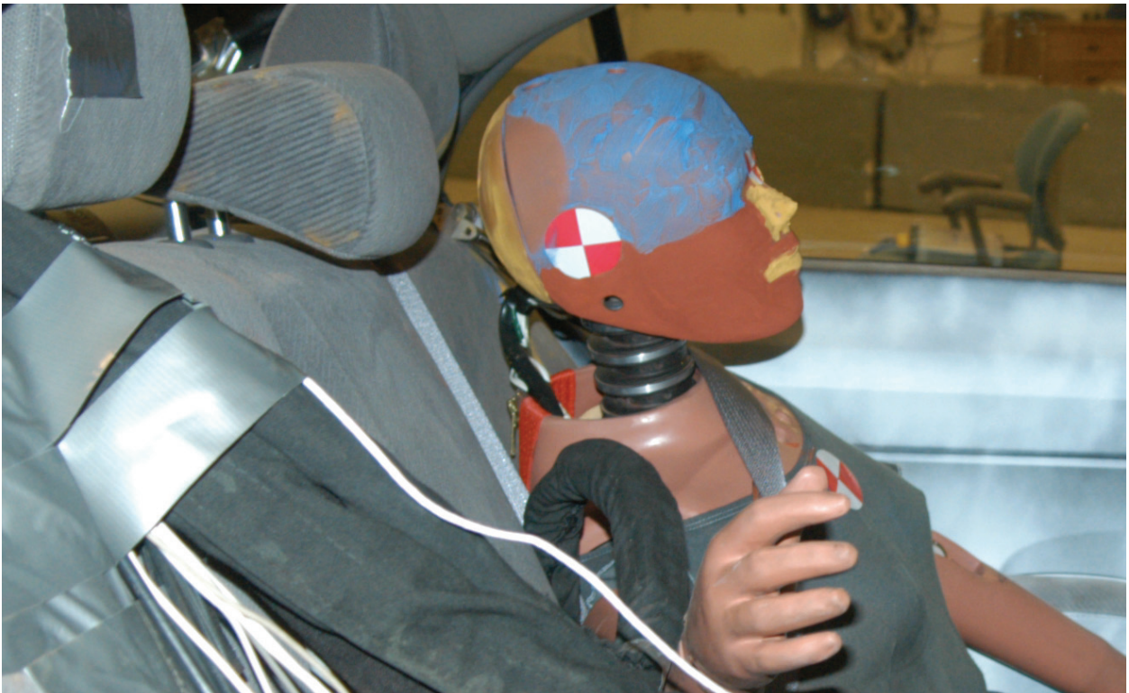
Figure A-62: Post test passenger head contact
