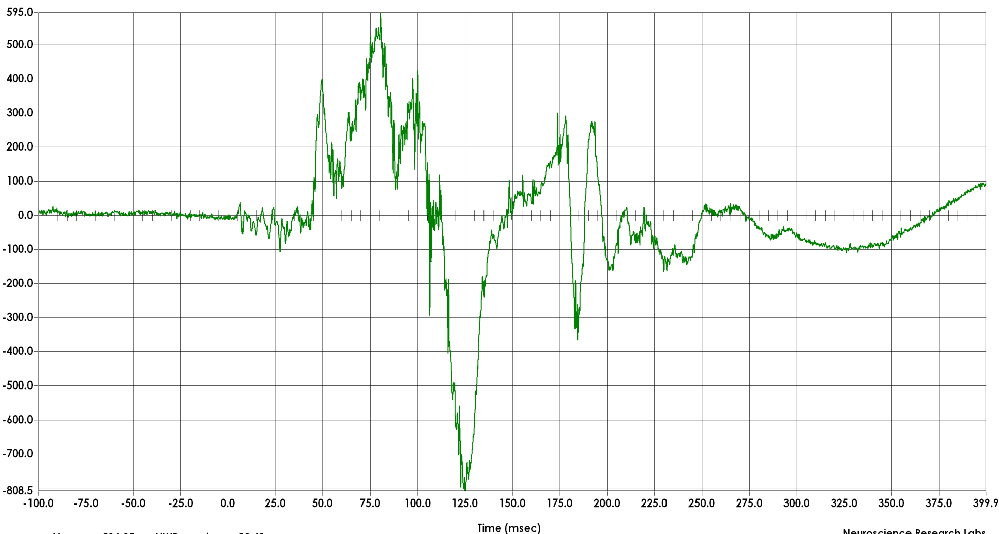
NWT Driver lower neck loadcell force ZL
