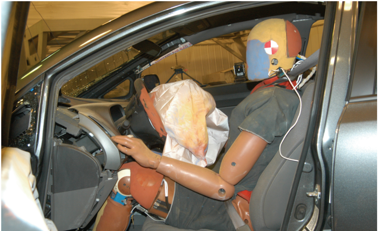
Figure A-38: Post test driver (door open)
