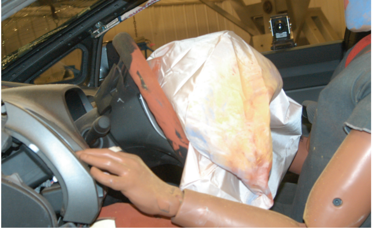
Figure A-51: Post test driver airbag contact
