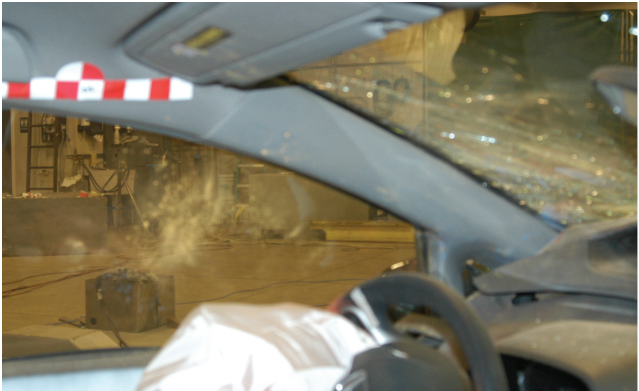
Figure A-48: Post test driver head contact
