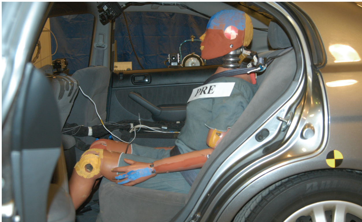
Figure A-56: Pre test passenger door open
