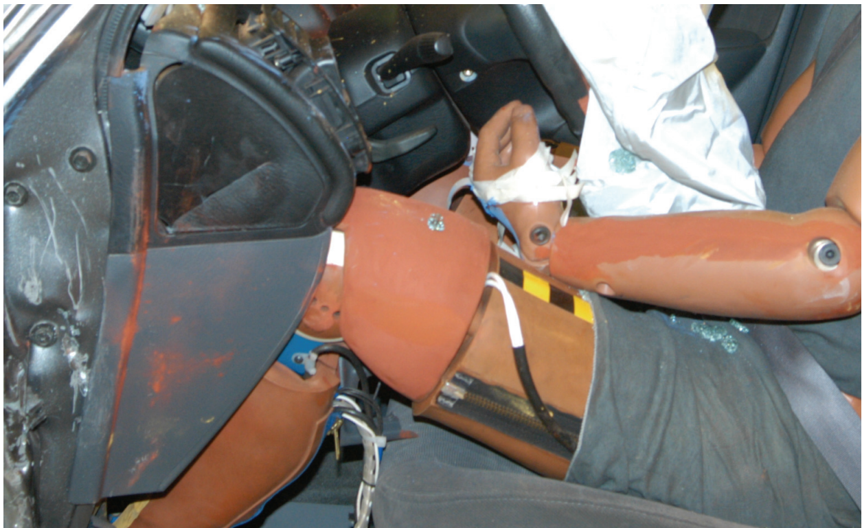
Figure A-44: Post test driver foot/leg close-up
