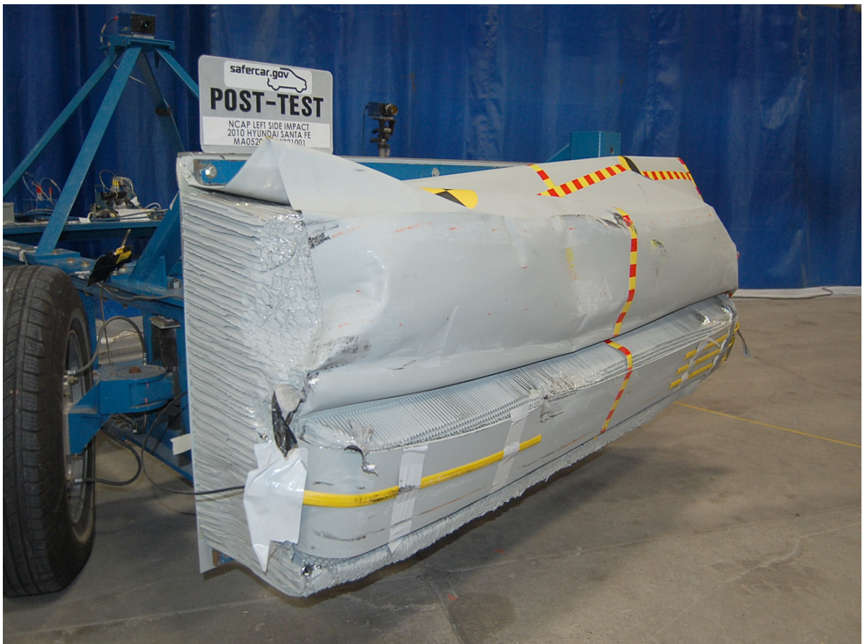
Post-Test Right Side View of Deformable Barrier
