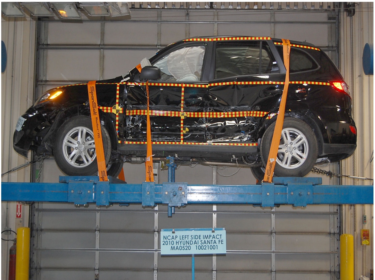
Vehicle on Rollover Device (360 Degrees)
