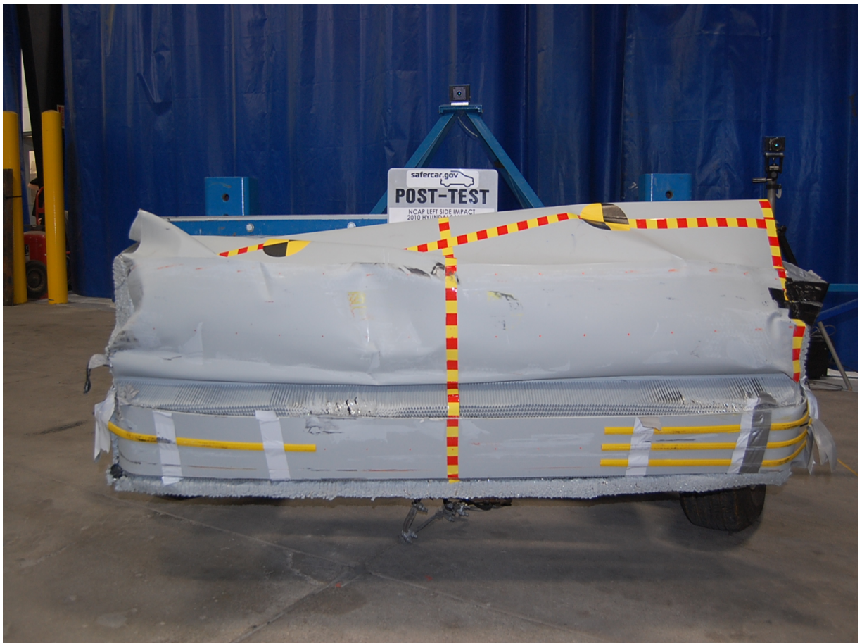
Post-Test Front View of Deformable Barrier
