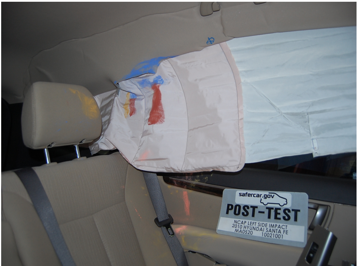
Post-Test Passenger Dummy Head Contact View
