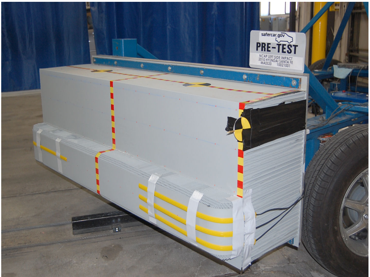
Pre-Test Left Side View of Deformable Barrier
