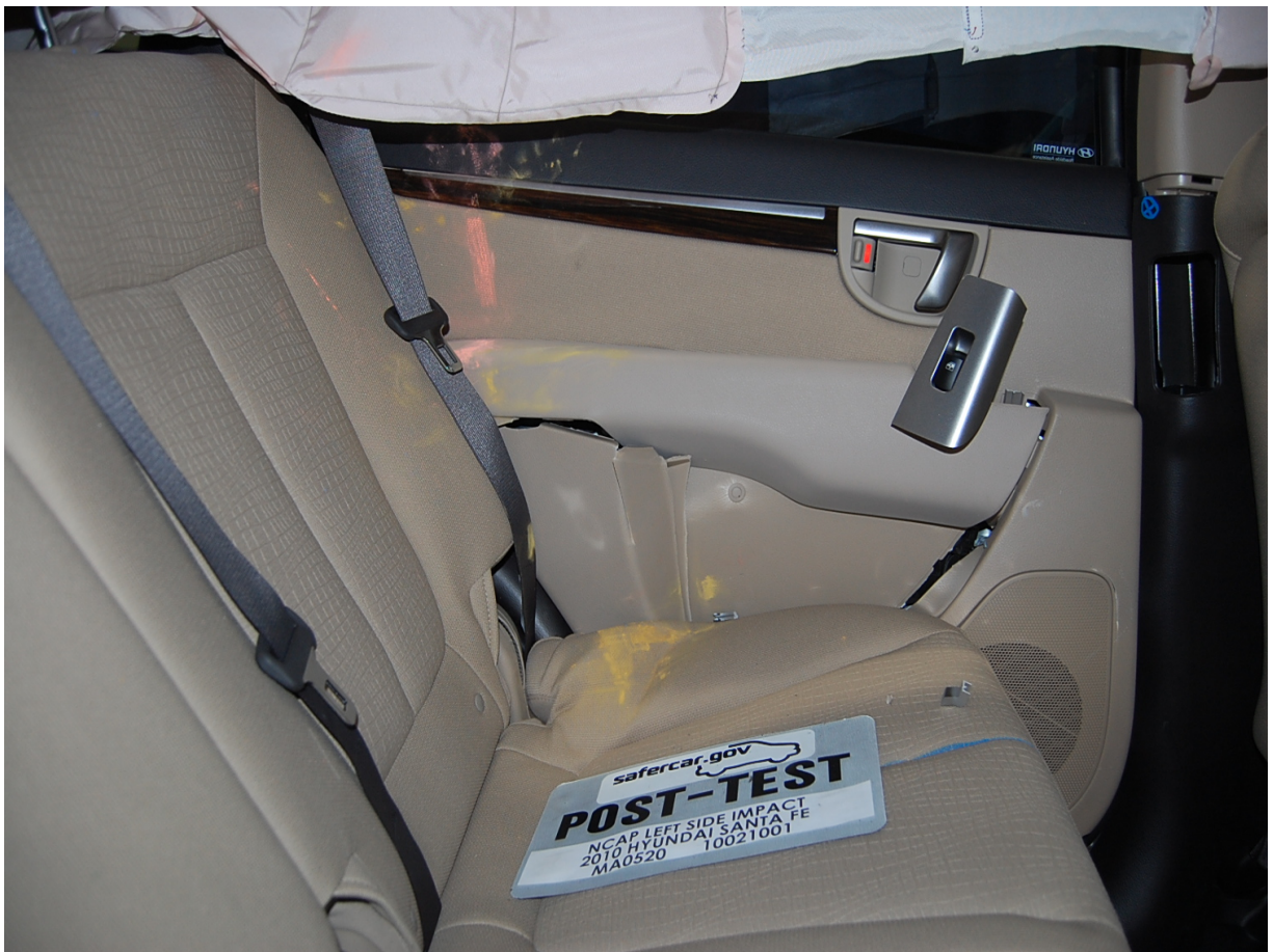
Post-Test Passenger Dummy Torso Contact
