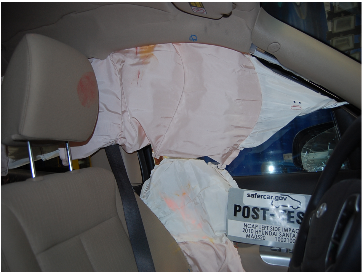
Post-Test Driver Dummy Head Contact View
