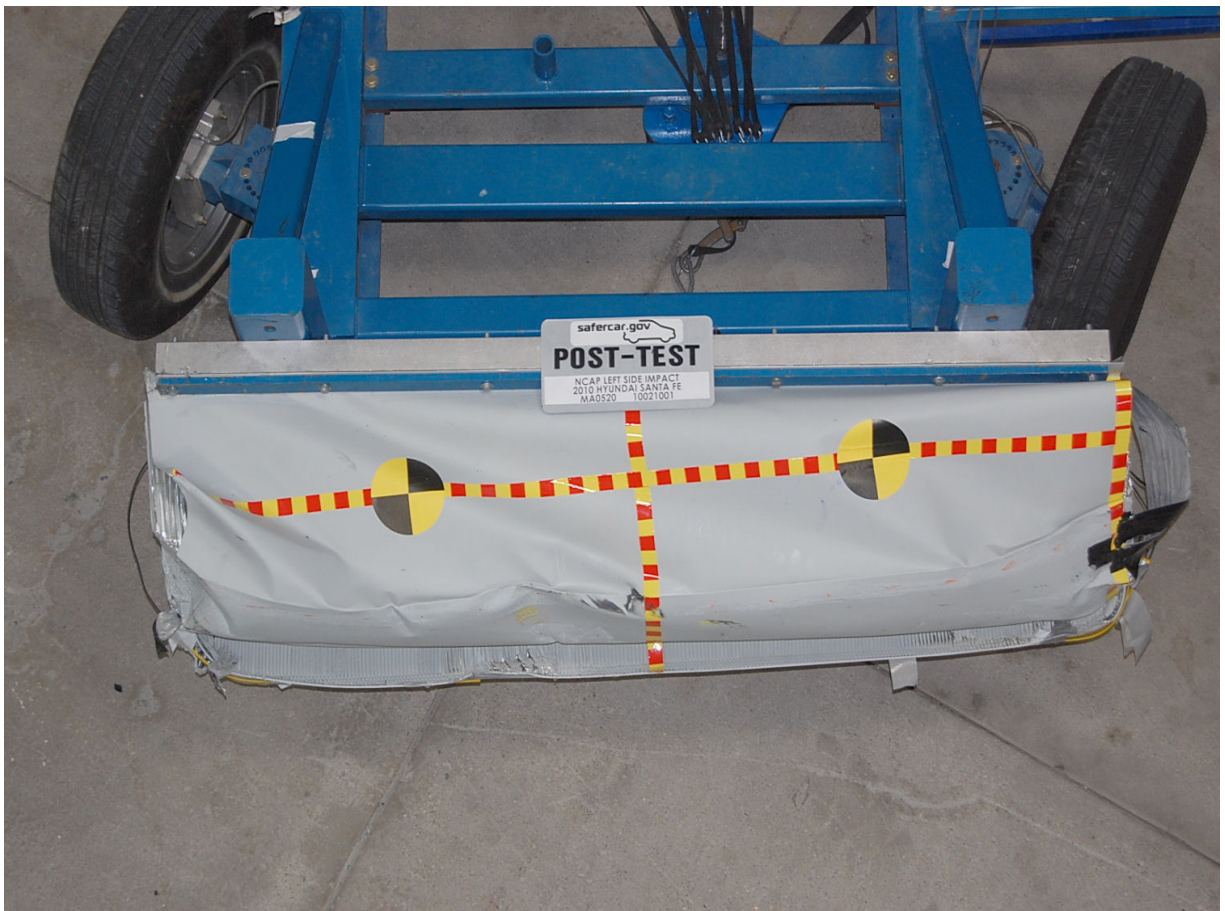
Post-Test Top View of Deformable Barrier
