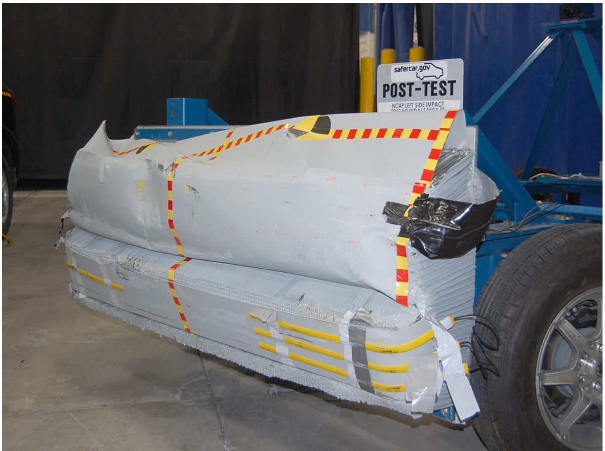
Post-Test Left Side View of Deformable Barrier
