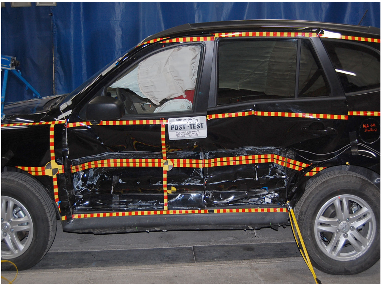
Post-Test Left Side Impact Close-up
