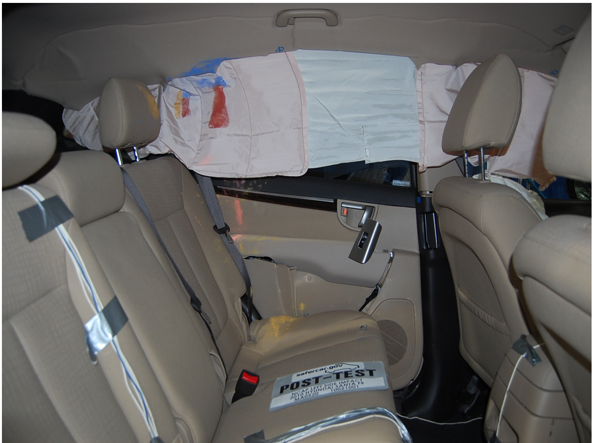
Post-Test Passenger Dummy Contact
