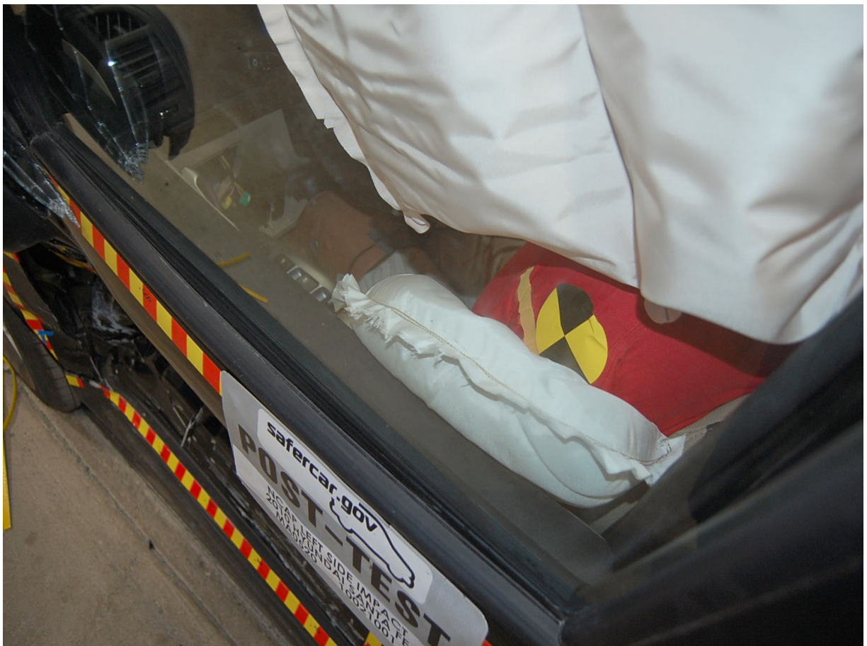
Post-Test Driver Dummy Clearance From Door
