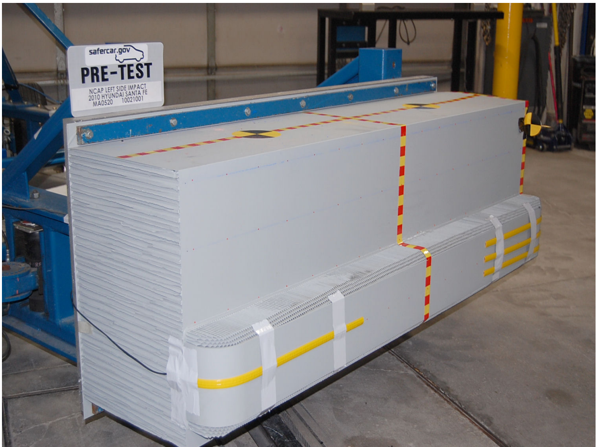
Pre-Test Right Side View of Deformable Barrier
