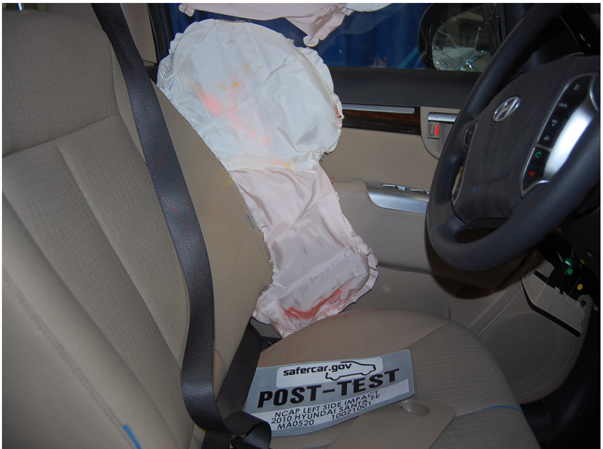
Post-Test Driver Dummy Torso Contact
