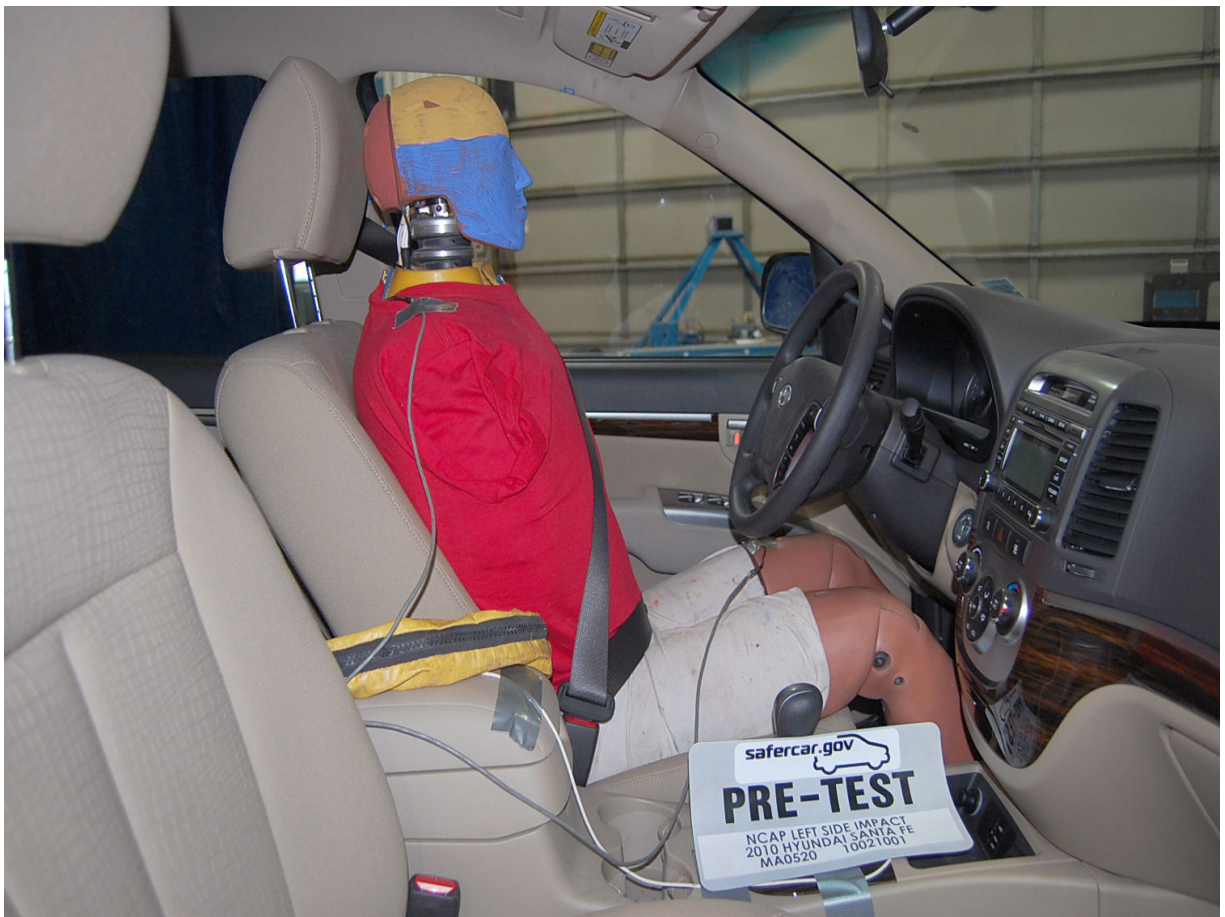
Pre-Test Driver Dummy Right Side View
