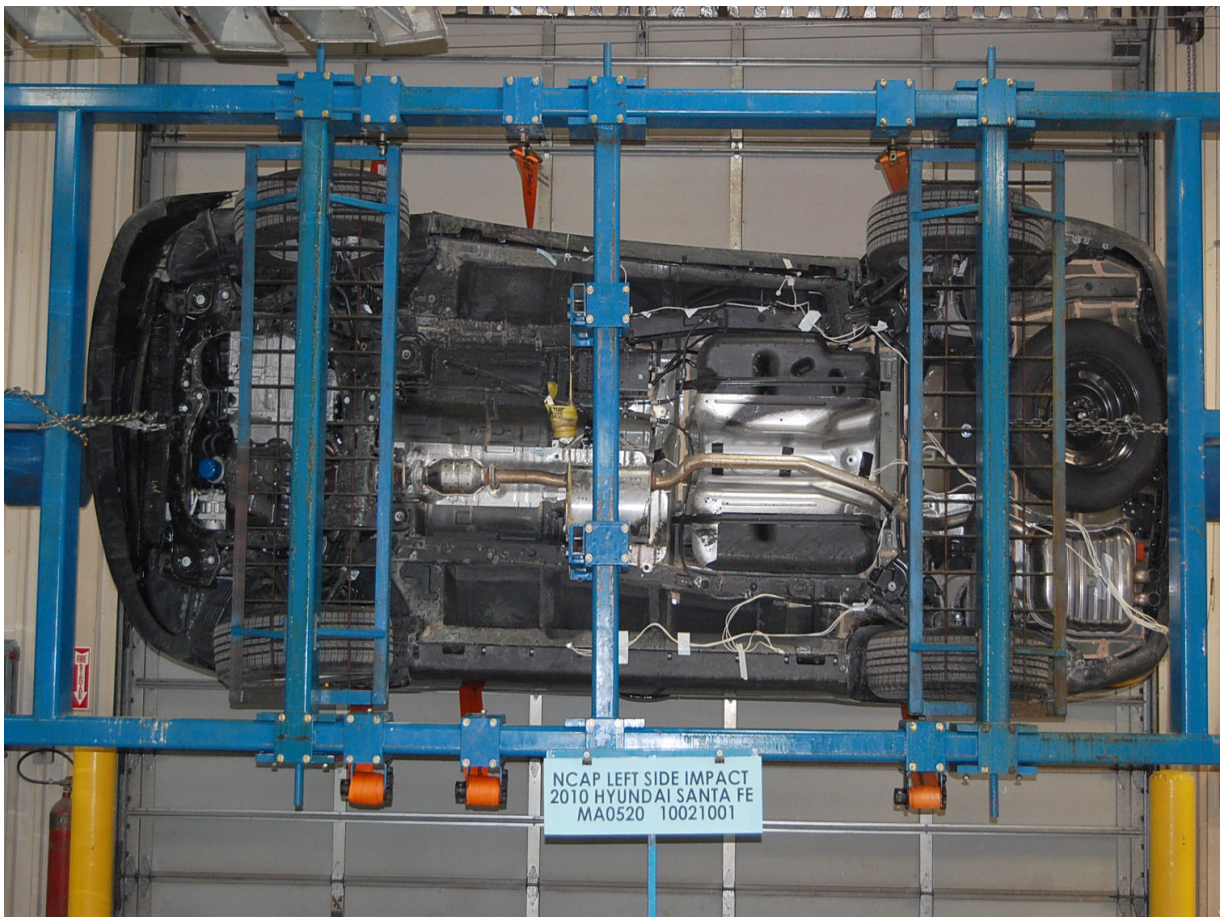
Vehicle on Rollover Device (270 Degrees)
