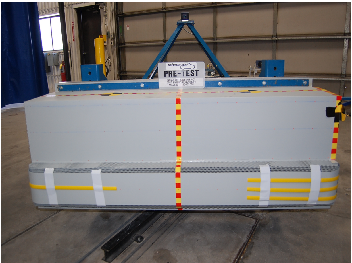
Pre-Test Front View of Deformable Barrier
