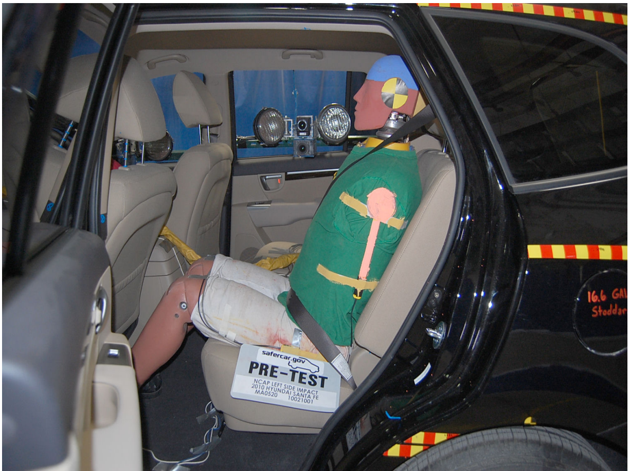
Pre-Test Passenger Dummy (Door Open)
