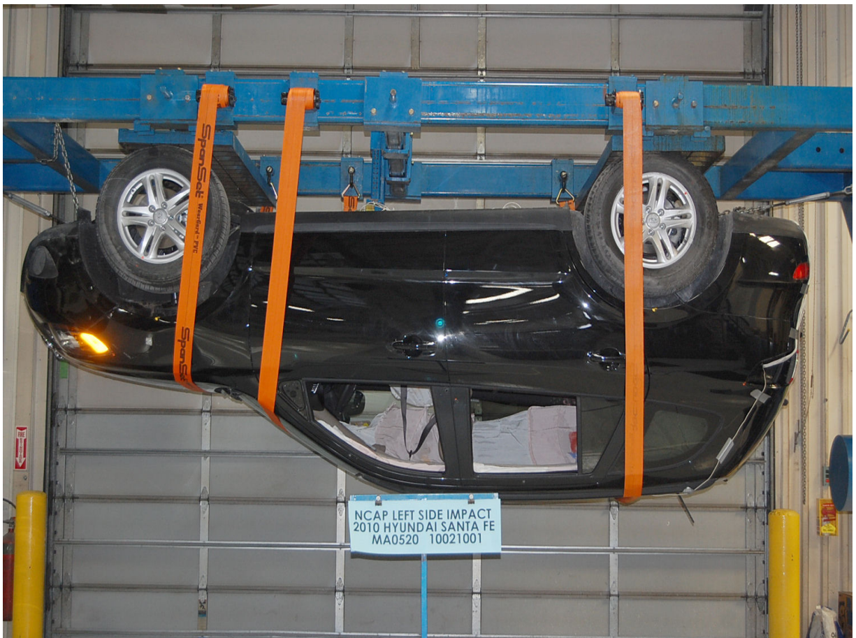
Vehicle on Rollover Device (180 Degrees)
