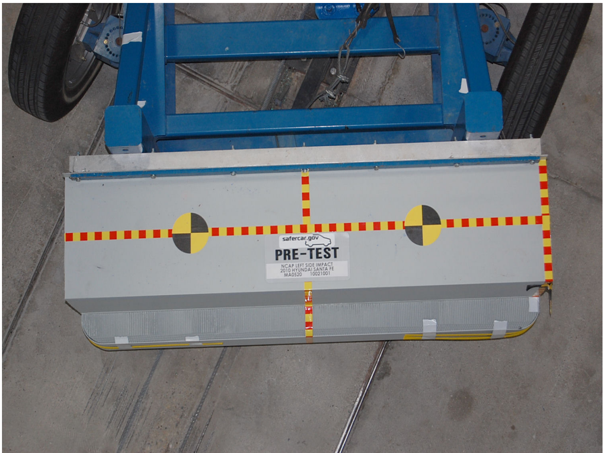
Pre-Test Top View of Deformable Barrier
