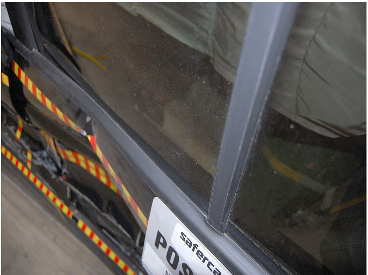
Post-Test Passenger Dummy Clearance From Door
