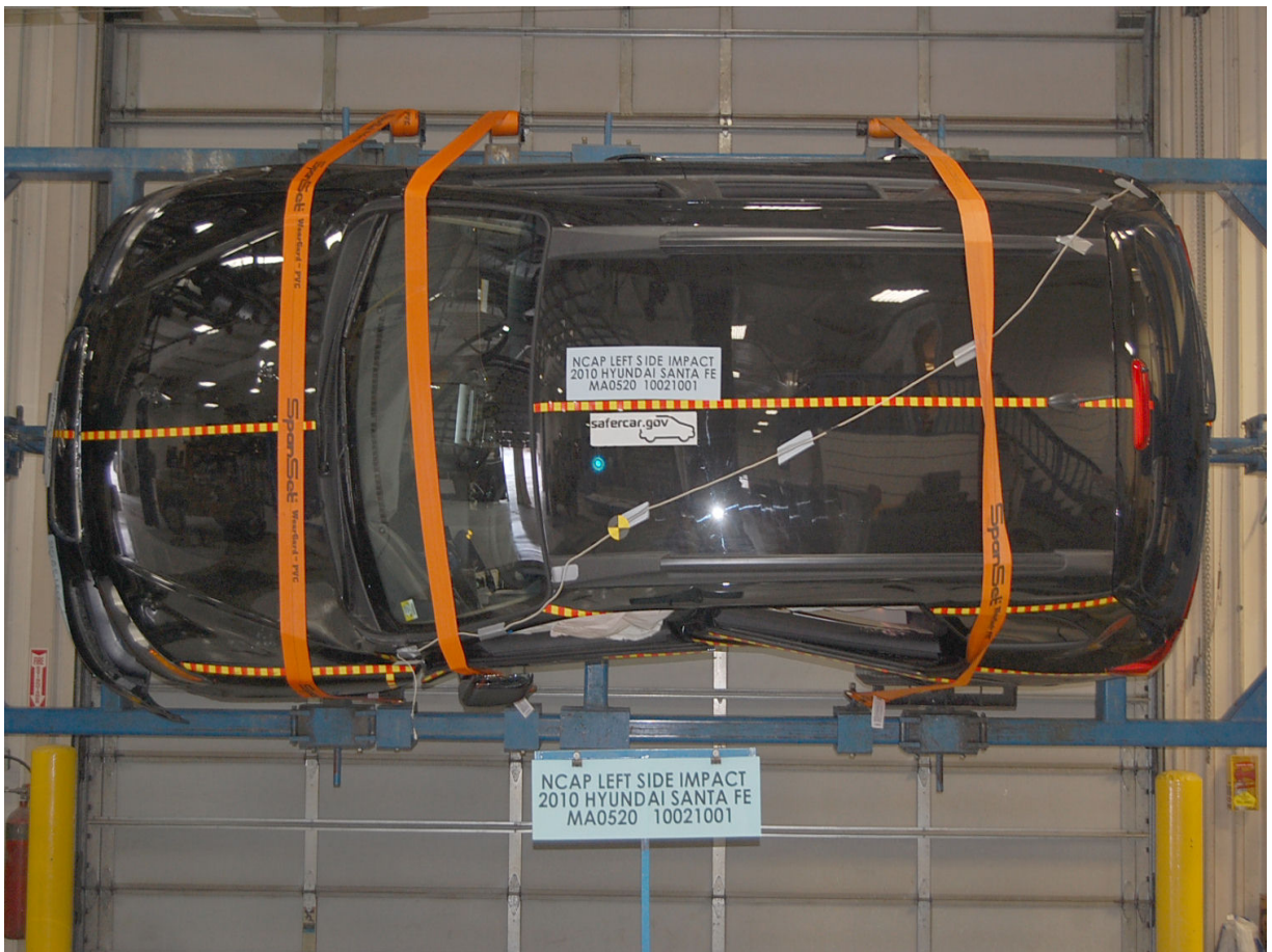
Vehicle on Rollover Device (90 Degrees)
