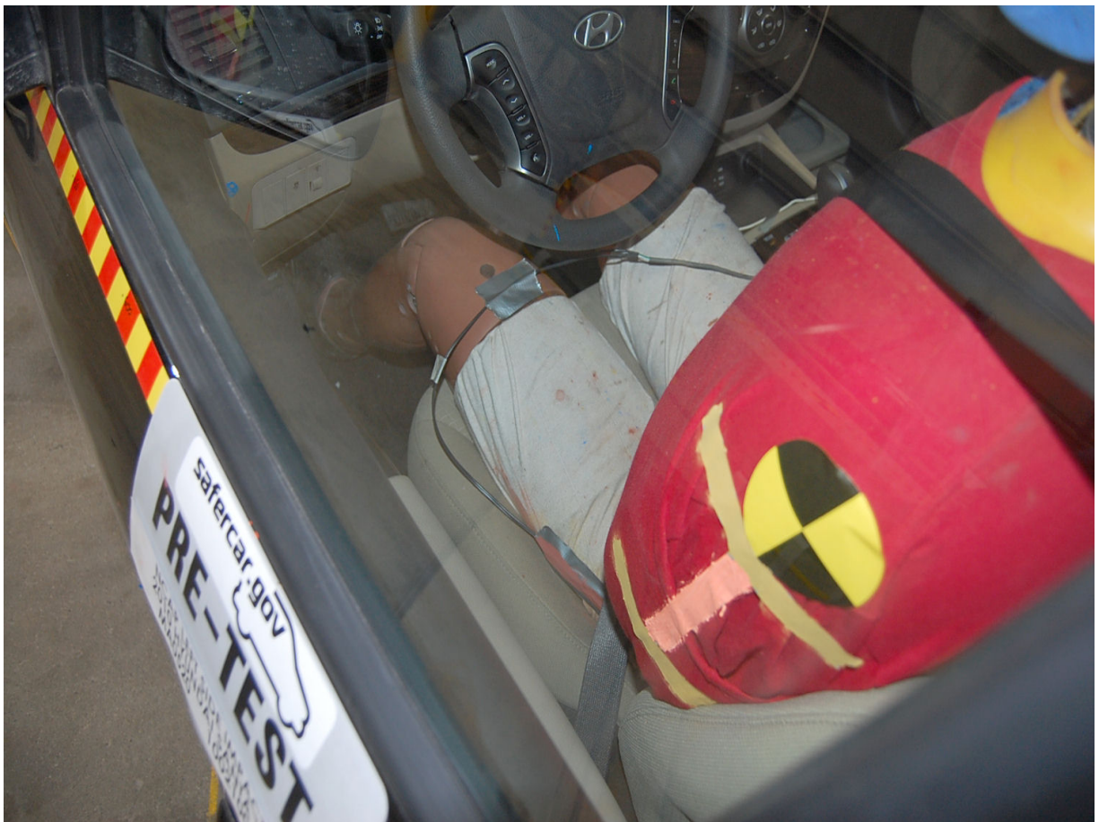
Pre-Test Driver Dummy Clearance From Door
