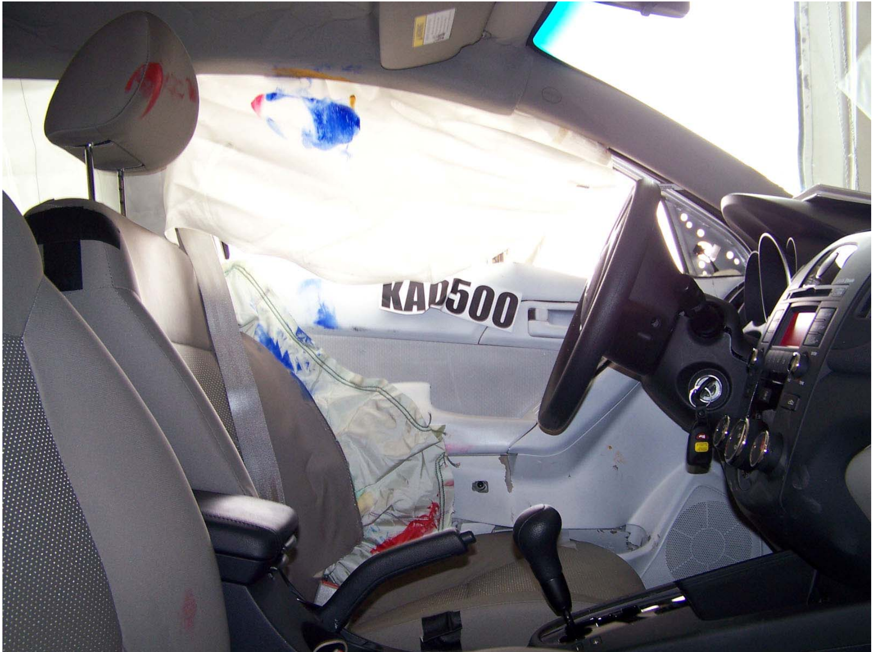
Figure A-43: Post-Test Front Door Panel (Interior)
