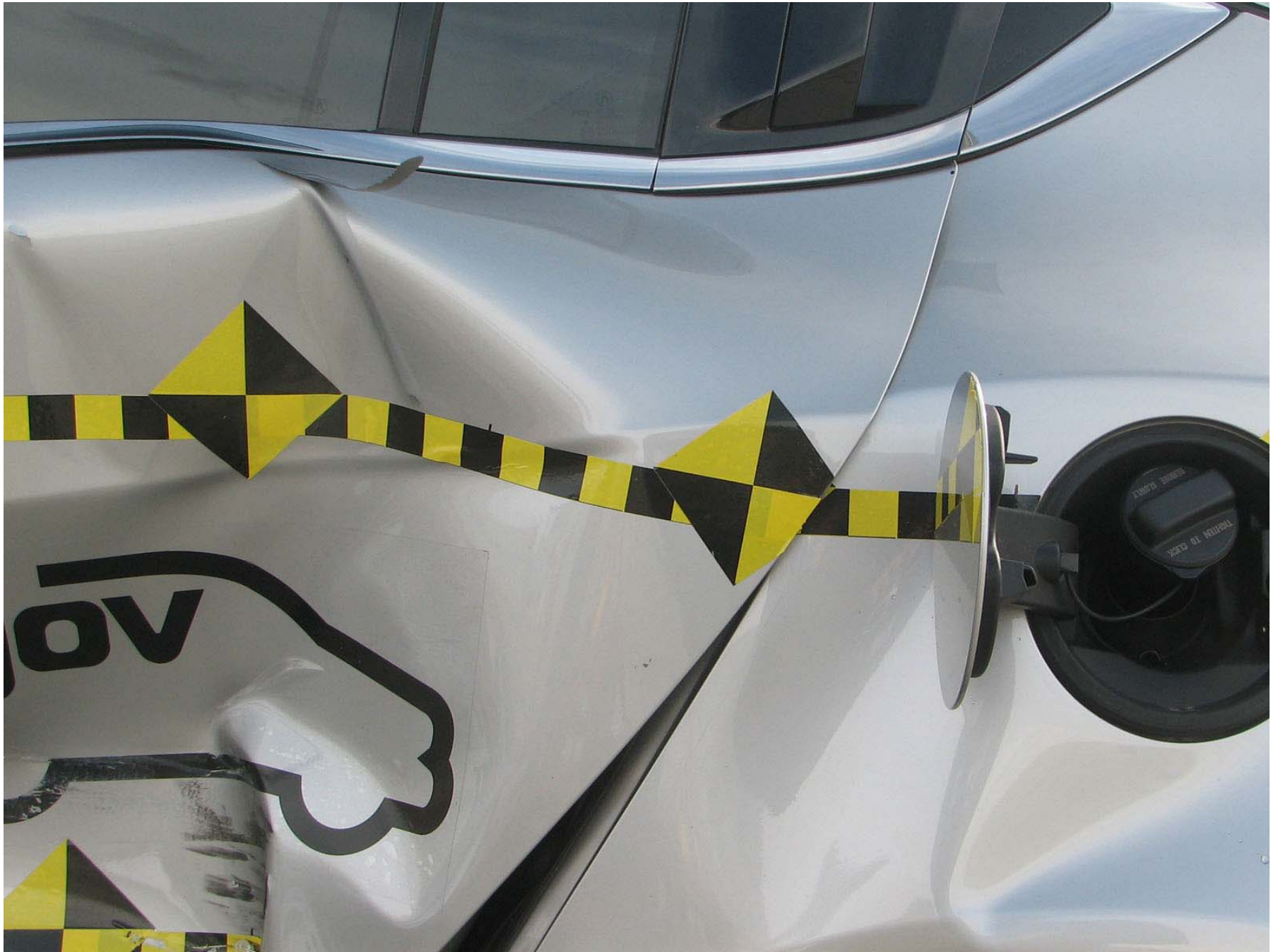
Figure A-34: Post-Test Left Rear Door
