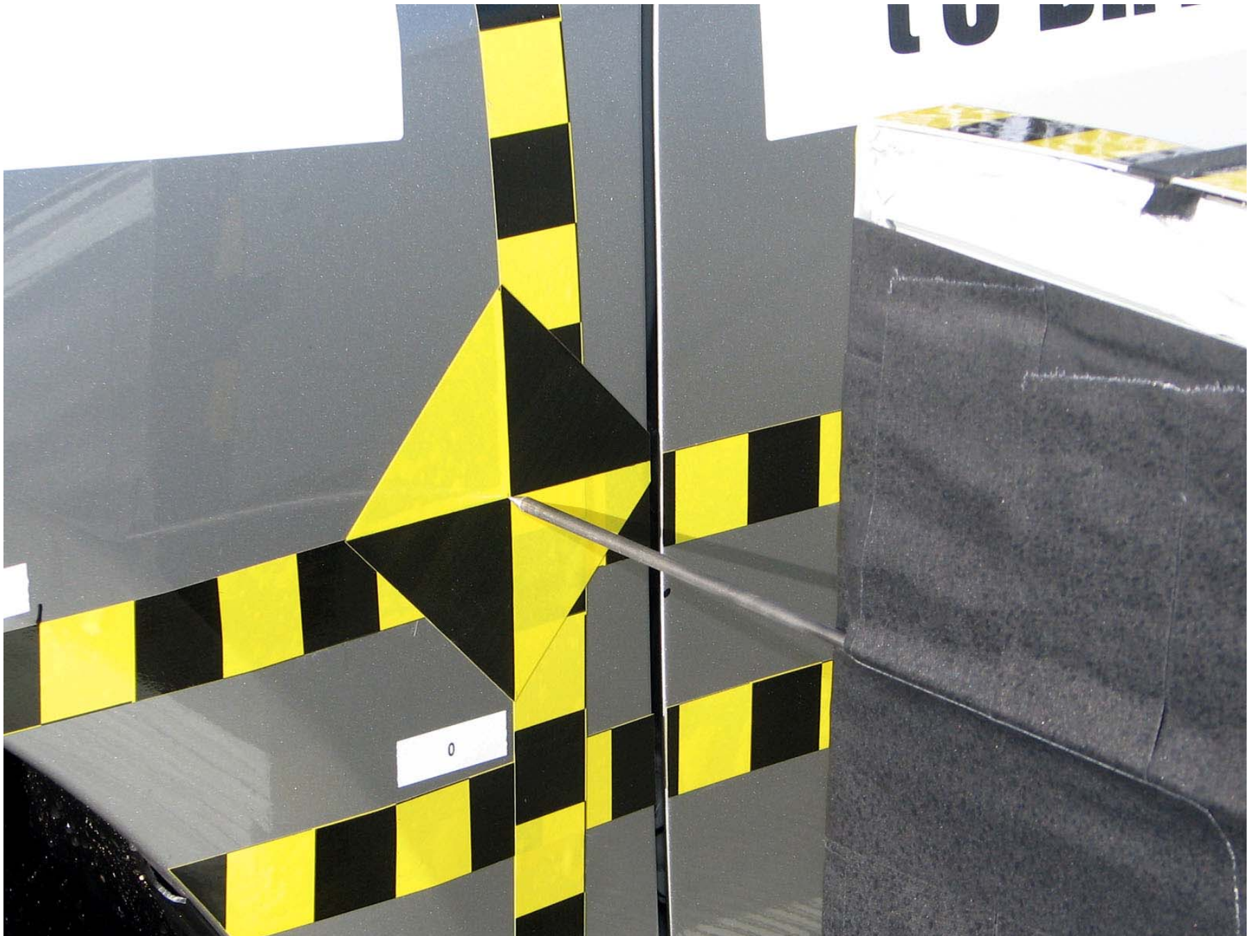
Figure A-25: Pre-Test Left Impact Point
