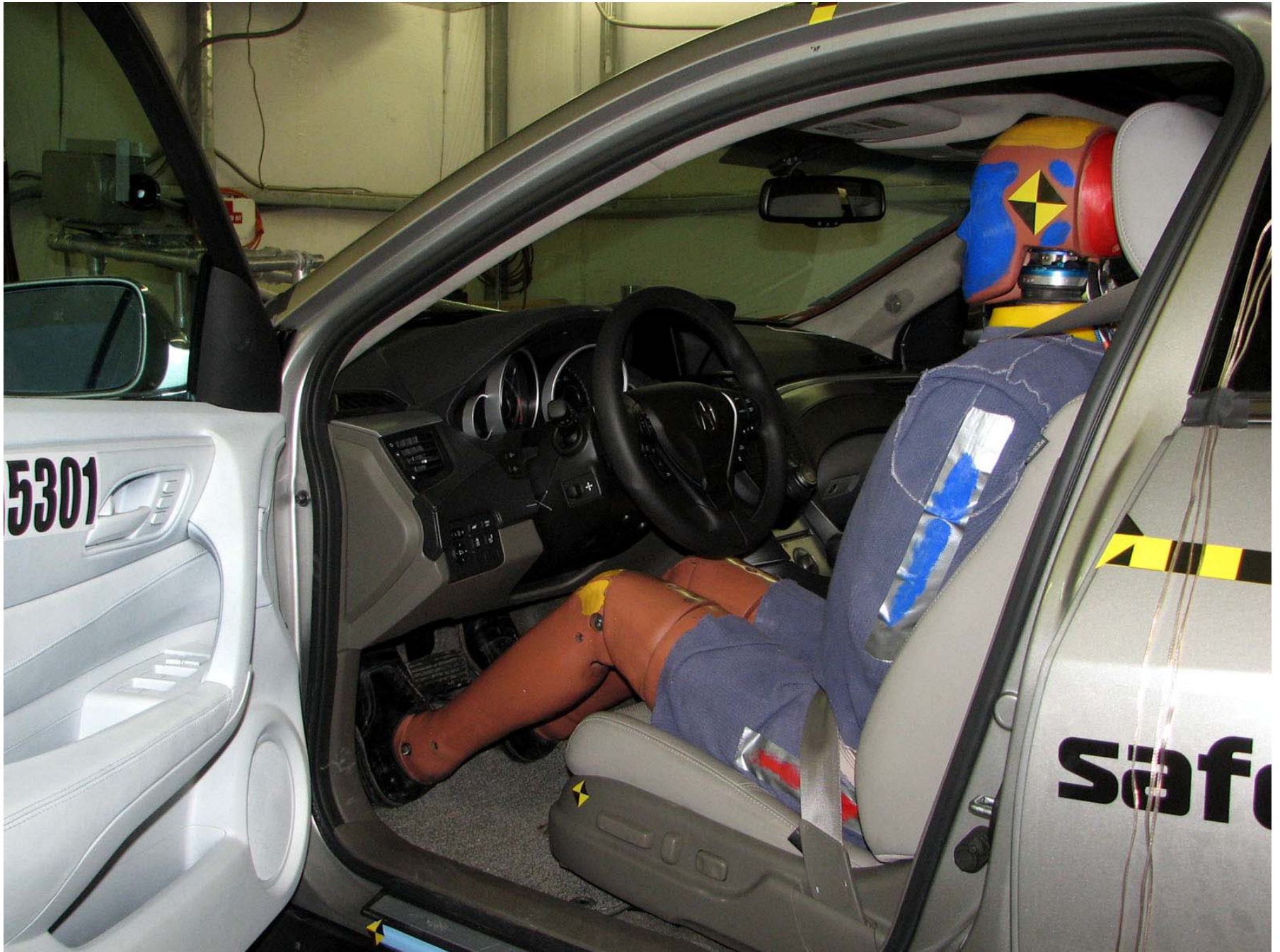
Figure A-35: Pre-Test Driver Dummy (Door Open)
