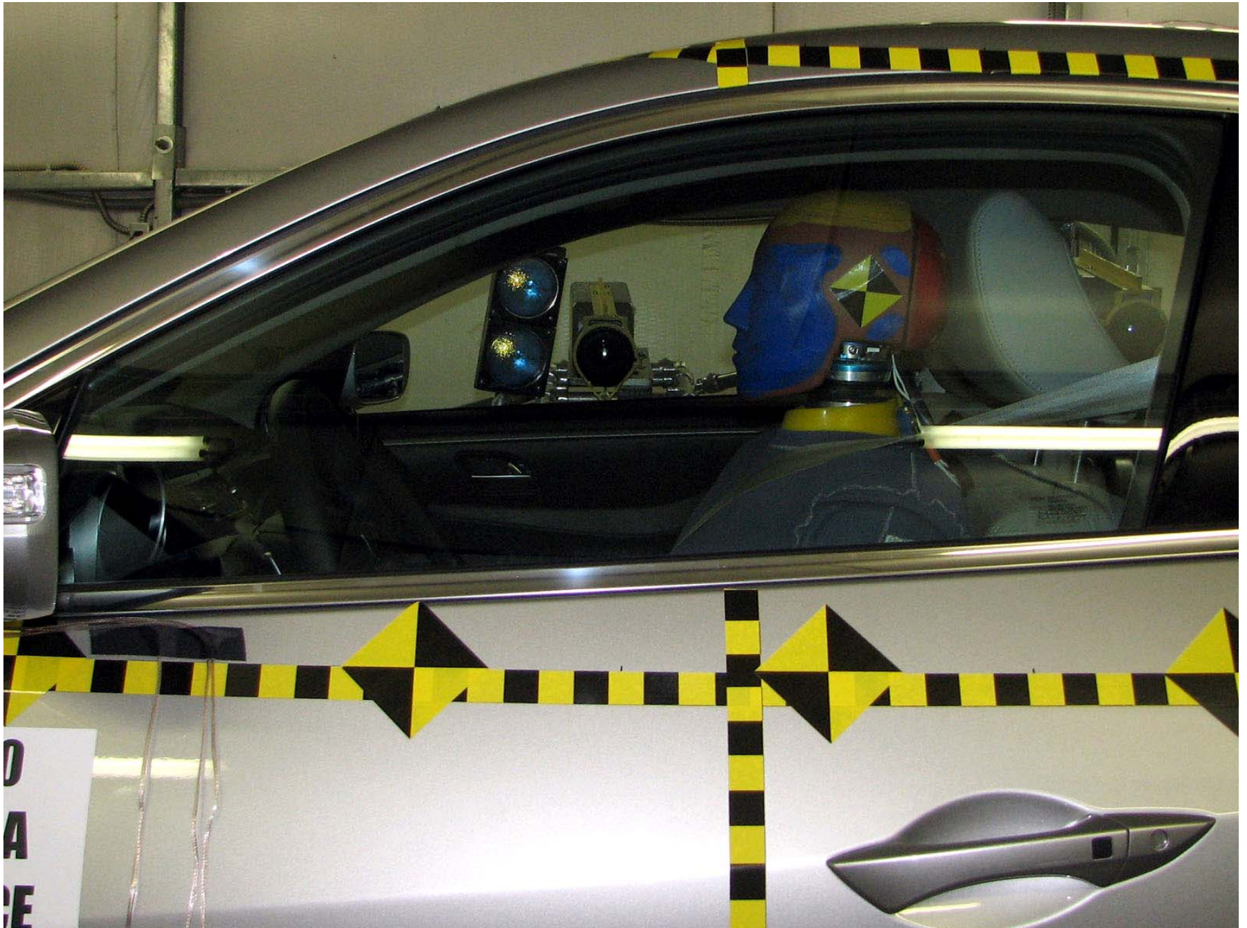
Figure A-36: Pre-Test Driver Dummy (Through Window)
