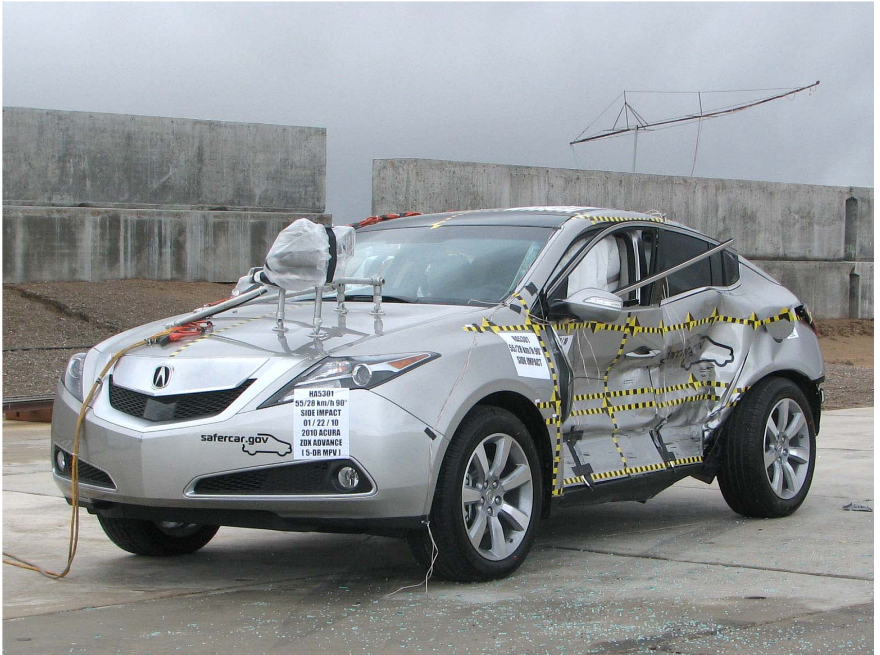
Figure A-8: Post-Test Left Front \frac{3}{4} View
