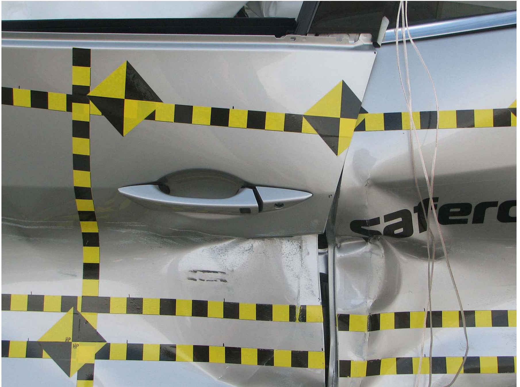
Figure A-32: Post-Test Left Front Door
