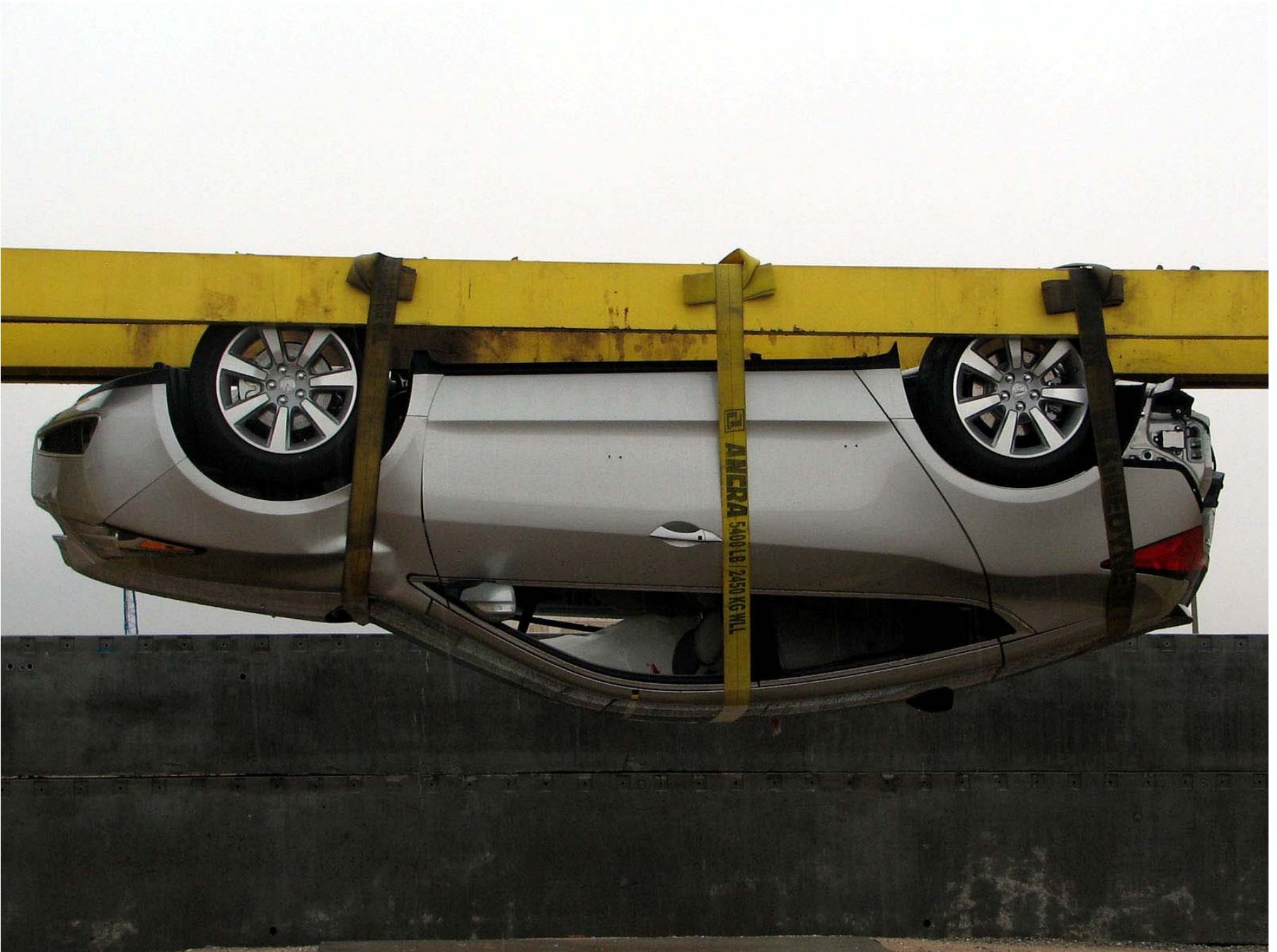
Figure A-63: Vehicle on Rollover Device (180°)
