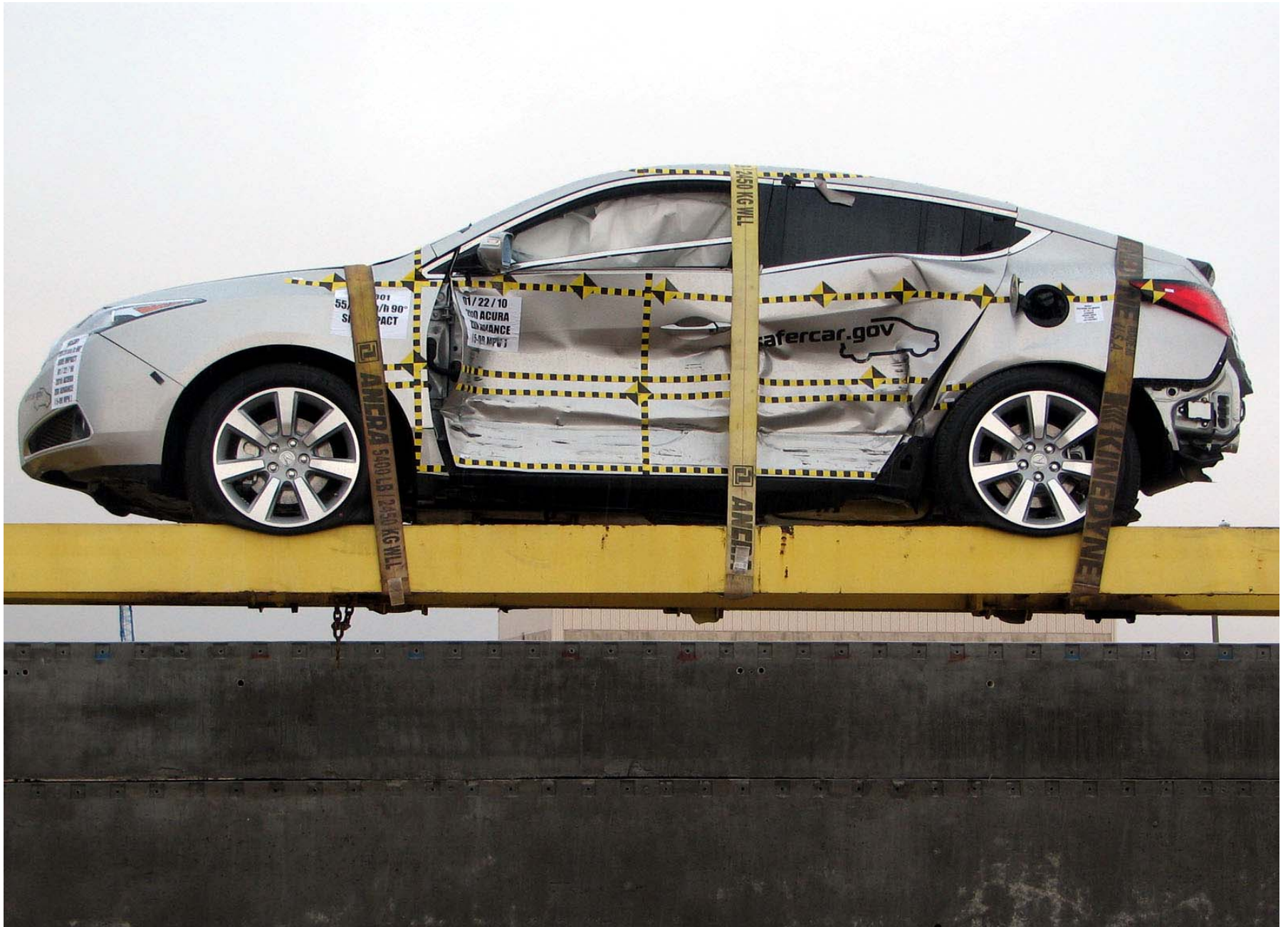
Figure A-65: Vehicle on Rollover Device (360°)
