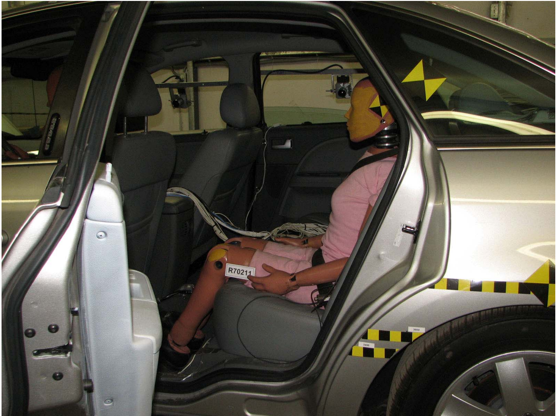
Figure A-294: Target Vehicle Pre-Test Passenger Dummy Left Side View (Door Open)
