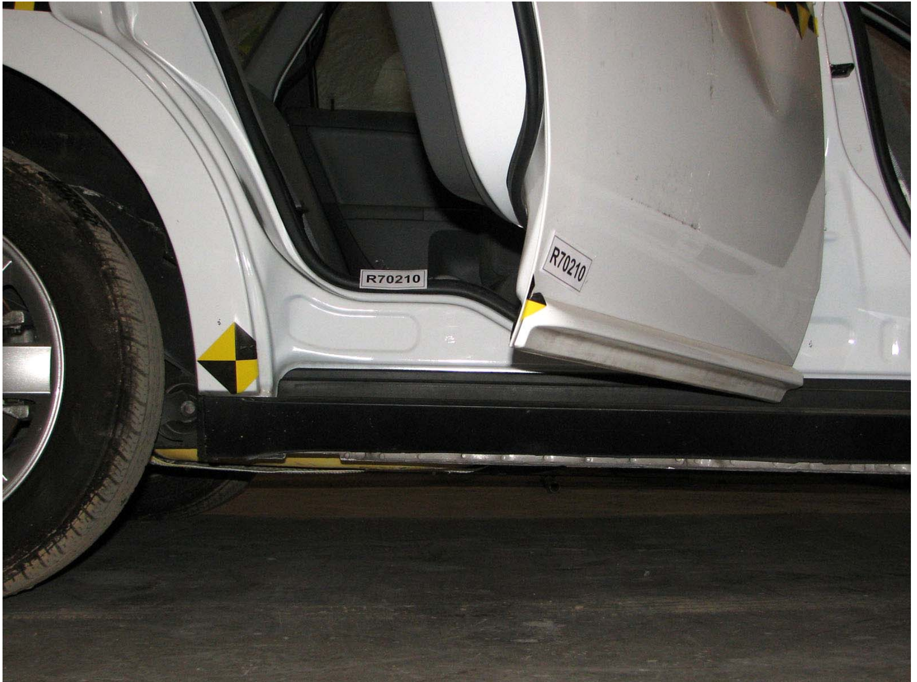
Figure A-419: Bullet Vehicle Post-Test Right Rear Sill Side View, Door Open
