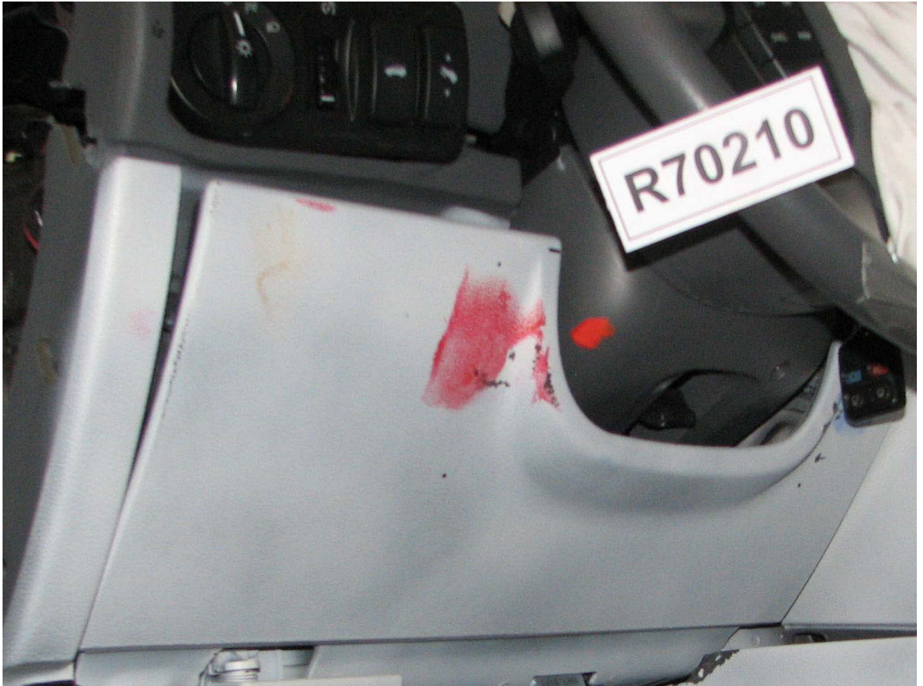
Figure A-571: Bullet Vehicle Post-Test Passenger Dummy Contact, Knee Bolster
