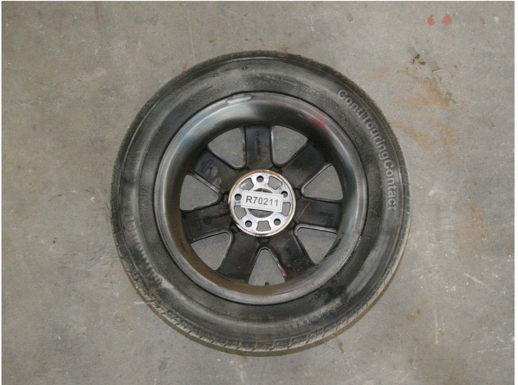
Figure A-162: Target Vehicle Post-Test Right Front Wheel Damage (Inside)
