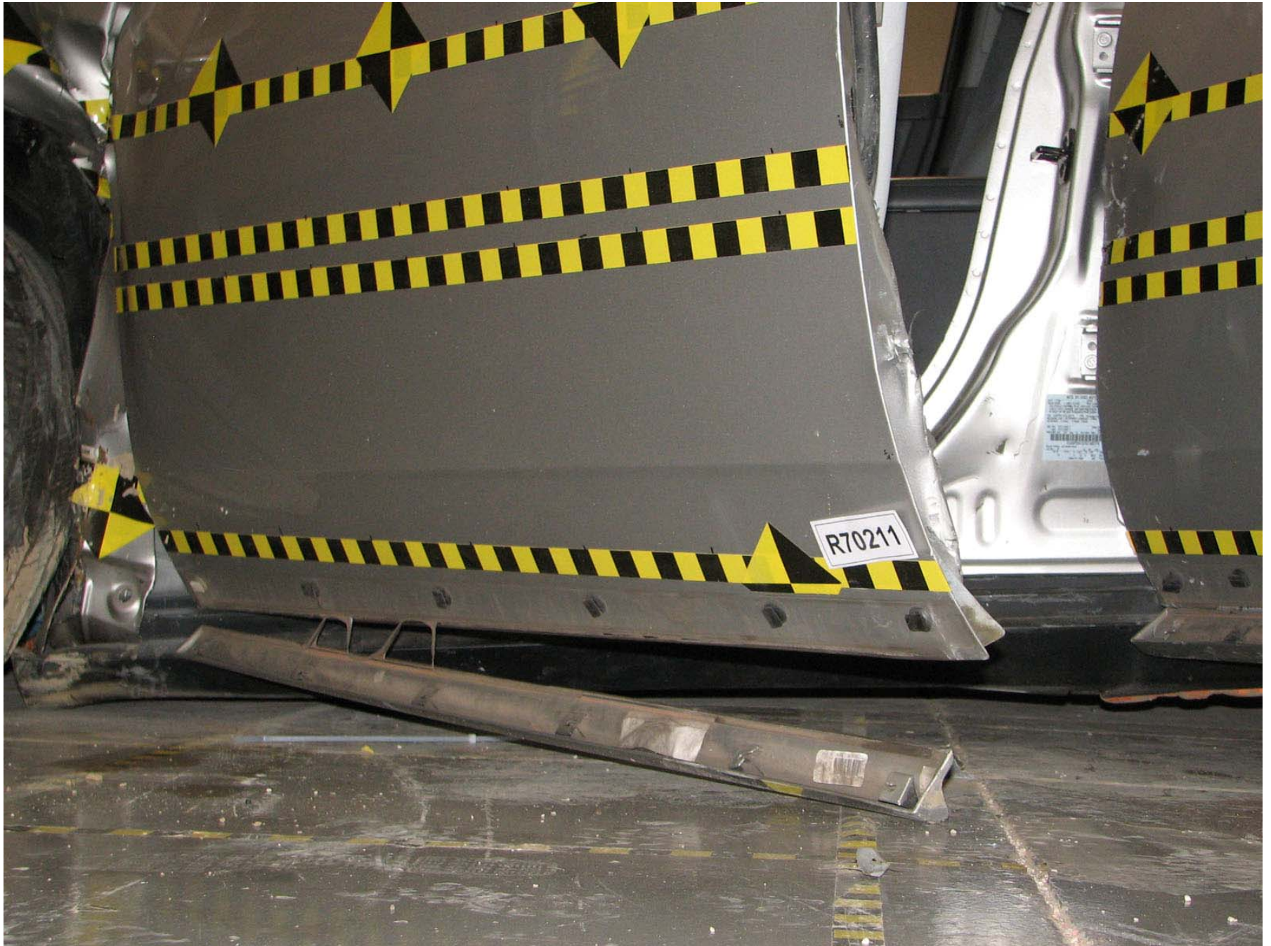
Figure A-96: Target Vehicle Post-Test Left Front Sill Side View, Door Open
