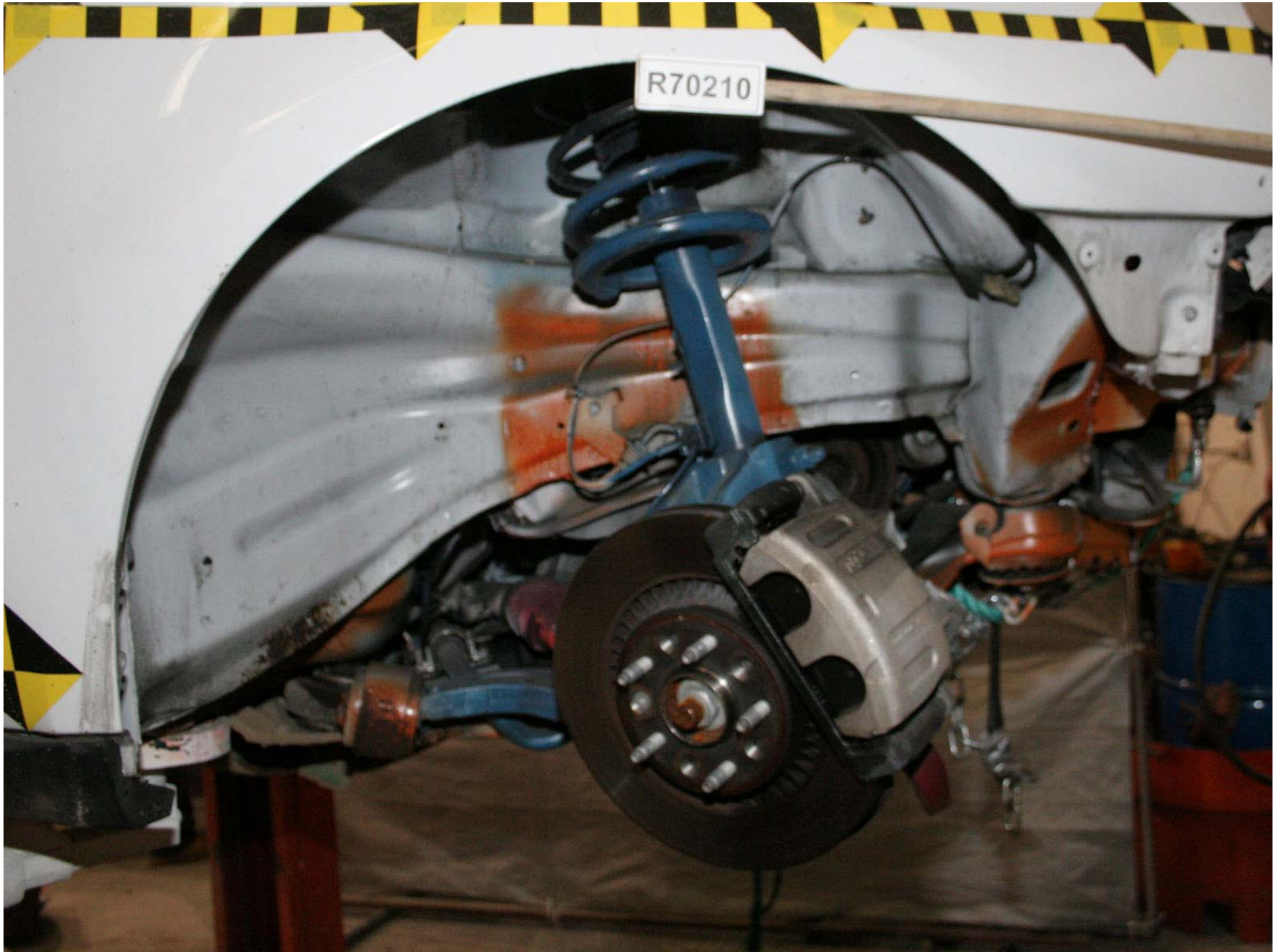
Figure A-491: Bullet Vehicle Post-Test Right Front Wheel Well (Tire Off), Inner Fender Removed
