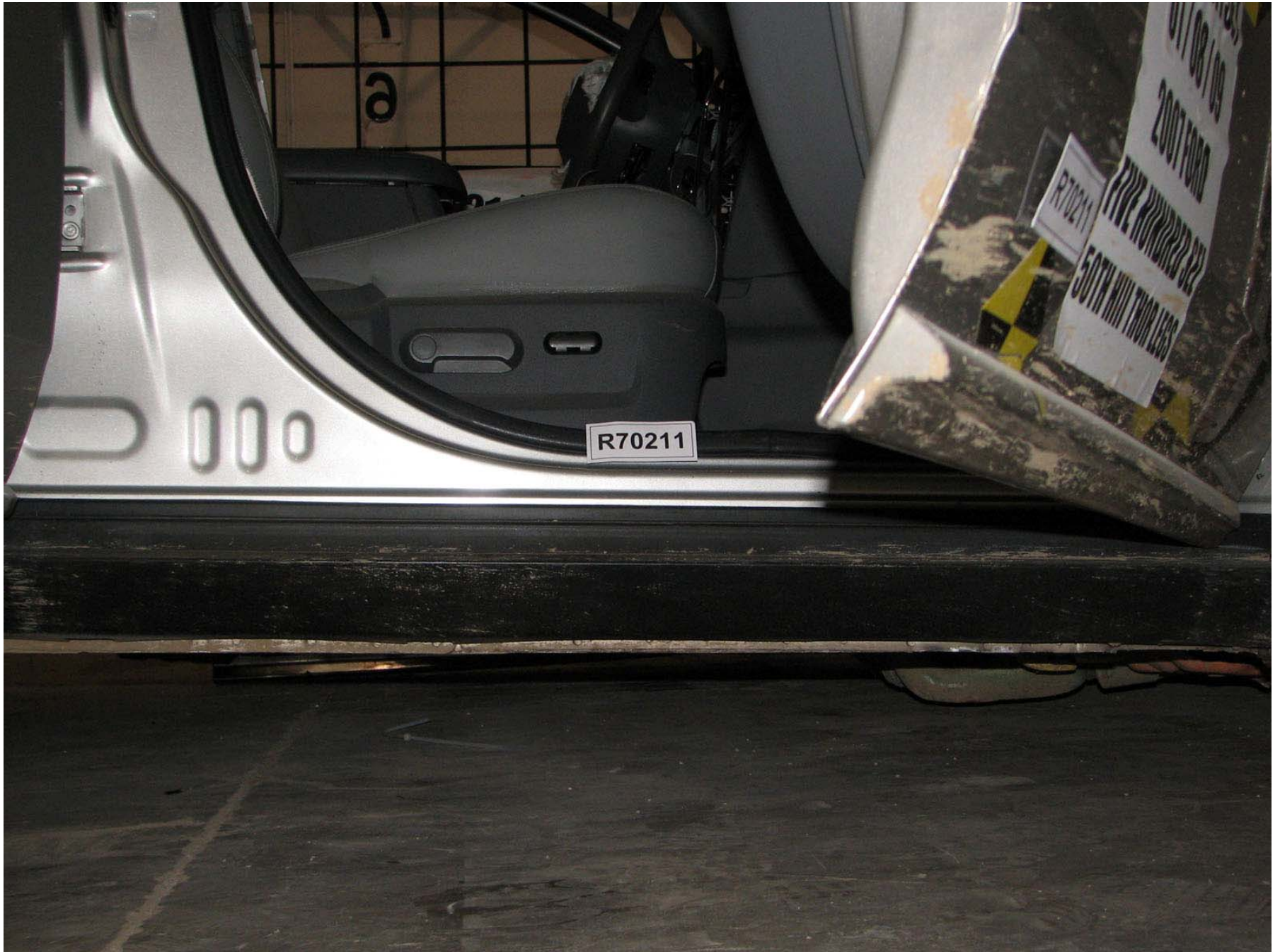
Figure A-124: Target Vehicle Post-Test Right Front Sill Side View, Door Open
