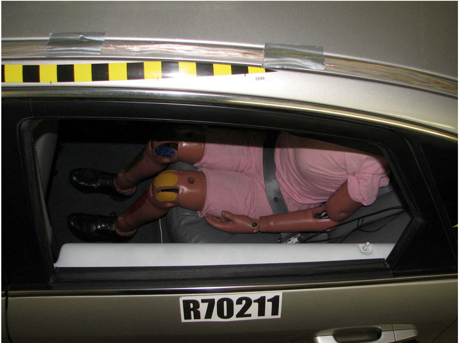
Figure A-305: Target Vehicle Pre-Test Passenger Dummy Clearance from Door
