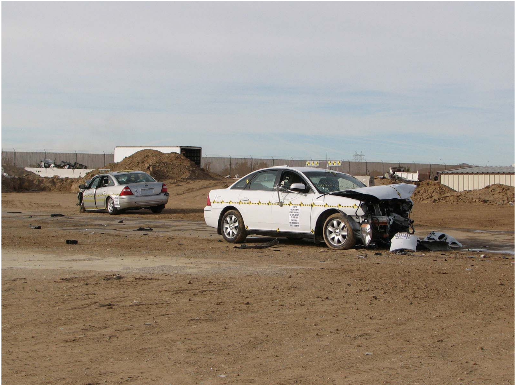
Figure A-54: Test Set-Up Post-Test Right Front \frac{3}{4} View
