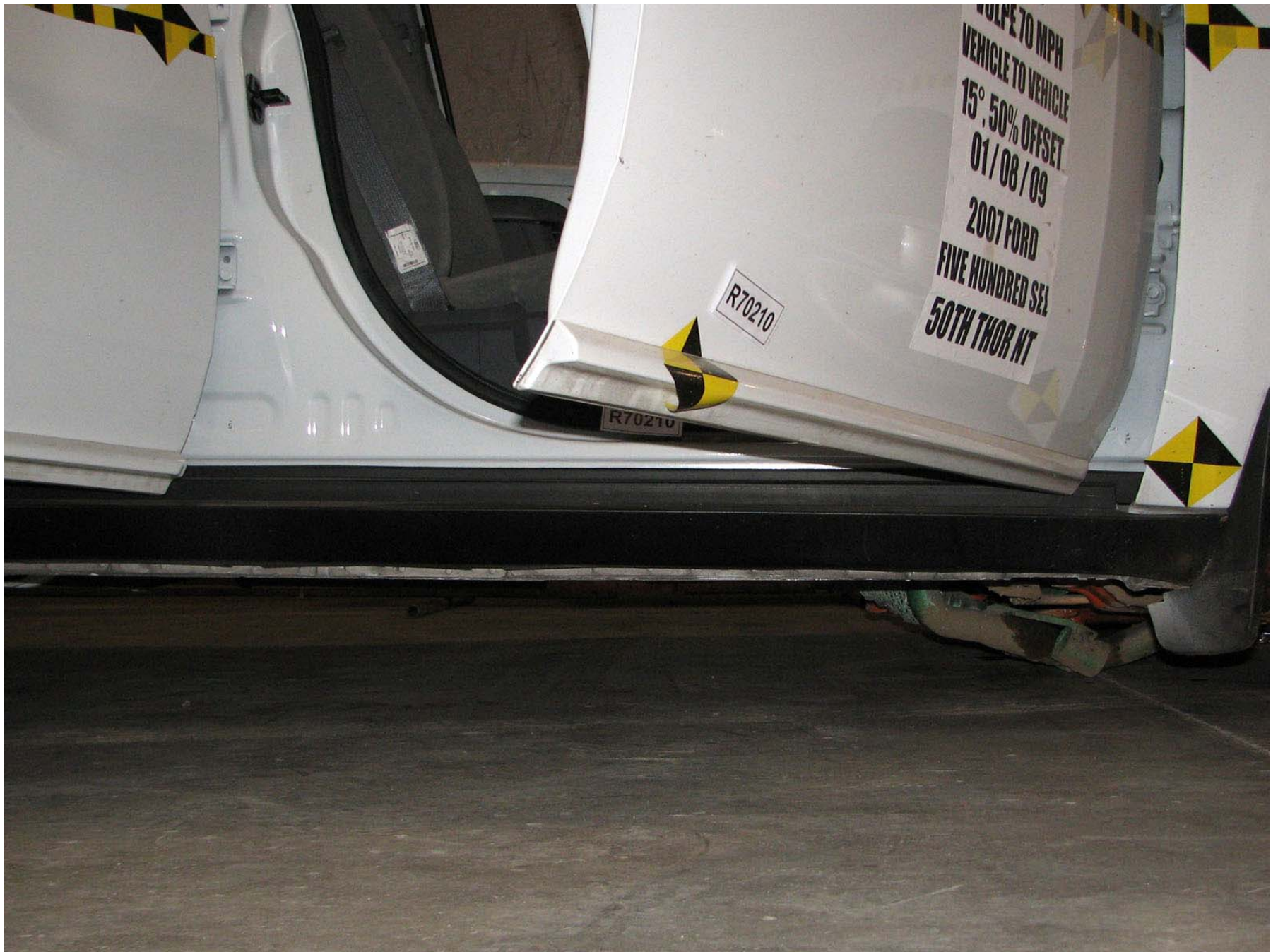
Figure A-411: Bullet Vehicle Post-Test Right Front Sill Side View, Door Open
