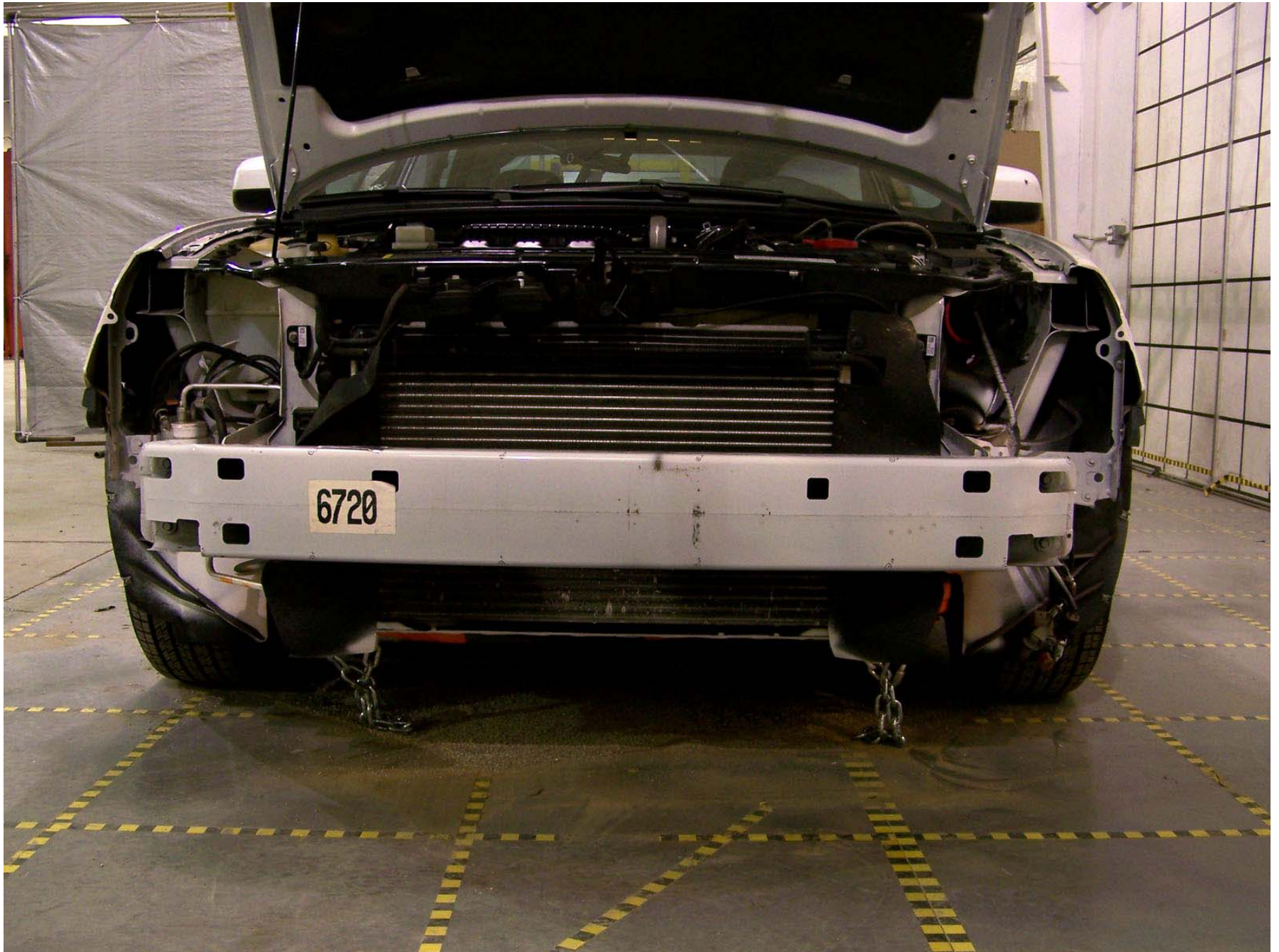
Figure A-600: Bullet Vehicle Pre-Test Structural Member Crush Measurement
