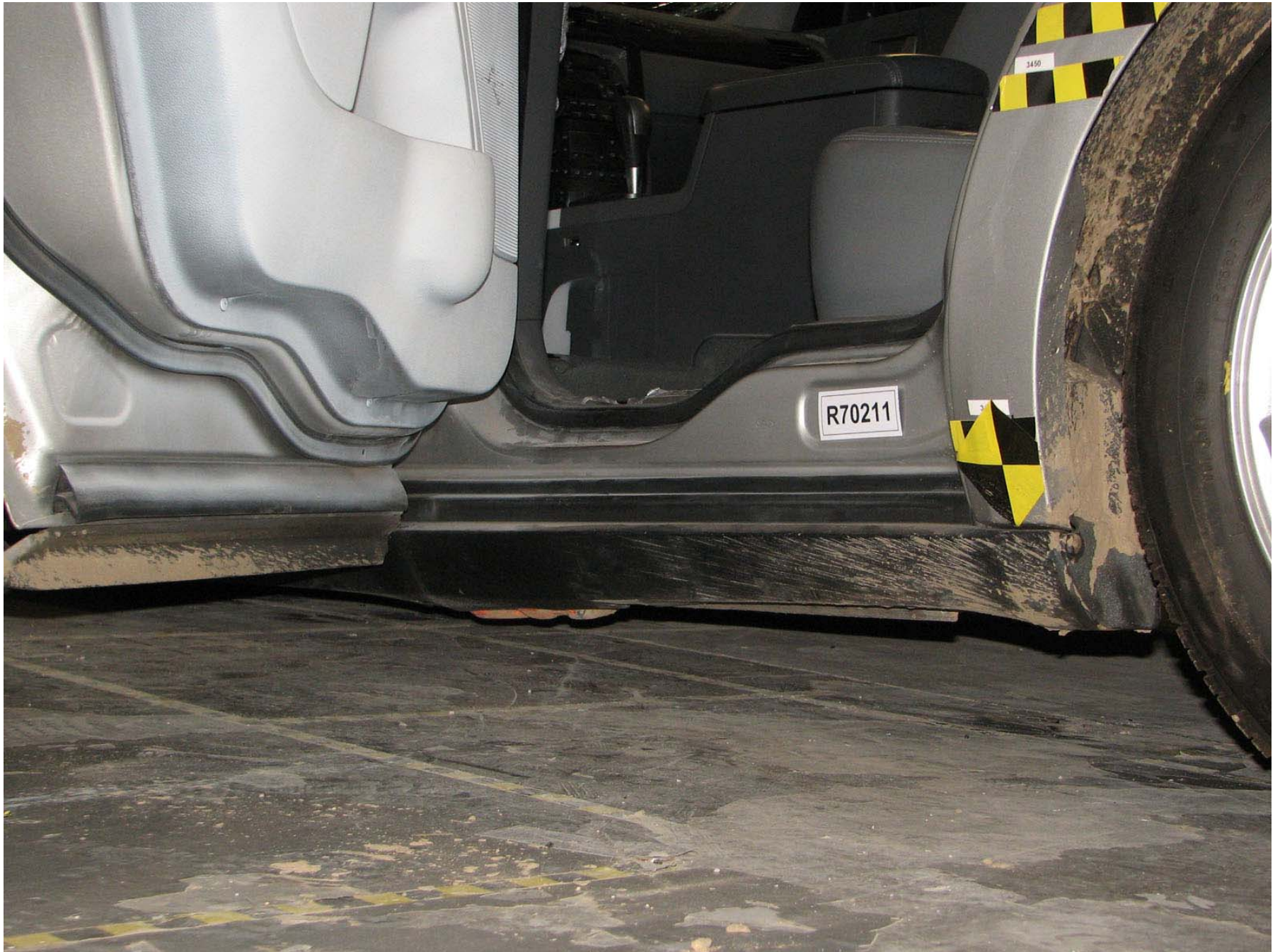
Figure A-108: Target Vehicle Post-Test Left Rear Sill Rear \frac{3}{4} View, Door Open
