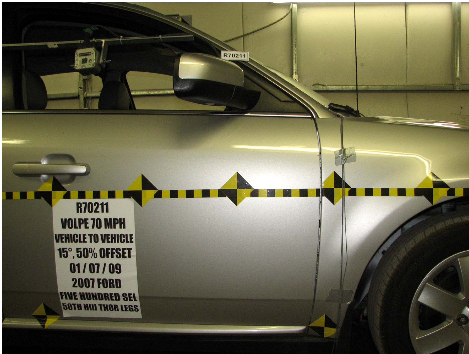
Figure A-109: Target Vehicle Pre-Test Right Side A-Pillar Side View
