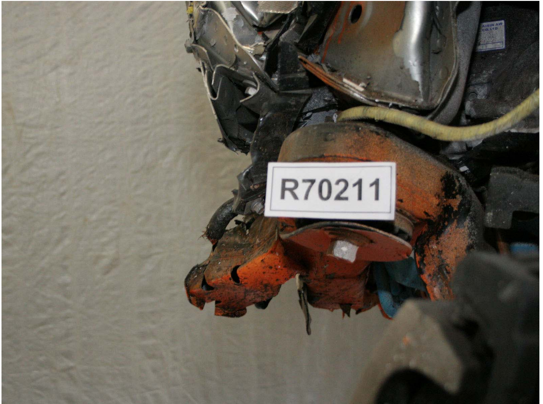
Figure A-190: Target Vehicle Post-Test Left Side Crush Initiators
