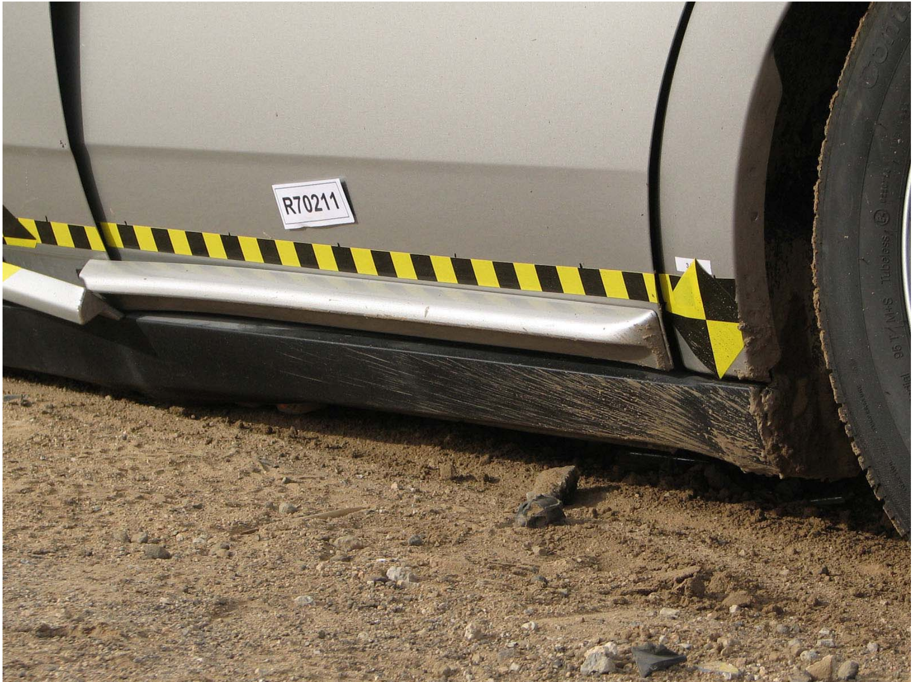
Figure A-106: Target Vehicle Post-Test Left Rear Sill Rear \frac{3}{4} View, Door Closed
