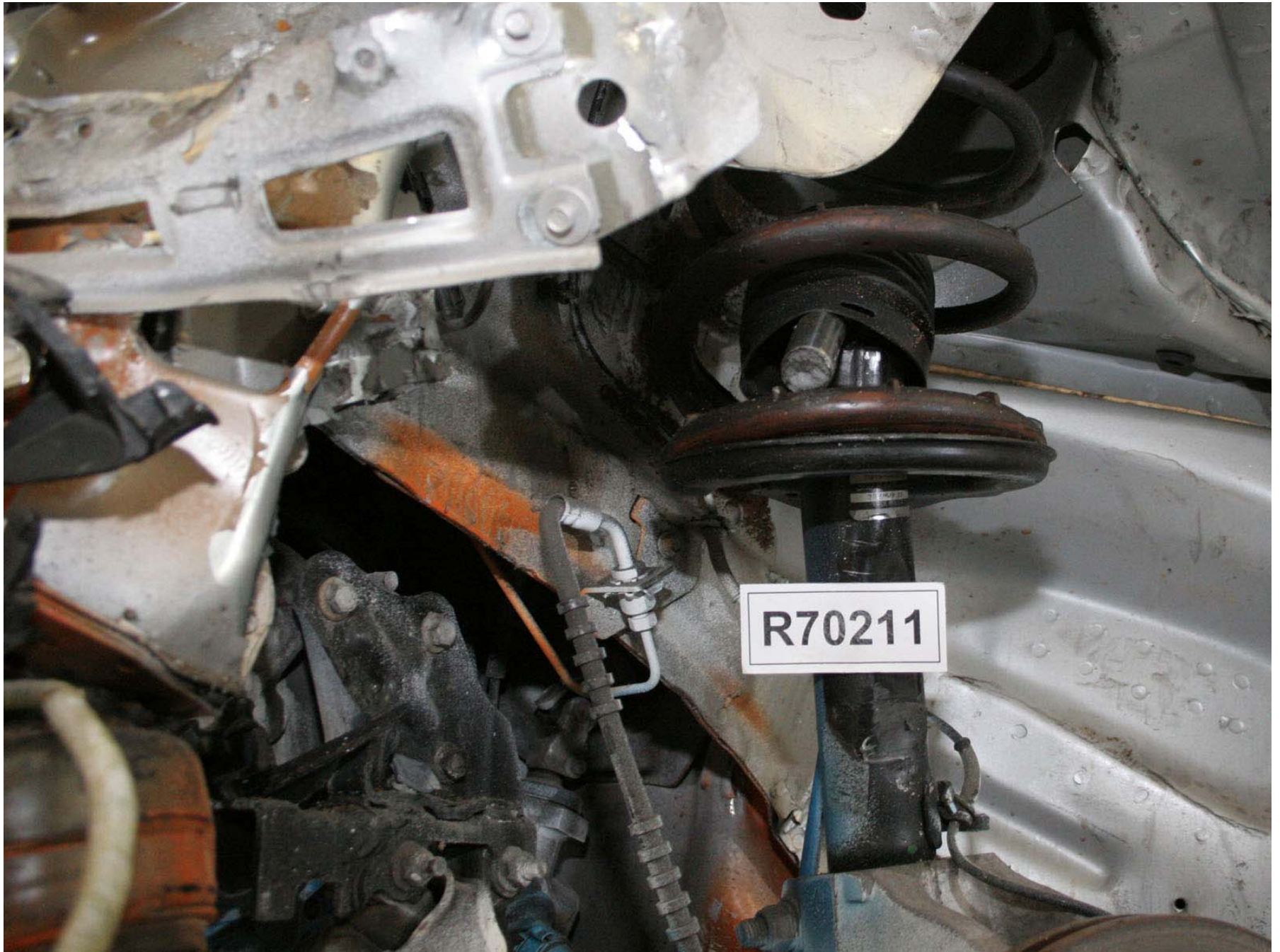
Figure A-186: Target Vehicle Post-Test Left Side Upper Sway Bar Attachment Point
