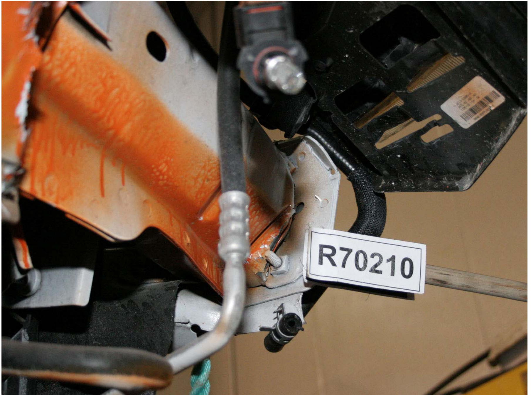
Figure A-517: Test Vehicle Post-Test Right Side Bumper Attachment Point
