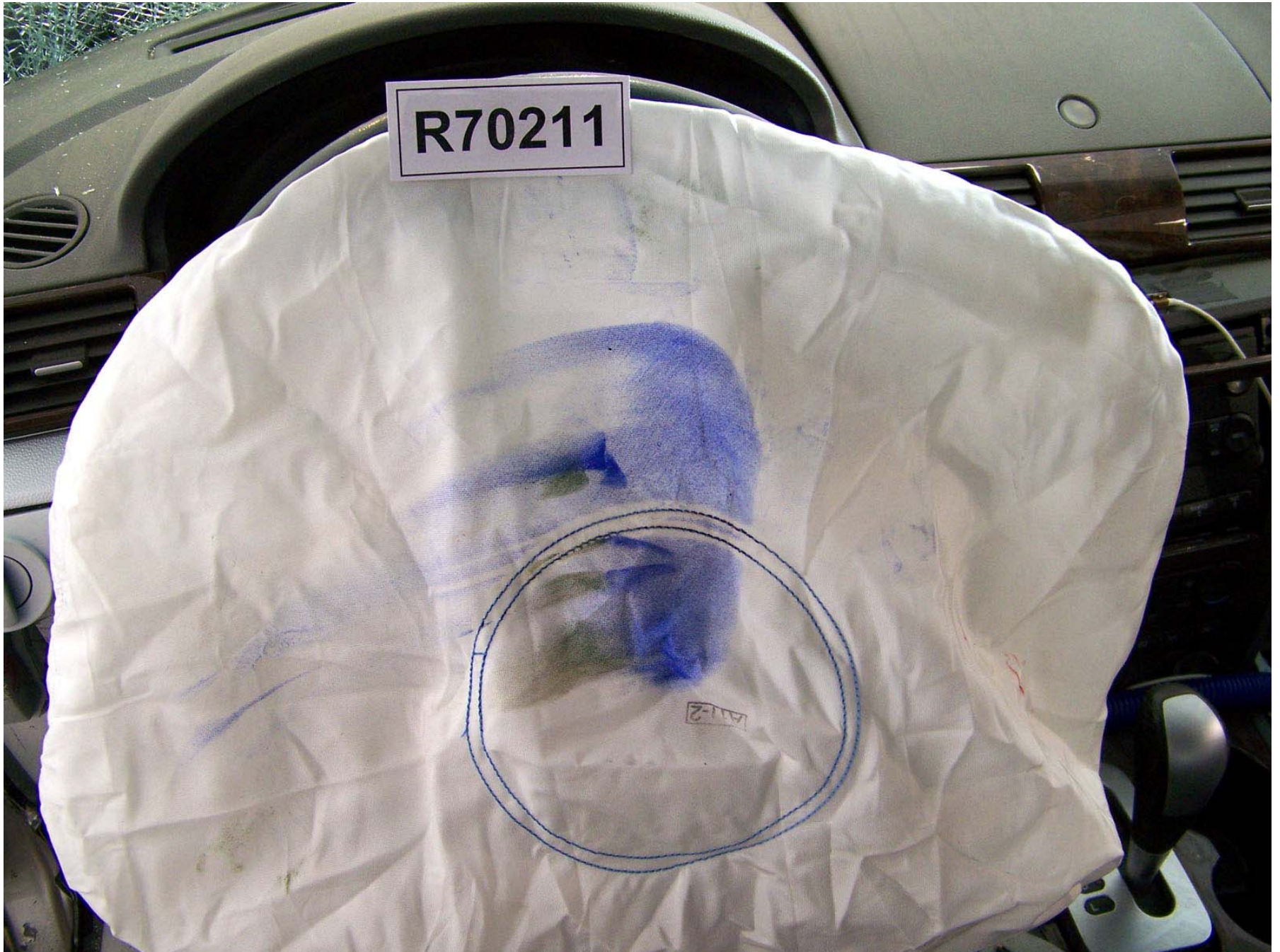
Figure A-282: Target Vehicle Post-Test Driver Dummy Contact, Airbag
