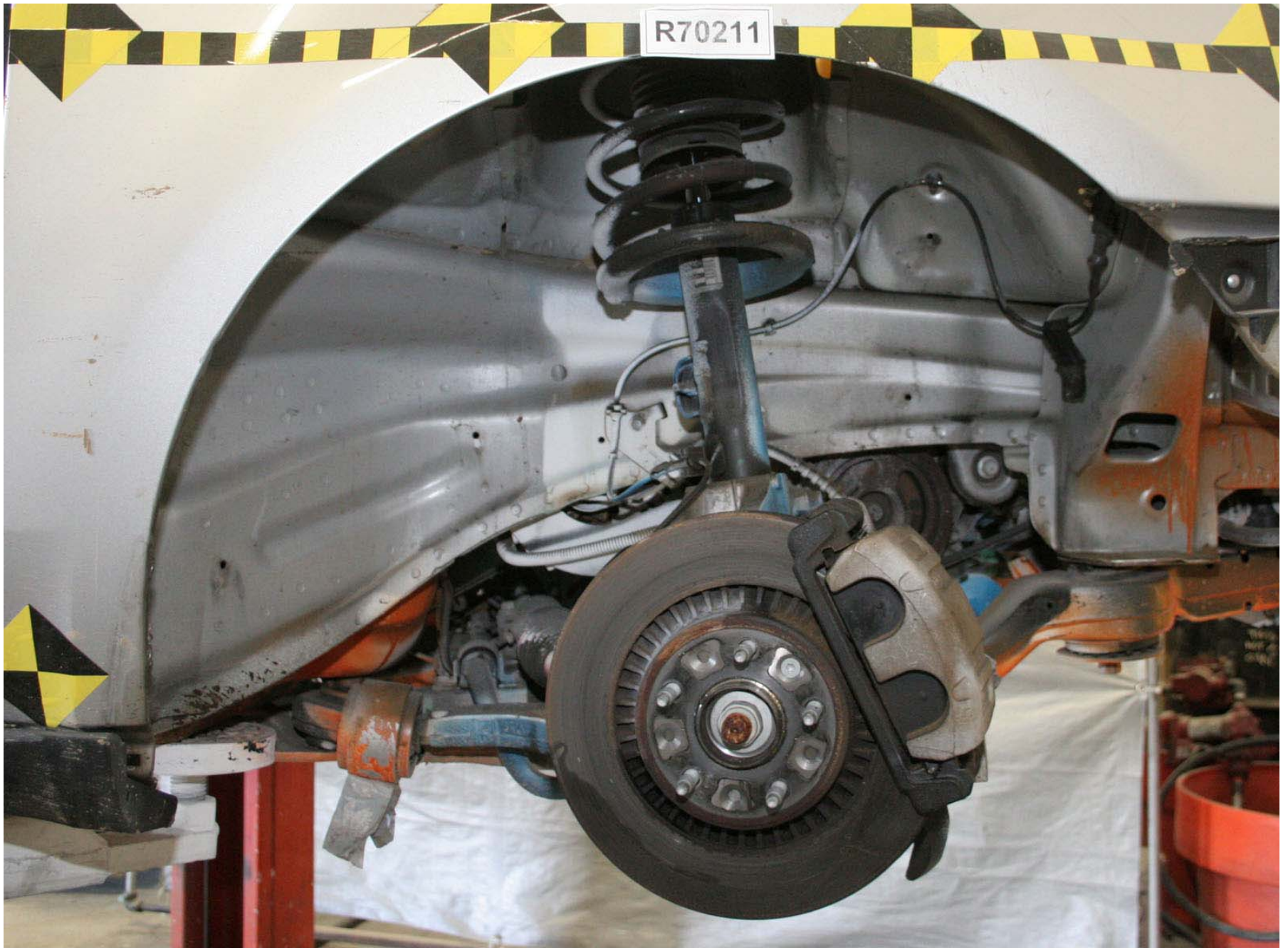
Figure A-204: Target Vehicle Post-Test Right Front Wheel Well (Tire Off), Inner Fender Removed
