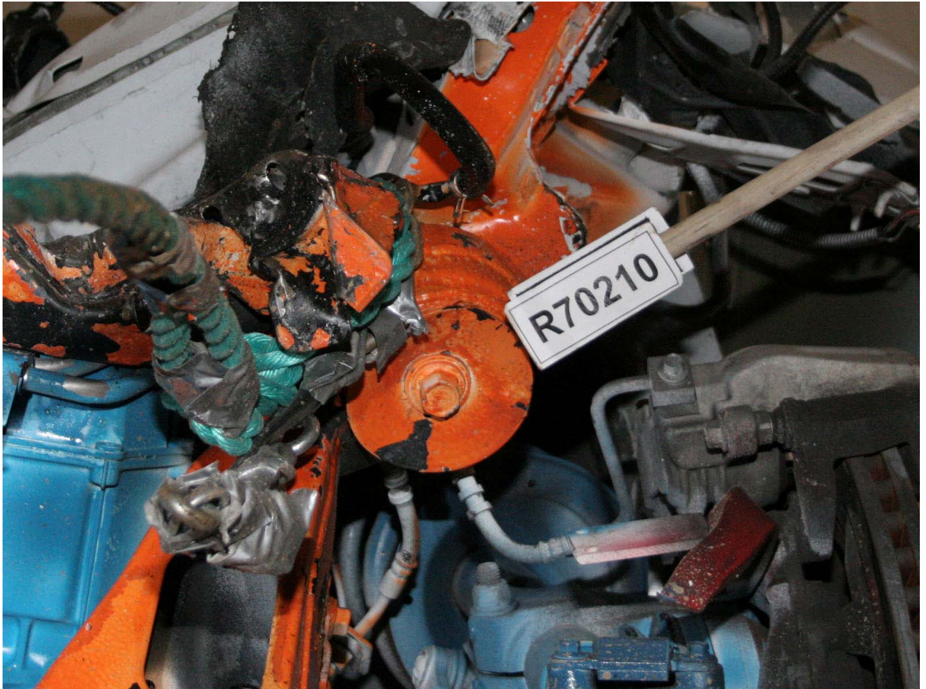
Figure A-483: Bullet Vehicle Post-Test Left Front Sub-Frame Mounting Point
