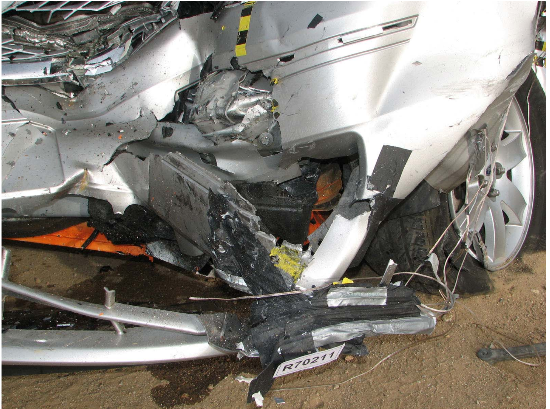
Figure A-48: Target Vehicle Post-Test Impact Point Marker
