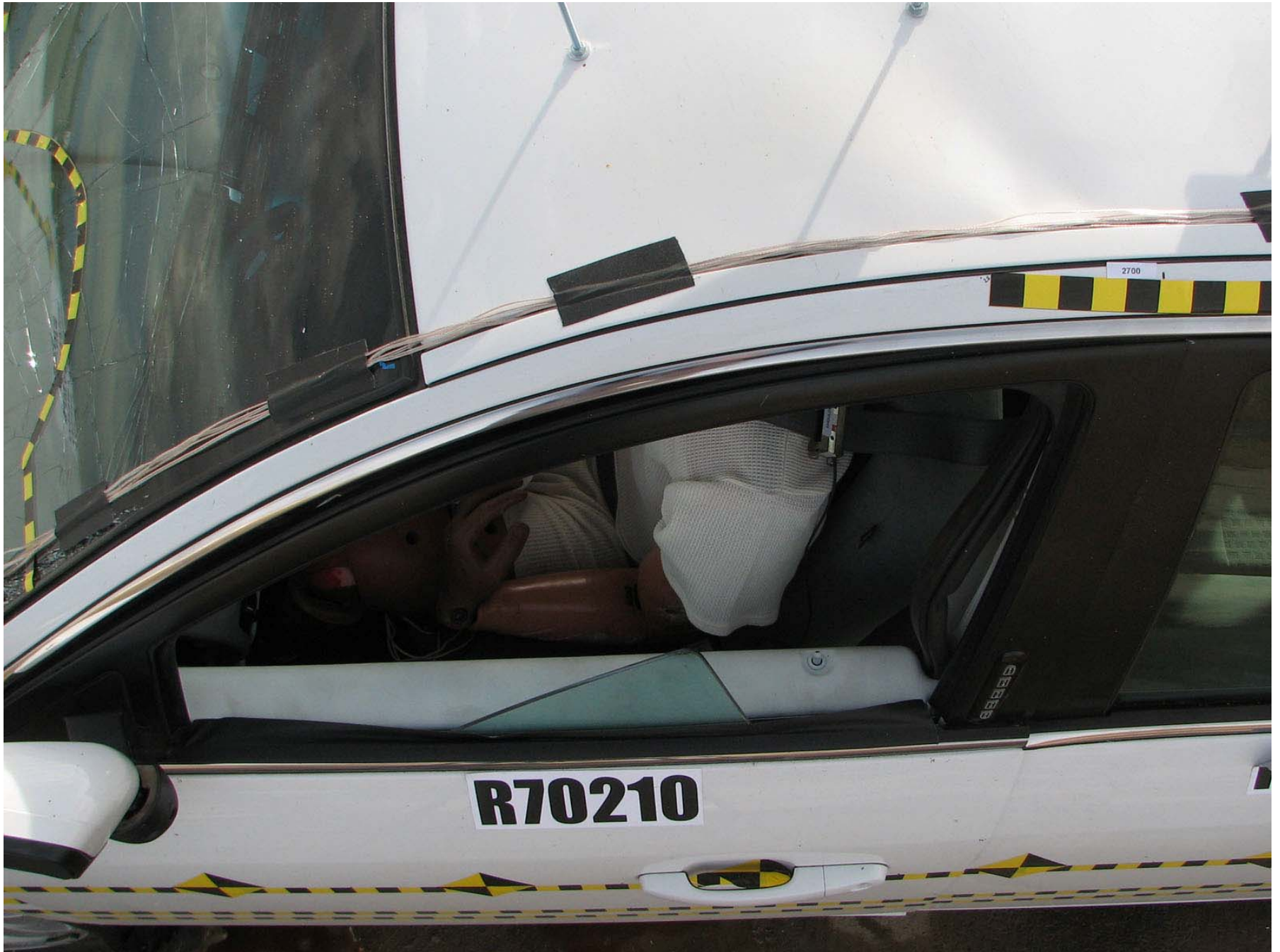
Figure A-559: Bullet Vehicle Post-Test Driver Dummy Clearance from Door
