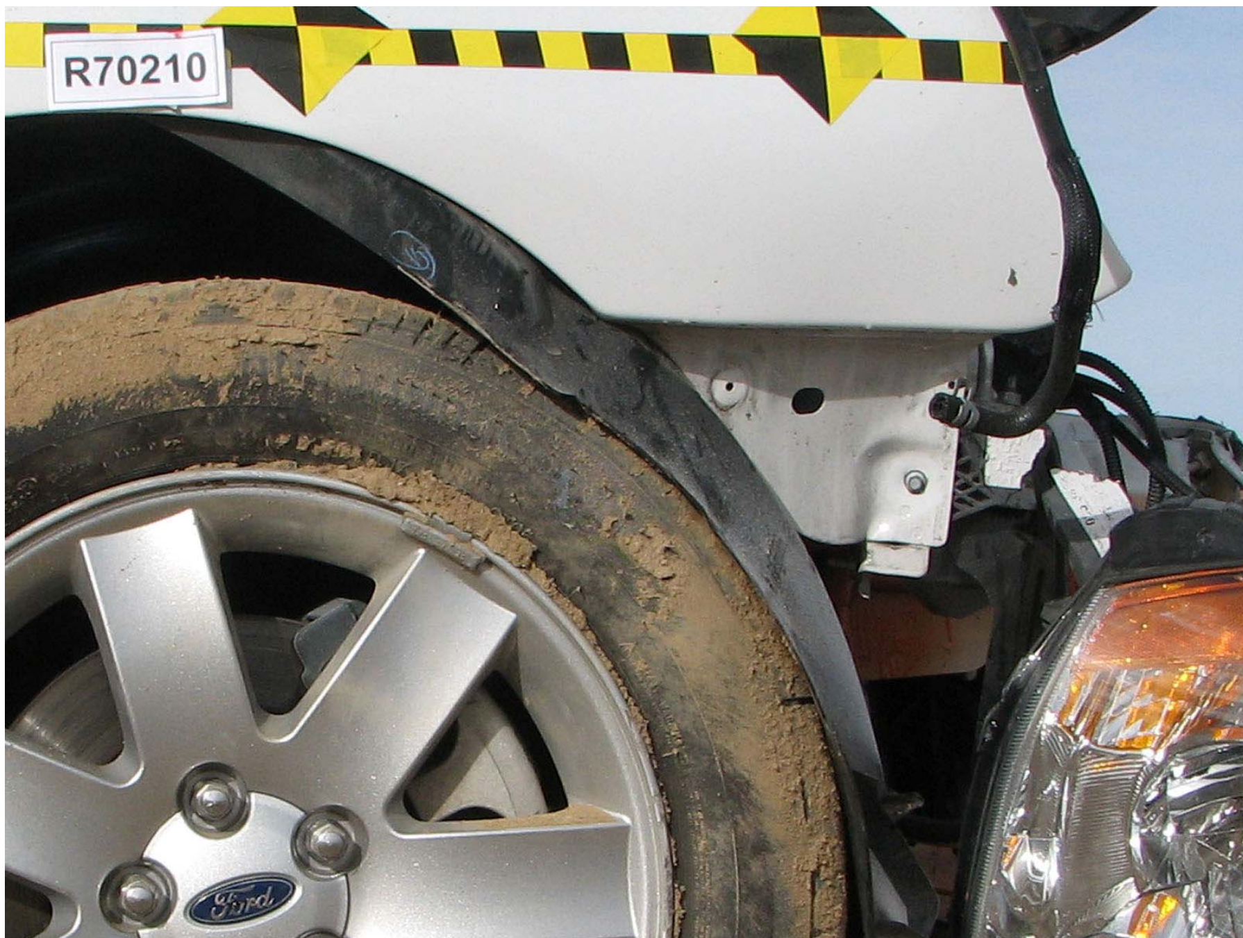
Figure A-445: Bullet Vehicle Post-Test Right Front Wheel A-Pillar/Rocker Contact
