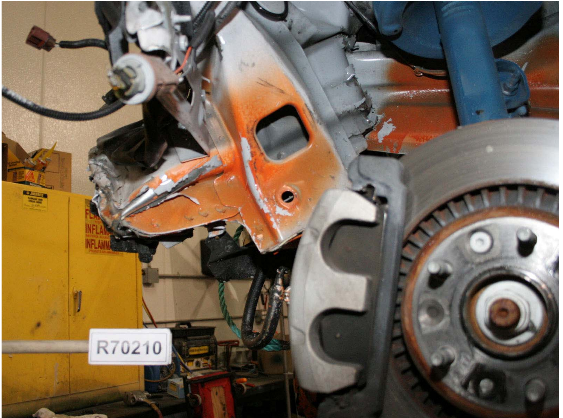
Figure A-477: Bullet Vehicle Post-Test Left Side Crush Initiators
