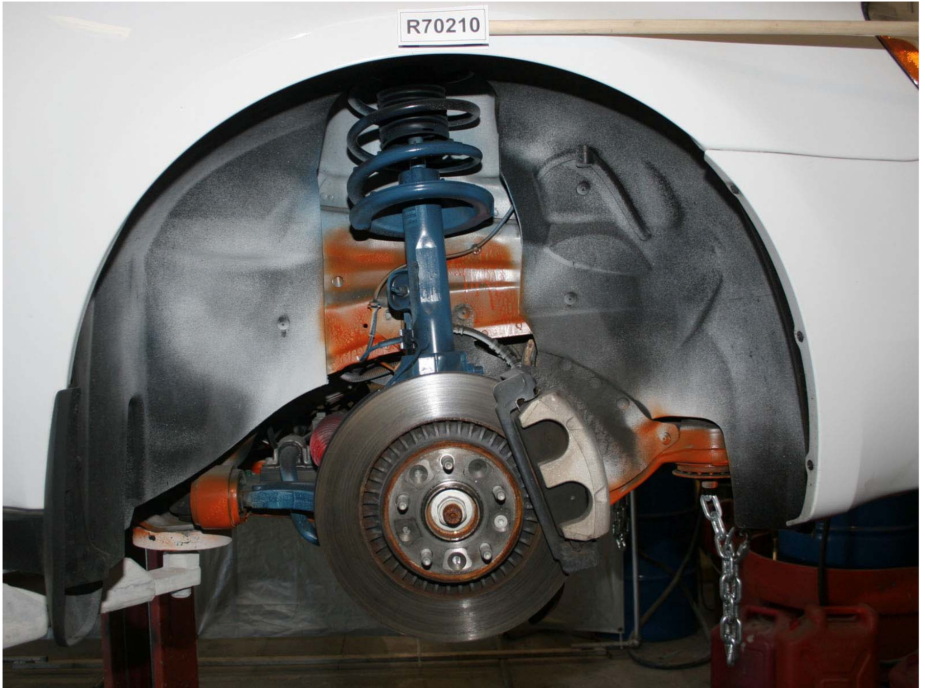
Figure A-488: Bullet Vehicle Pre-Test Right Front Wheel Well (Tire Off)
