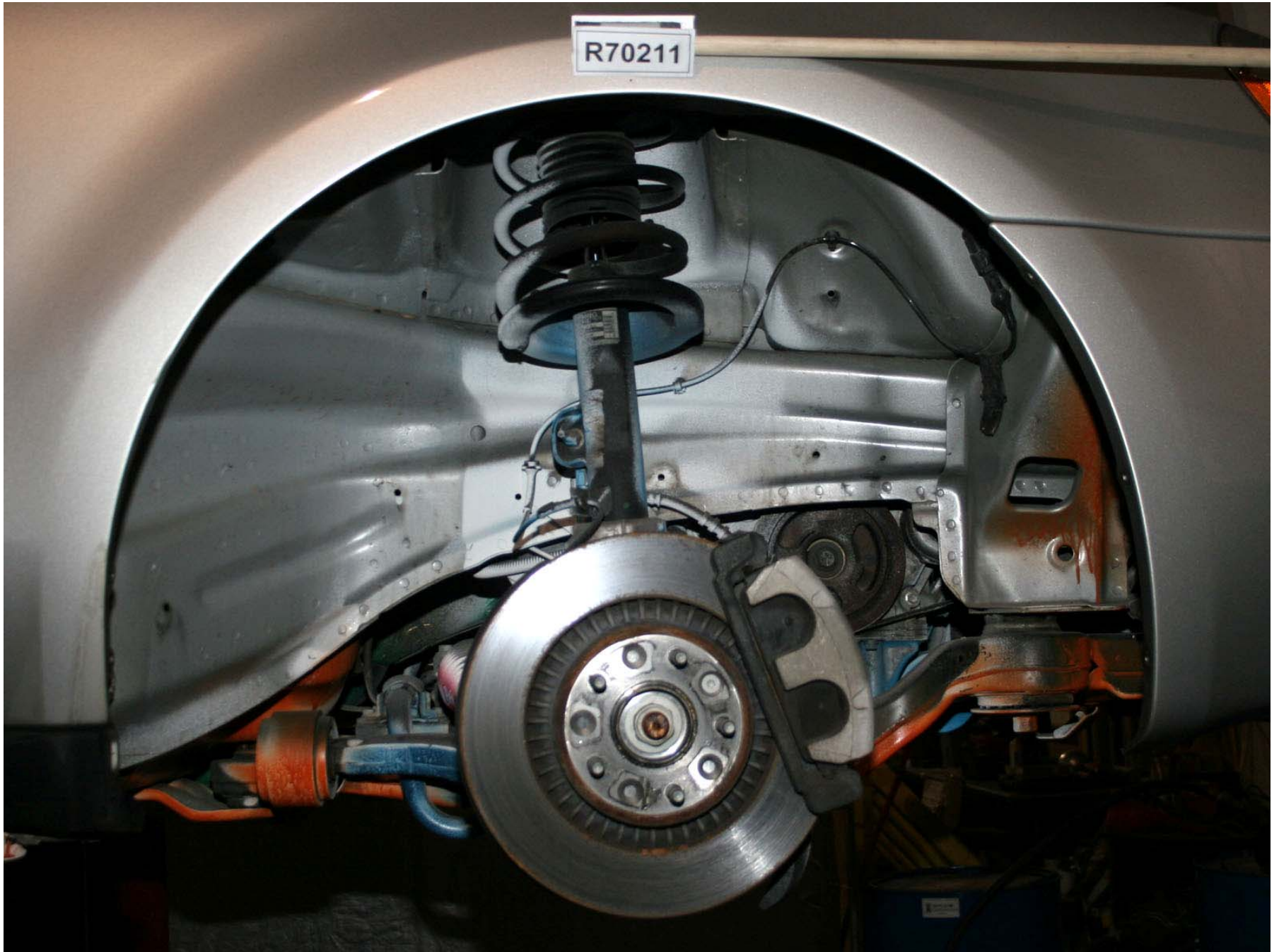
Figure A-203: Target Vehicle Pre-Test Right Front Wheel Well (Tire Off), Inner Fender Removed
