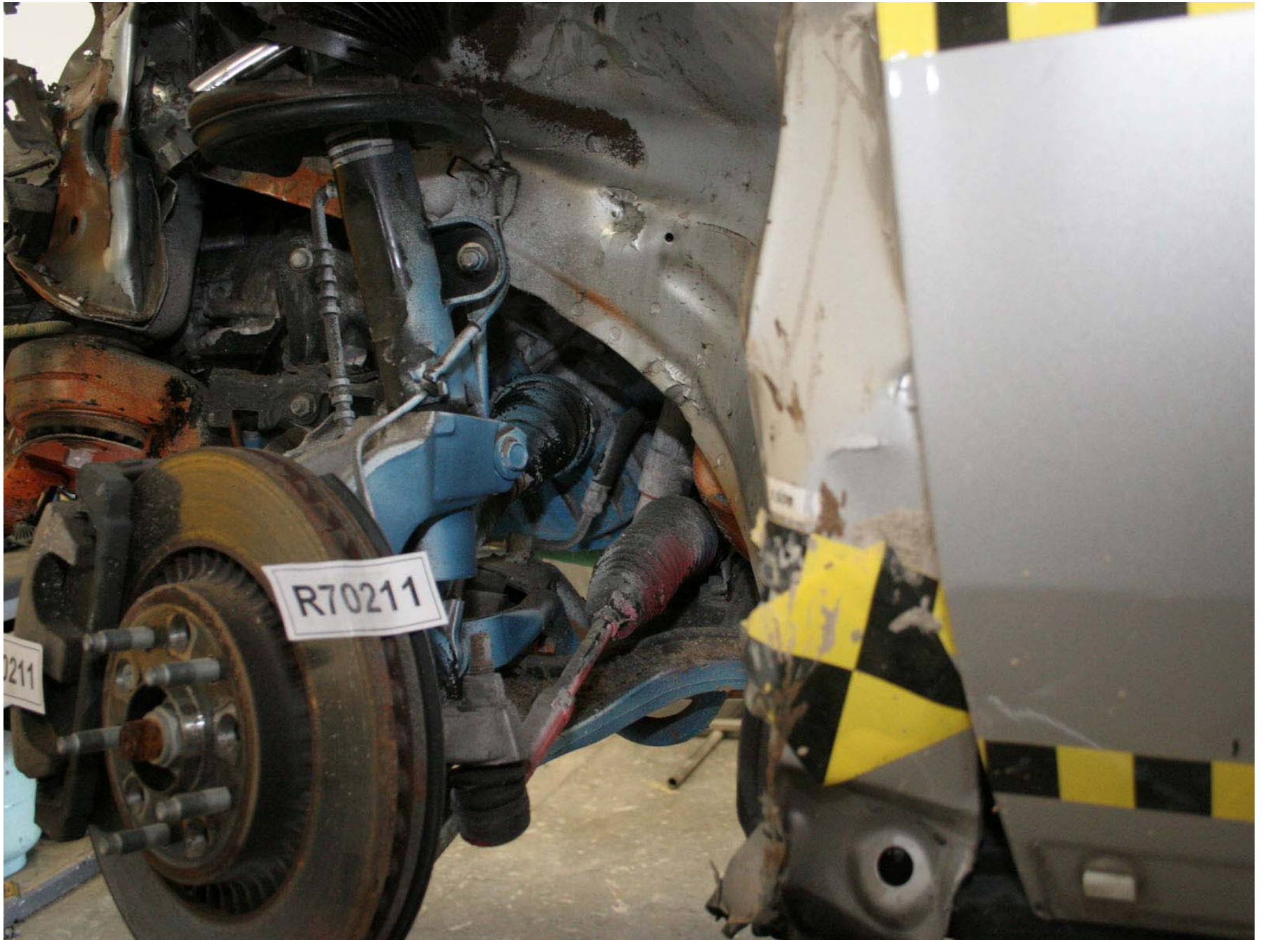
Figure A-184: Target Vehicle Post-Test Left Side Tie Rod and Sway Bar Attachments Points
