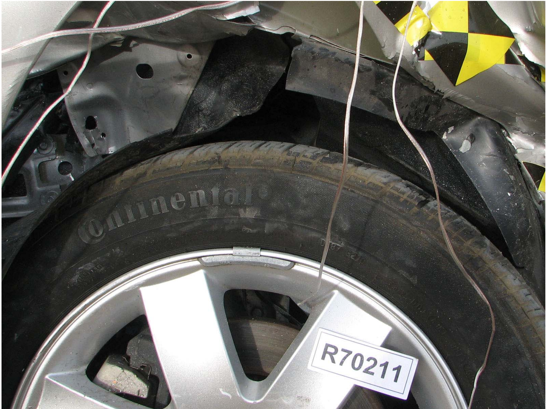
Figure A-146: Target Vehicle Post-Test Left Front Wheel A-Pillar/Rocker Contact
