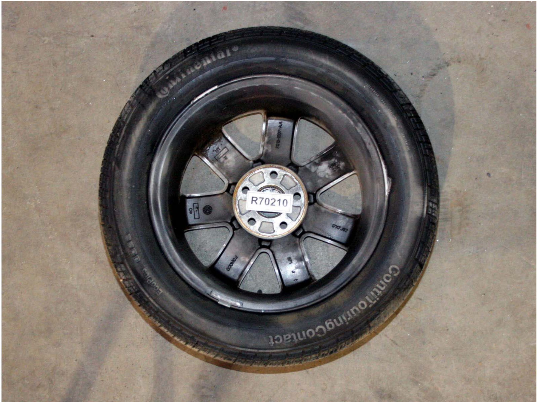
Figure A-449: Bullet Vehicle Post-Test Right Front Wheel Damage (Inside)
