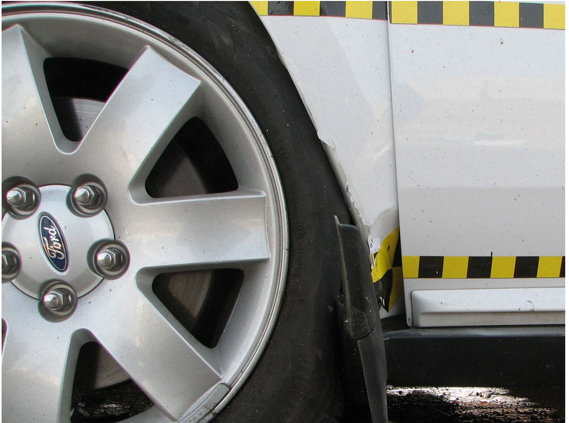
Figure A-434: Bullet Vehicle Post-Test Left Front Wheel A-Pillar/Rocker Contact
