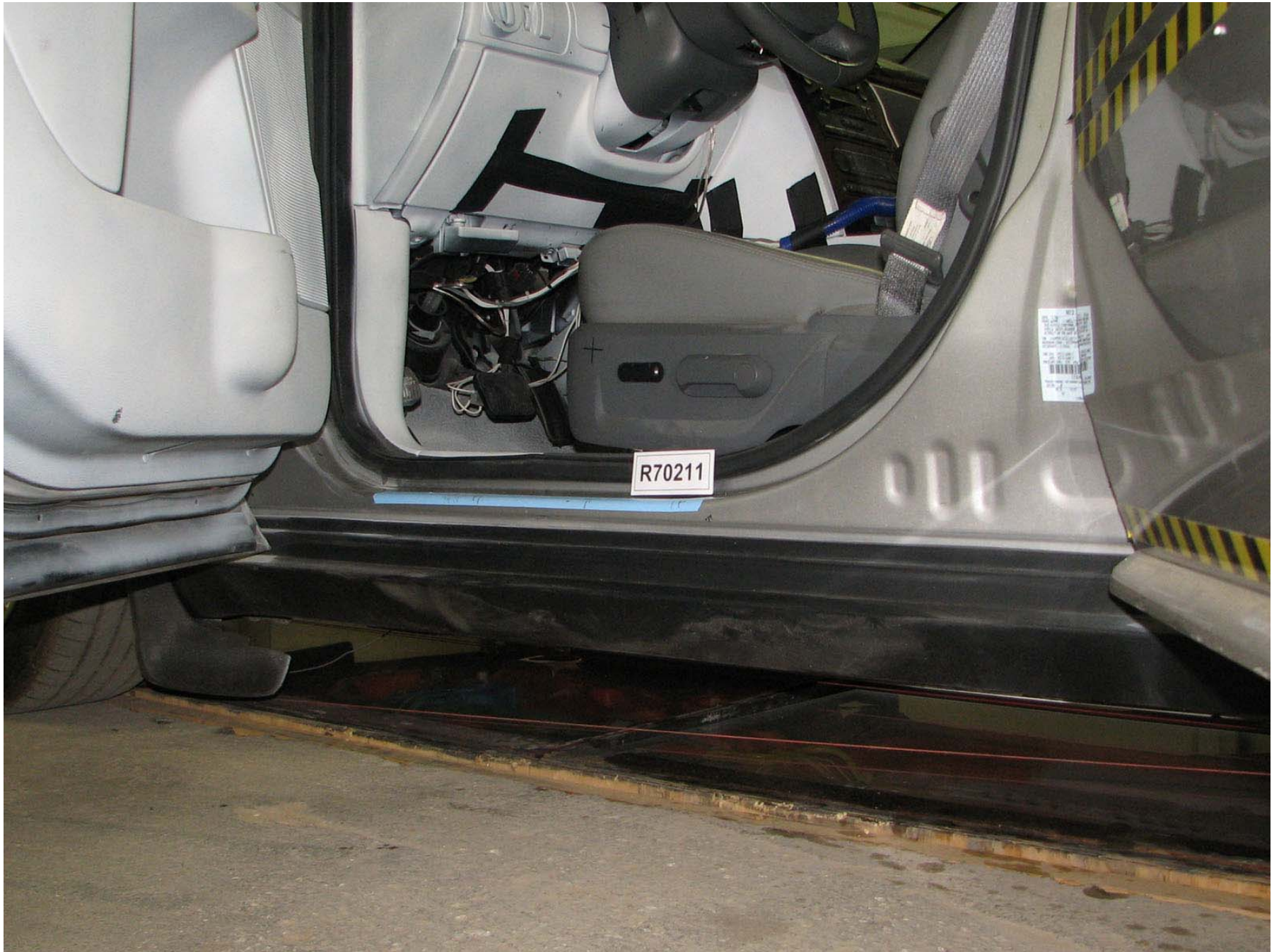
Figure A-99: Target Vehicle Pre-Test Left Front Sill Rear ¾ View, Door Open
