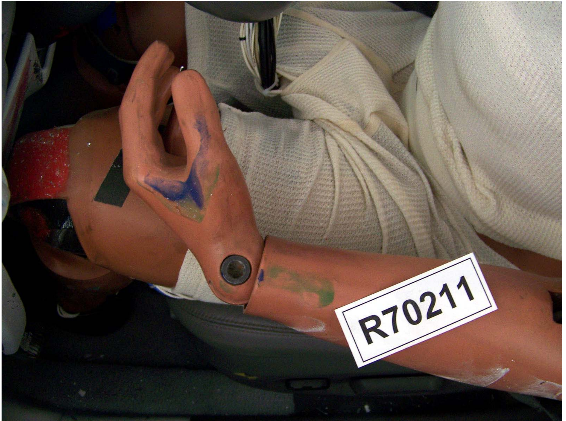
Figure A-285: Target Vehicle Post-Test Driver Dummy Contact, Left Arm
