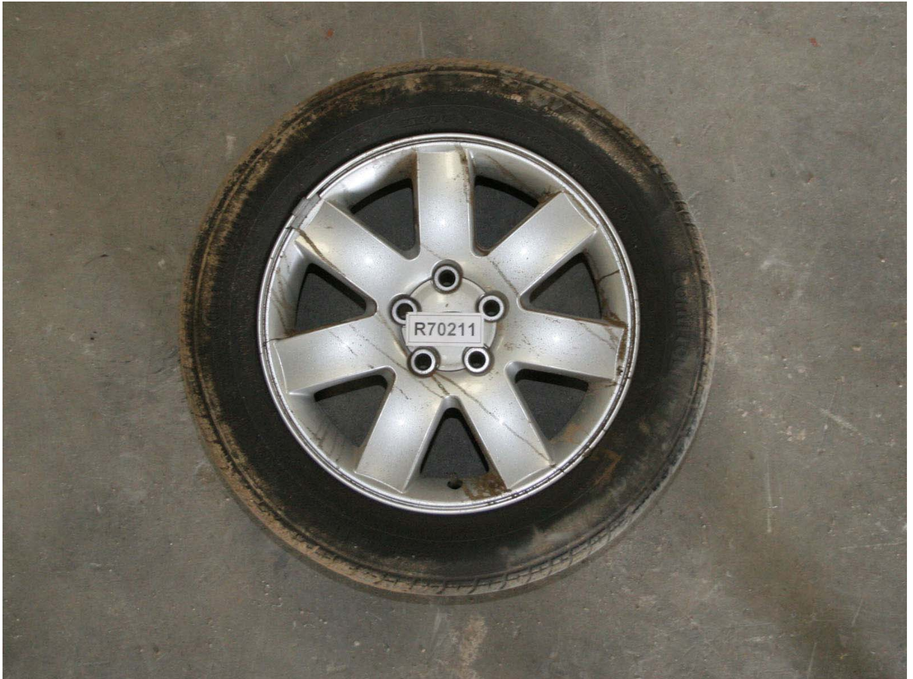
Figure A-161: Target Vehicle Post-Test Right Front Wheel Damage (Outside)
