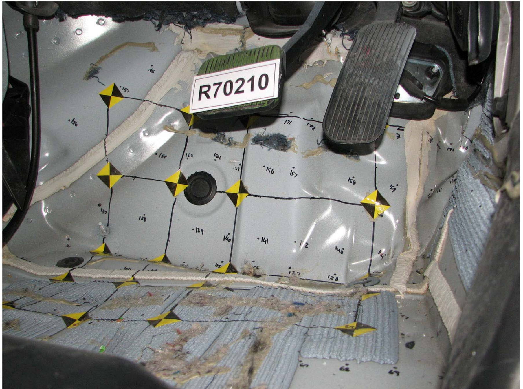
Figure A-585: Bullet Vehicle Post-Test Driver Floorpan Right ¾ View, Sill Height
