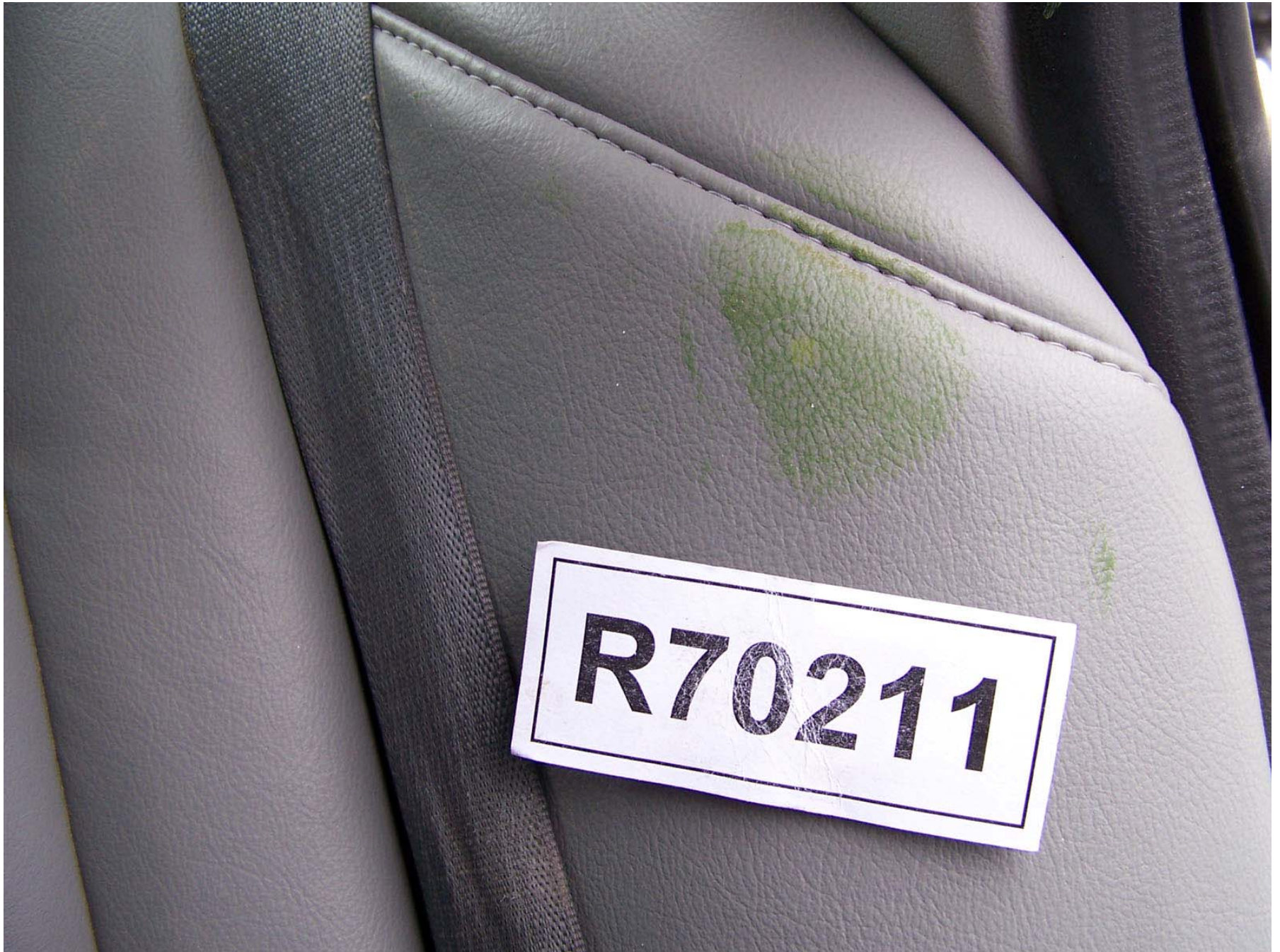
Figure A-312: Target Vehicle Post-Test Passenger Dummy Contact, Seat Back
