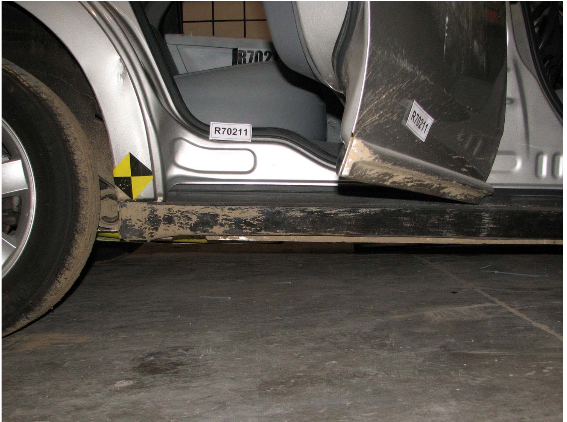
Figure A-132: Target Vehicle Post-Test Right Rear Sill Side View, Door Open
