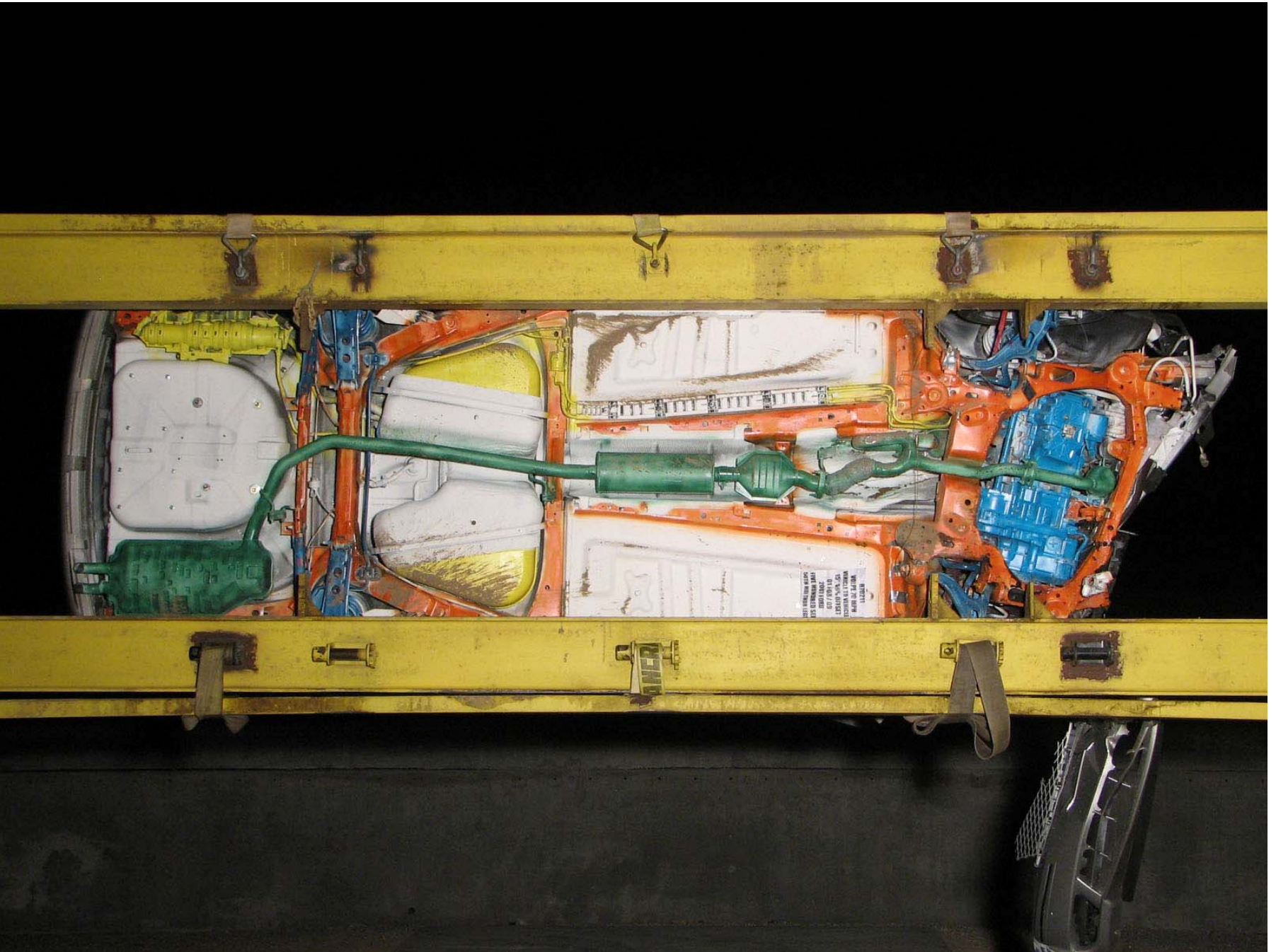
Figure A-607: Target Vehicle on Rollover Device (270°)
