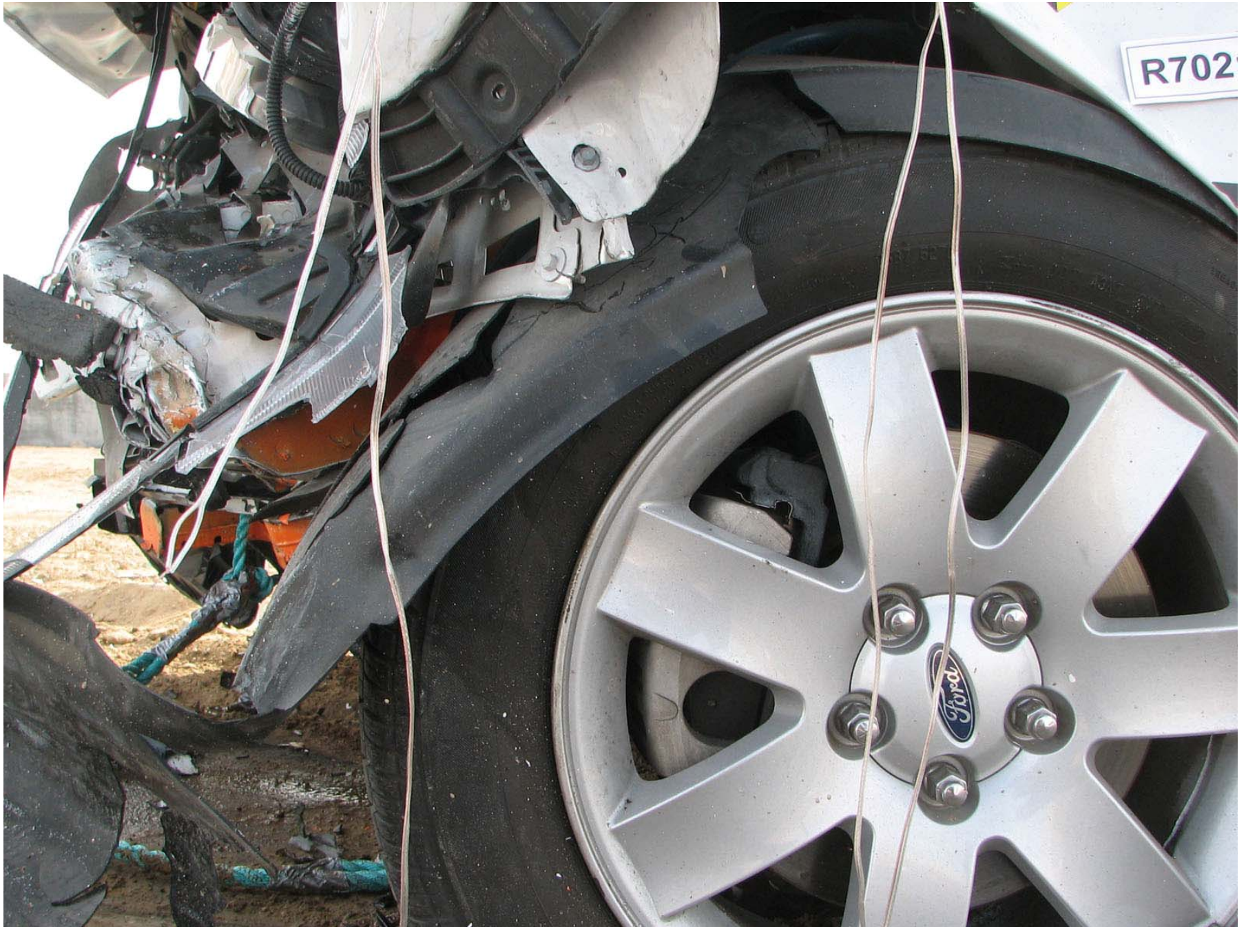
Figure A-432: Bullet Vehicle Post-Test Left Front Wheel A-Pillar/Rocker Contact
