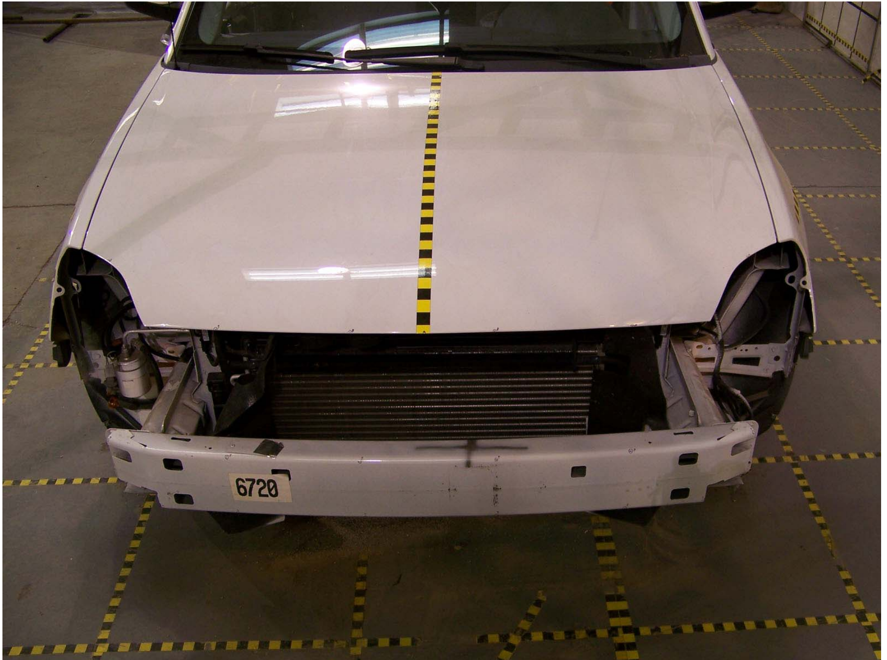
Figure A-598: Bullet Vehicle Pre-Test Structural Member Crush Measurement
