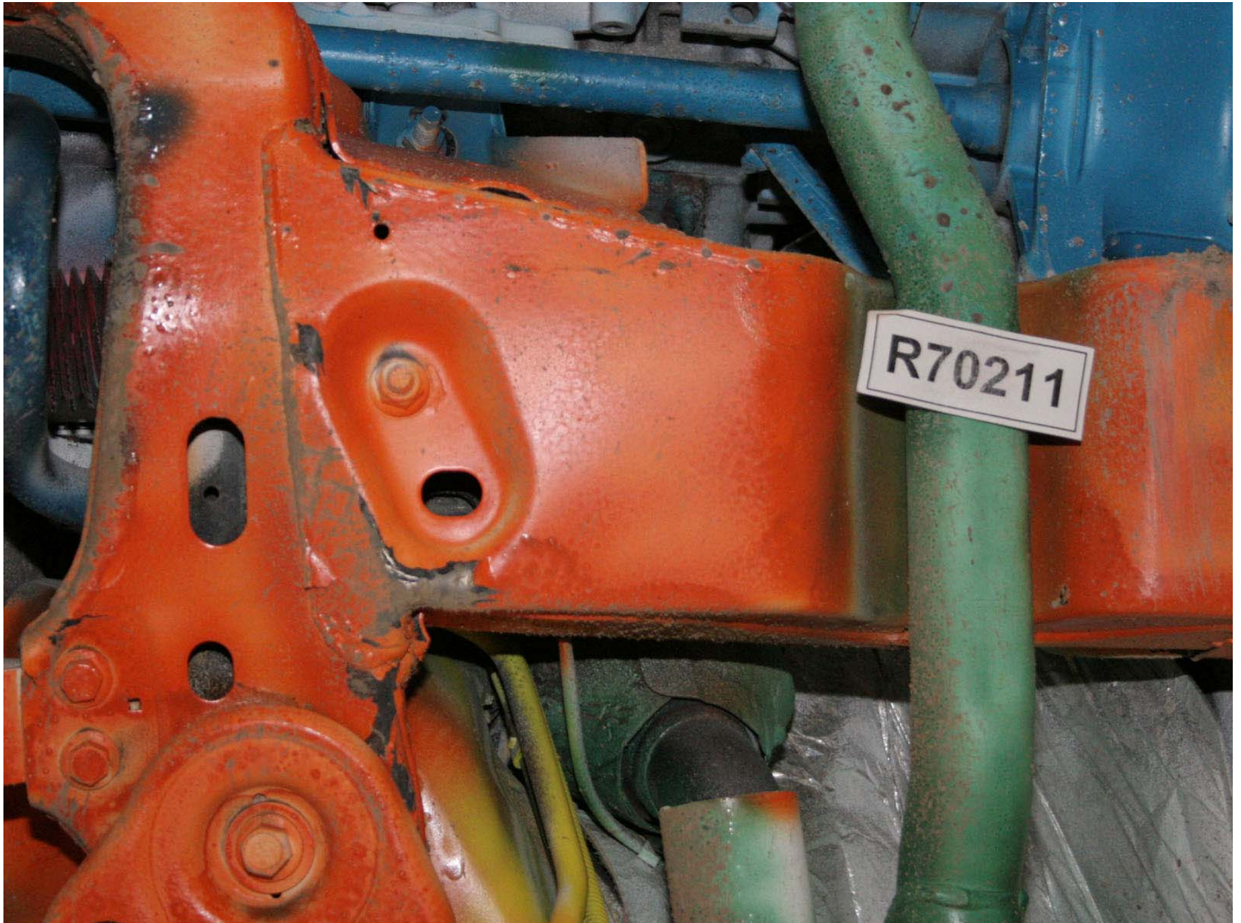
Figure A-246: Target Vehicle Post-Test Steering Rack Right Side Mounting Bolt
