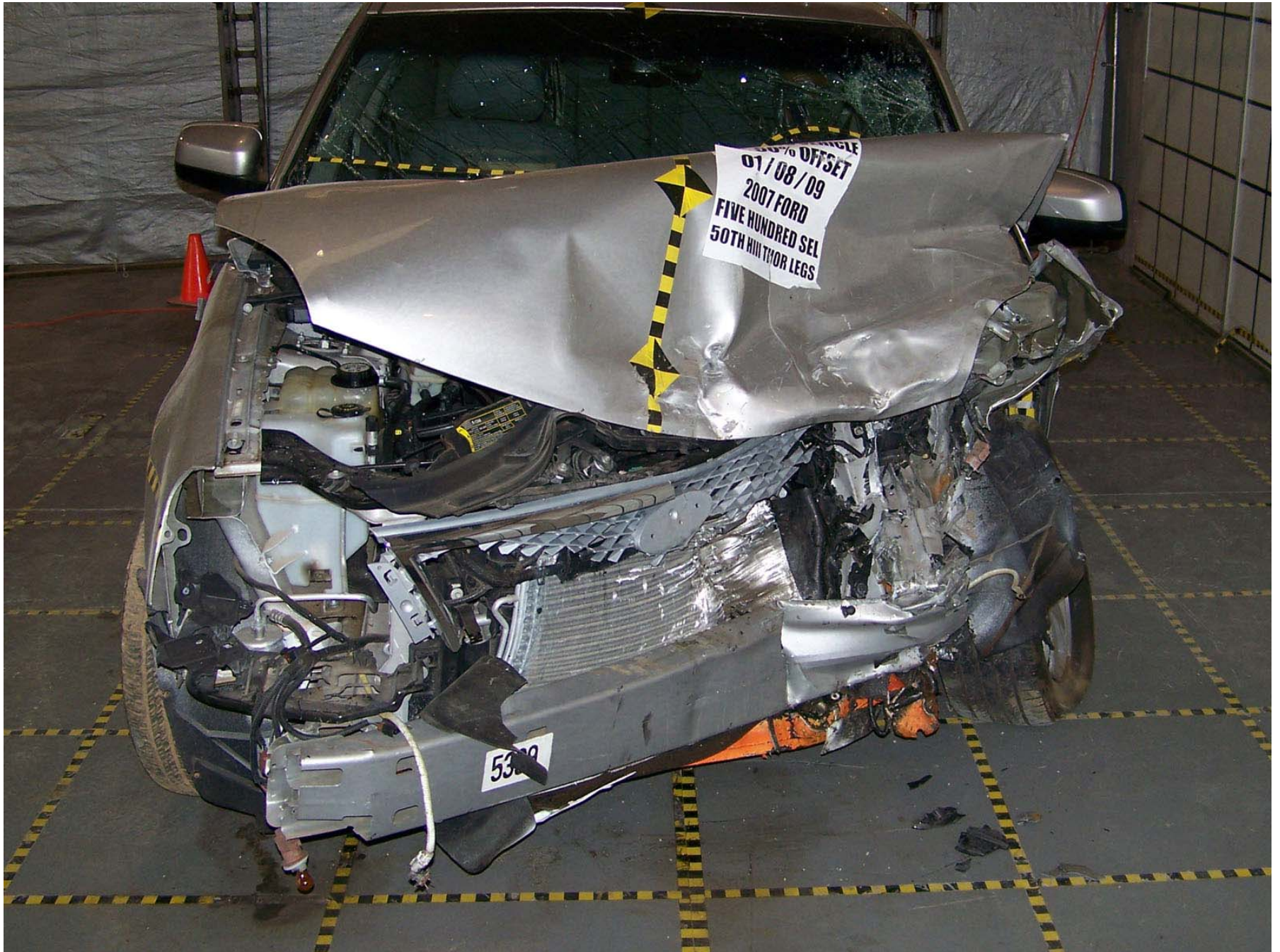
Figure A-341: Target Vehicle Post-Test Structural Member Crush Measurement
