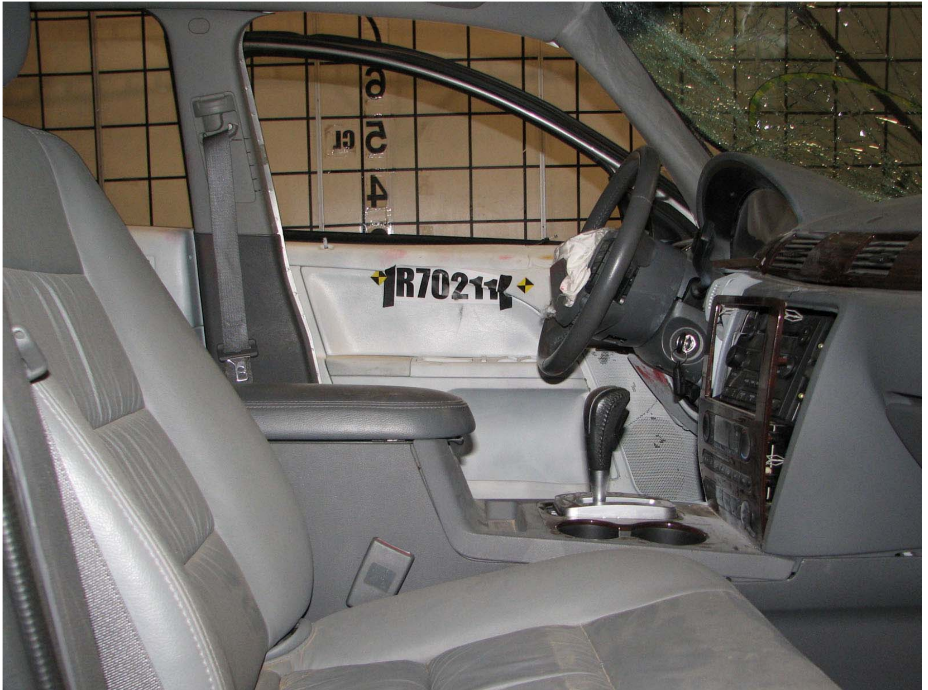
Figure A-252: Test Vehicle Post-Test Front Door Panel
