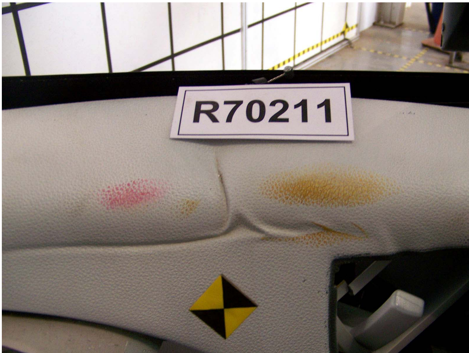
Figure A-286: Target Vehicle Post-Test Driver Dummy Contact, Door Panel
