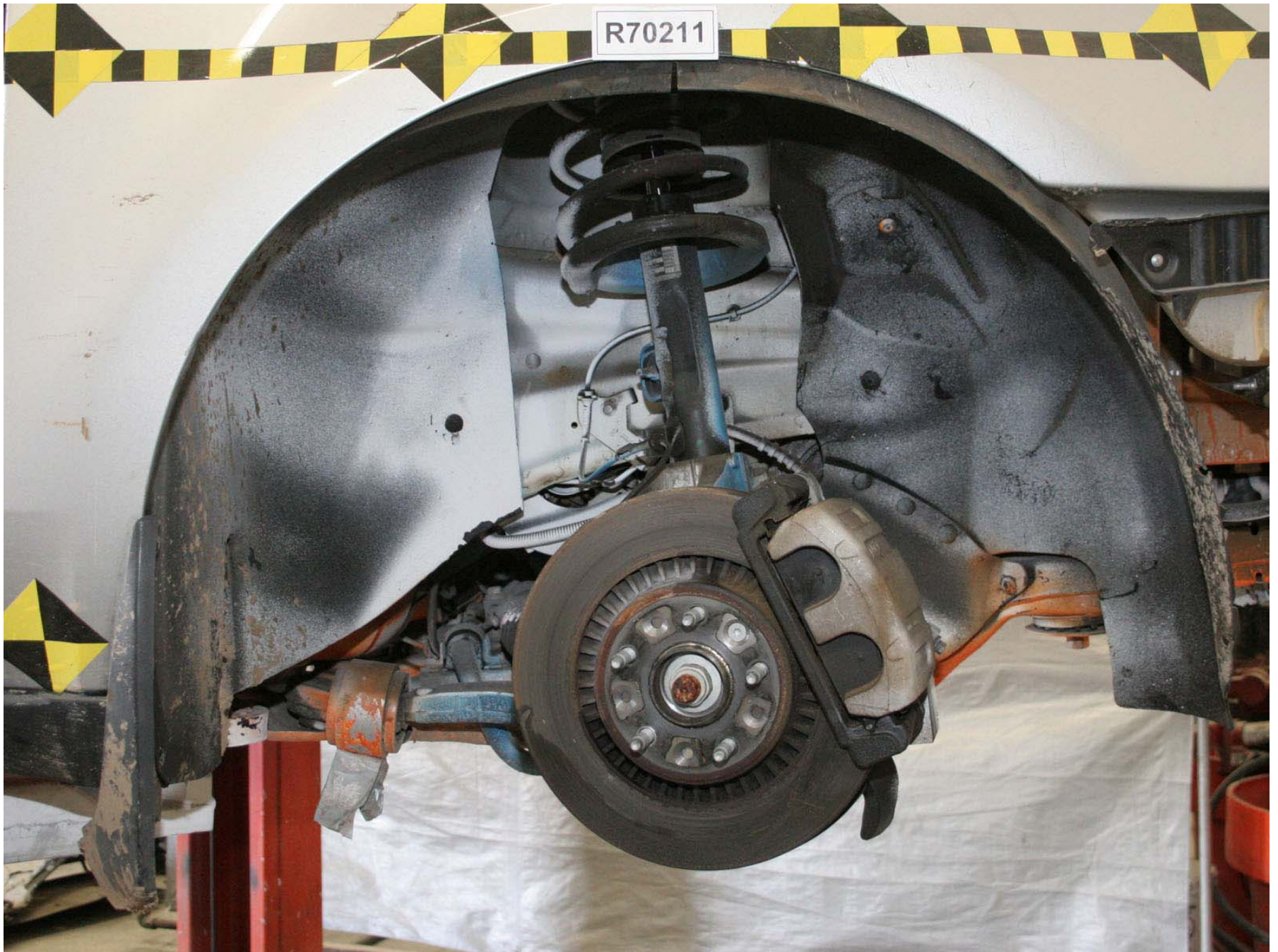
Figure A-202: Target Vehicle Post-Test Right Front Wheel Well (Tire Off)
