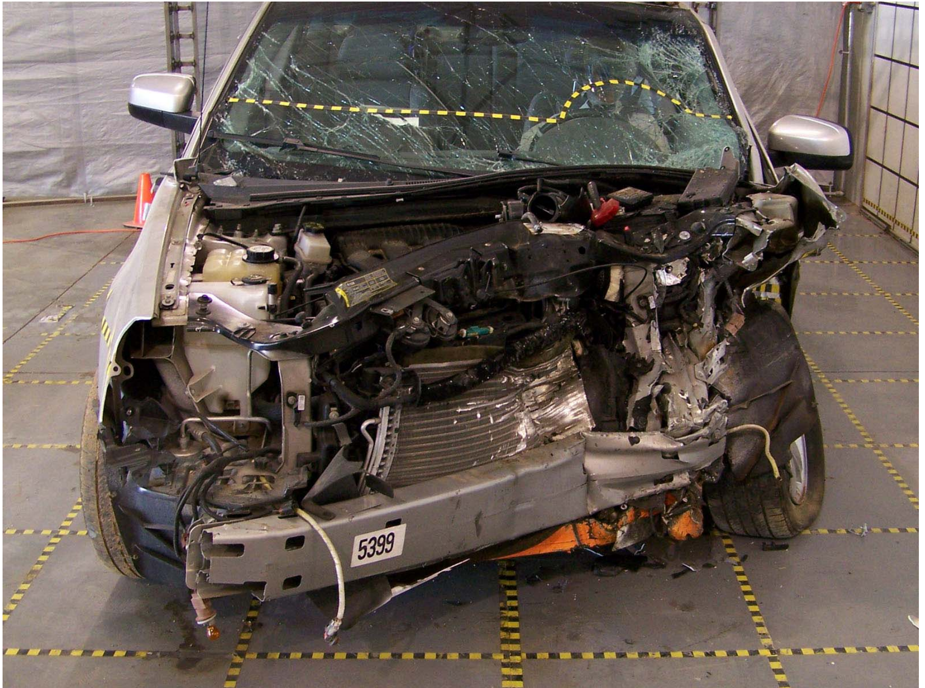
Figure A-345: Target Vehicle Pre-Test Structural Member Crush Measurement
