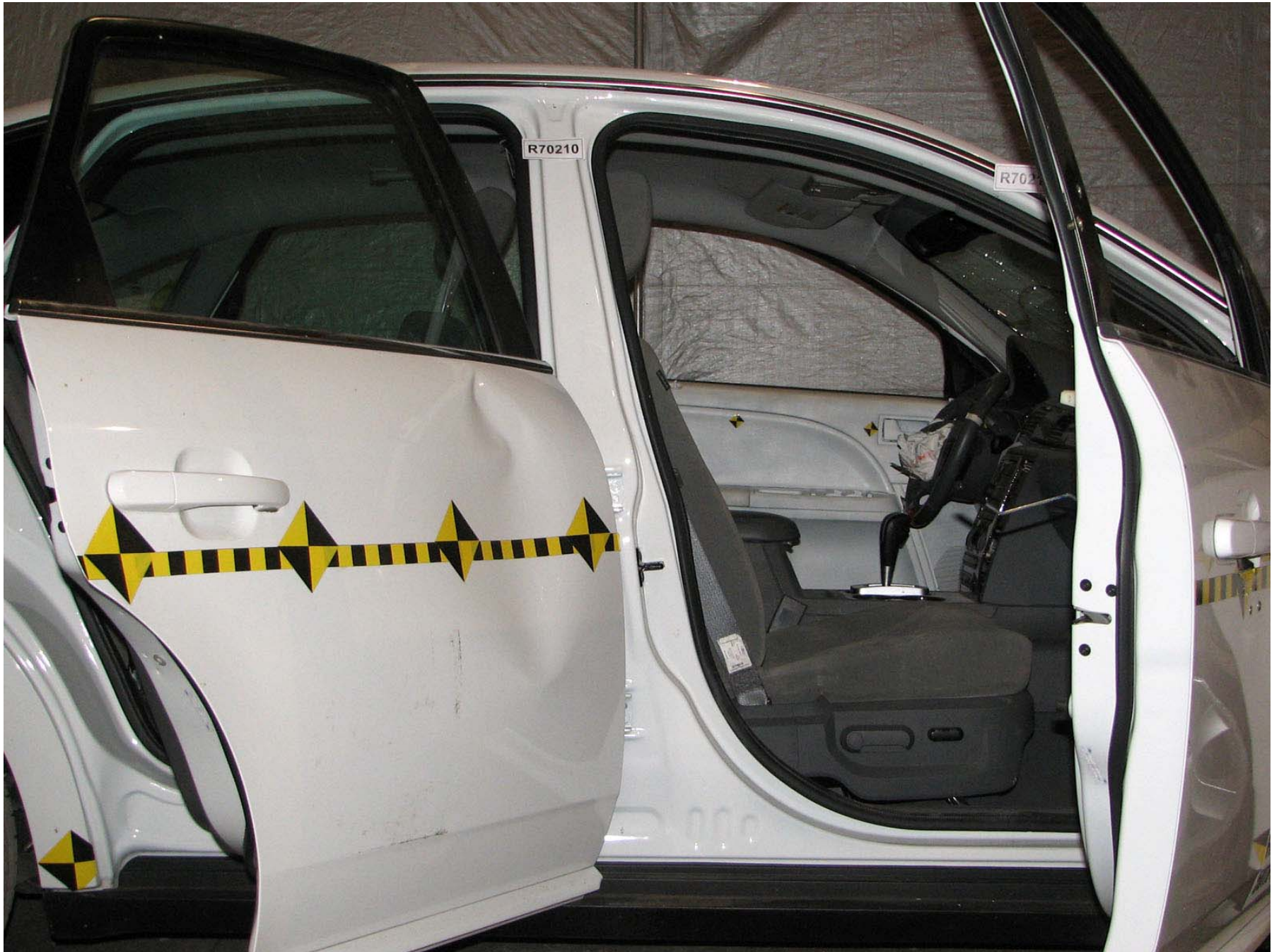
Figure A-401: Bullet Vehicle Post-Test Right Side B-Pillar Side View
