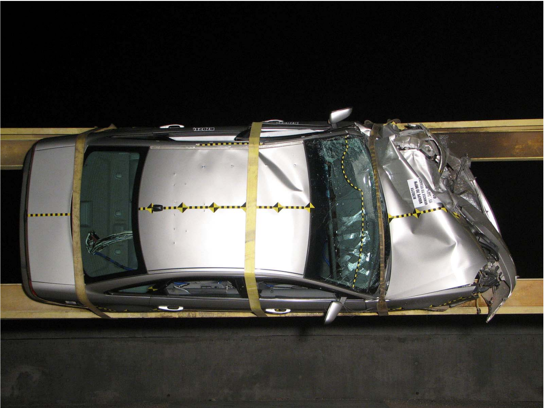
Figure A-605: Target Vehicle on Rollover Device (90°)
