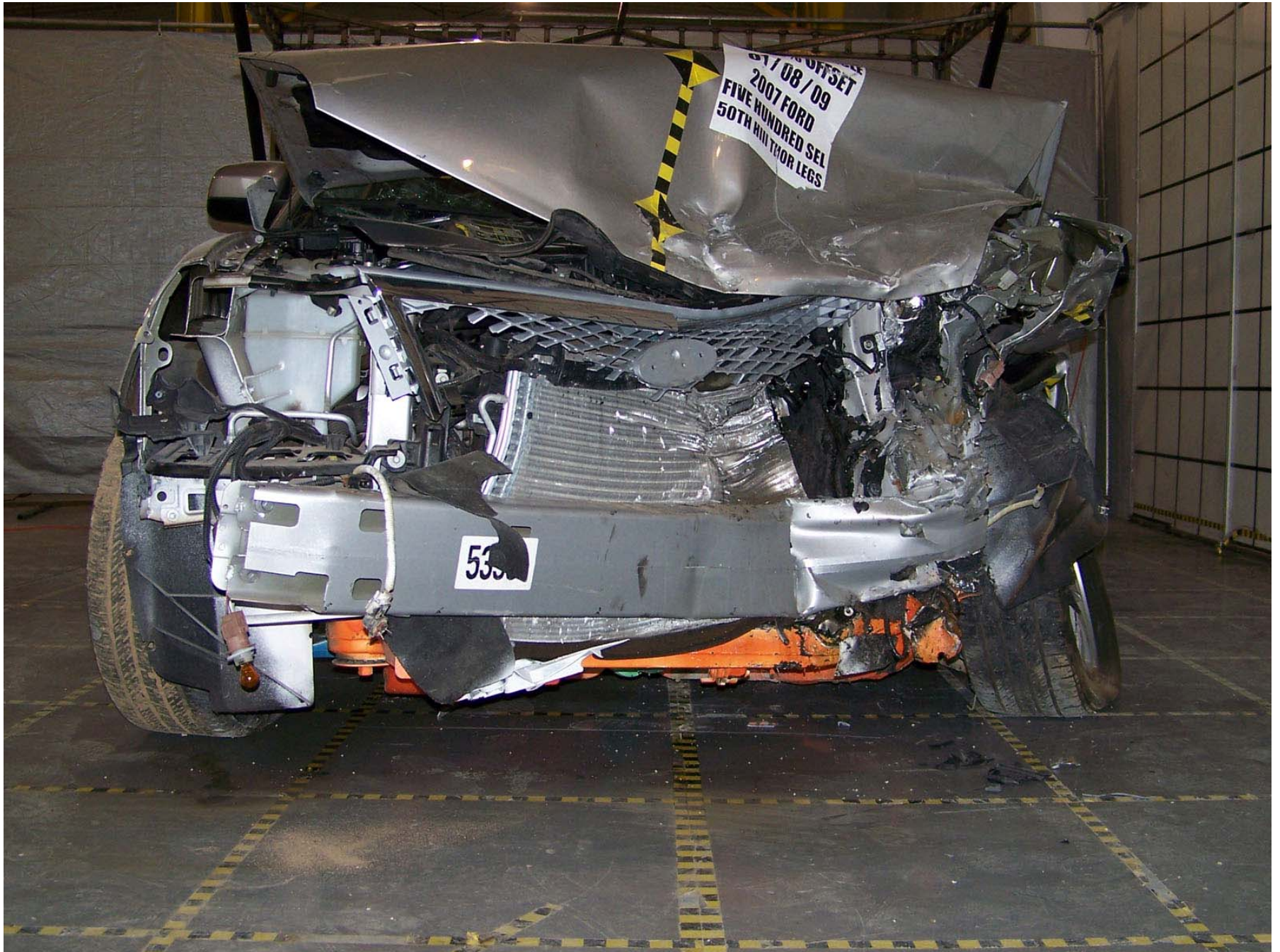
Figure A-339: Target Vehicle Post-Test Structural Member Crush Measurement
