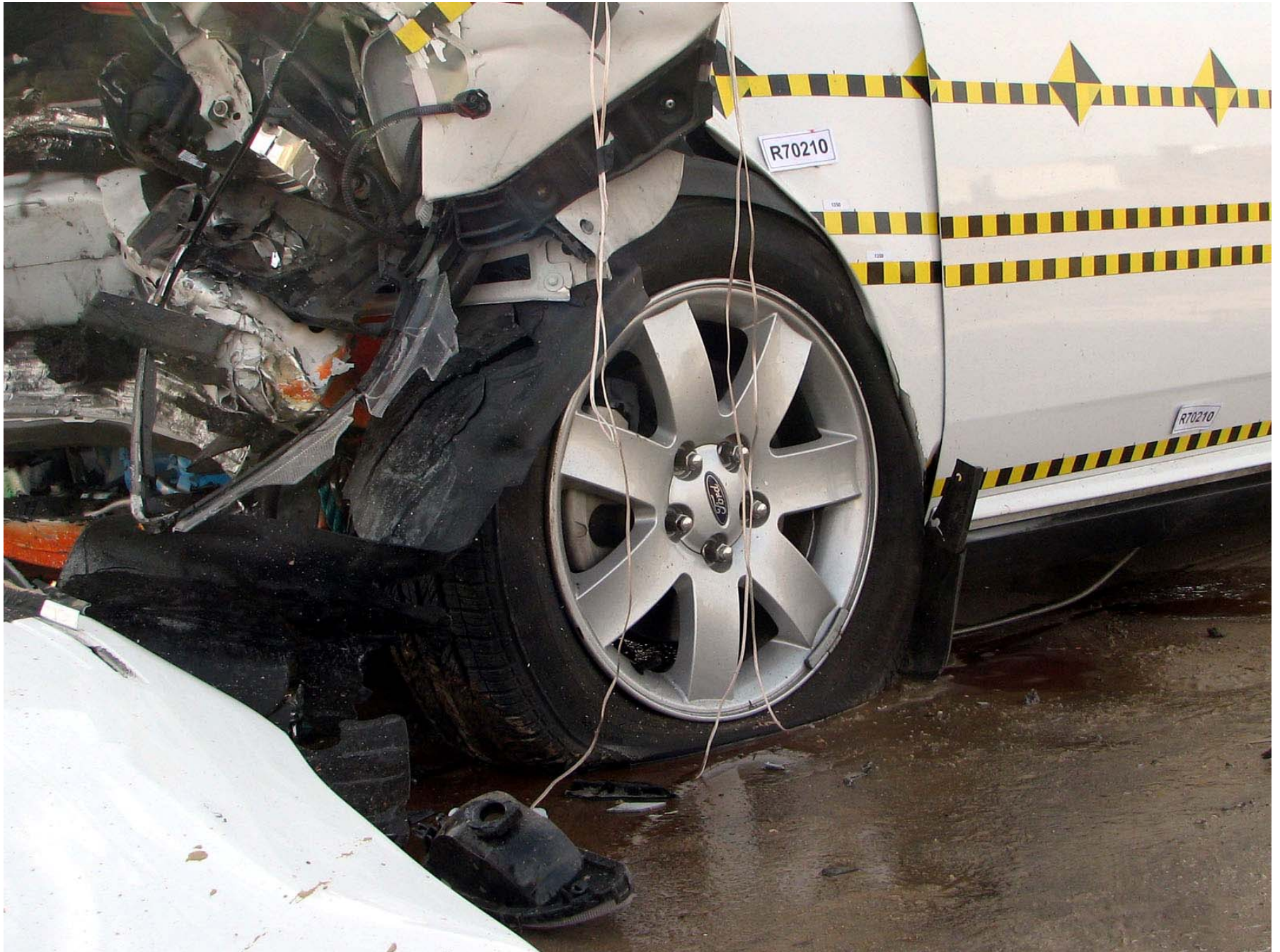
Figure A-427: Bullet Vehicle Post-Test Left Front Wheel Front \frac{3}{4} View
