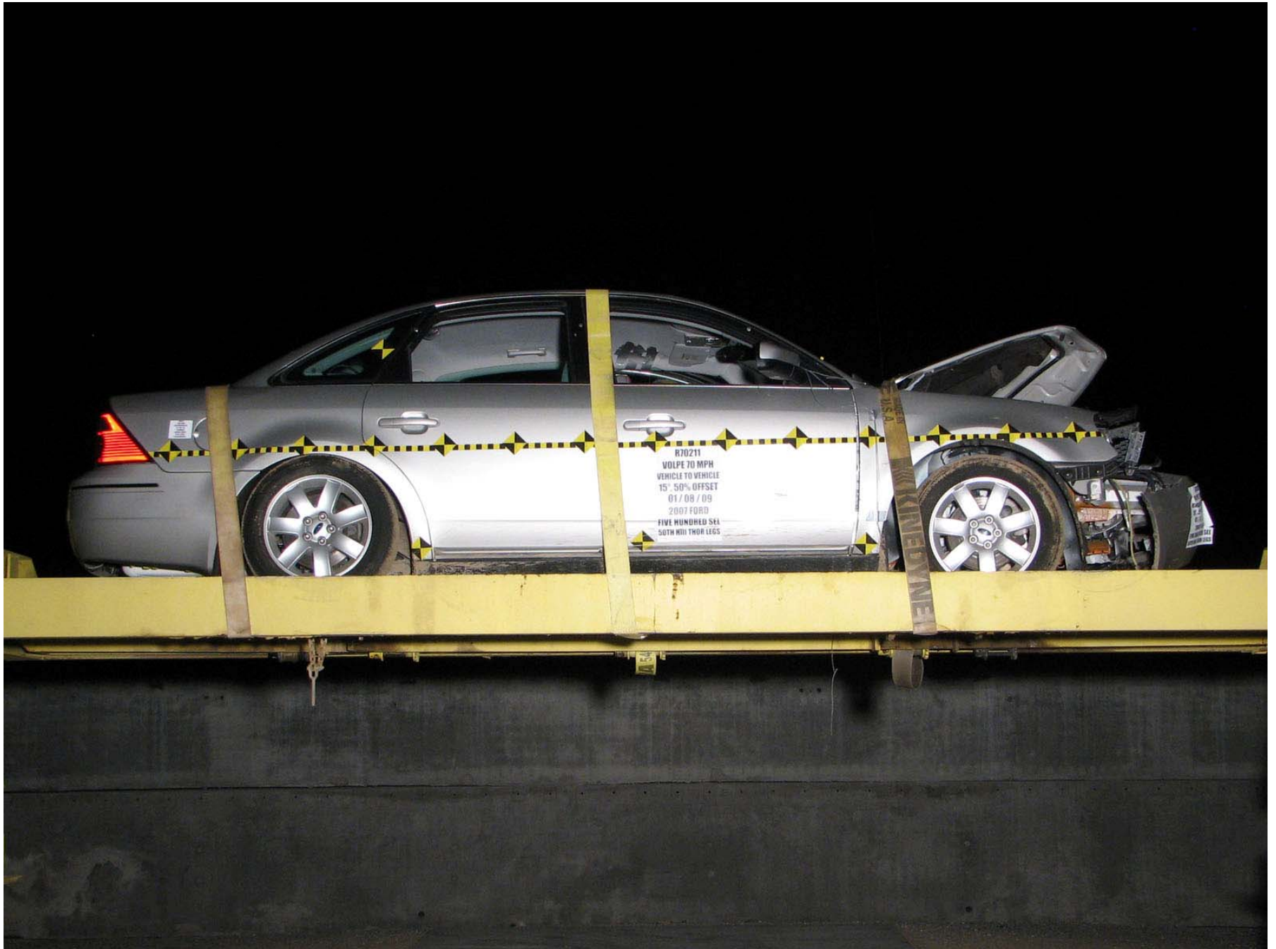
Figure A-604: Target Vehicle on Rollover Device (0°)
