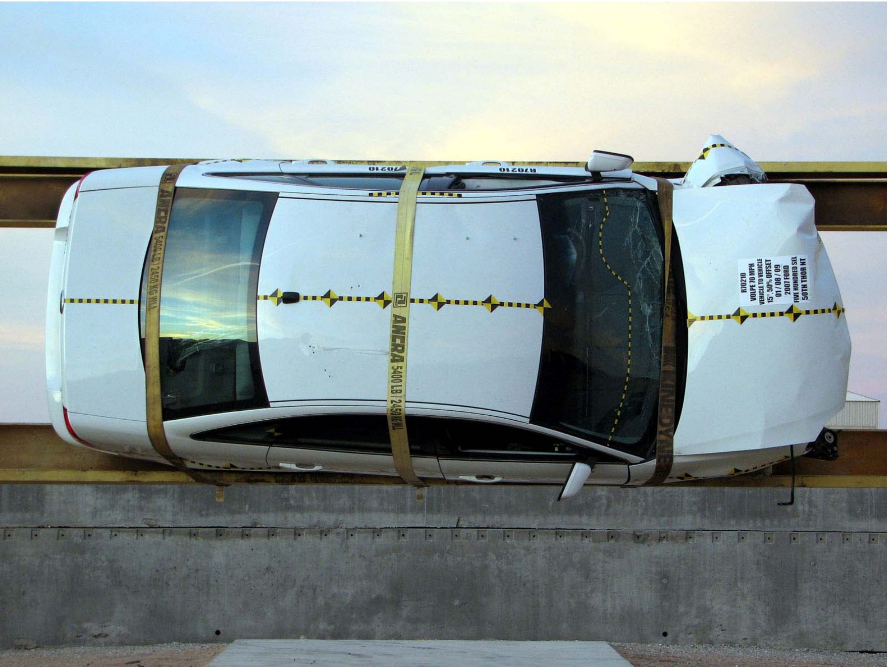
Figure A-610: Bullet Vehicle on Rollover Device (90°)
