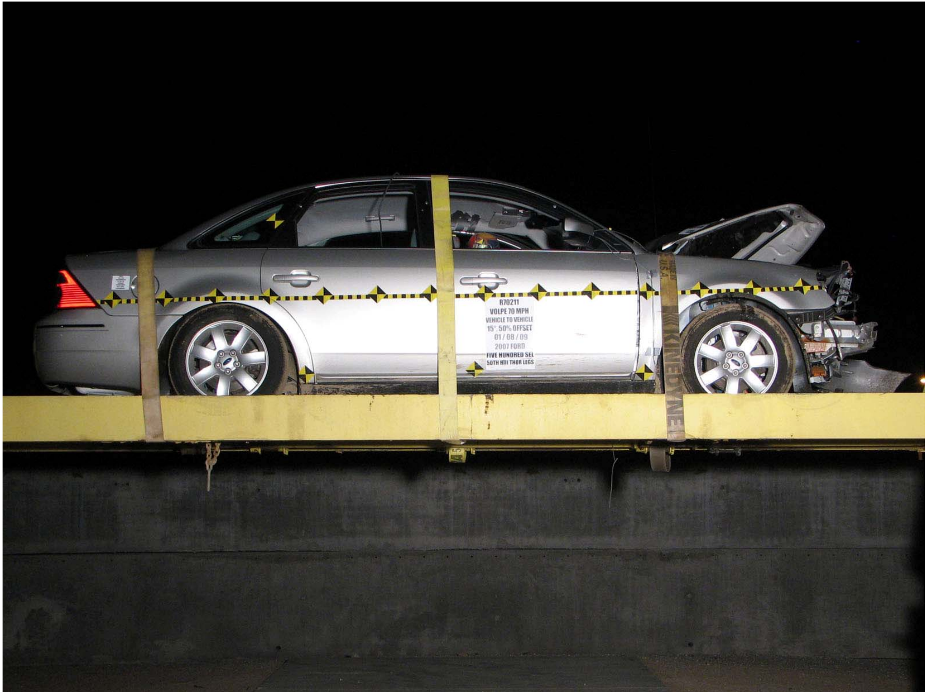
Figure A-608: Target Vehicle on Rollover Device (360°)
