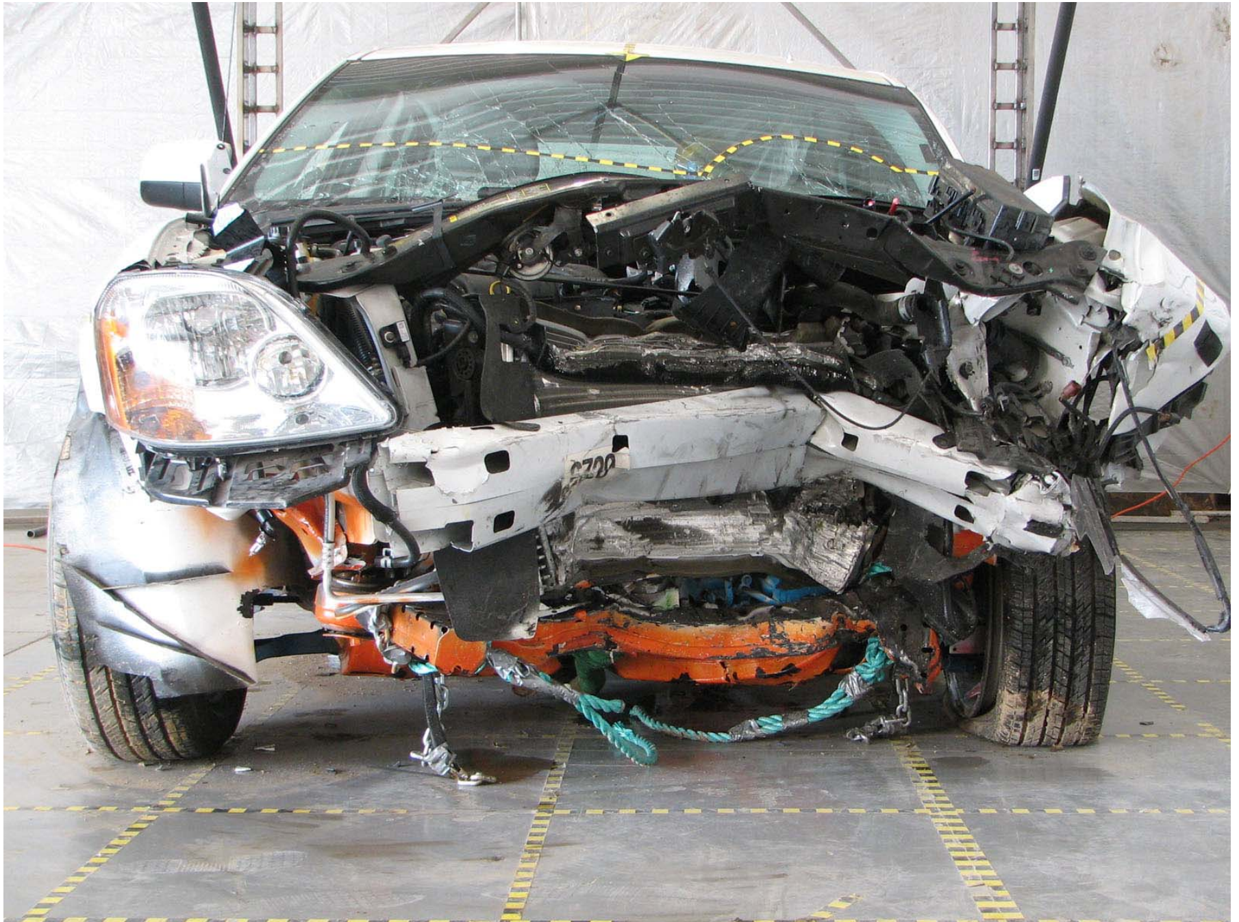
Figure A-601: Bullet Vehicle Post-Test Structural Member Crush Measurement
