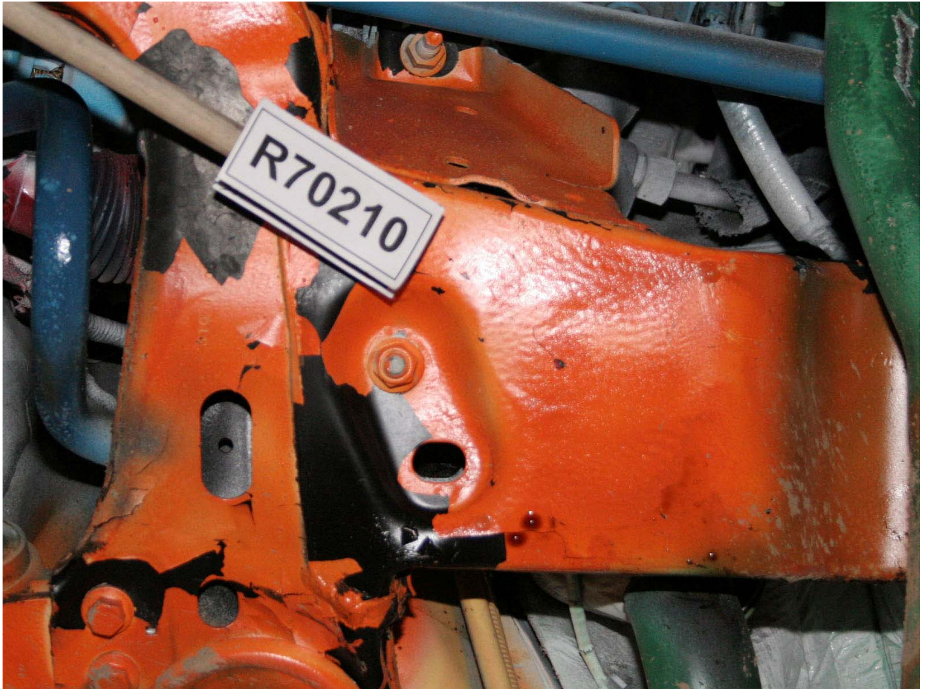
Figure A-533: Bullet Vehicle Post-Test Steering Rack Right Side Mounting Bolt
