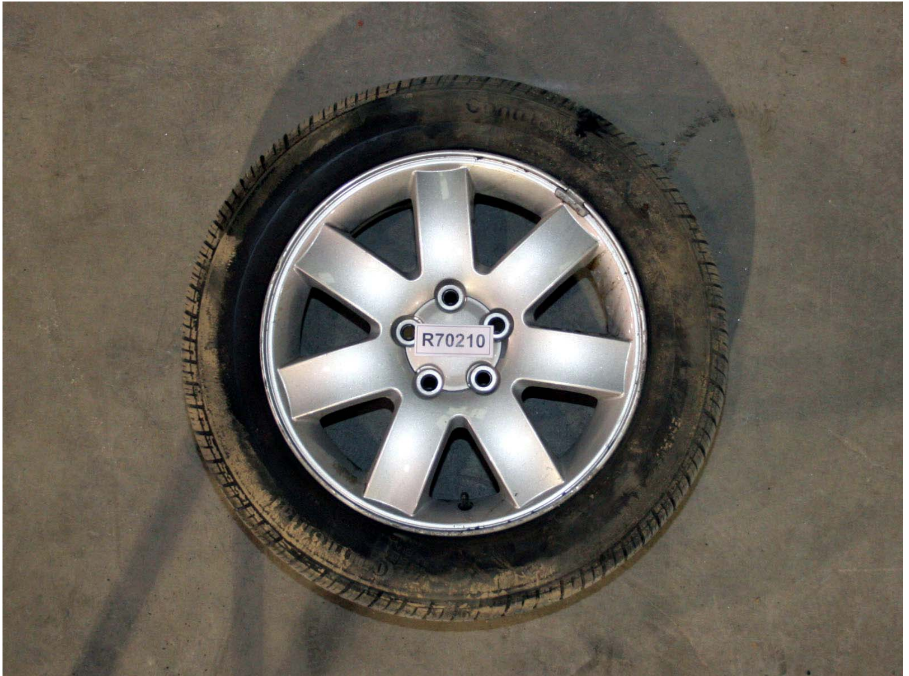
Figure A-448: Bullet Vehicle Post-Test Right Front Wheel Damage (Outside)
