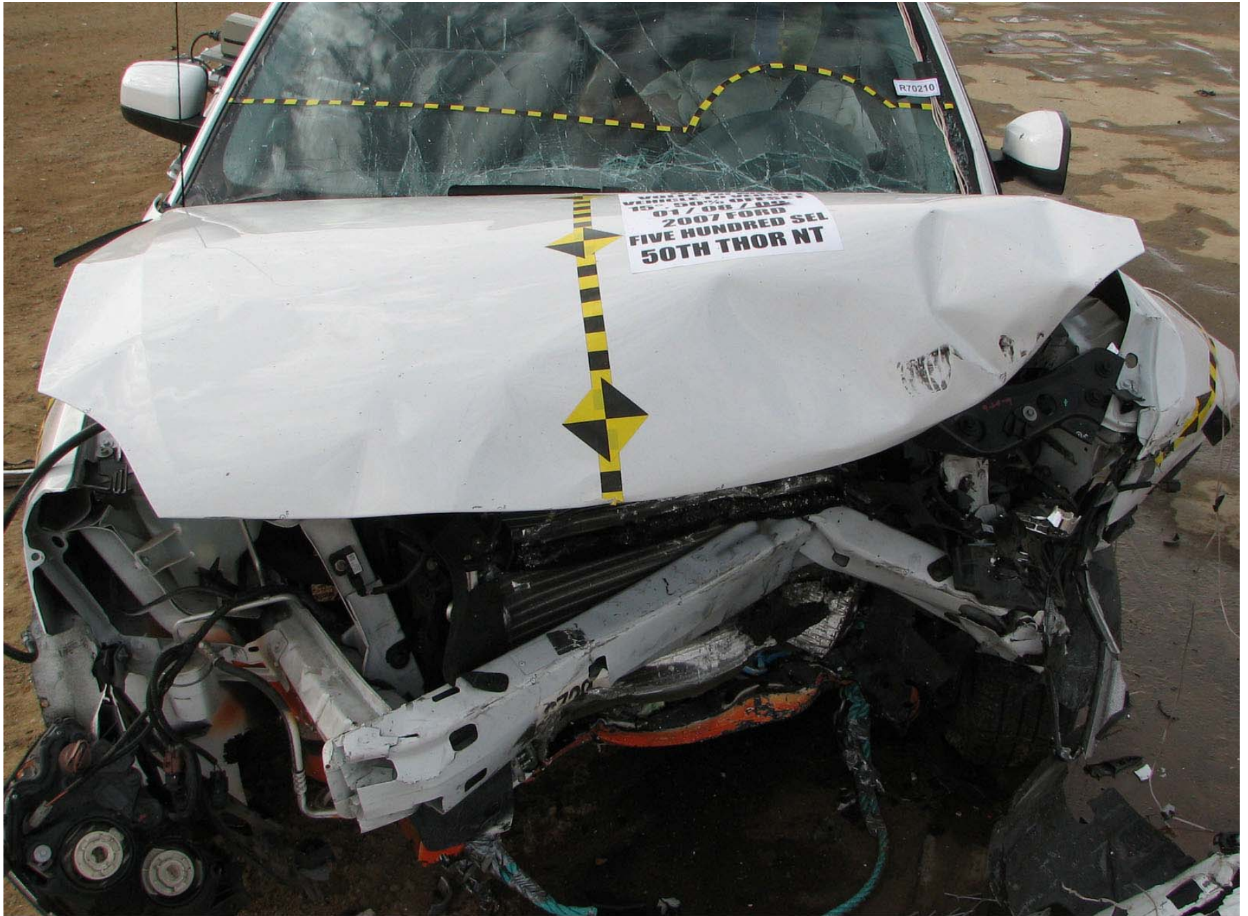
Figure A-365: Bullet Vehicle Post-Test Engine Compartment View
