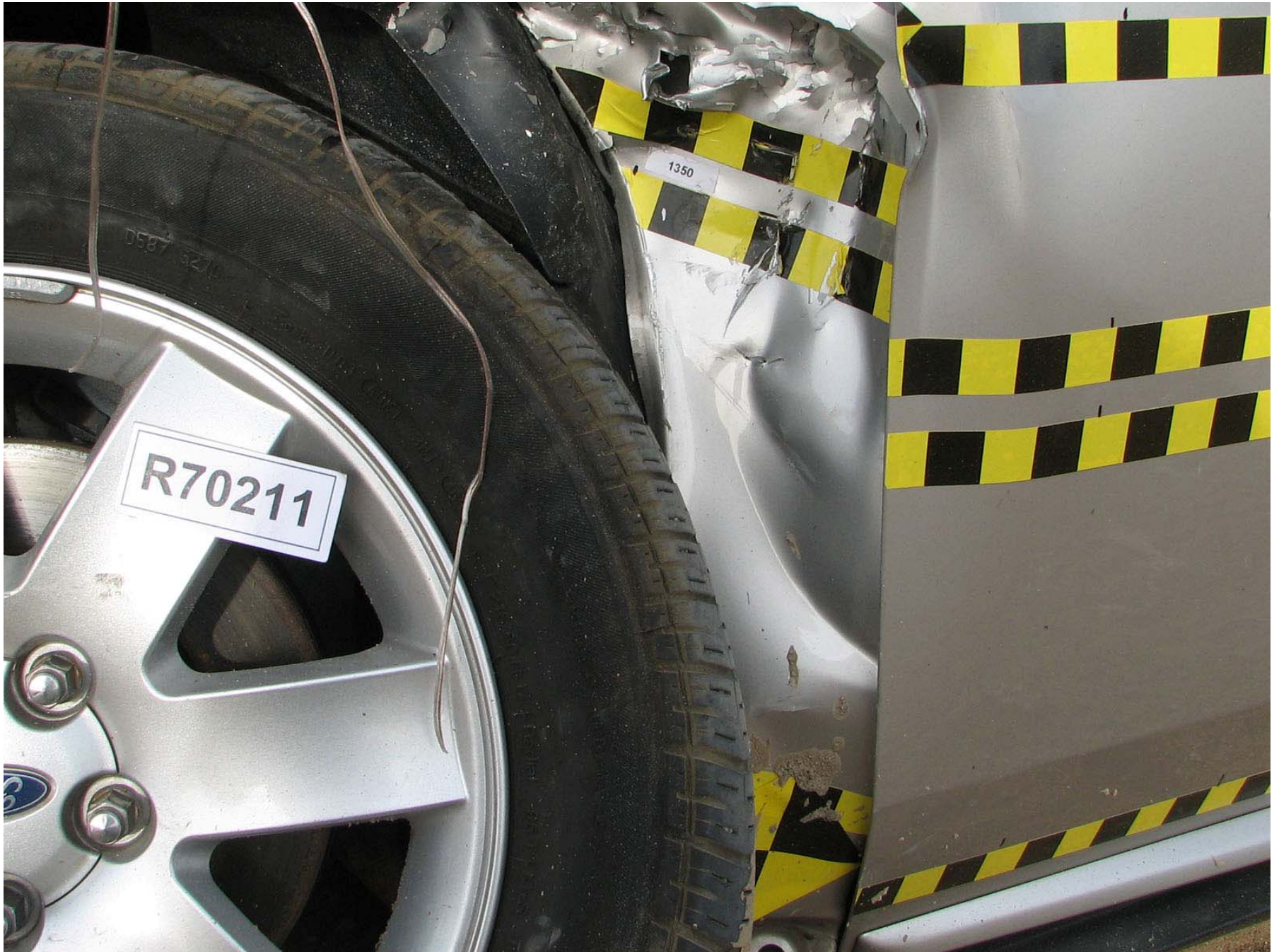
Figure A-145: Target Vehicle Post-Test Left Front Wheel A-Pillar/Rocker Contact
