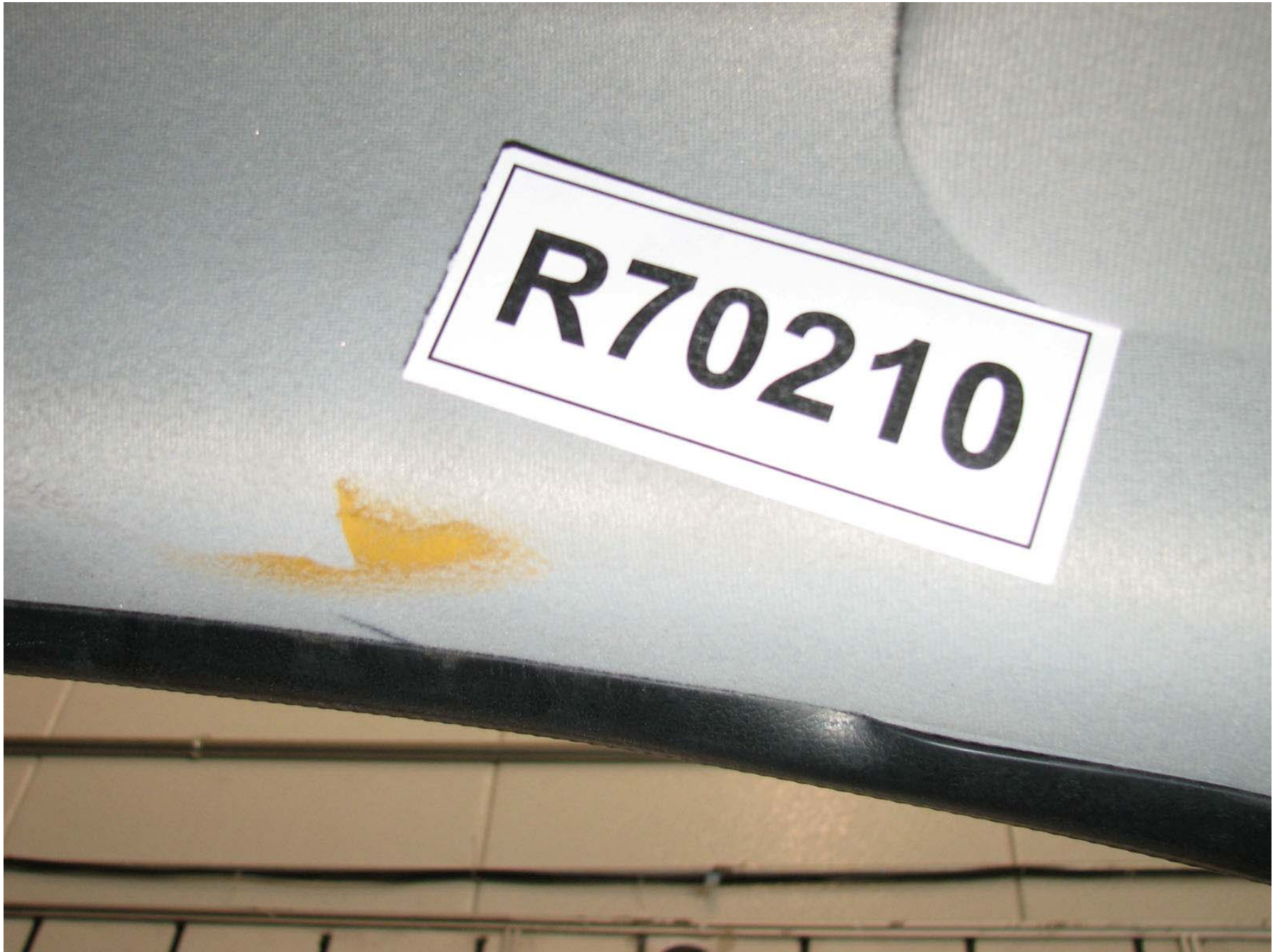
Figure A-570: Bullet Vehicle Post-Test Driver Dummy Contact, Roof
