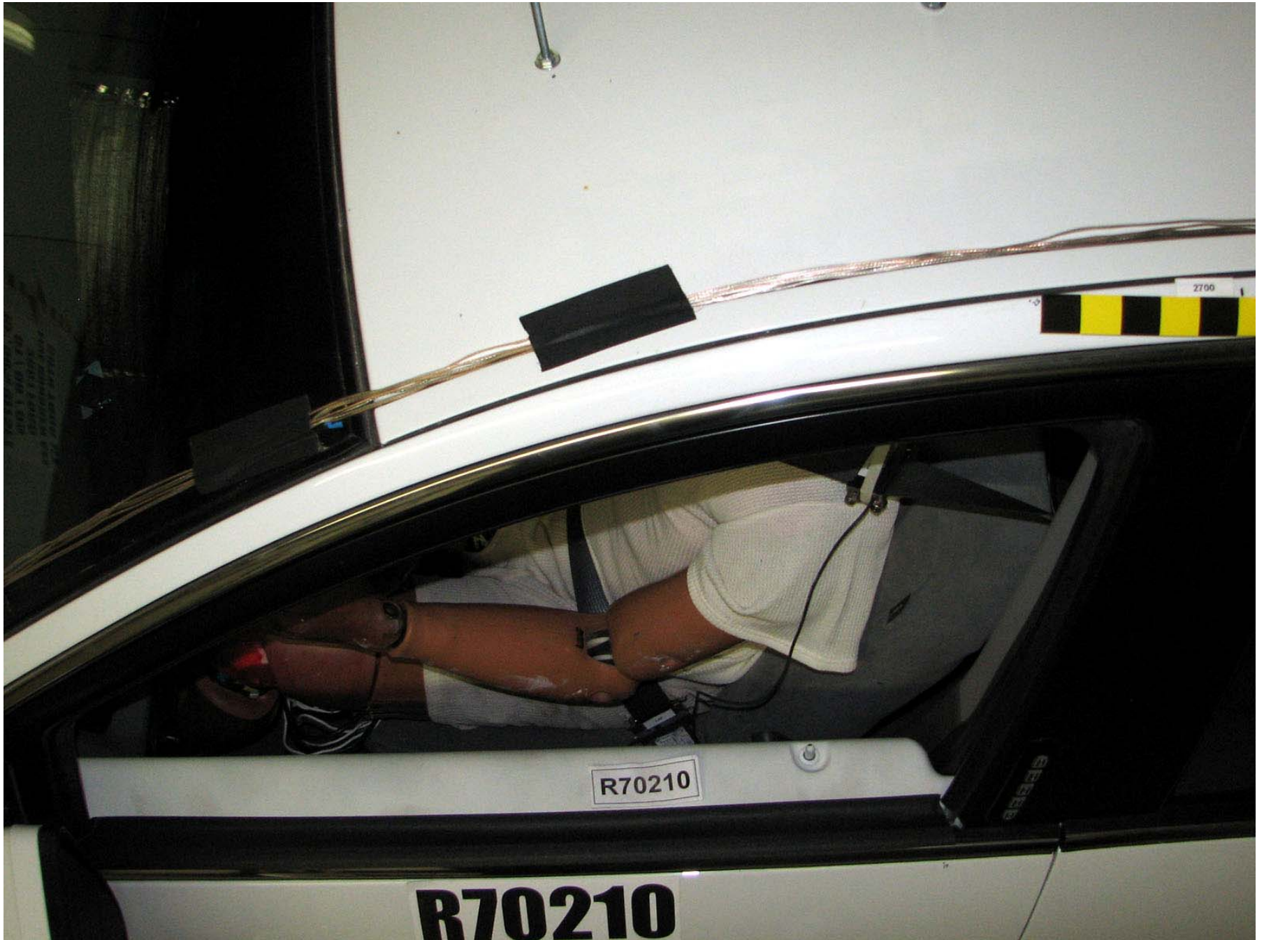
Figure A-558: Bullet Vehicle Pre-Test Driver Dummy Clearance from Door
