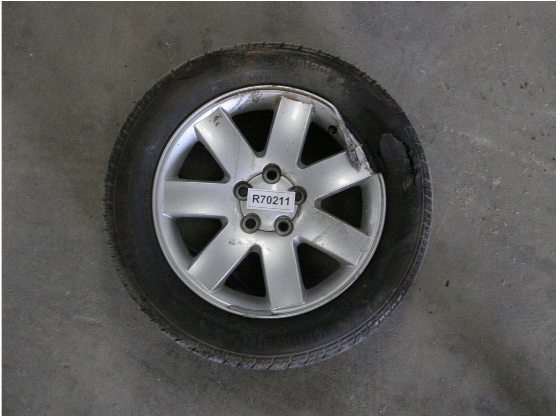
Figure A-148: Target Vehicle Post-Test Left Front Wheel Damage (Outside)
