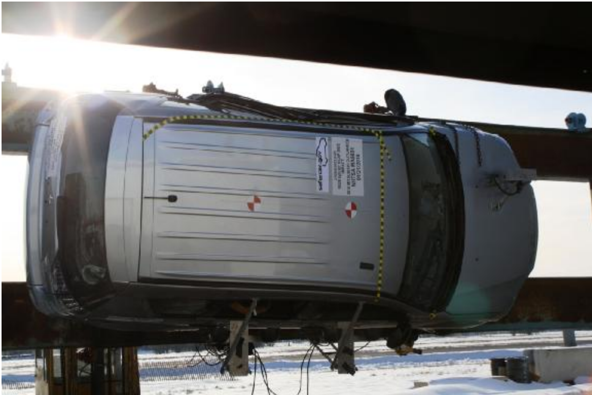
Figure A-53: Rollover 270 Degrees
