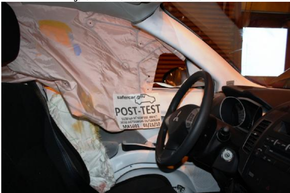
Figure A-44: Post-Test Left Front Interior Trim
