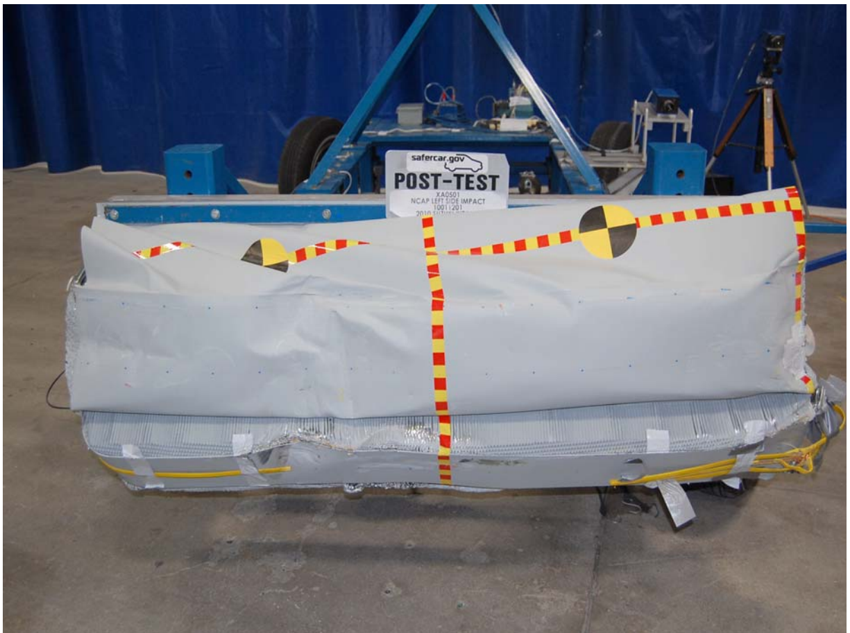
Post-Test Front View of Deformable Barrier
