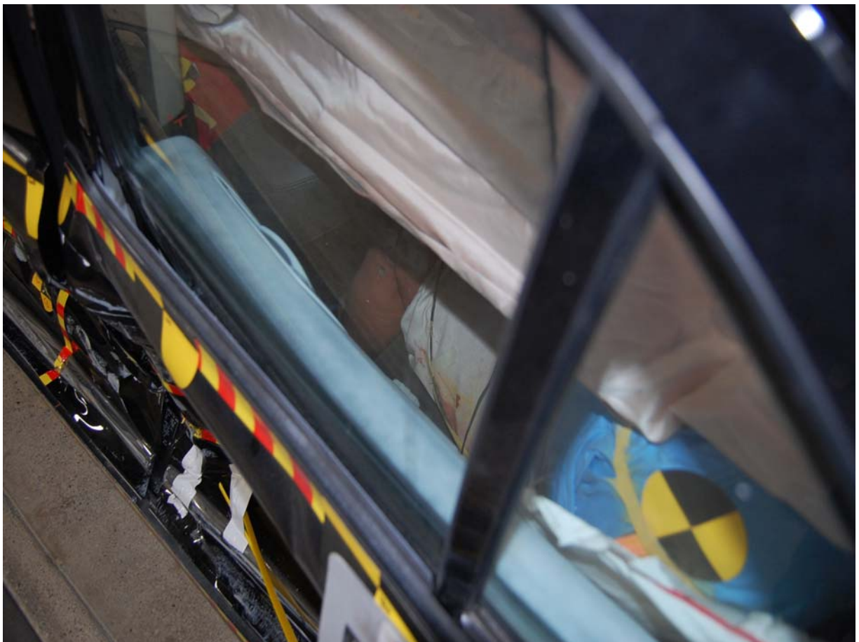
Post-Test Passenger Dummy Clearance From Door
