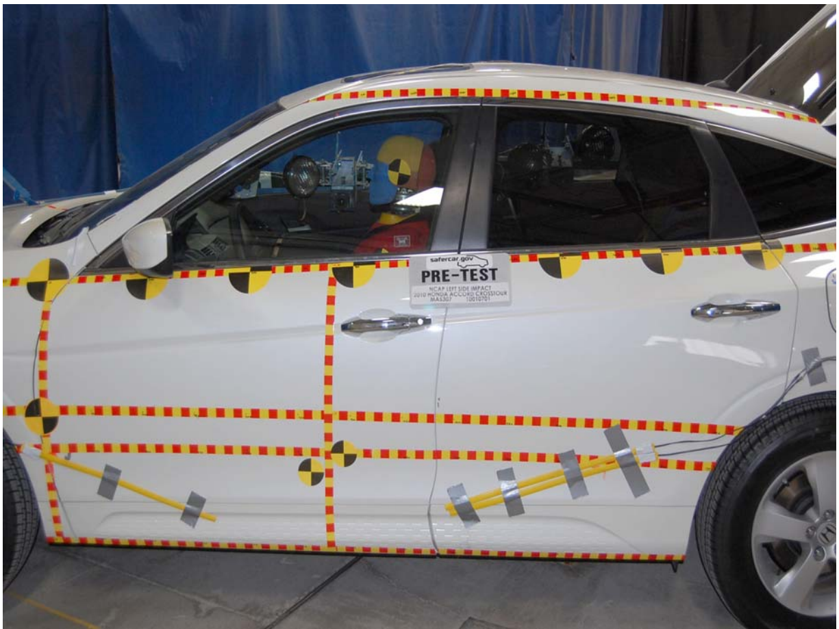
Pre-Test Left Side Impact Close-up
