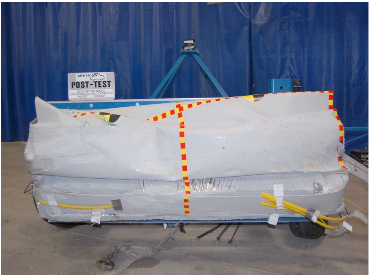
Post-Test Front View of Deformable Barrier
