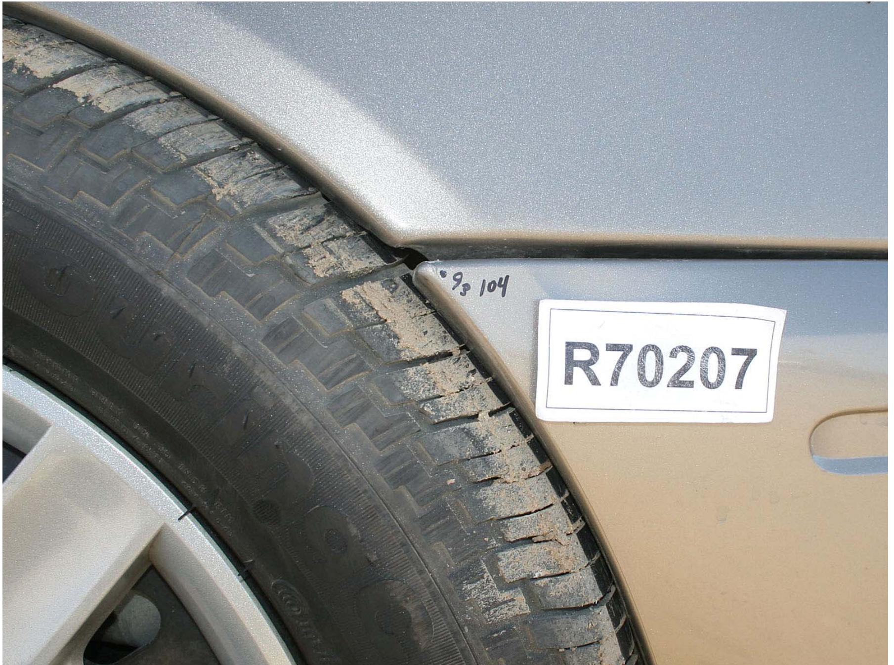
Figure A-129: Test Vehicle Post-Test Right Front Wheel A-Pillar/Rocker Contact
