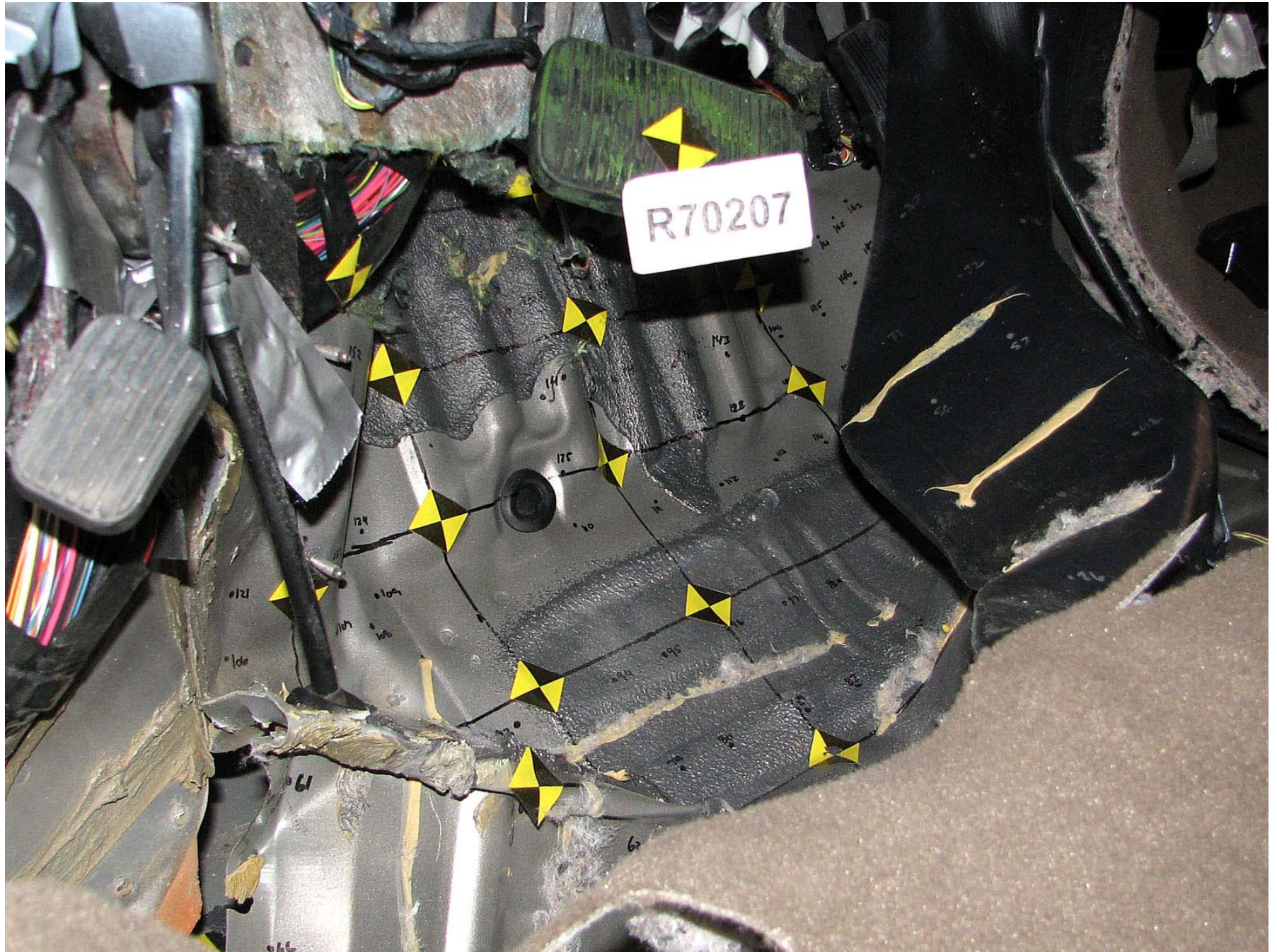
Figure A-288: Test Vehicle Post-Test Driver Floorpan Left \frac{3}{4} View, Seat Cushion Height
