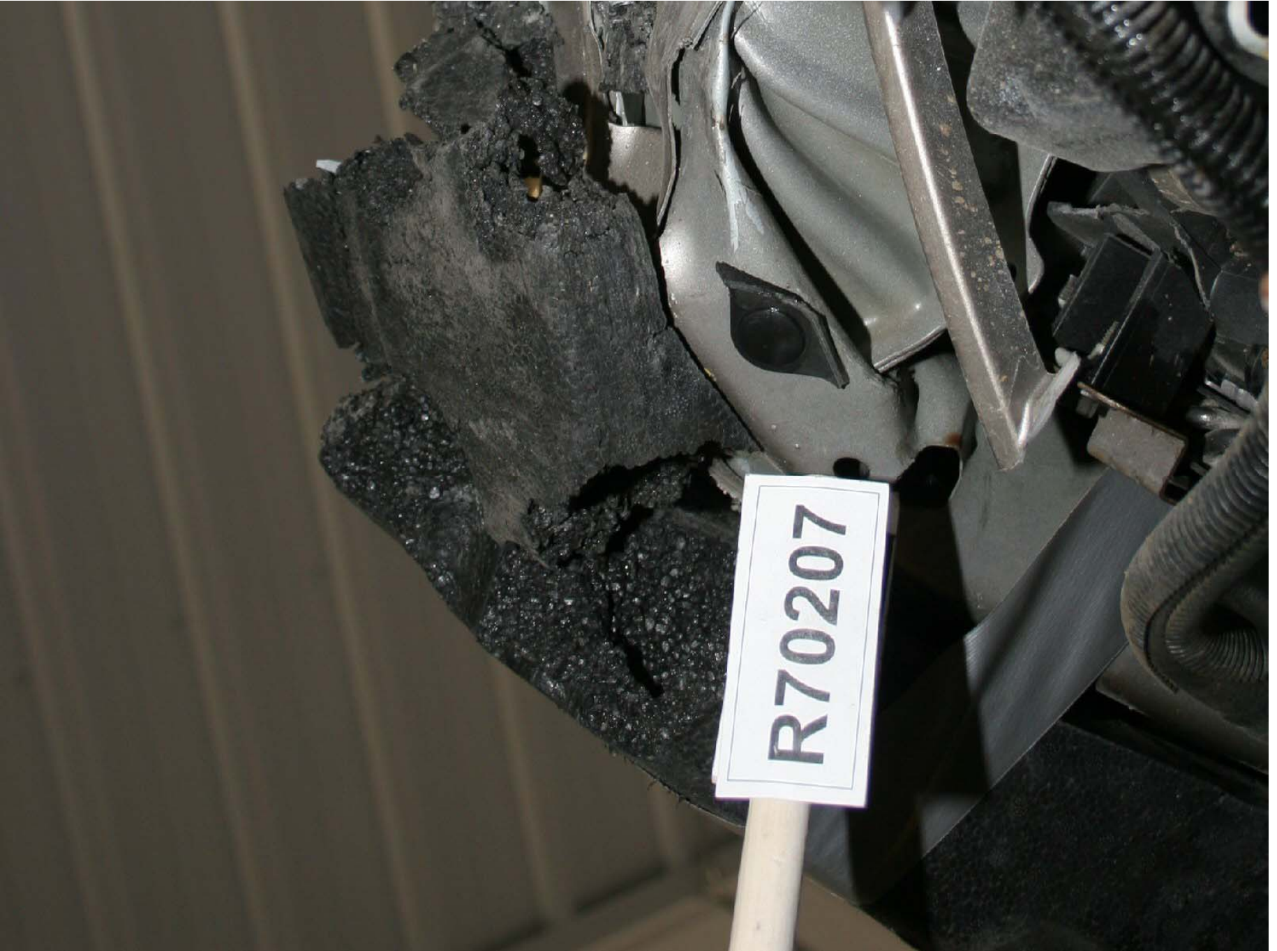
Figure A-164: Test Vehicle Post-Test Left Side Bumper Attachment Point
