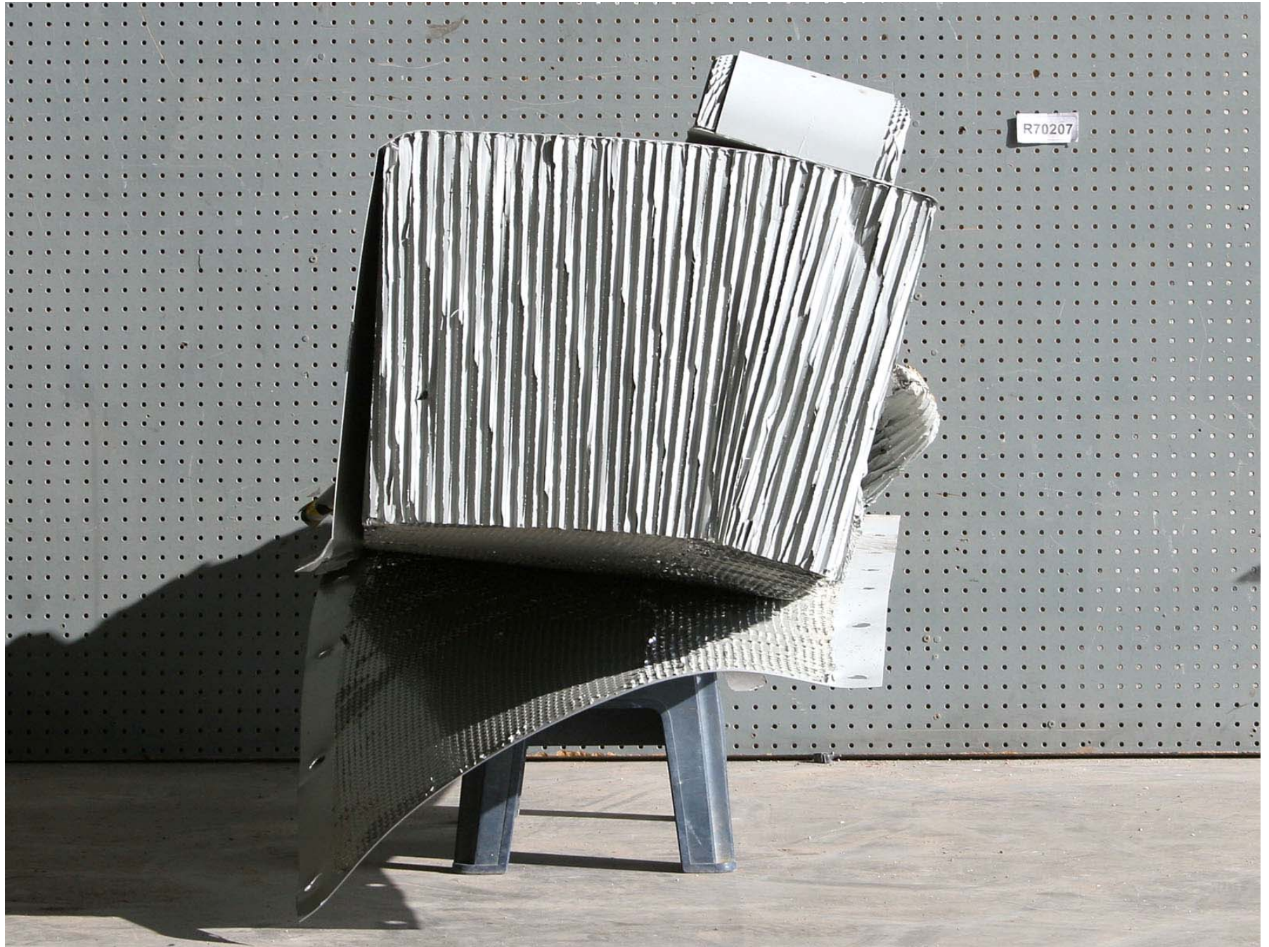
Figure A-329: Test Vehicle Post-Test Right Side View of Deformable Barrier
