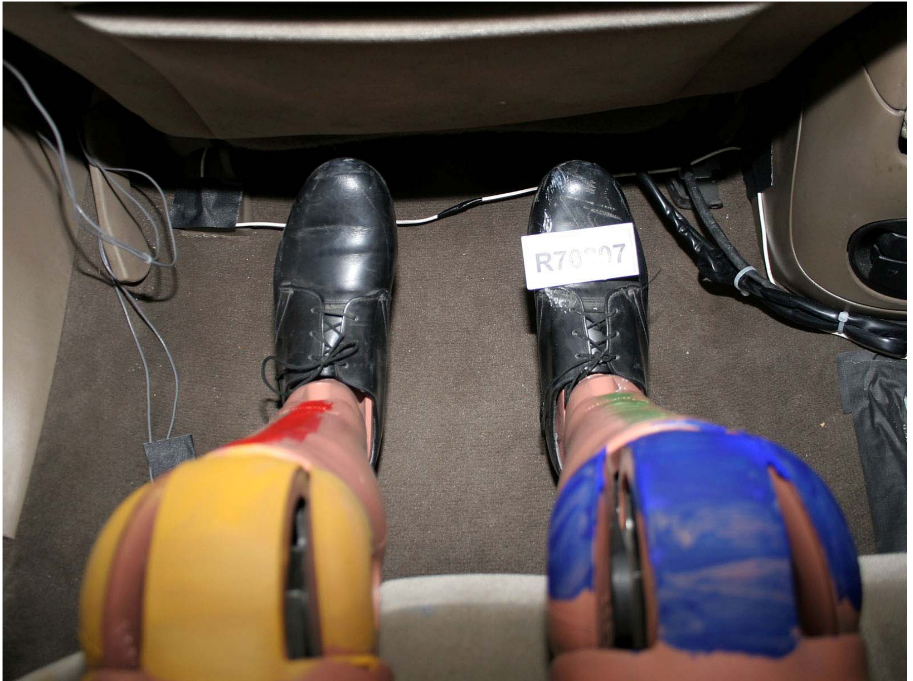
Figure A-268: Test Vehicle Pre-Test Passenger Dummy Feet Positioning
