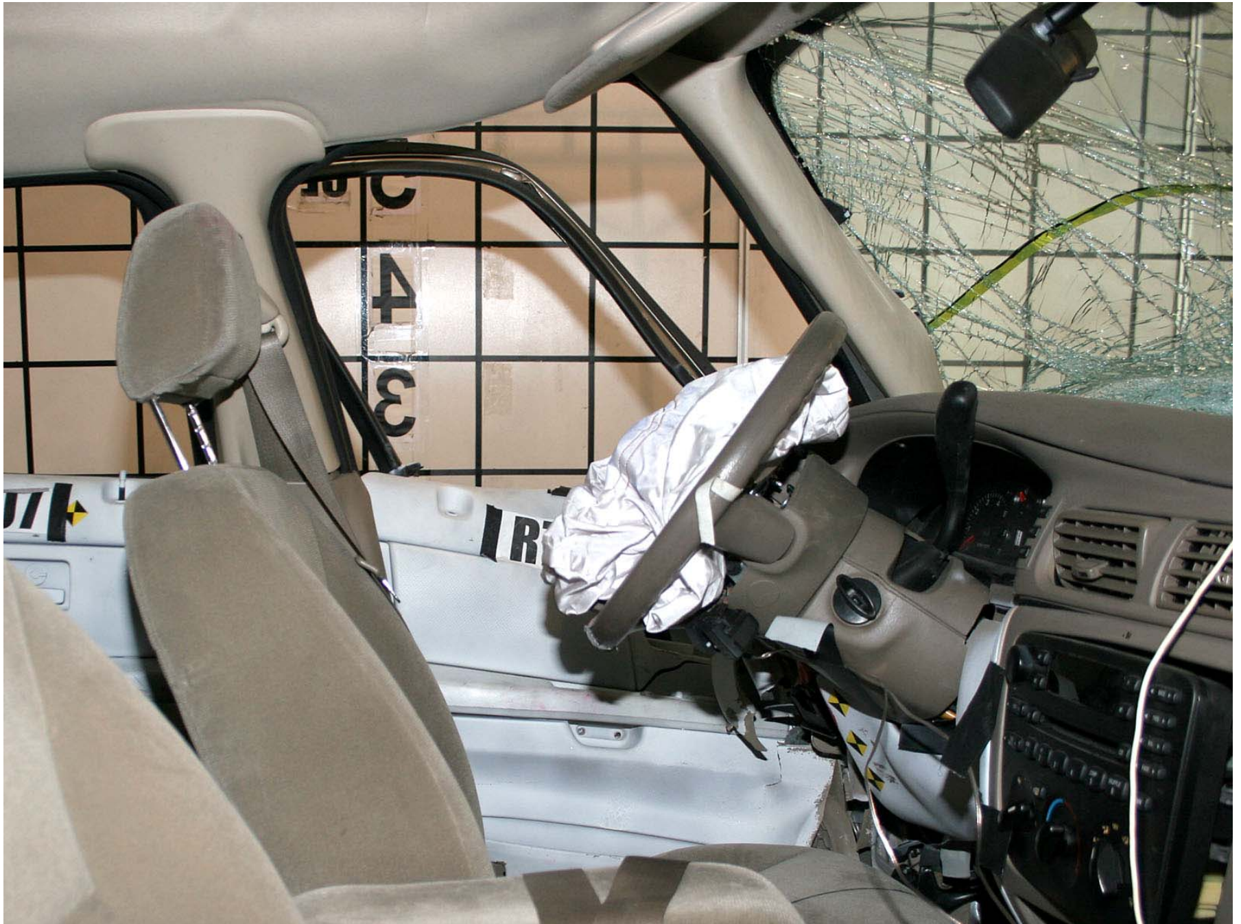
Figure A-222: Test Vehicle Post-Test Front Door Panel
