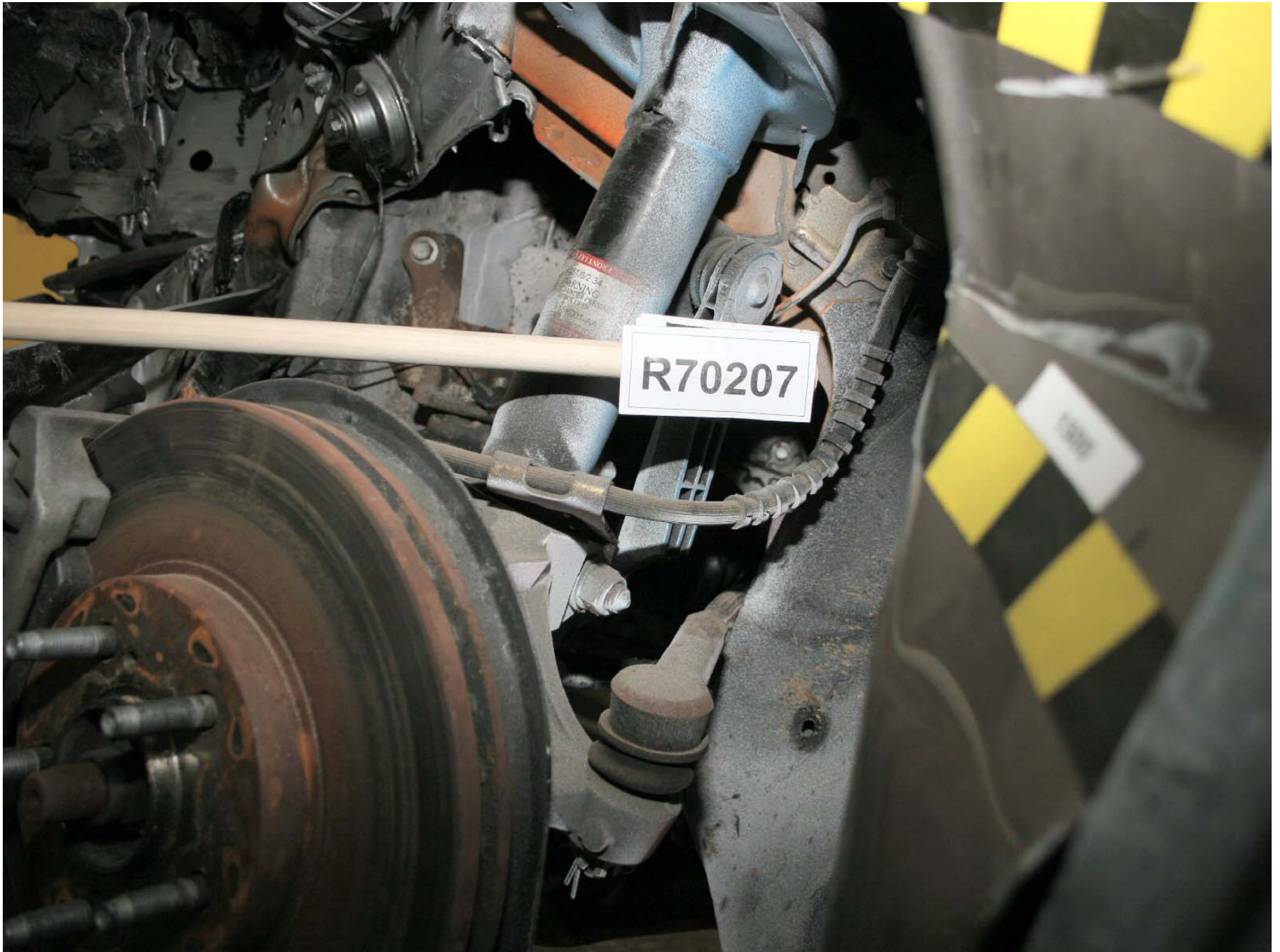
Figure A-154: Test Vehicle Post-Test Left Side Tie Rod and Sway Bar Attachments Points
