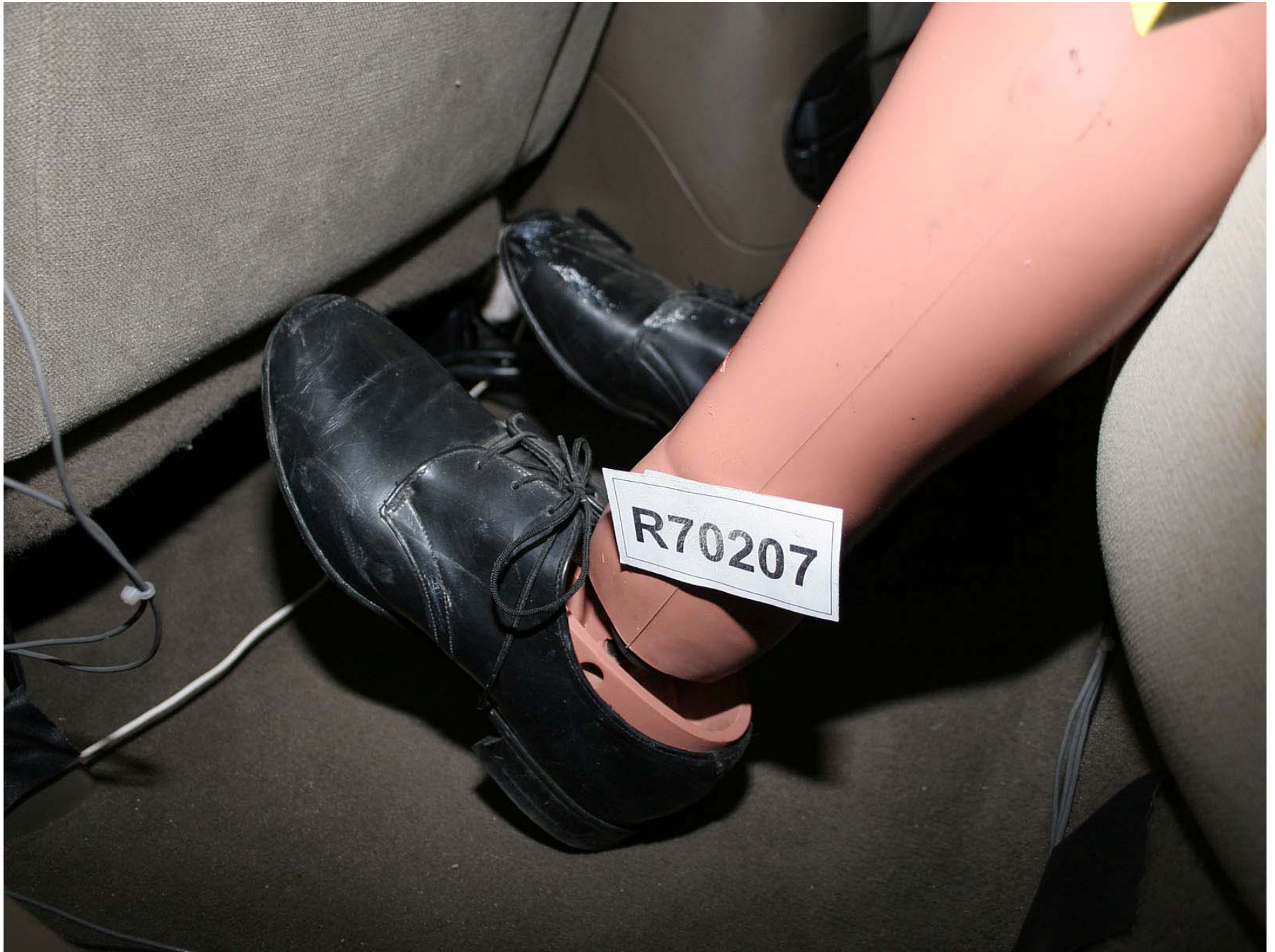
Figure A-267: Test Vehicle Pre-Test Passenger Dummy Feet Positioning
