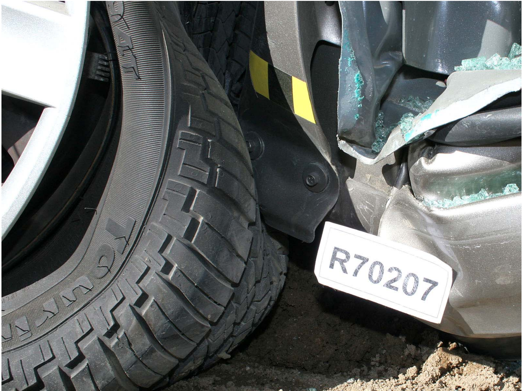
Figure A-117: Test Vehicle Post-Test Left Front Wheel A-Pillar/Rocker Contact
