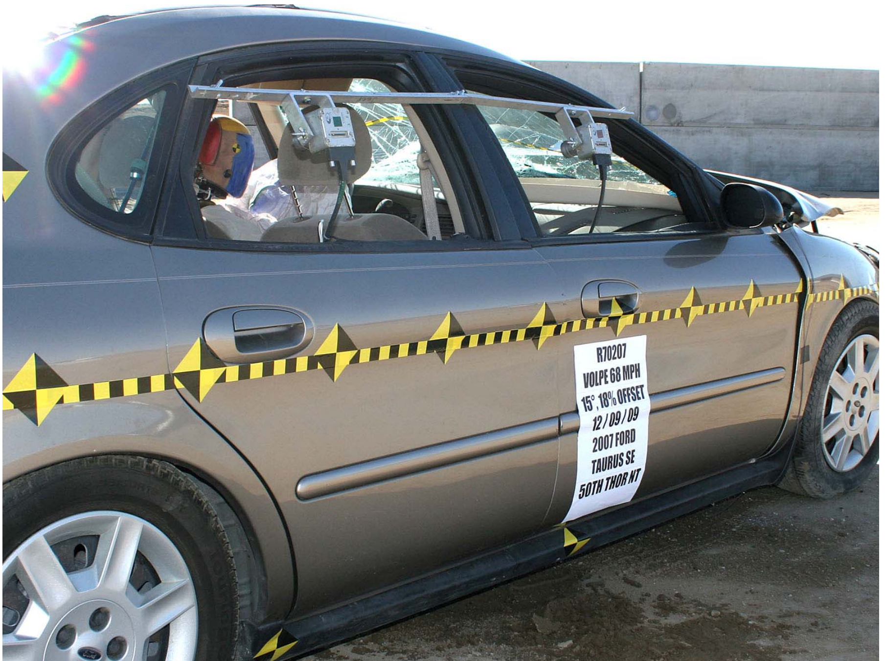
Figure A-36: Test Vehicle Post-Test Rear \frac{3}{4} View of Right Side Doors
