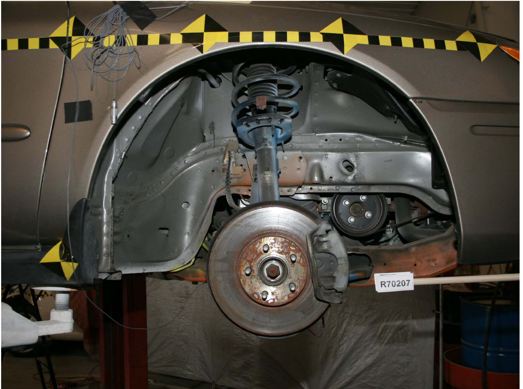
Figure A-173: Test Vehicle Pre-Test Right Front Wheel Well (Tire Off), Inner Fender Removed
