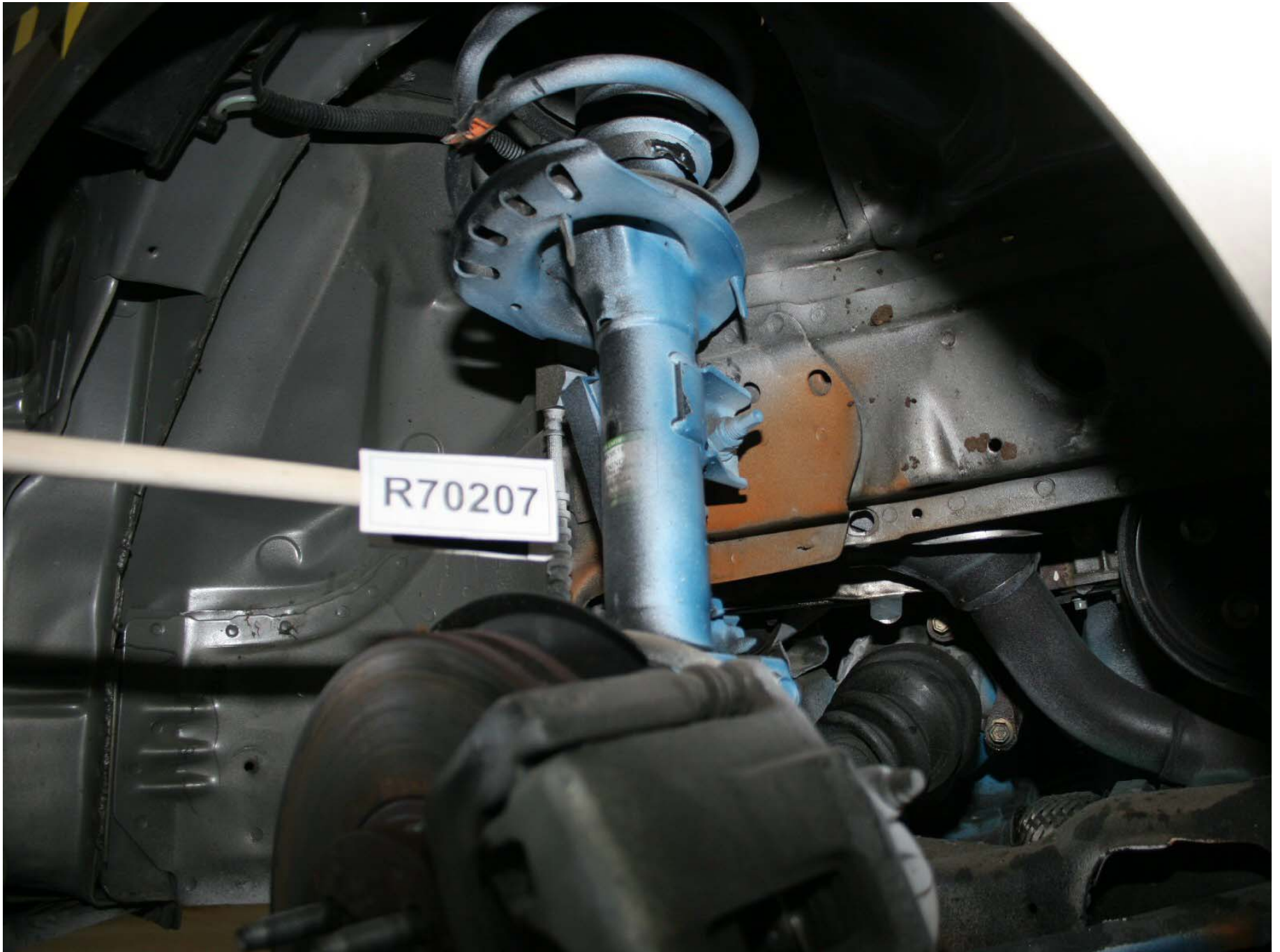
Figure A-192: Test Vehicle Post-Test Right Side Tie Rod and Sway Bar Attachments Points
