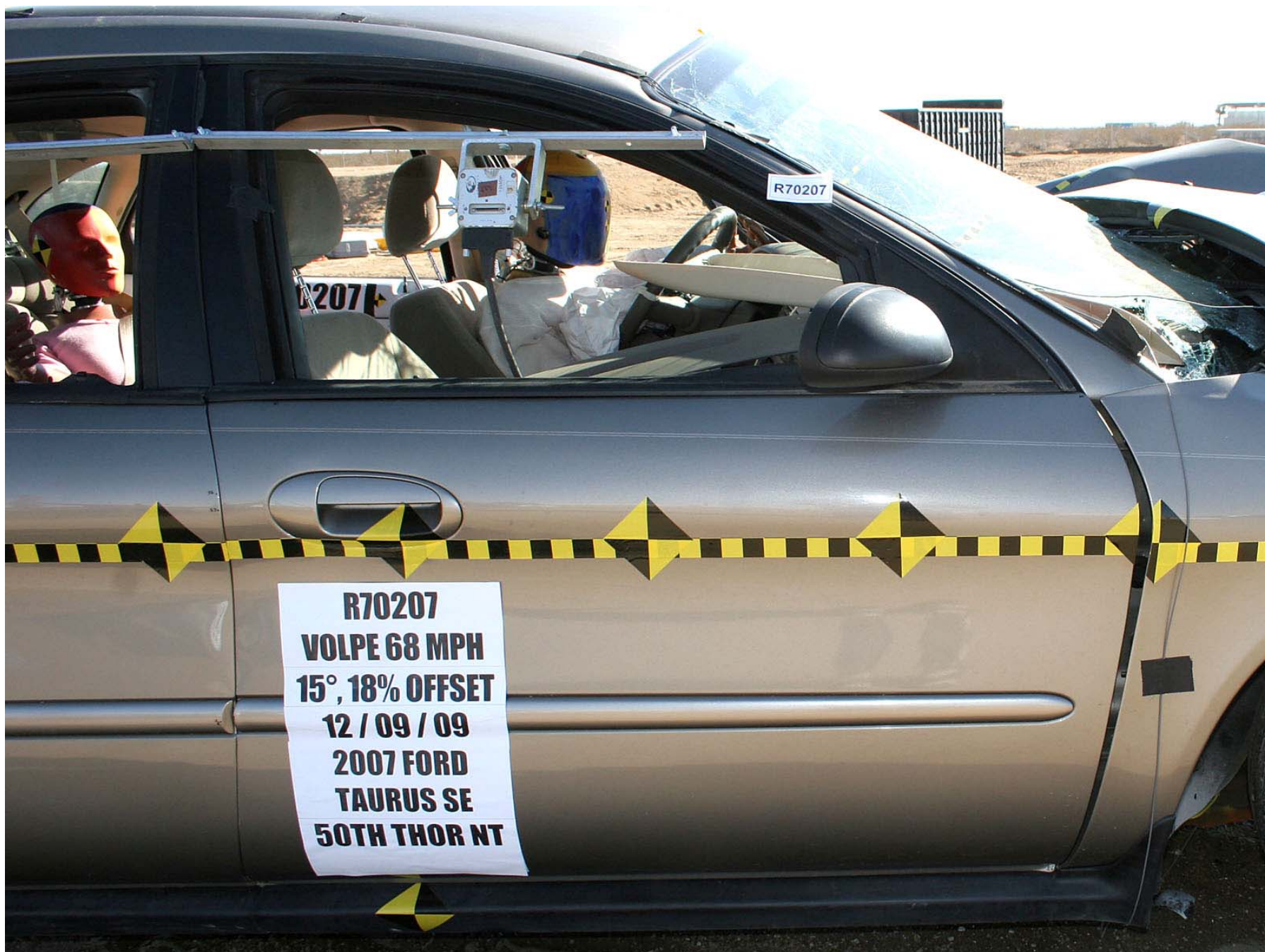
Figure A-42: Test Vehicle Post-Test Right Front Door
