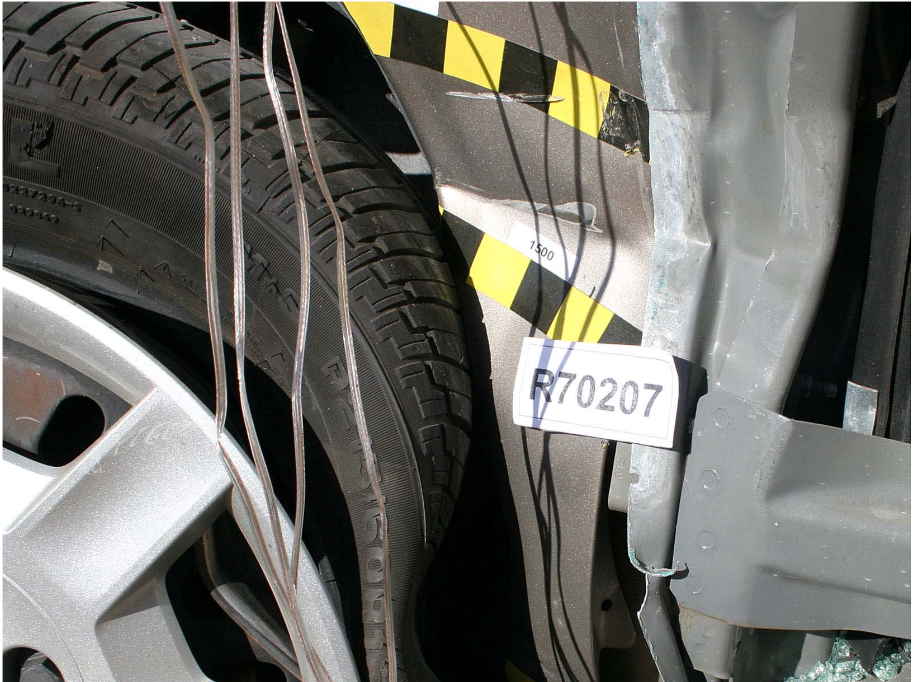
Figure A-115: Test Vehicle Post-Test Left Front Wheel A-Pillar/Rocker Contact
