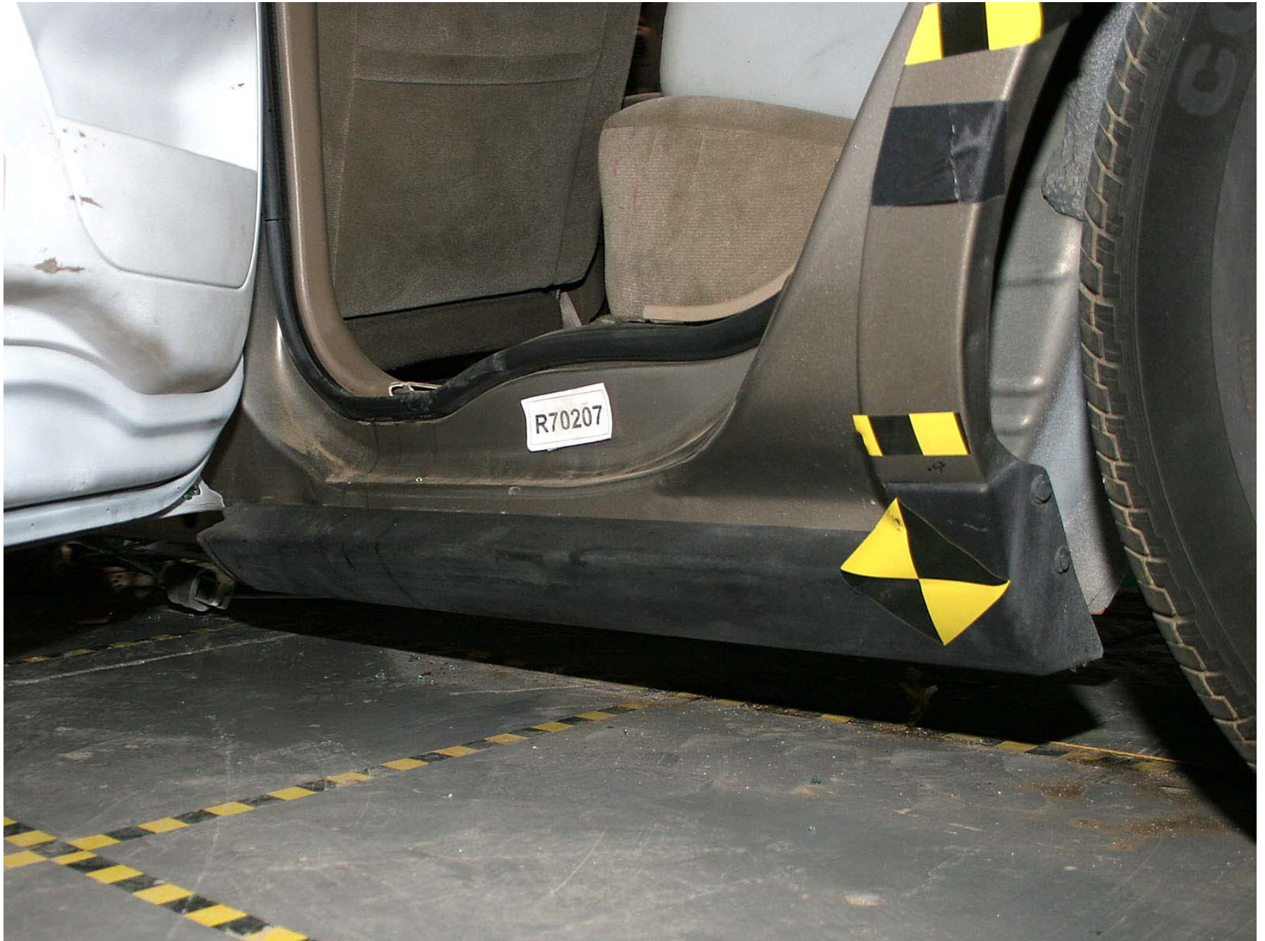
Figure A-78: Test Vehicle Post-Test Left Rear Sill Rear \frac{3}{4} View, Door Open
