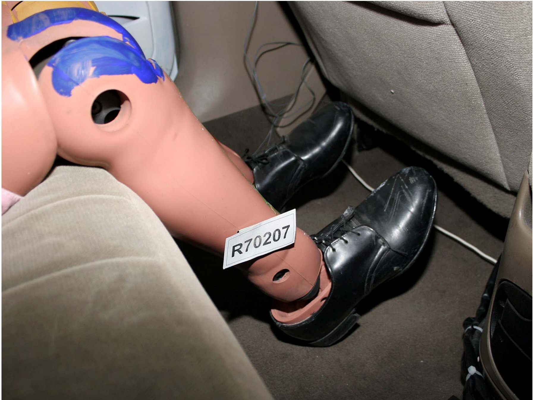
Figure A-269: Test Vehicle Pre-Test Passenger Dummy Feet Positioning
