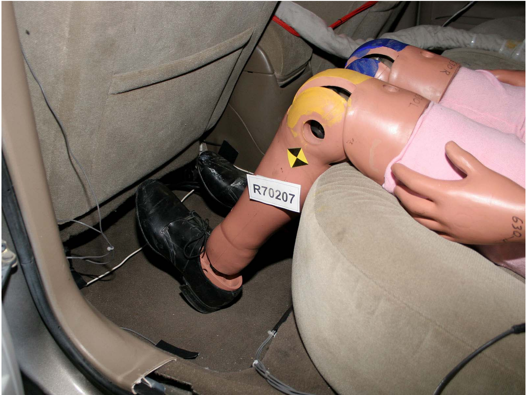
Figure A-266: Test Vehicle Pre-Test Passenger Dummy Feet Positioning
