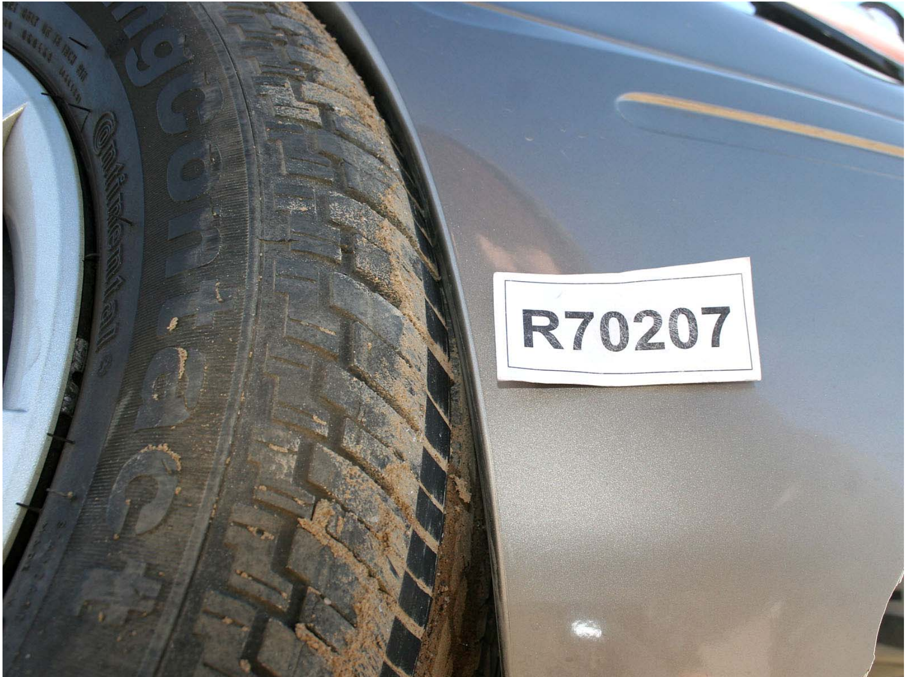
Figure A-130: Test Vehicle Post-Test Right Front Wheel A-Pillar/Rocker Contact
