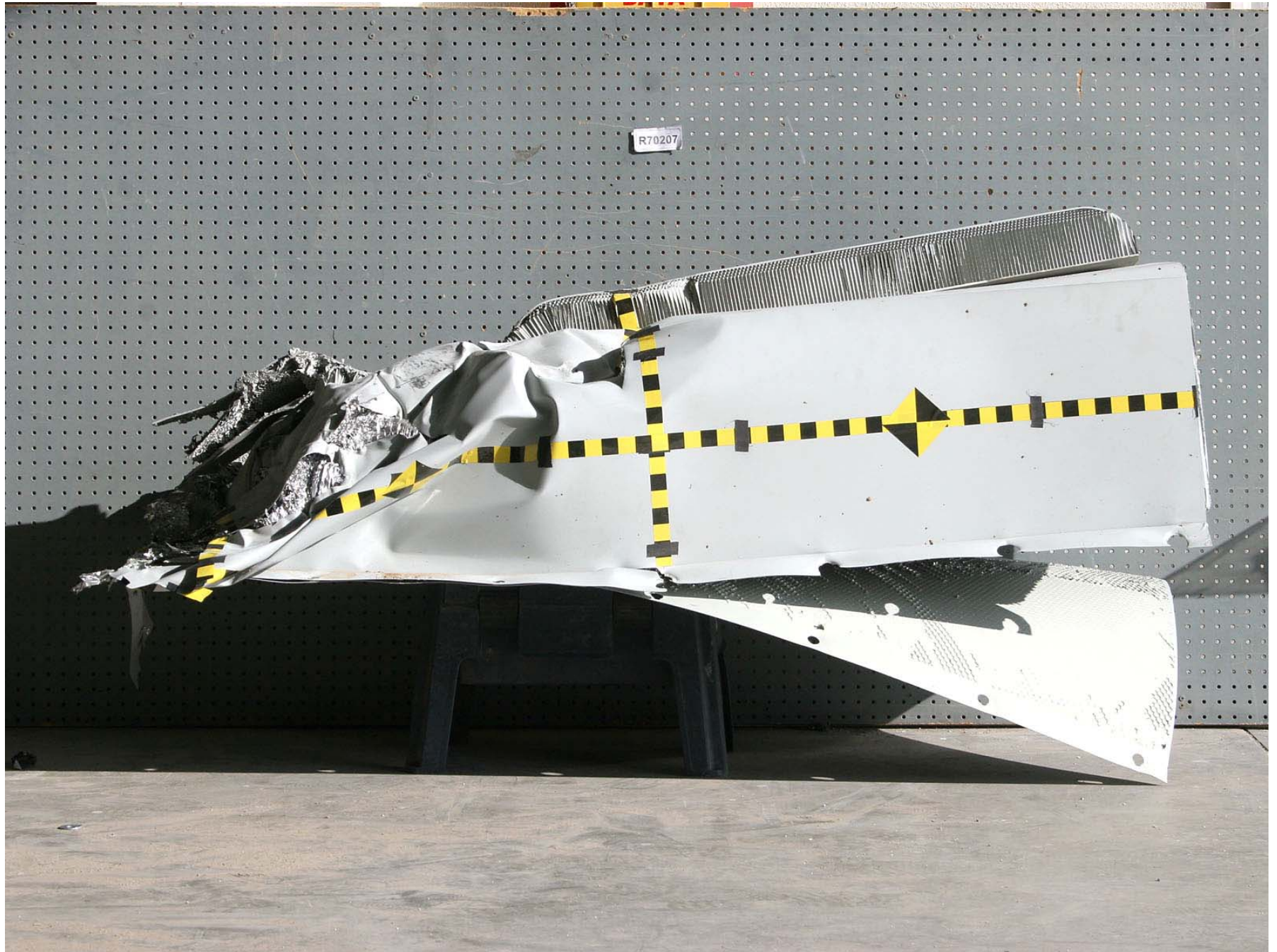
Figure A-327: Test Vehicle Post-Test Top View of Deformable Barrier
