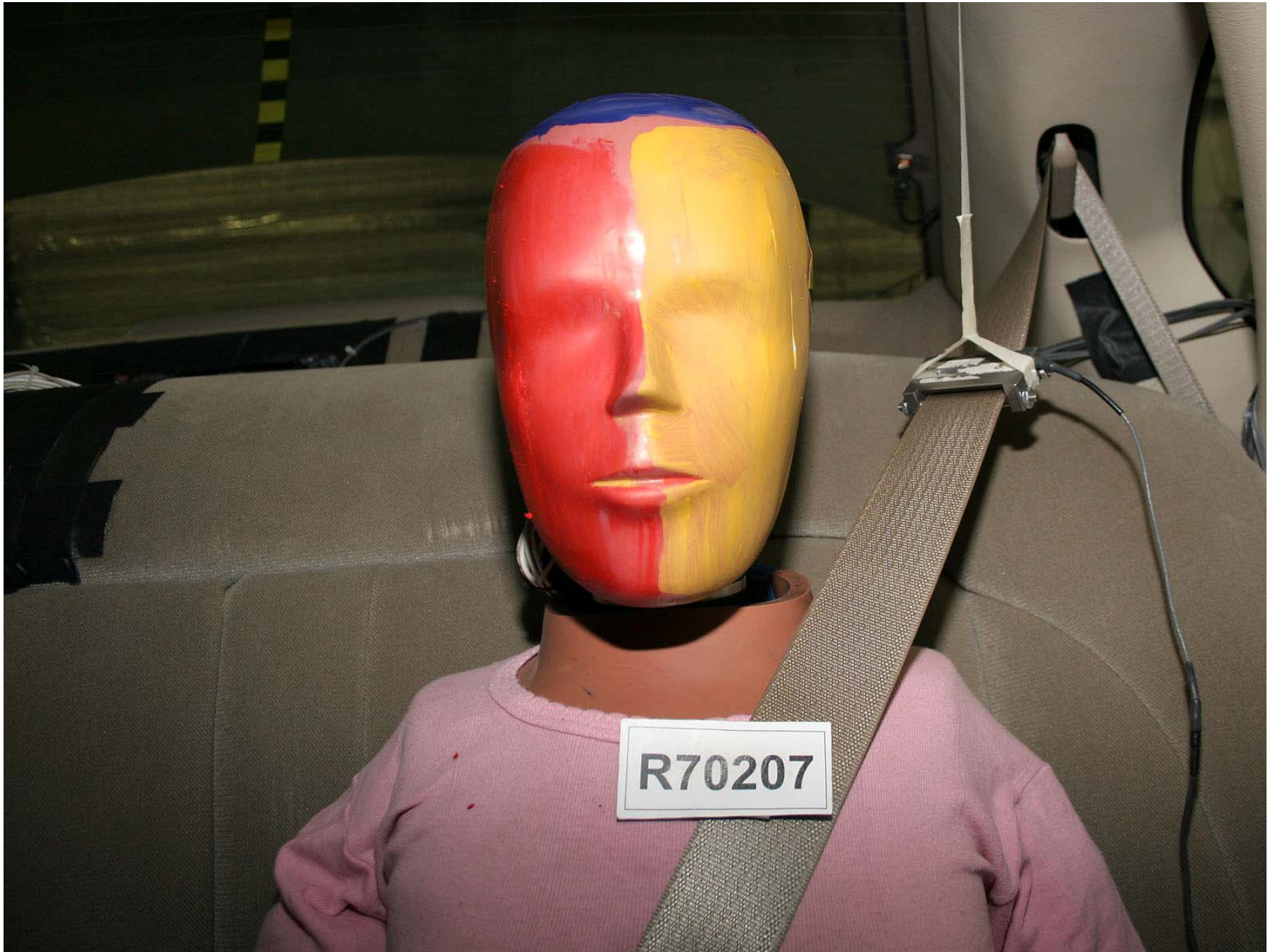
Figure A-262: Test Vehicle Pre-Test Passenger Dummy Front View
