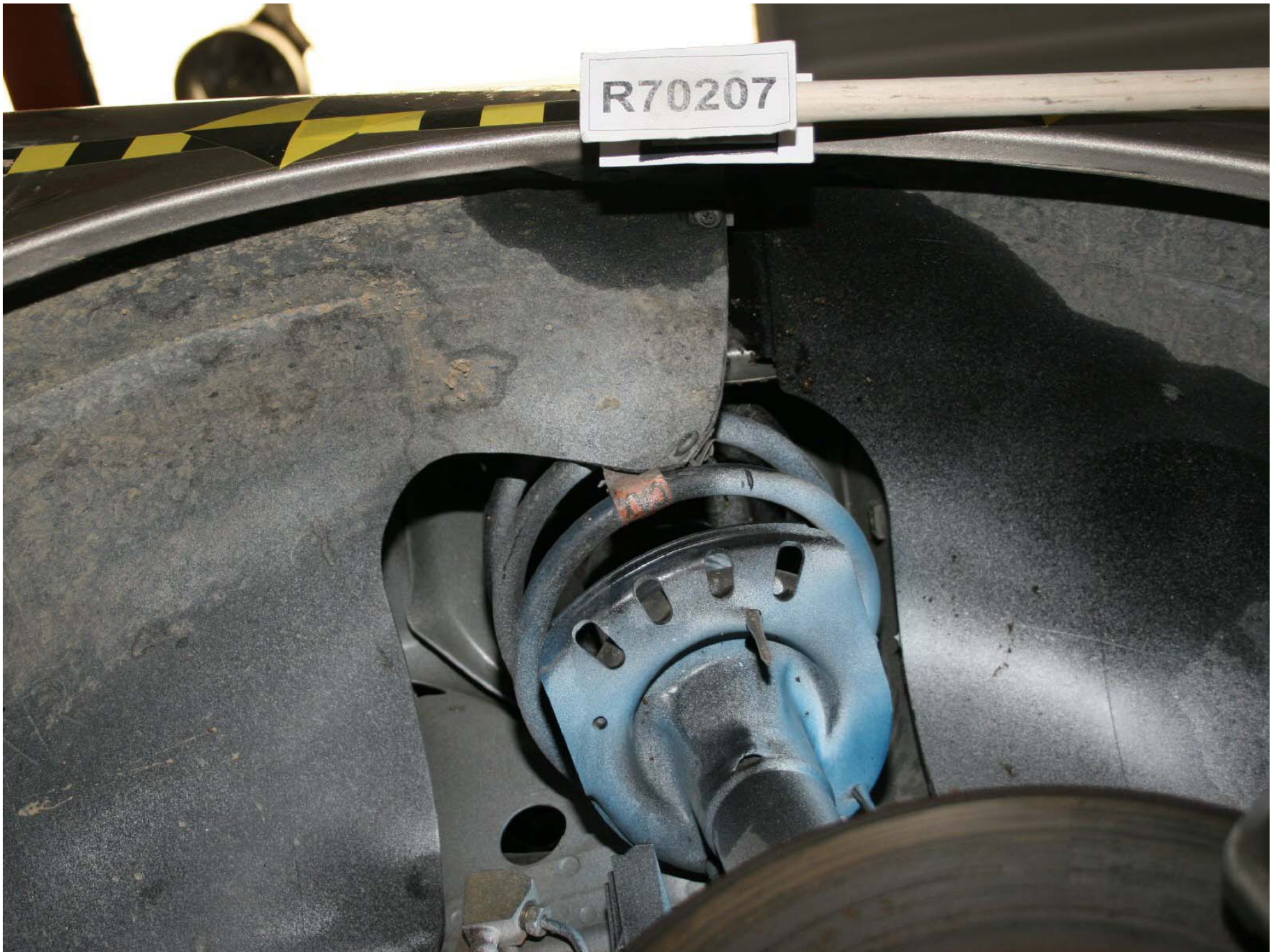
Figure A-178: Test Vehicle Post-Test Right Inner Fender Well View
