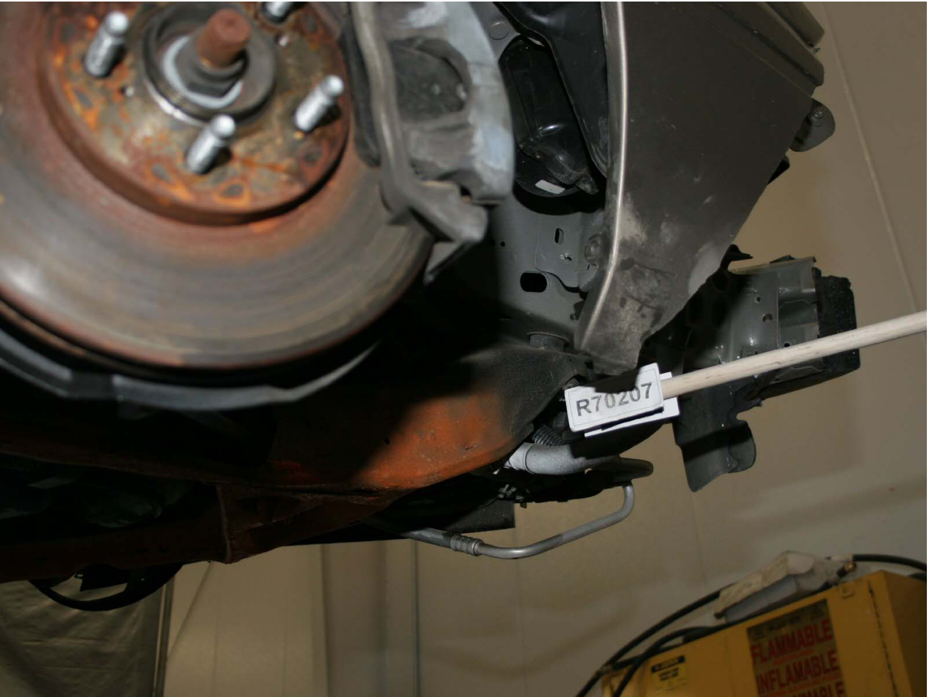
Figure A-196: Test Vehicle Post-Test Right Side Crush Initiators
