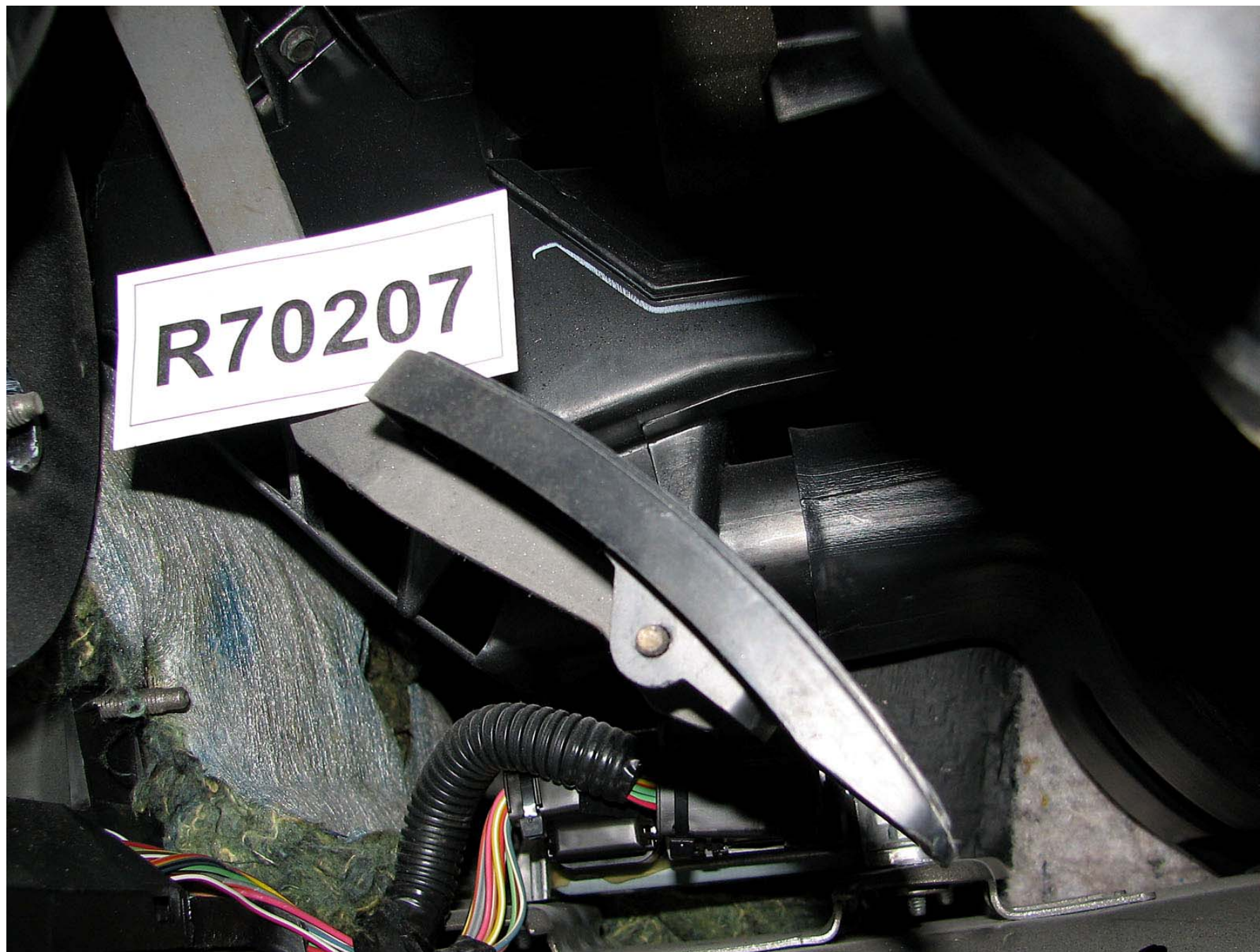
Figure A-303: Test Vehicle Pre-Test Accelerator Pedal Side View, Behind Brake Pedal
