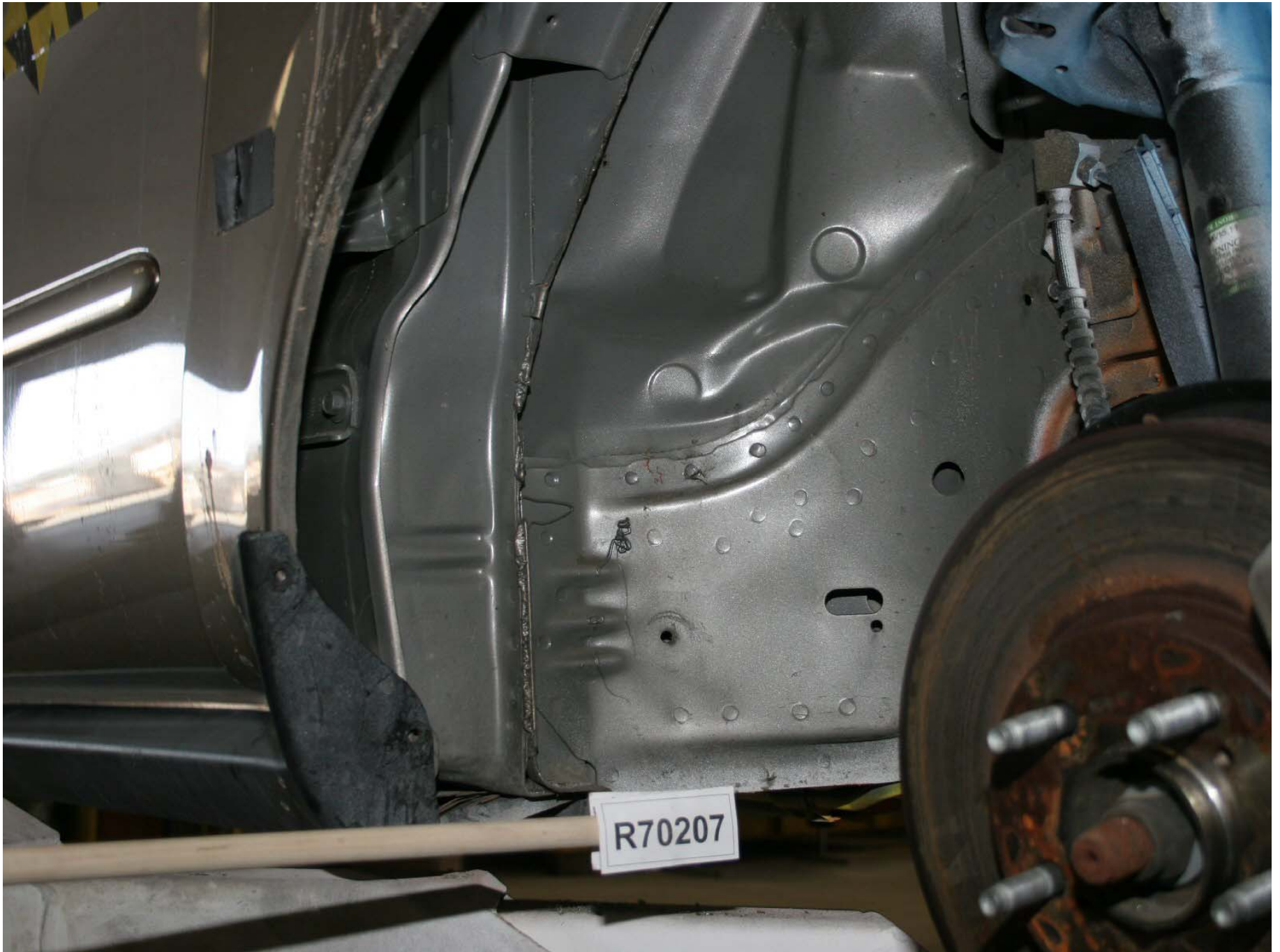
Figure A-194: Test Vehicle Post-Test Right Side Upper Sway Bar Attachment Point
