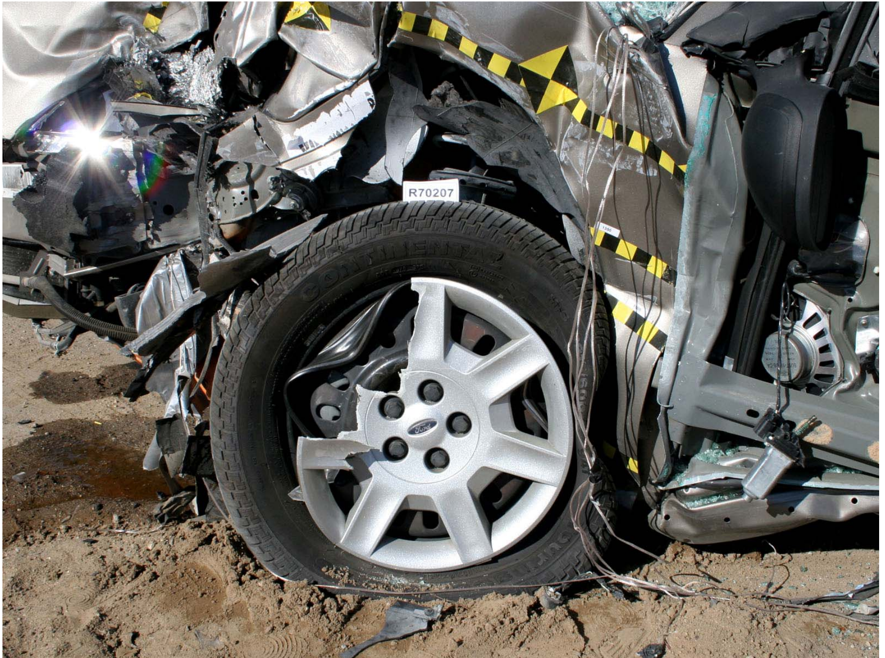
Figure A-108: Test Vehicle Post-Test Left Front Wheel Side View
