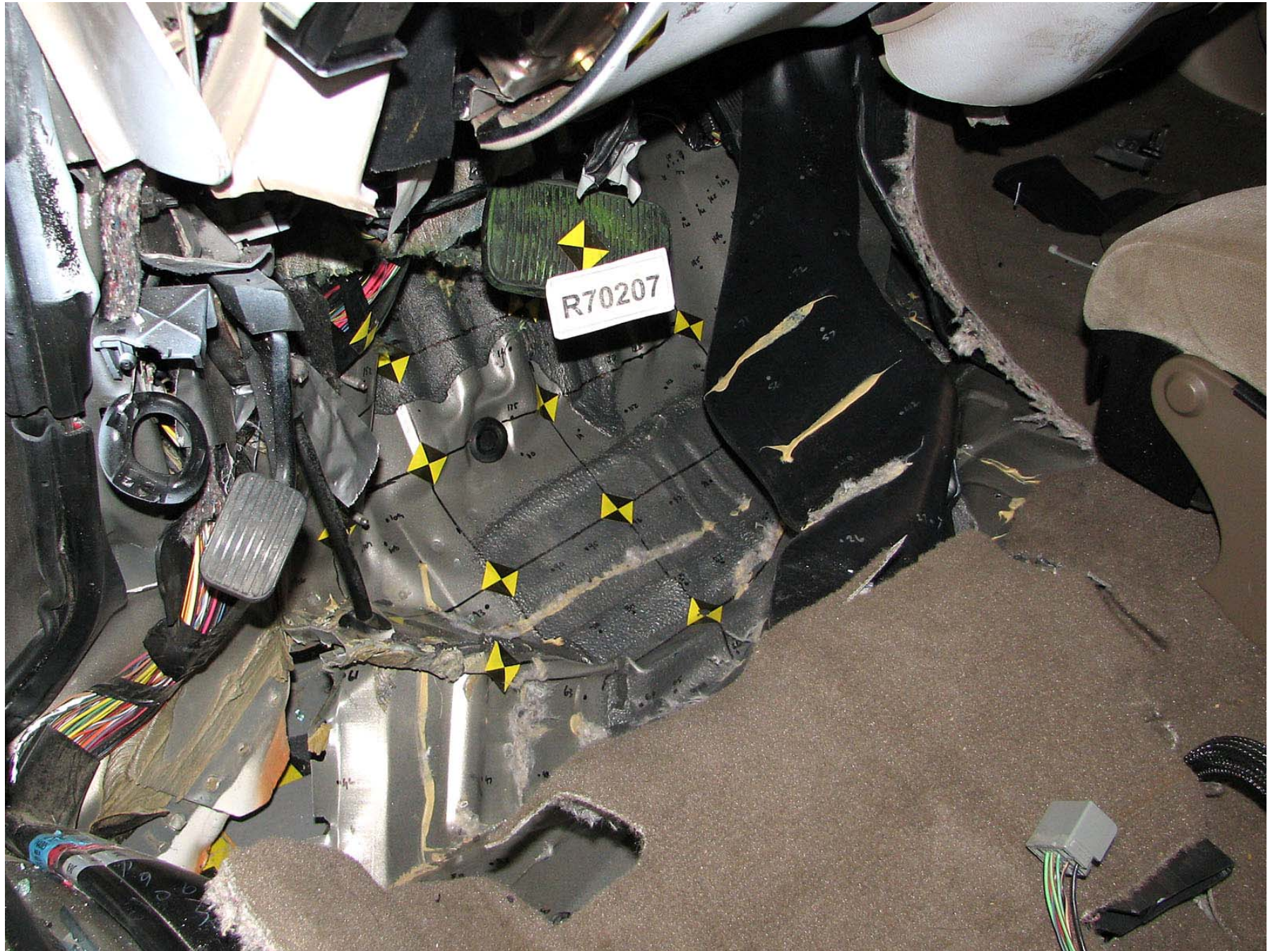
Figure A-286: Test Vehicle Post-Test Driver Floorpan
